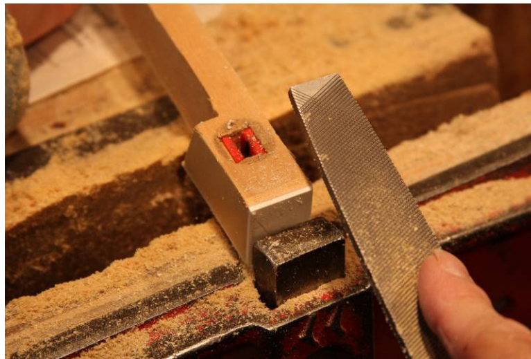
Photo 8: Finishing the bottom of the keyfront.
