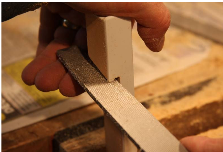
Photo 6: Finishing the notch.
