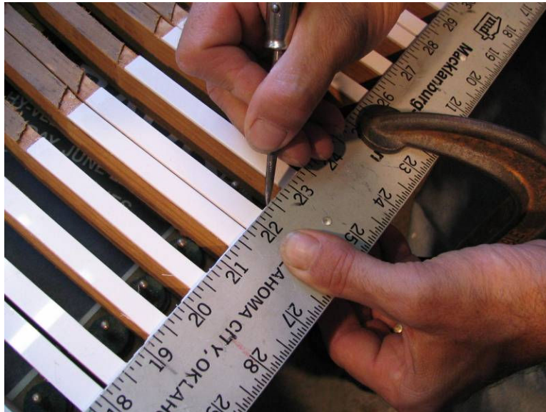
Photo 3: Making a scratch line
