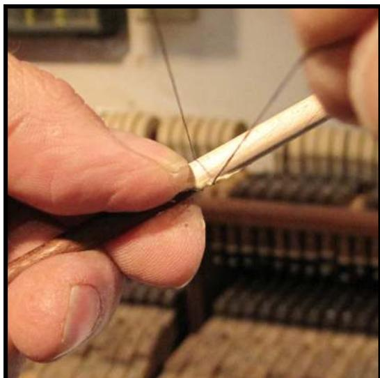
**Step 15:** Start your winding by wrapping the thread up and over the splice just above where you are pinching the two halves of the splice together. Make three tight windings going in the direction **away** from your left hand.
