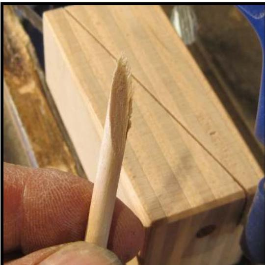
*The matching gluing surface on the new splicer. One convenient thing about using the hammer shank miter box is that you never need to worry about the angle to cut. You will automatically have matching surfaces to work with.*
