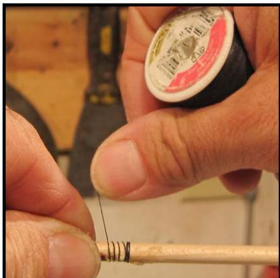
**Step 14:** Position the spool of thread in your right hand as shown in the photo so that you may unwind as much thread as you need as you wrap the spliced shanks. Unwind an adequate amount of thread to work with, then grip the spool tightly to keep the tension on the thread.
