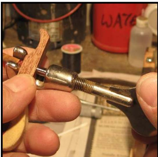
**Step 30:** Use a [grand shank press \(Cat. No. 131\)](#) to extract the old stub. To do this, remove the hammer head from the vise, and place it in the press as shown with the point of the plunger lined up with the hole that you marked in the top of the shank. Carefully steam the glue joint where the shank is inserted, then begin turning the screw down.
