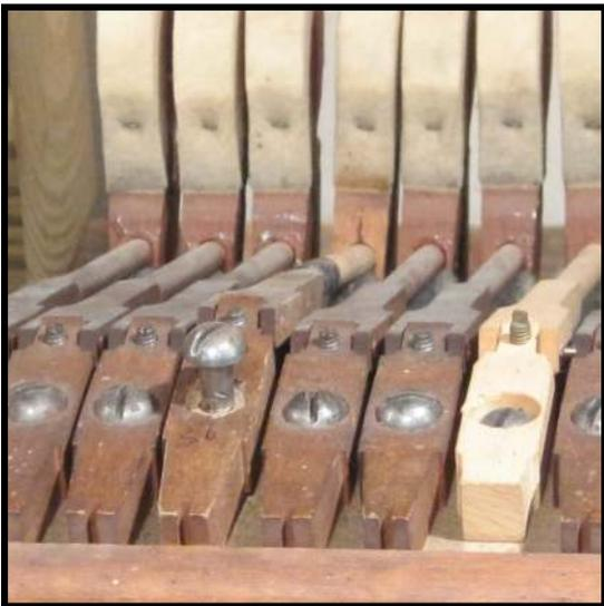
**Step 40:** To finish marking the reference lines for gluing, put the shank in place with the hammer attached (but not yet glued). Tighten the flange screw down, checking to see that the shank is parallel to its neighbors, then pivot the hammer to the right or left until it is correctly aligned.
