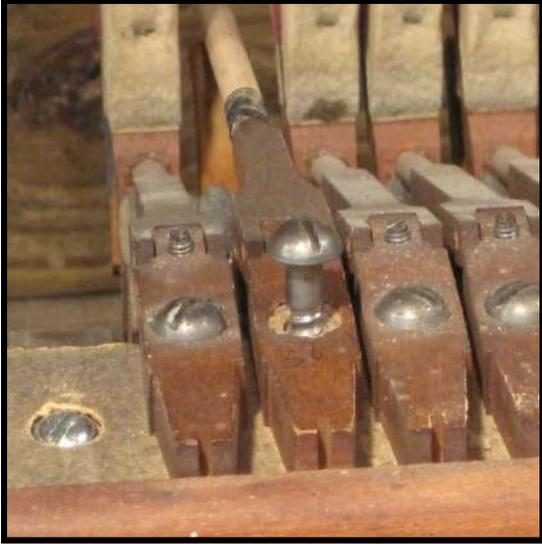
**Step 26:** To cut the new shank to the approximate length, first screw the flange back in place. It takes just a few extra seconds, and will insure that the flange and shank stay put and that you cut the shank at the correct spot.
