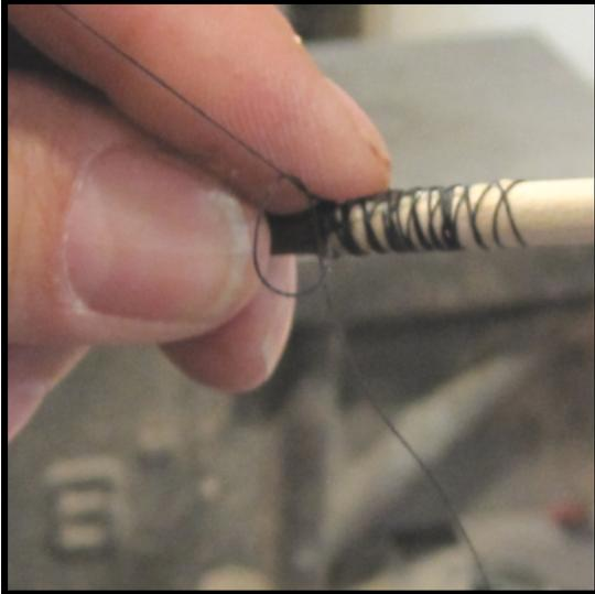
**Step 22:** With the first knot tied tightly, maintain the tension with the segment held in your teeth while holding the juncture in place with your thumb. Knot the thread two more times for insurance.
