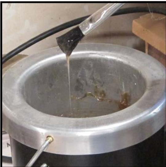
*Hint: Check your glue before applying to the shank and hammer head. It should be fairly runny (but not watery), with no evidence of unmelted crystals in the mix. Add a bit of water, or a few more crystals to obtain the correct consistency as needed. Allow a few more minutes to come back up to correct temperature, or for new crystals to melt..*
