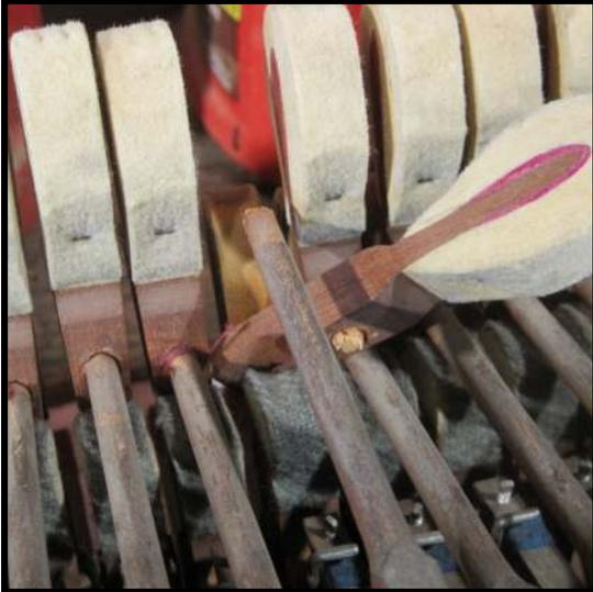
*Note: This type of break necessitates either replacement of the shank, or splicing in with a segment of new shank.. In the case of this particular piano, a new set of shanks and hammers were recommended and were slated to be installed at a future date. For the time being, however, repairing the piano to work was the order of the day. A simple splicing of several broken shanks was recommended as an temporary measure so that the piano might be played again.*
