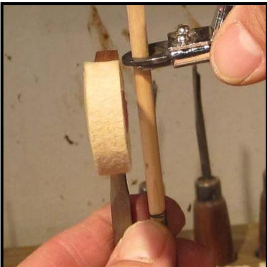
**Step 28:** Using a pair of [hammer shank cutters \(Cat. No. 237\)](#), snip the shank a bit long. Once the hammer is glued in place, the excess shank will be further trimmed and filed flush with the tail.
