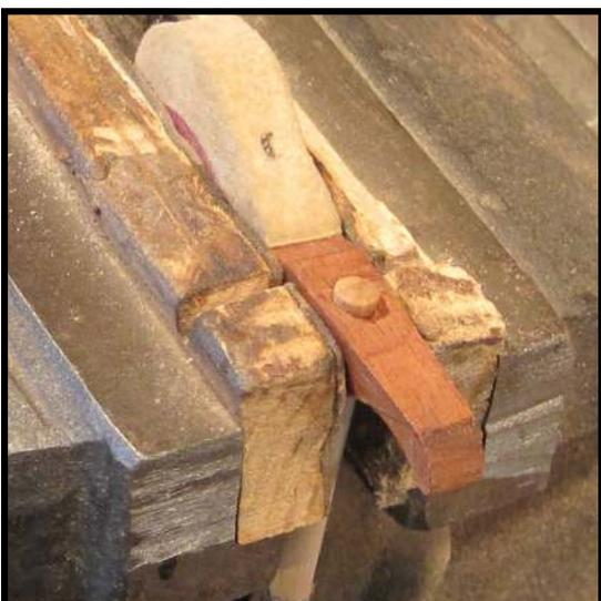
**Step 48:** After the glue has cured, remove the assembled shank and hammer and place the hammer in the vise once more in order to trim off the excess shank.
