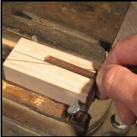
**Step 5:** Begin the repair process by gauging the amount of shank to insert into the miter box. Hold the shank along a line drawn on the box to represent the alignment of the hole. Make sure the entire break will lie beyond the cut line in the box. Grip the shank at the point to which the shank needs to be inserted.
