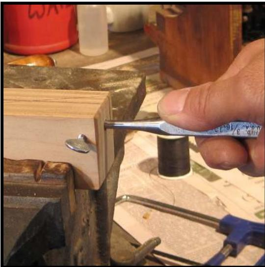
**Caution:** *Before proceeding any further, clear out the hole in the miter box. If the left over stub doesn't fall out, use a blunt ended punch to tap it out. If you forget this step, you'll likely have a "log jam" develop at some point, when the split end of a shank, and the tapered end of a sawed off shank get jammed together. If this happens, you'll most likely need to drill the hole out again.*
