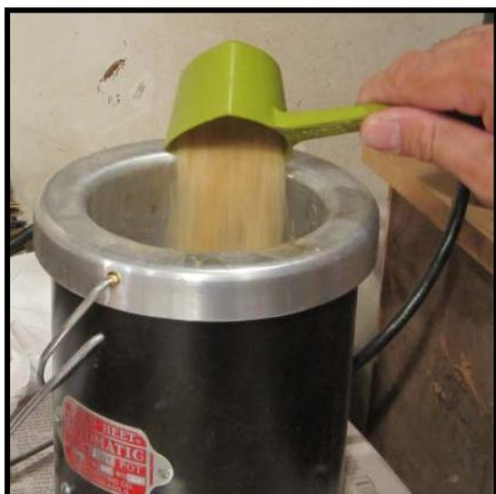
**Step 33:** If you intend to use hot animal hide glue in gluing the hammer to the repaired shank, now would be a good time to prepare the glue. I would recommend the [Hold-Heet Electric Glue Pot \(Cat. No. G-1155\)](#), used along with [dry cabinet glue \(Cat. No. 399-12\)](#). For this type of job, you only need to prepare a very small batch. Simply mix the glue crystals with water, and plug the pot in. Stir occasionally to maintain an even consistency.
