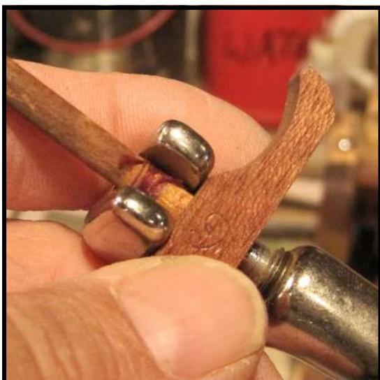
**Step 31:** As you turn the screw of the press down, you should feel the shank give way and begin to move. Watch underneath the hammer for evidence of the old shank emerging from the hammer head. On an old hammer and shank, the emerging shank will be lighter in color.
