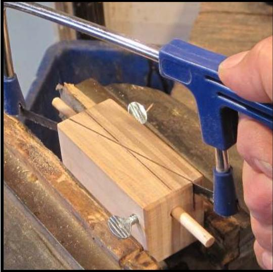
**Step 9:** Taking a new hammer shank, insert it into the miter box for cutting. Unless an extra long segment of shank is needed for a splice close to the flange, you can usually cut the shank at its center to produce two splicing shanks for use.
