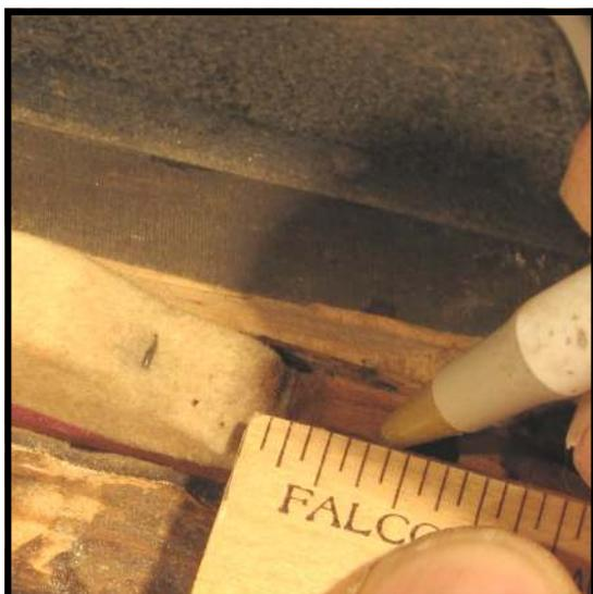
**Step 38:** If you wish to have a useful reference to use during gluing, draw a line on the underside of the molding bisecting the shank hole.
