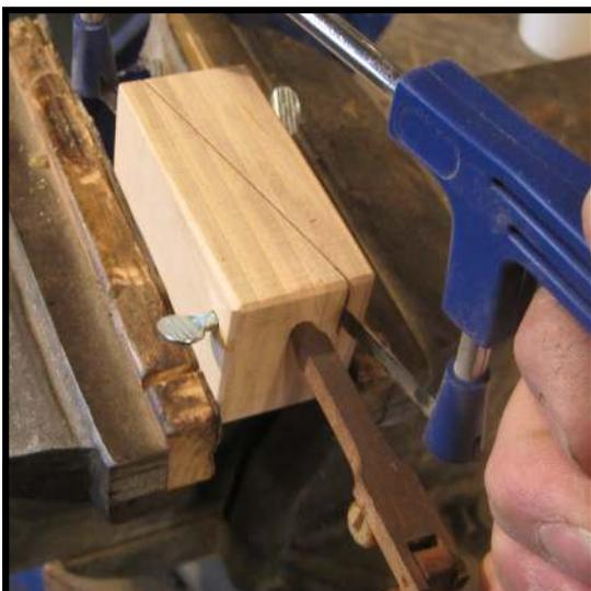
**Step 7:** Using your Handy Hacksaw, cut through the shank with even strokes. You'll feel the blade drop in the slot slightly when the shank has been sliced all the way through.
