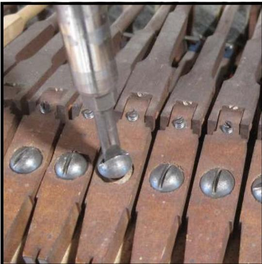
**Step 1:** Remove any broken shanks from the action. Number the flanges, if more than one shank is involved. Locate the broken off hammers. If several shanks close together have been broken off, match hammers to shanks by examining the broken ends. Number the hammers before going any further to avoid confusion.
