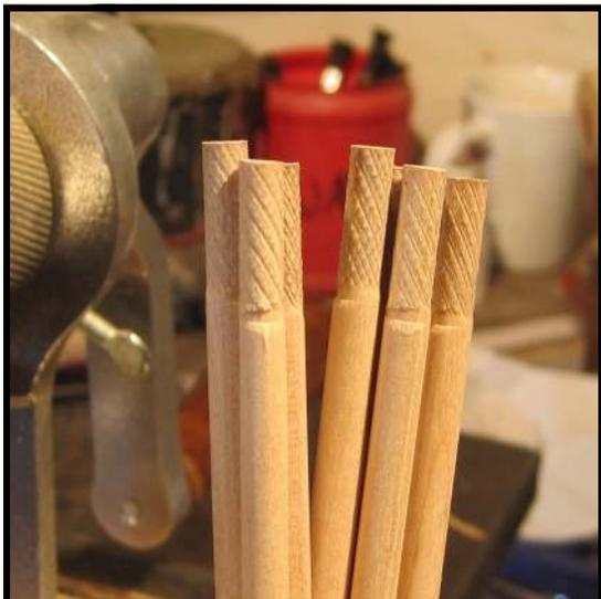
*Note: Using the hammer shank knurler results in an evenness of results that is hard to achieve with the file rolling technique. It is especially useful on complete hammer replacement jobs, where every shank needs to be accurately knurled. For more complete information, refer to the article "[Using the Hammer Shank Knurler - Basic Tips](#)," which will be available soon for download on your Schaff eStore.*
