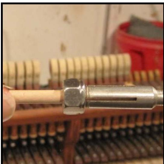
**Step 35c:** Instead of knurling hammer shanks, a correct fit may also be obtained by using a [hammer shank reducer](#), (Cat. No. 75) along with a [combination tool handle](#), (Cat. No. 26).
