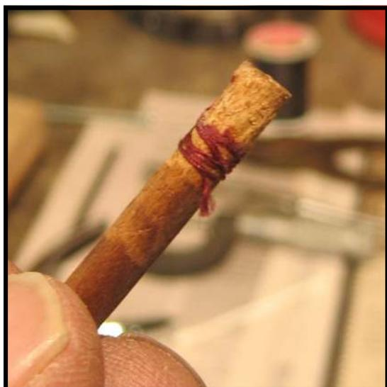
*Note: This photo explains a lot about past work done on the instrument. The hammers on this piano are replacement hammers, and are lightly worn. They are bored, however, for a .204" shank, while the original shanks only measured .199". The thread helped obtain a tighter fit.*
