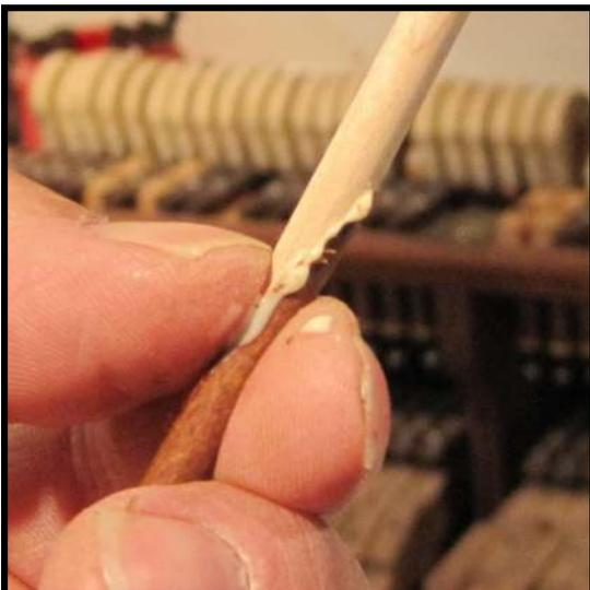
**Step 12:** Hold the joint tightly together at approximately the half way point with your left hand, pinching the joint with your thumb and forefinger. Double-check alignment.
