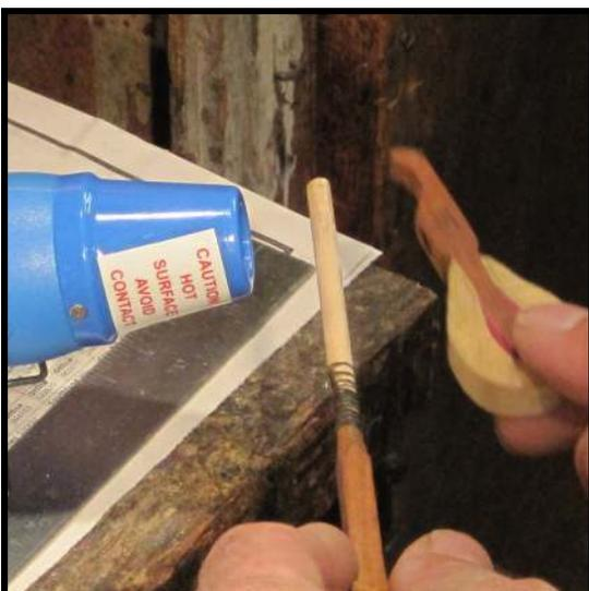
**Step 43:** Preheat the end of the hammer shank, and the tail end of the hammer surrounding the hole. The [Ungar Heat Gun, \(Cat. No. 416\)](#) works well for this process. Gently wave the hammer and the shank back and forth across the stream of hot air, until they are noticeably warm to the touch. This step will help prevent the glue from gelling too quickly, giving you a bit more time to align the hammer precisely once it is returned to the action.
