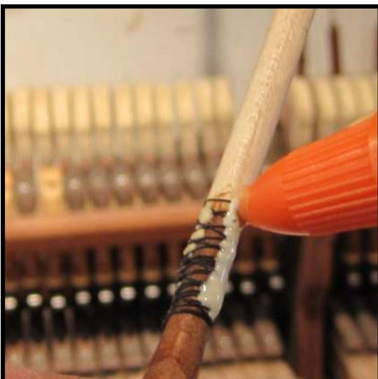
**Step 24:** If you intend on leaving the wrapping on the shank, spread a bead of Titebond glue across the windings.
