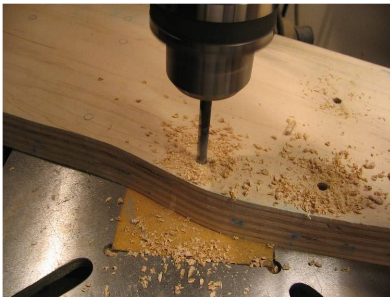
Photo #3: Drilling the pilot holes for the plate screws
