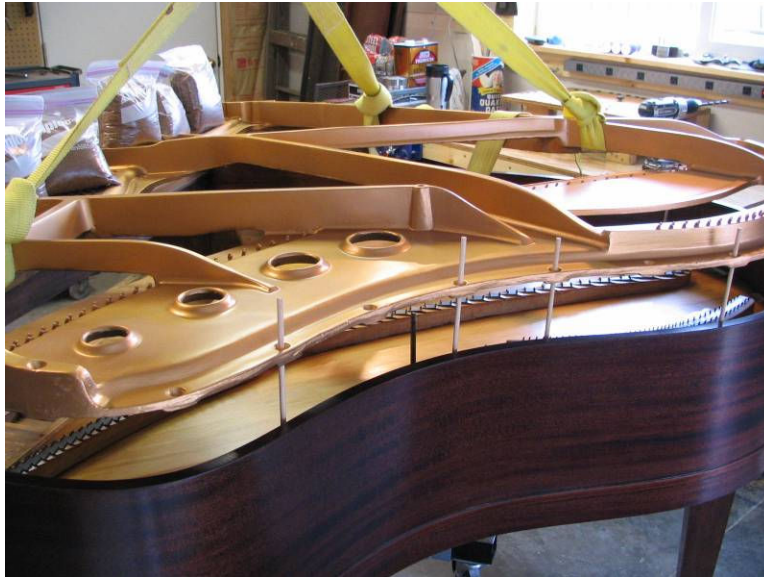
Photo #11: Guide dowels help lower the plate safely
