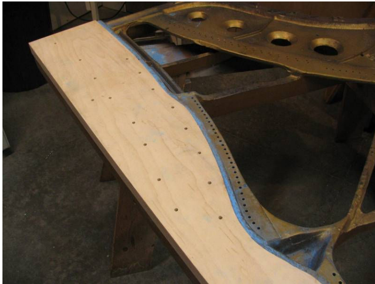
Photo #4: Pinblock back in place with plate screw holes drilled
