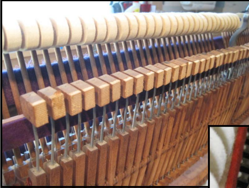
Once all the dampers have been removed, and the damper blocks have been reinstalled, it is time to return the action to the piano.
