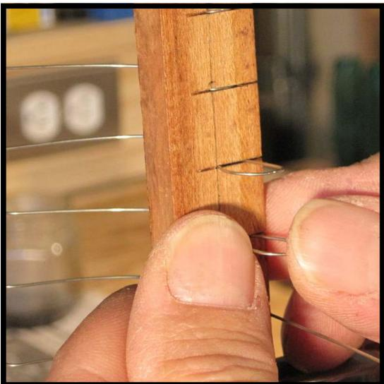
**Step 26 :** Working with three to six springs at a time, insert the tails, then turn the rail over to push the end of the tails through the new holes in the rail. Use your two thumbs as shown to accomplish this process quickly
