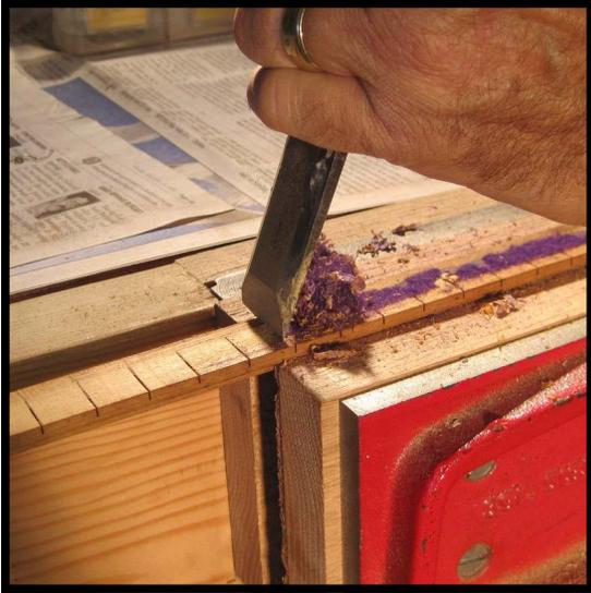
**Step 10 :** Use a sharp 3/4" or 1" wood chisel ([Chisel set - Cat. No. 292](#)) to scrape the felt remnants from the rail. With the flat side of the blade towards you, pull the edge of the blade over the rail in a scraping motion as shown.
