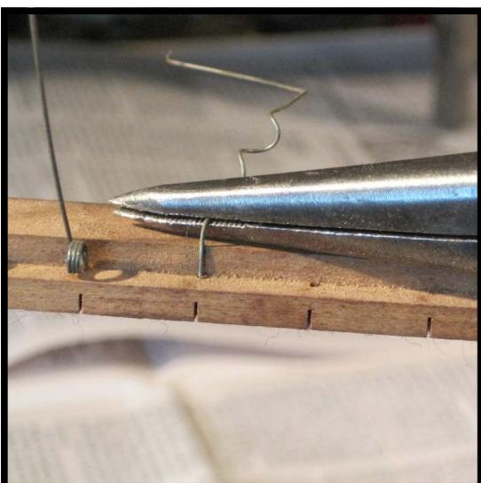
**Step 6 :** Reposition your pliers to grasp the spring directly over the rail. With the spring held tightly, turn the pliers clockwise. The spring should begin to slide from the hole in the rail.
