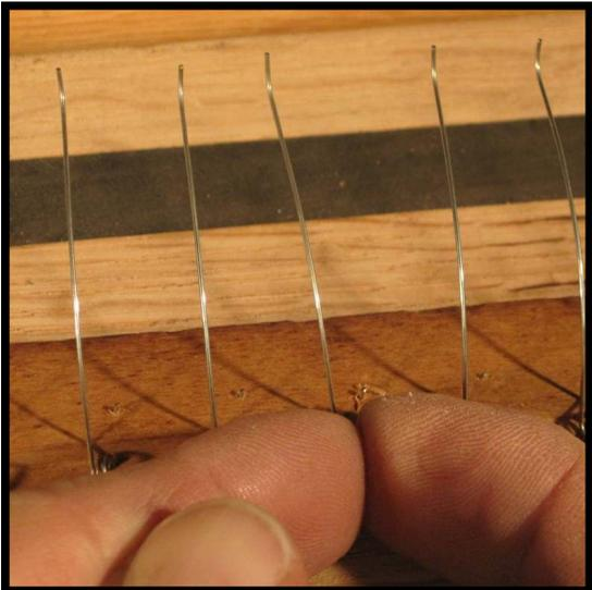
**Step 31:** Side-to side misalignment may be corrected by pinching the coil of the spring in between the forefinger of either hand. Press inwards on the coil from both directions, but slightly harder on the side opposite to that you wish the spring to move in the direction of.
