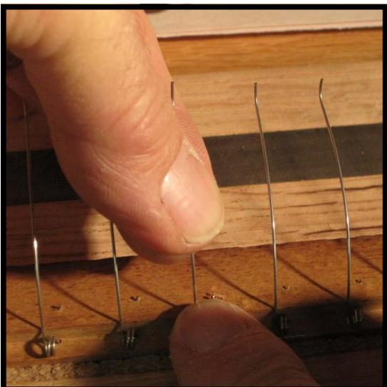
**Step 32:** Correct the slant forward or backward by "massaging" the spring. Hold the coil firmly in place with the forefinger of you right hand, while pulling upwards on the spring itself with the thumb and forefinger of your left hand. As the wire of the spring slides between your thumb and forefinger, encourage it to go downwards or upwards, according to the direction desired.
