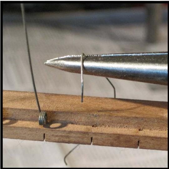
**Step 8:** When the end of the spring pulls loose from the rail, discard and go on to the next spring.
