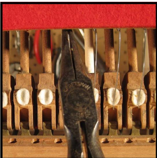
**Step 43:** If a spring is not aligned (such as the left hand spring in photo 42), grasp the coil of the spring with your needle nose pliers and twist in the desired direction.
