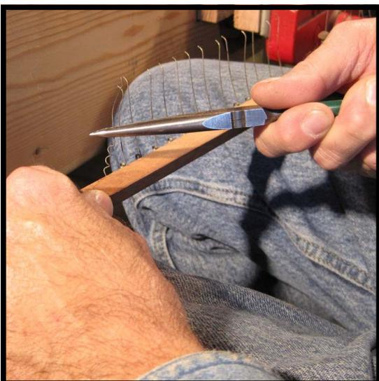
**Step 3 :** Remove the old hammer butt springs. Holding the rail in your lap, as shown, use a pair of [needle nose pliers \(Cat. No. 239\)](#) to pull the old springs free. The following directions will help you avoid having springs break off in their holes.
