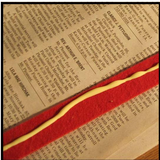
**Step 34:** Run a bead of glue along the strip of spring rail felt. Spread the glue evenly over the surface. If necessary, make a second application to complete the coverage.
