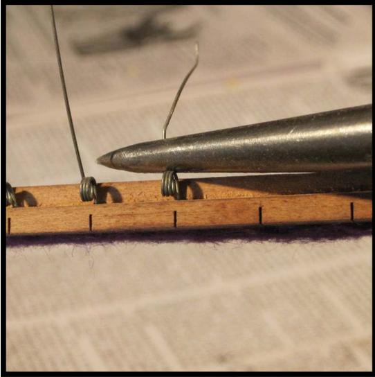
**Step 4 :** Use the pair of needle nose pliers to grasp the old spring directly over the coil. (Photos taken with rail on bench for sake of clarity.)
