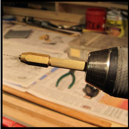
**Step 15:** The pin vise may be used in either a hand-held electric drill, or a drill press. Before using, make sure that the bit is centered by turning the drill on and observing the point of the bit. If not centered, the bit will need to be re-chucked, to avoid breakage.
