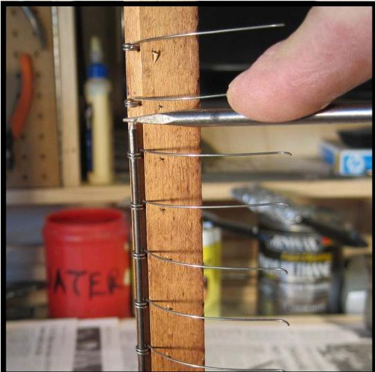
**Step 29:** As the process continues, use a [jeweler's screwdriver \(Cat. No. 3275\)](#) to push the coat hanger wire through a new set of wires and repeat steps 25 - 28. Move the rail upward in the vise as you move downward in the installation of the set of springs.
