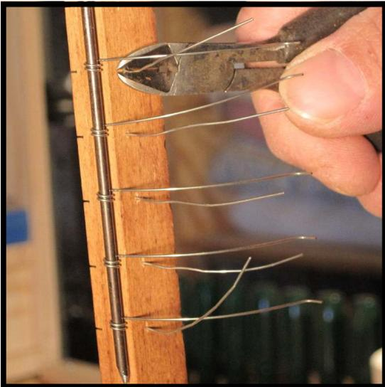
**Step 28 :** Once all the tails are pulled tight, snip the excess of each tail.
