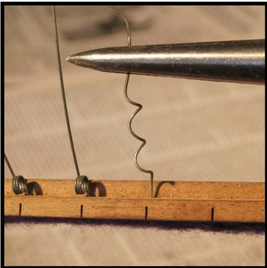
**Step 5:** Gently pull upward on the coil, somewhat straightening it out as shown.
