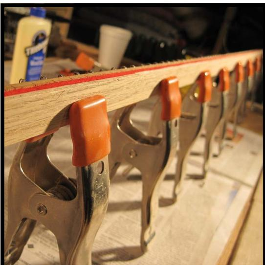
**Step 37:** Clamp along the center of the gluing block every 6 inches. Double check to make sure that the felt hasn't slid out of place. Set the clamped rail to dry on the bench as shown.
