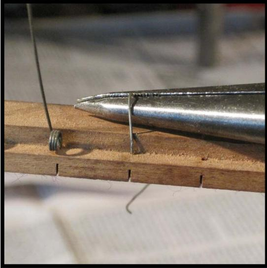
**Step 7 :** Continue to slowly turn the pliers clockwise, keeping the side of the tool in contact with the rail. Avoid any type of yanking motion which would likely snap the spring, leaving the hole plugged.
