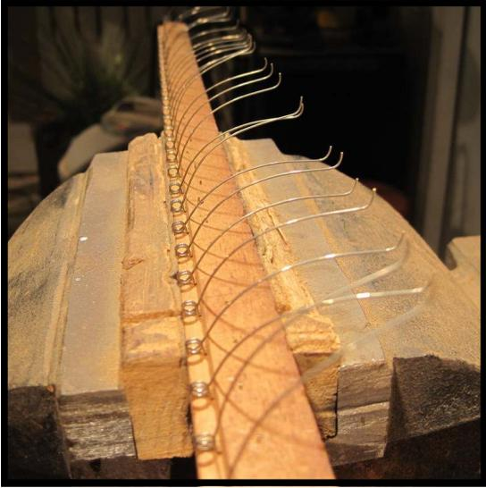
**Step 30:** Once the entire set of new hammer butt springs has been installed, place the rail in a vise with the springs pointing up and away from you as shown. Make sure that the spring coils are up above the jaws of the vise. Unless you have been fine-adjusting the orientation of the springs as you've worked, your set will probably look something like the set in the photo, with springs going at odd angles to each other. This should be corrected to ensure uniform tension.
