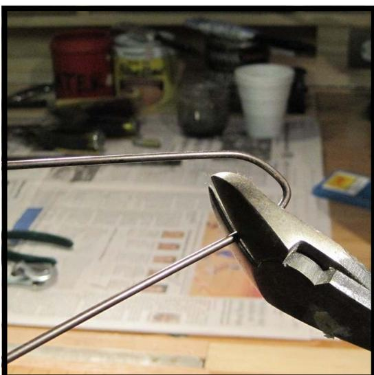
**Step 17 :** Taking an ordinary wire coat hanger, cut off a section of the long end of the hanger to use in the next steps. The diameter of the coat hanger wire should be such that the coil of the new hammer rail springs will free slide onto it.
