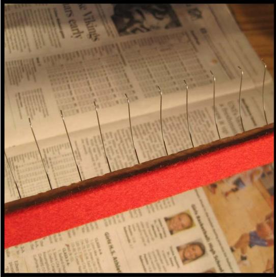
**Step 38:** After the glue has cured for at least an hour, the clamps and gluing block may be removed. If there is any glue squeeze-out between the felt strip and the wooden rail, remove with a sharp chisel.
