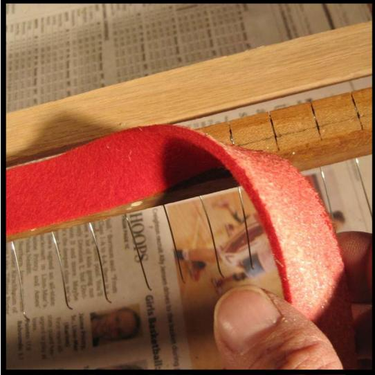
**Step 35:** Carefully stretch the spring rail felt on top of the rail itself. Flatten the felt out from the center toward the ends. Make sure that the felt covers the rail from side to side and is centered from top to bottom on the rail.
