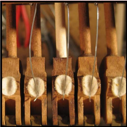
**Step 42:** With the springs positioned in the hammer butt grooves, check the orientation of each spring to make sure that they are not veering to one side or the other.
