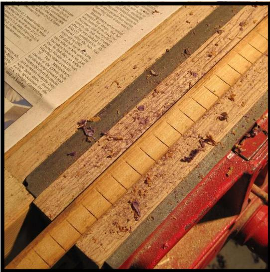
**Caution!** Move the rail from side to side in the vise as each section is scraped clean. Do not attempt to hold the rail with one hand, and scrape the rail with the sharp chisel with the other hand!
