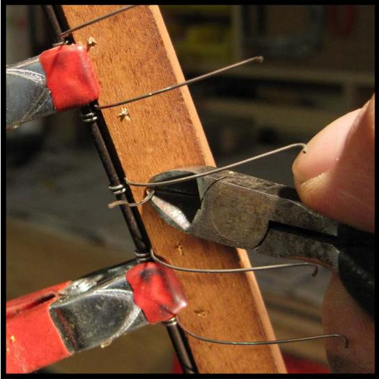
**Step 24 :** Use a pair of [center pin nippers](#) (Cat. No. 230) to snip off the excess flush with the rail.
