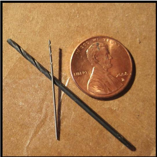
**Step 11 :** An ultra fine drill bit will be needed for the next step of the project. The size required is a [72 gauge drill bit, \(Cat. No. D-72\)](#) which has a diameter of .025". This size of bit is shown in the accompanying photo in comparison with a 1/16" bit, the smallest size found in most ordinary drill indexes. It would be a good idea to order several, in that they do break easily.
