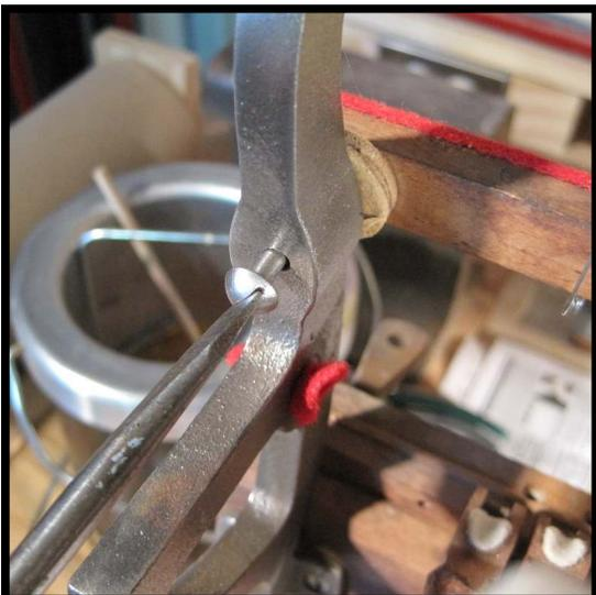
**Step 40:** The hammer spring rail is now ready to be screwed again to the action brackets. When returning the spring rail to the action, be careful not to bend any of the springs. Usually they will fit in between the hammer shanks as the rail is brought into position. At this point, do not try to position the end of the springs in the felted grooves in the hammer butts. If punchings were originally used to shim the rail out away from the brackets, either return or replace those.
