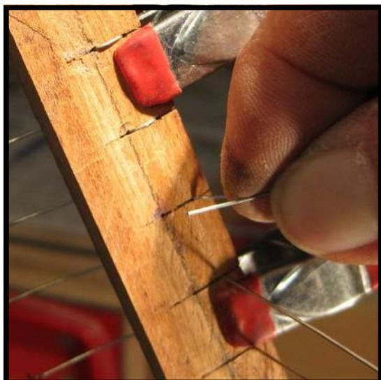
**Step 22 :** Turning the spring rail over, grasp the tail of a spring and bend it in towards the new hole that has been drilled. Try to bend the spring in a half-loop, and not a sharp bend. Push the end of the tail through the hole as far as possible.
