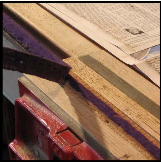
**Step 2 :** Remove hammer butt spring rail from piano action, and strip the spring rail felt from the back side of the rail. Don't scrape the remnants of the felt from the rail yet.
