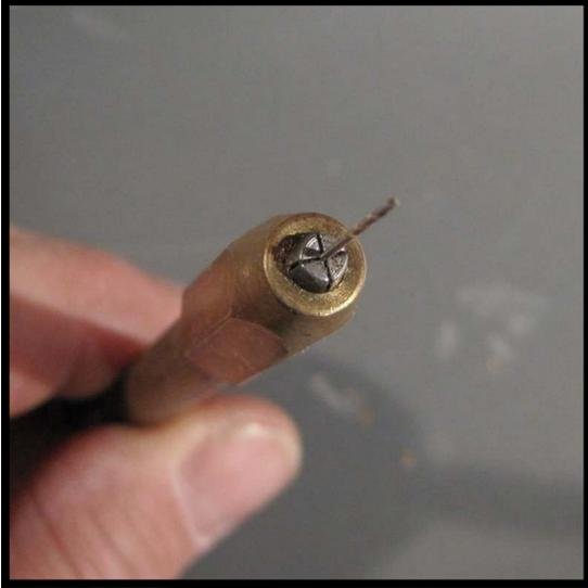
**Step 12:** One tool commonly available which will hold this size of drill bit is a [pin vise \(Cat. No. 152\)](#), or [double ended pin vise \(Cat. No 149\)](#). Another option would be to use a [Dremel reducing collet \(Cat. No. D-483\)](#) in a [Multi Pro \(Dremel\) Tool \(Cat. No. D-275 \[single speed\] or D-395 \[variable speed\]\)](#).
