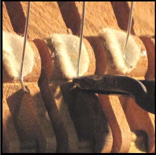
**Step 44:** If the hammer springs are a bit too long, they may be trimmed and re-shaped on the end. First, use your pair of center pin nippers to snip each spring at the very bottom of the corresponding spring punching.
