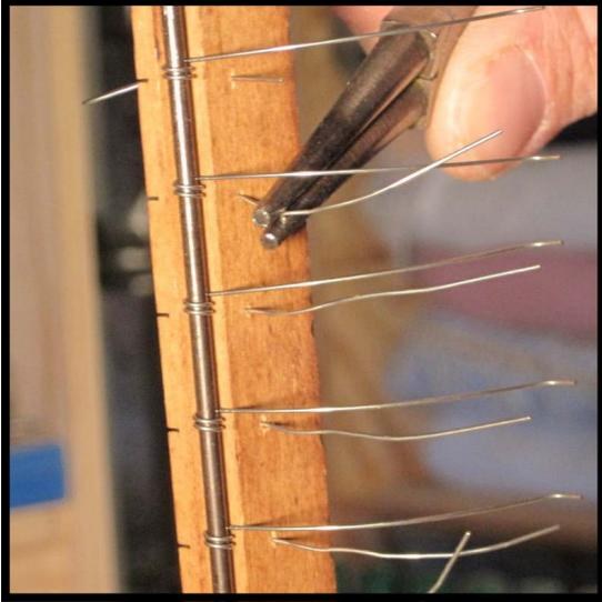
**Step 27 :** Turn the rail back around again, and pull the excess through for each spring, working from the bottom to the top. Pull the springs tightly, but not so firmly that the tails break off. If you feel the loop as it tightens on the other side of the rail, you should be able to feel the wire seat itself in the slot.
