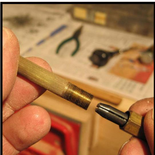
**Step 14 :** If a double end pin vise is to be used, remove the collet and holder from one end of the vise, and set aside for the time being.
