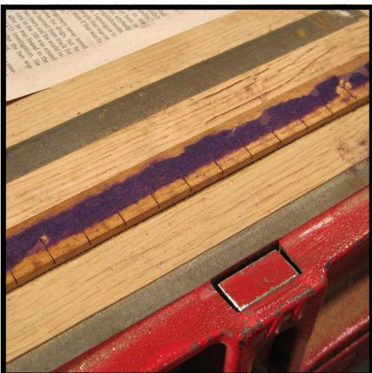
**Step 9:** With all the springs removed, place the rail in your vise in order to scrape off the remnants of the spring rail felt from the backside of the rail.
