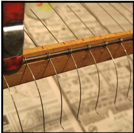
**Step 21:** Once a initial section of springs have been anchored with the coat hanger wire, secure the end opposite the rubber band with a small clamp.
