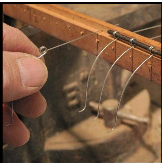
**Step 20 :** Continue on with this process until you have a dozen or so springs held in place by the coat hanger wire.
