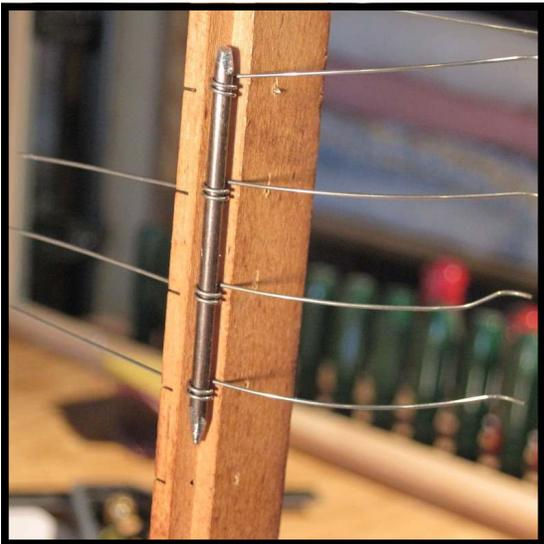
**Step 25 :** Once the first springs have been installed, the process may be sped up by putting the rail up and down in a vise, and by sliding a short segment of coat hanger wire down through the coils as the process continues. A short segment of wire, extending through four to seven coils, will be easier to slide along than a long segment of wire. As long as at least one coil holding the coat hanger wire has been pulled tight, this technique will work.
