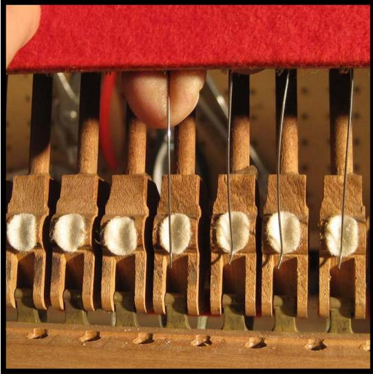
**Step 41:** To perform the last few steps of fitting and adjusting the hammer springs, it is best to remove the dampers and damper levers, number them and set to one side. With the dampers out of the way, you may easily push each spring forward to position it in the groove of the hammer butt.
