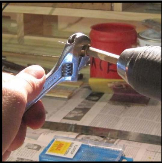
**Step 13 :** If you do chose to use a simple pin vise, tighten the collet down firmly on the bit by using an [adjustable wrench \(Cat. No. 3200\)](#).
