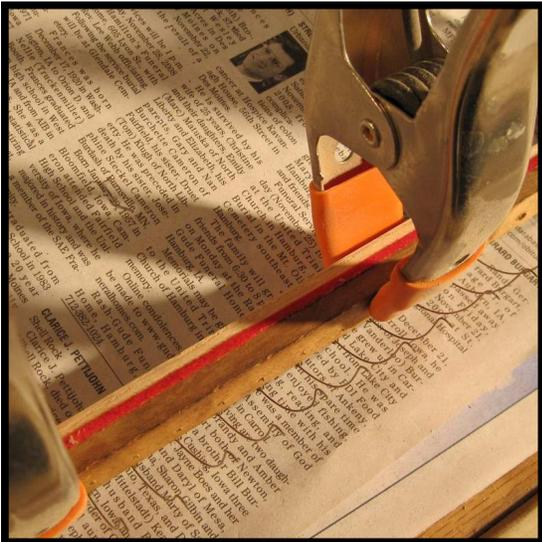
**Step 36:** Place the gluing block over the felt and use a [key spring clamp \(Cat. No. 247\)](#) on the side of the rail opposite the spring coils to hold it in place.
