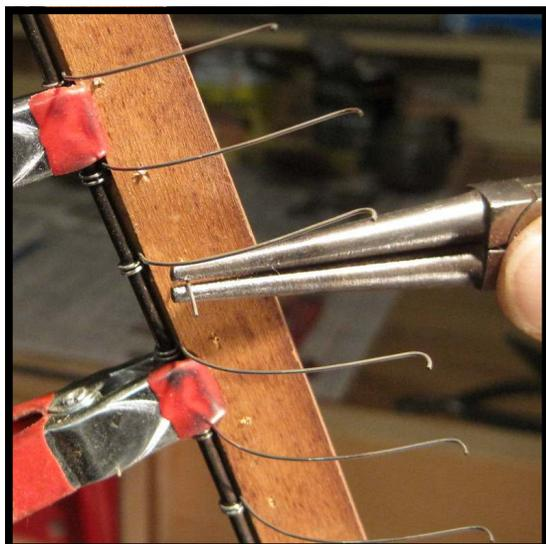
**Step 23 :** From the front side of the rail, grasp the end of the tail of the hammer spring with a pair of [round nose pliers \(Cat. No. 241\)](#) or needle nose pliers. Pull the slack out of the tail, then complete the process by grasping the tail again next to the rail and use the pliers as a lever against the edge of the rail. You will see the segment of coat hanger wire pull up firmly in the dado slot as the slack is completely removed.
