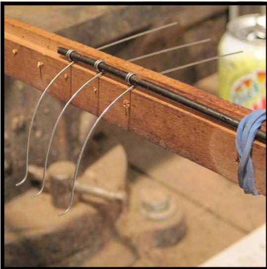
**Step 19 :** Begin the process of installing the new hammer butt springs by sliding the tail of the first spring through the original hole in the rail. With the coil of the initial spring in the dado slot, push the end of the coat hanger wire through the eye of the coil. Insert the tail of the second spring, and repeat the process. For this starting section of springs, use a rubber band to keep the coat hanger wire in place as it is pushed along the slot.
