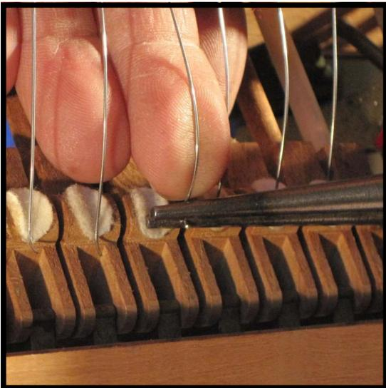
**Step 45:** To reshape the end of the spring, hold the bottom of the spring firmly with your pair of round nose pliers. Then, while pushing forward on the lower portion of the spring with the middle finger of your left hand, turn the round nose pliers slightly clockwise to put a partial bend in the very bottom of the spring.
