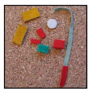
The Choice: In this instance, the choice was made to restore the original parts. There was a slight difference in the placement of the catcher shanks which would cause a slight difference in the geometry of the action. The desire to keep as much of the piano as original as possible was also a factor. The felts and leathers pictured are what's replaced in this type of restoration. Following are step-by-step procedures to complete this repair.
