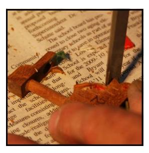
**Step 7:** Turning the hammer over to the opposite side, use your chisel to slice off the hammer butt felt with one clean stroke.
