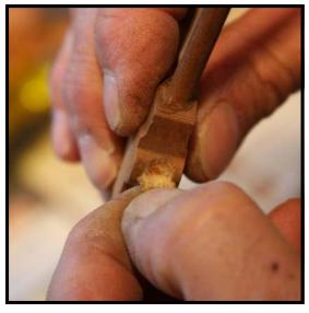
**Step 12:** Peel the old spring punching from the groove on the back of the hammer butt. Clean out any residue with a rat tail file
