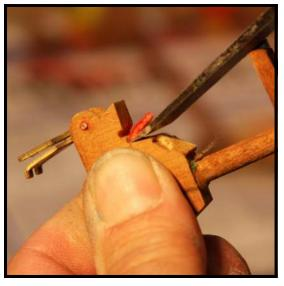
Step 9: Use your 1/2" chisel one last time to remove the piece of underfelt nearest the flange. Turn the chisel so that the bevel is down, and rock it back and forth slightly as you push to cut the felt loose. (Note: On some pianos this felt will not appear to be glued in place, and will simply fall out when the buckskin is removed.) Use the chisel turned on edge to clean any residue from the corner.
