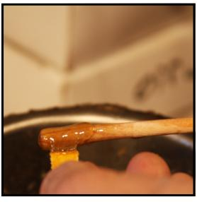
**Step 30:** Apply a small amount of hot glue to the correct end of the hammer butt buckskin using a hammer shank as an applicator. Make sure you have glue on both sides and on the very end of the piece of leather.
