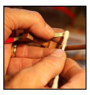
Step 19: Insert the bridle strap through the hole in the catcher. Holding the hammer butt as shown, with your middle finger supporting the end of the strap, apply a drop of Titebond glue (Cat. No 392-4). A small amount put in a bottle cap, then applied with a Q-Tip, makes for less mess than using out of the squeeze bottle.
