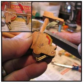
Step 33: With the squared off end of your coarse file, push the buckskin up towards the catcher shank. The teeth of the file will grip the leather, and you will see the leather stretch over the underfelts as you firmly push upward. Hold the buckskin in place for a slow count of 10, then release. If the consistency of the glue is correct, the buckskin will stay in place. Use a small rubber band around the body of the hammer butt to clamp the end of the buckskin while the glue cures.
