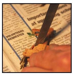
**Step 6:** The last step with the hammer butt oriented this way is to slice down between the hammer butt buckskin and the beveled corner of the hammer butt next to the catcher shank. The buckskin is stretched, not glued, over the two pieces of underfelt, and will come loose from them once the corner edge is sliced free.
