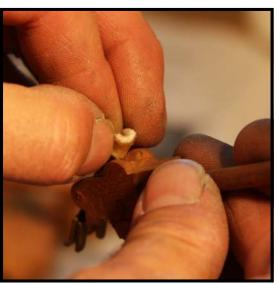
Step 23: Before the glue is allowed to cool, hold the felt between your thumb and third finger, and push together slightly to pucker it outward. Insert into the spring groove on the back side of the hammer butt. Push into place.
