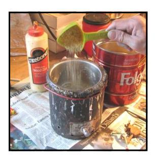
Step 13: With all the felt and leather removed from the hammer butt (the center pin bushings were not replaced on this particular piano), it's now a good time to prepare for installation of new materials used in restoring the hammer butt. First, a small batch of hot animal hide glue should be prepared, using an electric glue pot (Cat. No. G-1155), and dry cabinet glue (Cat. No. 399-1/2). Use slightly more water than glue for the correct consistency.
