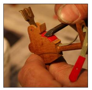
**Step 27:** Apply glue to the second piece of underfelt and position into place. It should fit snugly up against the edge of the slot which is intended for the end of the hammer butt buck skin. Use the flat end of your small screwdriver to tamp it down. Clamping is not required.
