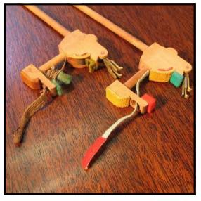
Before and after: With hammer butts outfitted with new leather and new felt, regulating the action for consistent response is a much more attainable goal. A job well worth the time and effort.
