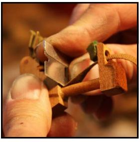
**Step 3:** Holding the hammer butt assembly by the hammer shank with the hammer butt up, cleanly cut the end of the bridle strap by rocking a sharp razor back and forth over the catcher shank flush with the body of the hammer butt.
