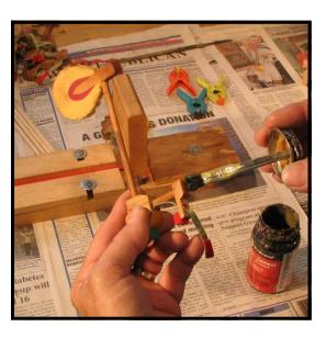
Step 34: Cut catcher buckskin approximately to size. Apply contact cement to both the catcher and the buckskin and allow to sit for at least 15 minutes, or until tacky. An alternate method is to clamp together a number of hammer butts with the catchers in line and to glue a strip of buckskin over the catchers from one end to the other.
