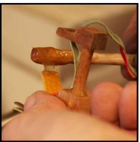
Step 32: After the glue has set on the end of the buckskin inserted into the slot, apply a small amount of hot glue to the other end, on the inside edge only. (The glue will work best for this step if it is a little less runny than before.) Attach the glued end of the buckskin to the beveled wood of the hammer butt closest to the catcher shank. Go immediately to the next step.
