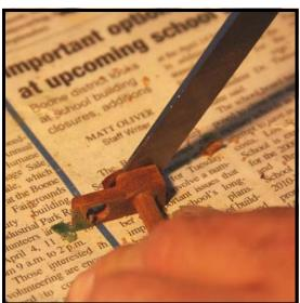
Step 5: Without putting your chisel down, proceed to the removal of the catcher buckskin. Start from the back, working from the corner down. Try to keep the flat edge of the chisel against the wood of the catcher as you shave the leather off. This takes one or two strokes of the chisel on the flat end of the catcher and one more stroke straight downward on the curved end. You will be left with a small amount of leather residue to file off.
