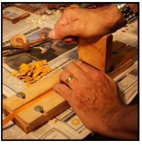
Step 15: Cut the replacement felts and leathers to the correct size using the Hale felt cutter (Cat. No. 279). To replace the buckskin on the hammer butts, use upright butt leather (Cat. No. 329B or 2350B). For the catchers, use upright catcher leather (Cat. No. 329A, or 2350A). The lower priced leathers are cow hide, and the higher priced leathers are actual deer hide.
