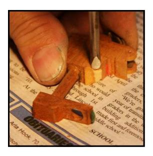
**Step 10:** Use either a small chisel, or a small, flat-bladed screwdriver that has been filed to a sharp edge to scrape out the underfelt in the recessed slot.
