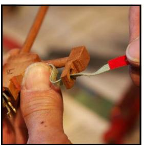
**Step 20:** Holding the end of the strap firmly in place for a moment, pull the excess of the bridle strap on through the hole in the catcher.
