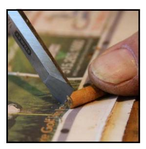
Step 2: If a stub of glue or wood remains on the end any of the hammer shanks, use a 1/2 inch chisel from chisel set (Cat. No. 292) to remove. The best method is to put the hammer shank flat on the bench, and to pivot the sharp edge of the blade, with the flat side in towards the end of the shank, across the surface of the wood. Use the bench to steady the corner of the blade as shown.
