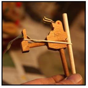
**Step 24:** Clamp in place using a hammer shank held in position with a small rubber band.
