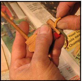
Step 35: At the point nearest the hole in the catcher for the bridle strap, press the buckskin and catcher firmly together. Push the buckskin up and over the hump and down upon the flat portion. The advantage of contact glue for this step becomes obvious here, as there is no difficulty in gluing up and over the bend in the surface of the catcher. The bond formed between the leather and wood is immediate
