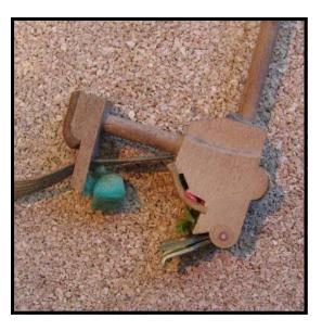
The Problem: Insect damage and wear would make fine regulating of the subject piano very difficult. Hammer butt felts were missing or damaged. The catcher buckskins were worn very thin, in places down to the wood. The most problematic situation was with the felts under the hammer butt buckskin. In places the underfelt was missing either partially or altogether. Plumping out with yarn would not be effective because of this inconsistency.
