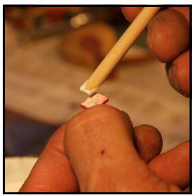
Step 25: Using a hammer shank flattened on one end apply PVC-E glue (Cat. No. 387-16) to the smaller of the two underfelts. The PVC-E glue will not harden as much as other glues, leaving the underfelt more resilient as a cushion.
