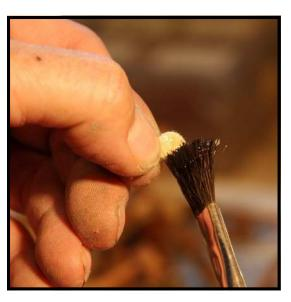
Step 22: Stir your hot glue again with the hammer shank. It should be the consistency of honey with the pot set at 160 degrees. Use a glue brush (Cat. No. 438) to apply a small amount of hot glue to a spring punching (Cat. No. 330E). If you're unable to grip the felt by the edge with your fingers, use the pointed end of a pair of needle nose pliers (Cat. No. 239) to grasp the felt while the glue is applied.
