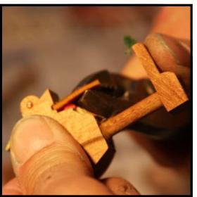
**Step 8:** Putting your chisel down and taking up a pair of ordinary pliers, grasp the hammer butt buckskin by the end, and pull it free from the notch which it is glued into. If any glue or leather remains in this notch use the flat end of a screwdriver from the mini screw driver and awl kit (Cat. No. 56) works perfectly to clean it out.
