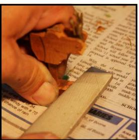
**Step 11:** Using a flat bastard, coarse cut 10" file (Cat. No. 252), clean off any remaining felt on the underside of the catcher and on the outer side of the catcher, where the catcher buckskin was removed. Be cautious not to remove any wood in the process.
