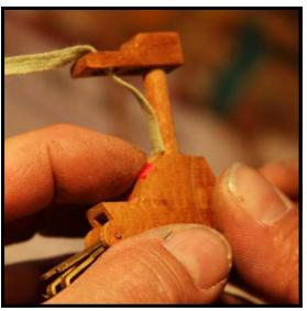
**Step 26:** The small felt should fit snugly into the groove in the hammer butt which is provided for it. Push it firmly into place. Wipe off any squeeze-out of glue.
