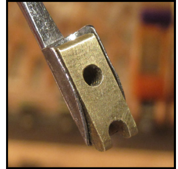
Replacement butt plate
