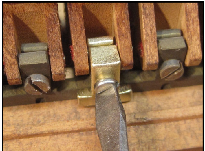
Repair clip for broken tongue being installed.
