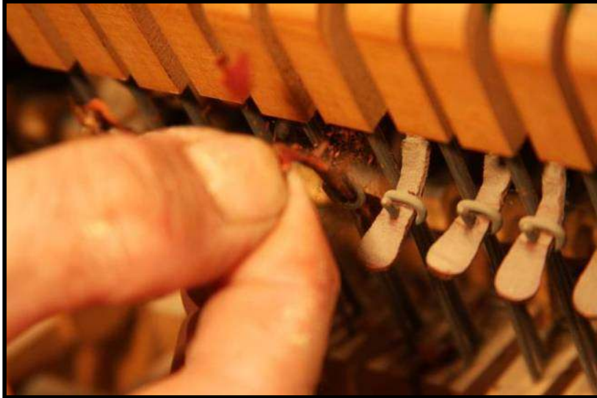
Photo 2: Factory tabs often crumble when pulled on.
