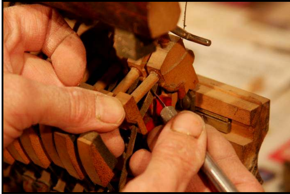
Photo 1: Cut the original straps between the catcher and hammer butt.
