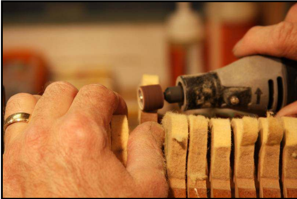
Photo 7: Dremel slightly tipped in to begin cut
