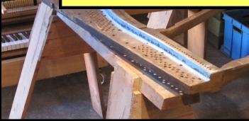
with a maner to snow where the high spots are. Obviously, the more care that was taken in the sawing procedure to match the profile of the flange, the less work will be needed at this stage of the job.
