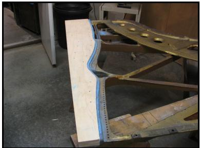
and drilling of the pinblock results in a perfect match of the new pinblock to the piano. A precision fit is essential for the tuning stability of the piano once the repairs are finished and the piano is returned to its home.
