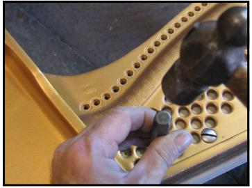
Once the pinblock has been successfully fitted to the plate, pilot holes for the plate screws are drilled, and the block is screwed down to the plate so that the pin holes may be marked with a punch. Once the pin holes are marked, the block is removed once again for drilling. (For certain instruments, the block may be drilled with the pinblock and plate installed in the piano.)
