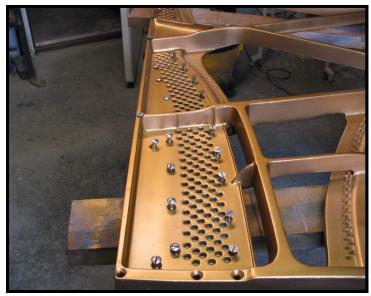
With the pin holes drilled, the pinblock is returned to the plate to be screwed down for good. A big advantage of a new pinblock is that new factory-size pins (usually .282" diameter) may be installed instead of oversized pins. This is important in terms of ease of tuning.
