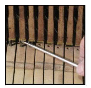
**Step 11:** Fine adjustments are made with the keystick in the piano. Turn the capstan up or down to produce the desired amount of lost motion.
