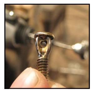
**Step 9:** Turn the capstan 360 degrees to inspect each inside corner.
