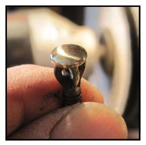
**Step 6:** Examine the surface carefully to make sure that you've removed all the tarnish and corrosion from the surface.
