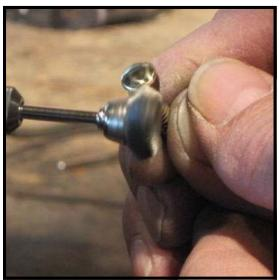
**Step 8:** Use the corner of the wheel to polish the inside corners of the wings.
