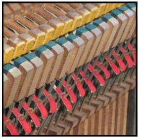
Step 12: To complete the fine adjustment, keep your eye on the backcheck as the key is pushed down with a light touch. There should be just a faint amount of movement of the backcheck before the hammer butt is perceived to be in motion. This slight amount of lost motion allows the jack to slip back unimpeded under the hammer butt in preparation for the note to be played.
