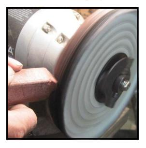
Step 4: Instead of a wire brush, a far better method is to use a buffing wheel (Cat. No. 452, 465 or 466) with a bar polish. Here the wheel is shown being loaded with Tripoli bar polish (Cat. No. 425), which works well on brass.
