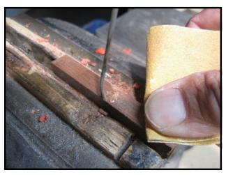
The lower surface of damper head is then scraped and sanded clean. The upper surface of the damper head may be cleaned and polished if the original lacquer finish is still in good shape. Otherwise, the old finish may need to be stripped off, so that a new lacquer finish can be applied (note-extra work =extra cost). A final step will be the polishing of the damper guide wires.
