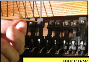
To access and remove the damper assemblies, the case will need to be disassembled to the extent that the action and keys may be drawn out of the piano. After removing the action from the piano, each damper will be taken out in order by loosening the set screw which holds the damper wire in place.
