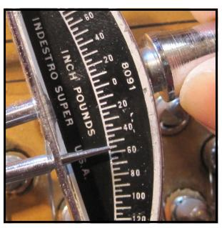
The above photos show torque reading measurements done on the same tuning pin before and after treatment was administered. In the photo on the left, the untreated pin measures just under 20 inch pounds of torque. After a single treatment the pin measures a much better reading of 55 inch pounds of torque.
