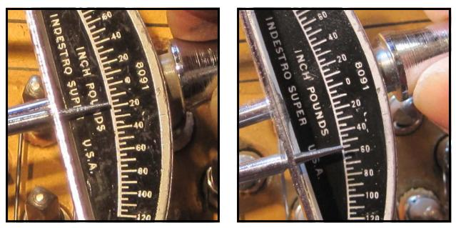
The above photos show torque reading measurements done on the same tuning pin before and after CA glue was administered. In the photo on the left, the untreated pin measures just under 20 inch pounds of torque. After a single treatment the pin measures a much better reading of 55 inch pounds of torque.
