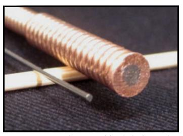
Cross sections of wires used for the highest and the lowest note on the piano, showing differences.
