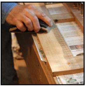
**Step 8:** With all the glue scraped off, finish the job with a sanding block and 60 grit sandpaper.
