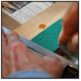
Step 14: Use either a felt cutting knife (Cat. No. 213), a square end knife (Cat. No. 216) or a single edge razor to cut the backrail cloth around the notches in the keyframe that fit around the supports for the action brackets. Either knife gives the advantage of an easy-to-grasp handle, that the razor blade does not have.
