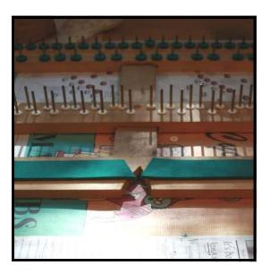
**Step 15:** With the backrail felt cut to fit on the keyframe, flip the felt over so that the underside is face up, and the front of the felt is now in the back.
