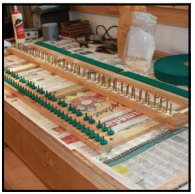
**Step 19:** Turn the keyframe back around in preparation for returning refelted frame to piano. If shims were removed from between the keyframe and the keybed in the disassembly process, return them to the correct position now and place keyframe back in piano.
