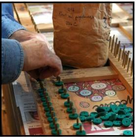
Step 11: After measuring the thickness of the old front rail punchings, select new punchings to install. Front rail punchings in white cloth, (Cat. No. 331), kelly green cloth (Cat. No. 335) and dark green cloth (Cat. No. 336 and 337) are available in two widths (3/4" and 7/8") and a range of thicknesses. If you do much of this work, you'll find that it's convenient to have a selection on hand to avoid having to wait to get to a job while supplies are ordered.
