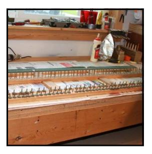
**Step 1:** Place keyframe on bench. Do initial vacuuming to remove bulk of debris.
