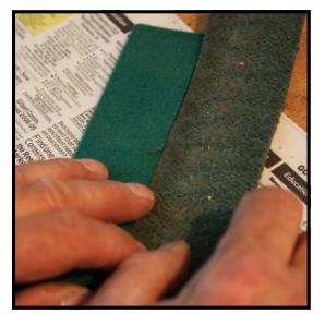
Step 13: Select the correct thickness of backrail cloth by comparing the thickness of the original cloth with the new. Lay a piece of the old side by side with the end from a new roll to determine which thickness is the best match.
