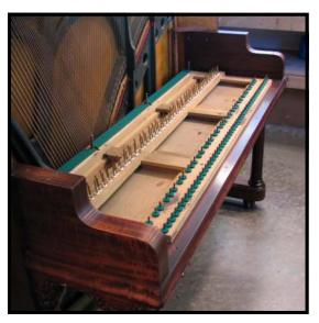
Step 20: To correctly position the keyframe over screw holes, put the right front screw in the screw hole of the keyframe and twist down by hand until the point protrudes slightly. Lift up the keyframe a bit, and eyeball the point of the screw into position in the hole in the keybed. Turn with a screwdriver a few turns (but not tight) into the hole, then repeat the procedure with the front screw on the opposite side. With the two front side screws in place, all the others will line up correctly.
