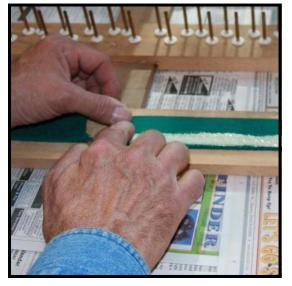
**Step 17:** With your finger, spread the glue on the half of the felt nearest to you. Do not get glue on the other half of the felt.
