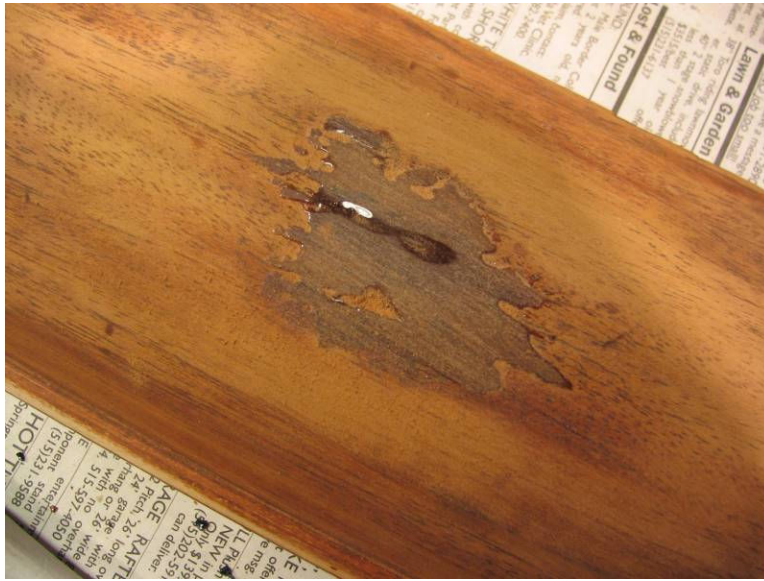
Photo 8: Sanding off the excess lacquer
