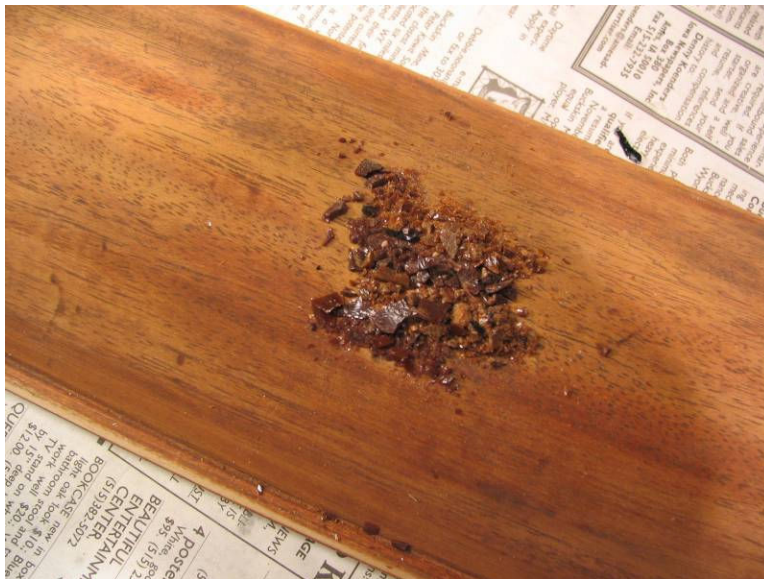
Photo 5: Crumbled lacquer ready for heating
