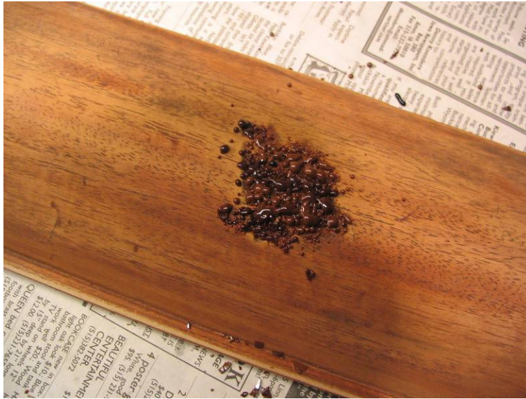
Photo6: Melting lacquer chips start to bead up
