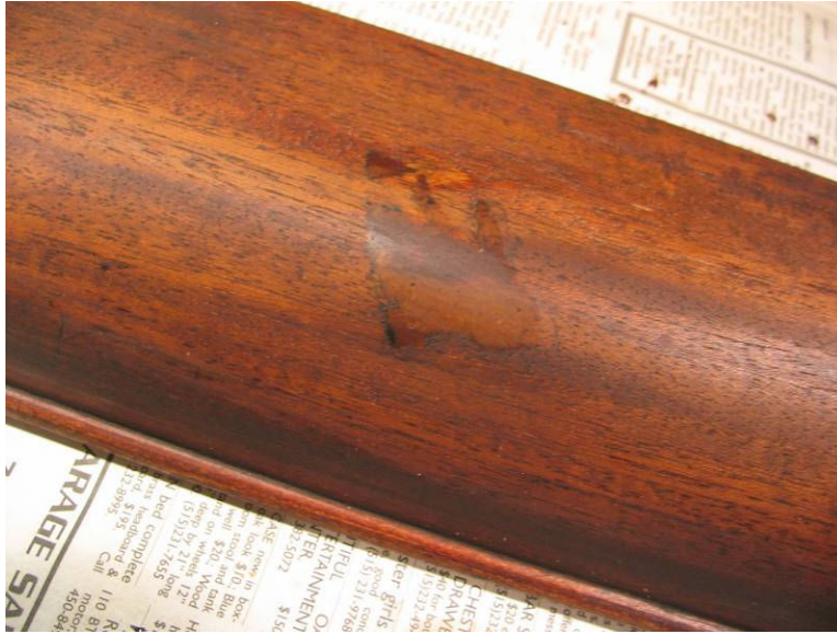
Photo 10: Staining helps blend in patch
