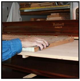
**Step 5:** Set the keys in correct numerical order in a safe location, such as the top shelf of the piano parts trolley. If no work is to be done involving the keys or the keyframe, the keys may be returned to the keyframe as soon as it has been removed from the piano.
