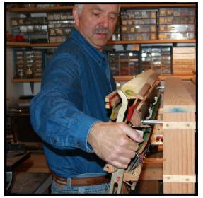
Step 2: Place the action in a secure location out of the way for the time being. If you have built a piano parts trolley, the bolts on the back of the trolley are intended for action storage. Slide the hammer rest rail over the bolts. The heads of the bolts will keep the action from falling off.
