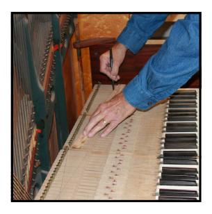
Step 3: Before removing the keys from the keyframe, consider marking the keys for easy identification. A slanted pencil line on either side, with a criss-cross set of lines in the middle, is commonly used. Although the keys are usually imprinted with numbers, 3's and 8's stamped into the wood look very much alike, as do other sets of numbers. If the keys get out of order while off of the key frame, having a backup method of sorting them out can be a real time-saver.
