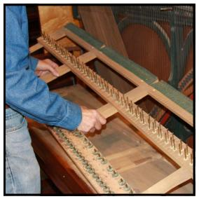
**Step 11:** With all screws removed the keyframe should lift out of the piano. If it still seems secured, check for missed screws. If shims are present under the middle rail (usually at the location of the screws), either tape them down in place, or number (both on the shims and on the keybed itself) and store with the screws.
