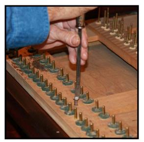
**Step 7:** Remove the screws from the front and center rails. Usually there will be four of each. On older uprights, these will almost always require a flat-bladed screwdriver. A 8" screwdriver (Cat. No. 90) teamed up with a combination tool handle (Cat. No. 26) is as good choice for the job.
