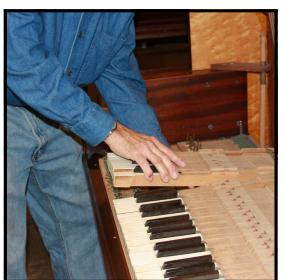
Step 4: Remove the keys from the keyframe. Usually these will lift out a section at a time. Slide your left hand under several keys in between the front rail and the center rail and lift, while using your right hand to hold the set together. A gentle rocking motion up and down while lifting will usually be enough to clear the keys of the center rail pins.
