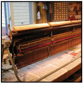
Alternatives for action storage: Another secure location for the piano action is an action cradle (Cat. No. 296). An action post extension (Cat. No. 297) or a Jaras upright action holder (Cat. No. 886), are also useful for the same purpose.
