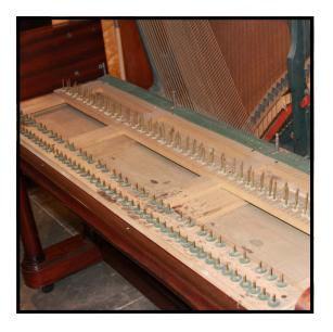
**Step 6:** Before proceeding any further, vacuum out the keybed. Use the hose attachment on a shop vac in combination with a 2" brush to remove stubborn dust. Finish by blowing out any remaining debris with compressed air.
