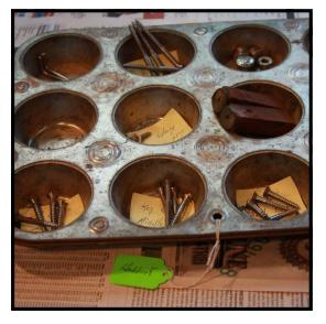
**Step 10:** Label each set of screws and store in a container such as this muffin tin. If several pianos are being worked on at a time, label each muffin tin with the name of the piano as well.
