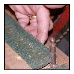
**Step 9:** If no screws are visible, check under the back edge of the backrail cloth. Many times the back edge of this cloth is not glued down and by lifting it the screws will be discovered. Occasionally the screws will be under this cloth even if it is glued down.
