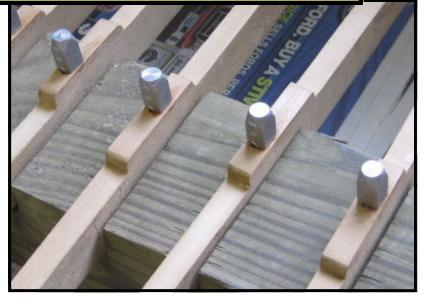
After the keys have been returned to the piano they will be given a final test for fit and will be eased (adjusted) if necessary for an absolute consistent feel from one note to the next. If your piano action is in good regulation and the hammers are in good shape, your piano should be as responsive to your touch as the day it left the factory and will be a pleasure to play once again.
