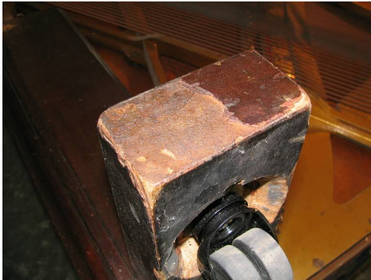
Photo 3: Front of toeblock with typical veneer damage
