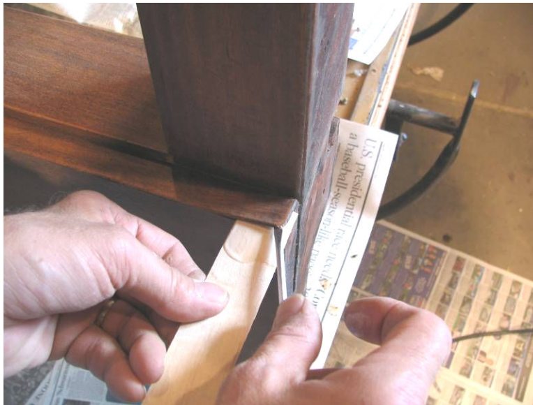
Photo 4: Application of Titebond to loose veneer.
