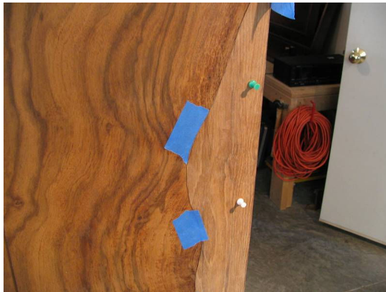
Photo 1: Fitting a new veneer patch in place
