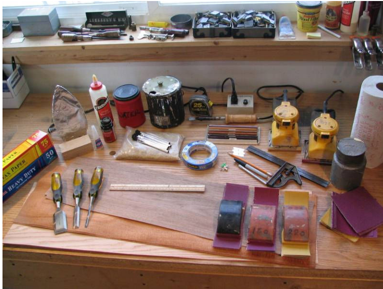
Photo 2: Supplies needed for veneer work and final sanding
