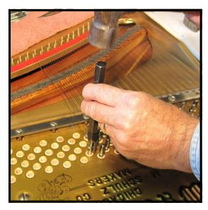
**Step 26:** Holding the pin punch in line with the pin, drive the pin into the pinblock using the ball peen hammer.
