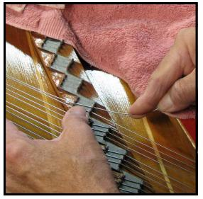
**Step 29:** Pulling the wire towards you, stretch it over the bridge, engaging it between the correct set of bridge pins. Pull the wire tight so that it doesn't slip off the pins.
