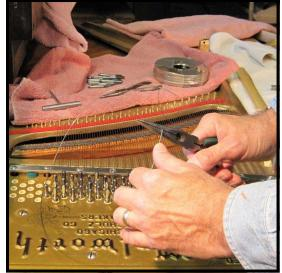
**Step 14:** Be sure to have ample wire unrolled from the spool as you begin. What you want to avoid is having the wire canister or reel being dragged over the hitchpins or bridge while you work because you don't have any slack in your wire.
