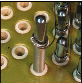
Note: The tuning pin is now ready to be driven in. Notice that the becket is at the 9 o'clock position When the tension has been added to the string, it will finish at approximately the 3 o'clock position. (This is, of course, relative to the fact that the piano is on its back - when the piano is put back on its feet, the position of the becket will appear different.)
