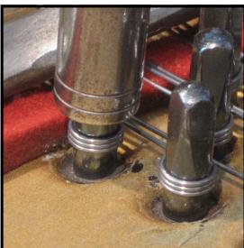
**Step 58 :** Finish adding tension to the string by alternating between the two pins in gradually bringing the pitch up.
