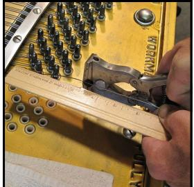
**Step 41:** Align the jaws of the wire cutters at whatever point you wish to cut the wire at. As long as your left hand is gripping both the ruler and the wire, you may lift the wire up from the plate in order to grip it with the wire cutters without affecting the critical measurement. Snip the wire.
