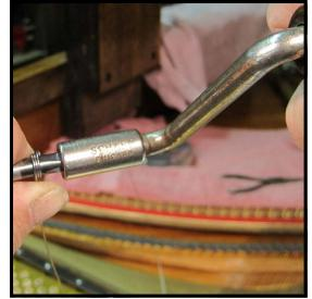
**Step 20:** Use your tuning pin crank (Cat. No. 109) to make the first coil. Use your left hand as the pivot point for the pin, with your thumb tightly holding the wire in place.
