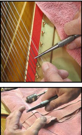
**Step 31:** Hold the wire taut directly over the hitch pin with your left hand. Grasp the wire with a pair of round nose pliers (Cat. No. 241) and line up the pliers with the center of the hitch pin. Clench the wire firmly with the pliers.
