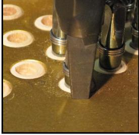
**Step 53 :** At this time, tap both tuning pins down the rest of the way so that the depth gauge is just touching the cast iron plate.
