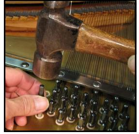
**Step 23:** With a ball peen hammer (Cat. No. 1916) lightly tap the pin in at the correct angle to get it started. Keep the pin slanted at the correct angle.
