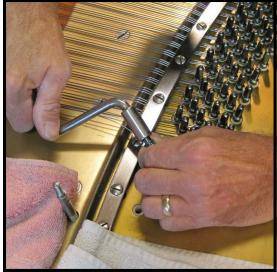
**Step 45 :** Using your tuning pin crank, put the second coil on the pin. For the pins closest to the pressure bar, it will be somewhat tight quarters.
