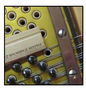
**Step 39:** Slide the ruler up or down slightly so that the very end of the ruler is exactly at the center of the target pin hole.
