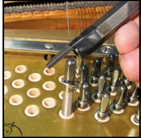
**Step 25:** A pin punch (Cat. No. 174a shown) used with the ball peen hammer is one way to drive the pin in the rest of the way. The rubber depth gauge shown in the photo is simple to make using a thin slice of rubber mute (Cat. No. 203 1/2) with electrical tape to hold it in place. Make the gauge a bit long to begin with, then shave off enough with a razor blade so that it corresponds to the correct height of a sample pin.
