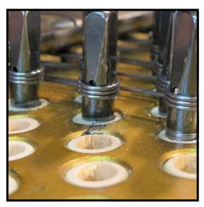
**Step 54:** Check the coils one last time to make sure that they are still perfectly tight. In the photo, the coil on the middle pin looks a bit loose, and should be re-tightened with the impact hammer. *Note: If the eye of the pin is partially covered by the upper winding of the coil, you've gone too far. Gently tap the coil back down with a flat-bladed screw-driver until the hole is fully exposed.*
