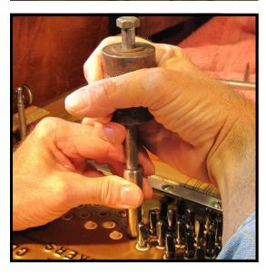
*Note:* The coil is fairly tight at this point, but not tight enough for the finished product. Also, the becket is not pushed in the entire way.
