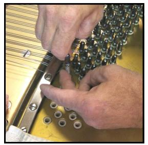
**Step 47:** Remove the tuning pin crank from the end of the pin, and insert the end of the pin into the target pin hole. Pull back on the pin from the top, if necessary, to achieve the correct slant.
