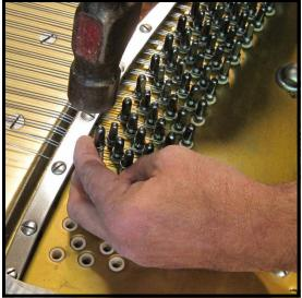
**Step 48:** Lightly tap the end of the pin with the ball peen hammer to start it.
