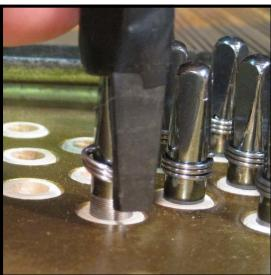
**Step 27:** Pound the pin down most of the way, but leave it a bit short at this point. You'll drive the pin in the rest of the way once both sides of the wire are in place.
