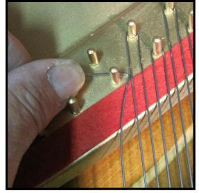
**Step 33:** The wire may now be placed around the hitch pin. Start with the bend in the wire about 1/2" from the pin, as shown, then pull the bend into place.
