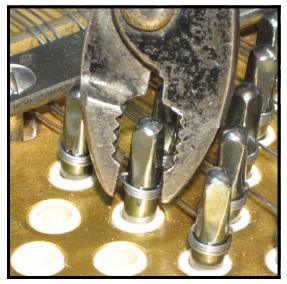
**Step 52:** With the coil tight, squeeze the becket tight to the pin using a pair of ordinary pliers.
