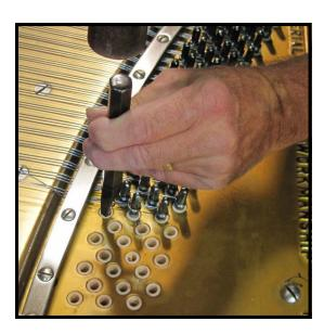
**Step 49:** As was done in step #27, pound the pin in most of the way, using the tuning pin punch with attached depth gauge.
