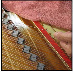
**Step 30:** With the string pulled tight, hold it directly over the hitch pin to which it will wrap around.
