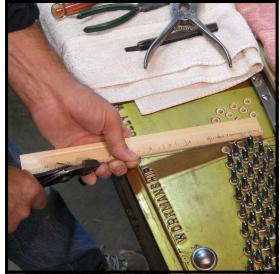
**Step 38:** To obtain an accurate measurement, it is necessary to pull the wire tight. Use a pair of ordinary pliers with your right hand to grip the end of the wire while holding the wire next to a ruler with your left hand. Pinch the wire between your thumb and forefinger, while grasping the ruler as shown.
