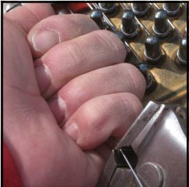
**Step 37 :** Following the procedure outlined in steps 15 and 16 on page 12, run the return length of wire under the pressure bar. Once the wire is under the bar, pull the slack out of it, but do not complete the bend for the becket, as the end of this wire will be cut off once it's measured to length.
