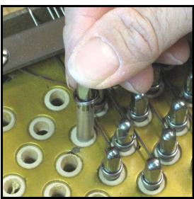
**Step 22:** Push the tuning pin slightly into the hole, just far enough that the tuning pin bushing grips it.
