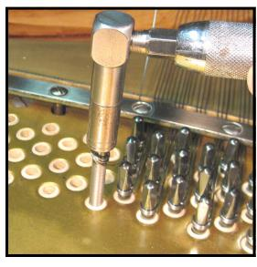
**Step 24:** Using your tuning hammer, if necessary, turn the pin so that the becket is 180 degrees from where you wish to have it end up. In other words, you're leaving one half of a complete turn for tensioning the string.
