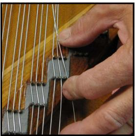
**Step 35:** Thread the return wire past the bridge pins. By having wire in place through the bridge pins, more precise measurement of the length of the wire needed to produce even beckets may be made once the wire is pulled tight.
