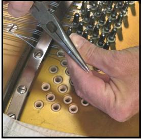
**Step 42:** At this point put a 90 degree bend into the end of the wire to form the becket.
