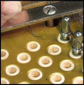
**Step 15:** For the first bend of the operation, put a 45 degree angle in the wire, which will allow you to easily slip the wire under the pressure bar.
