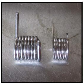
*Note:* A good starting point for this important measurement would be 3 1/4", as shown in the photo. As you go from one wire size to the next, you will need to make minute adjustments in the length of the string to produce the same number of coils. As the wire size decreases, so should the length of the wire.
