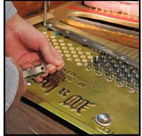
**Step 36 :** Stretch the wire across the pressure bar and cut it with some excess length. This will allow you to hold on to the end of the wire for making the final cut after it is run underneath the pressure bar.
