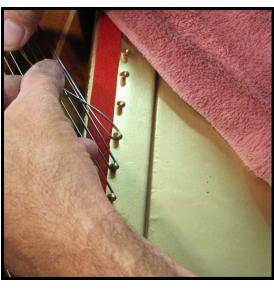
**Step 34:** Wrap the wire around the hitchpin a little further than it will end up to better set the bend.
