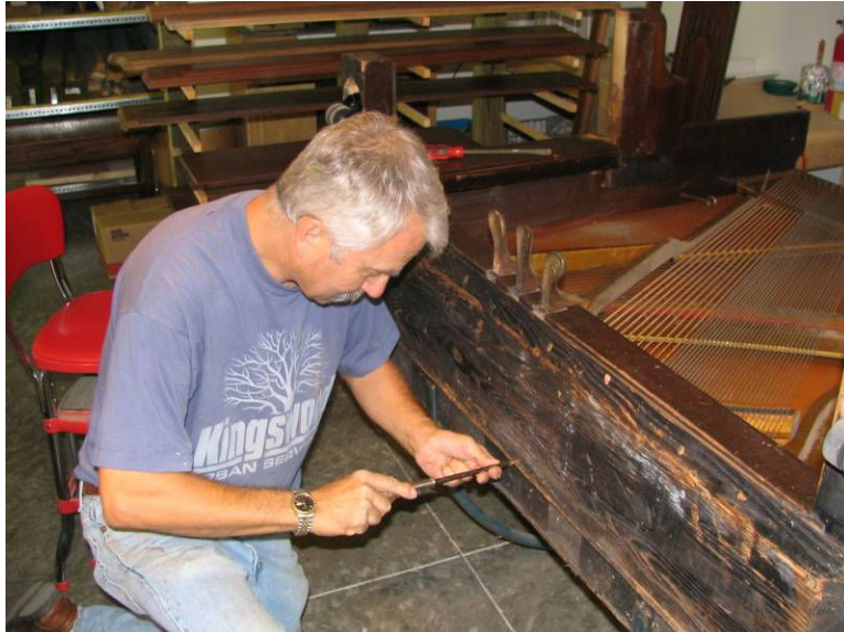
Photo 4: Removing the floor of the piano
