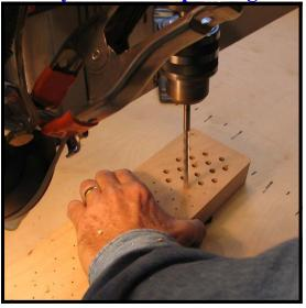
Step 8a: If new pinblock panels are being installed, the pin holes may be drilled at the drill press, as shown in the photo to the left. An alternative to this method is to use a portable drill press set-up which rolls over the pinblock after it is installed in the piano. Whenever methods vary, do the research and chose the approach that works the best in your own shop.
