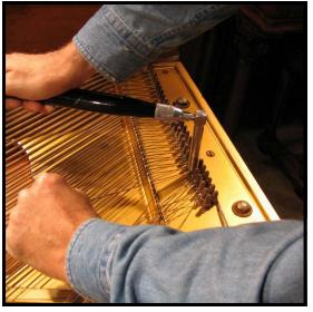
**Step 3:** At this time, removal of the old pins and strings will be necessary. A new set of tuning pins will be needed shortly. The bass strings will need to be sent off for duplication, while the treble strings will be replaced on site. (For a complete description of these procedures, refer to the article, "Removing Bass Strings for Duplication," and the companion article "Removing and Miking Treble Strings for Replacement," both available now for download from your Schaff eStore.)
