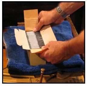
**Step 10:** Open the new box of tuning pins to be used, remove the paper covering the pins, and place them within easy reach of the work area.
