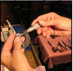
Second - If necessary, use a micrometer (Cat. No 3338, 4044, or 3299) to mike the drill bit to make sure you have selected the desired size (although the bits are numbered, sometimes the numbers wear off of the shanks). (For a discussion the differing opinions concerning approaches to preparing an old tuning pin hole for an oversized pin, refer to the Schaff article, "Repinning an Upright," available now for download from your Schaff eStore.)
