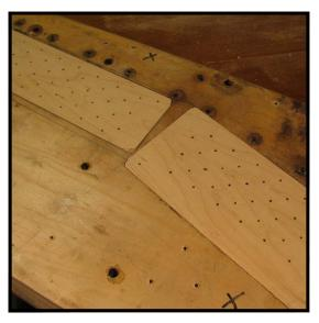
**Step 4c:** If you are installing a new pinblock or pinblock panels (as shown in photo to left), order size 2/0 X 2 3/8" or 2/0 X 2/1/2" pins, according to the thickness of the pinblock installed. Size 2 pins are generally the diameter pins that factories install. Thus, your newly repinned piano will be done according to factory specs.
