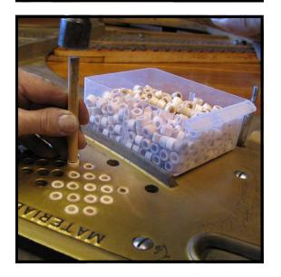
**Step 9:** One final decision to be made at this point is whether or not to install new tuning pin bushings (Cat. No. 346 A, B or C. Also 345A, B, or C).
