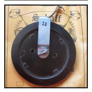
Step 7a: Piano wire is available from Schaff in coils of a variety of sizes. The most convenient and easy are the 1/3 lb. reels with brake, available for sizes 12 (.029") to size 22 (.049"). To avoid delays while in the middle of a restringing job, it is a good idea to stock a spare reel of each gauge, so that when one reel runs out, another is available immediately. Reorder spent reels to keep your supply updated.
