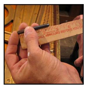
**Step 4b:** Also, for each diameter of tuning pin, 3 lengths are available (2-1/4", 2-3/8" and 2-1/2"). A more precise tool for such measurements (than what's shown here) would be a 6" tempered steel rule (Cat. No. 3197).
