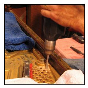
**Step 8b:** If the old pinblock is being utilized and oversized pins are being installed, a simple electric drill may be used to ream the old holes in preparation for new pins. Notice that the drill is not being used at a perpendicular angle to the plate, but is rather canted to follow the original slant of the pins.
