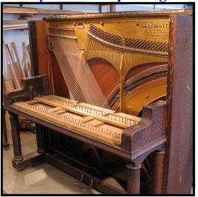
Step 1: Before a repinning / restringing job is begun in earnest, a substantial tear-down of the piano is in order.
