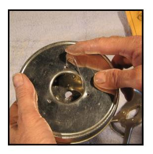
**Step 14:** Push the bent end of the wire into the nearest 1/8" hole.
