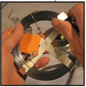
**Step 4:** The coil is maintained with a metal clamp and also with 3 separate wire ties. Loosen the clamp first by unbending the arms which are wrapped around the coil. *Note: The clamp is made of a soft metal and may be easily unbent by hand.*
