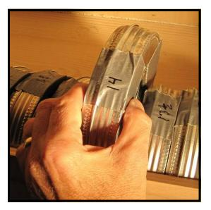
**Step 20:** Return wire coils not in use to storage shelf to avoid having more than one size on the work area at one time.
