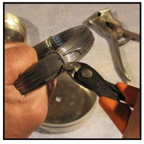
Step 6: While holding the coil firmly in your left hand (see cautionary note in step 6), snip the soft wire ties which are wrapped around the coil. As these wire ties are easily cut, any good nippers will do, such as the Maxi-Shear Flush Cutter (Cat. No. 215) shown here.
