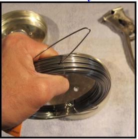
**Step 7:** With the tie removed, the end of the wire will spring out. Notice that the end which had the yellow tag has a long bend. The inside end has a shorter bend.
