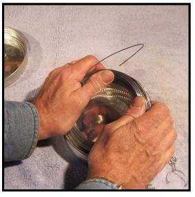
Step 9: Carefully insert the coil into the bottom half of the canister. It works best to put one side of the coil in first, and then push the other side in while maintaining your grip on the coil for as long as possible. Push down any stray loops that pop up so that they are within the rim of the canister. The exception to this is the bent end of the coil, which should remain on the outside of the canister as shown.
