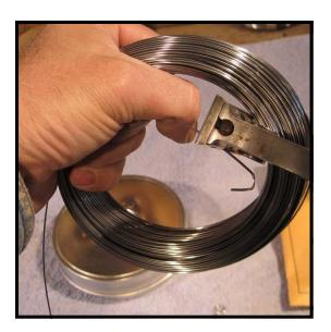
**Step 8:** Once all three wire ties are cut and removed, snip the inside bend of the coil with a pair of wire cutters, such as the Starrett Wire Cutters (Cat. No. 225B) shown. Note: If you don't cut this inside bend, it will tend to bind on the loops of the coil as you try to draw wire from the canister.
