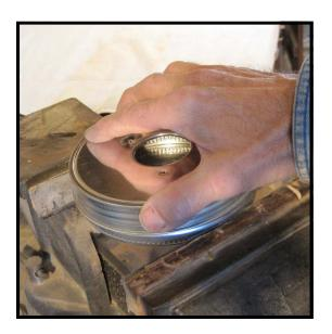
Hint: If the top of the canister is hard to turn, open your bench vise wide enough to accommodate the bottom half of the canister. (Leather or cork faces on the jaws of your vise will help here.) Turn the vise down just tight enough to grip the bottom portion of the canister, and rotate the top part counter-clockwise to loosen.
