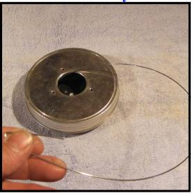
Step 15: Before finishing up the with the canister, check to make sure that there is no binding. Draw on the wire to see that it may be easily pulled out for use.
