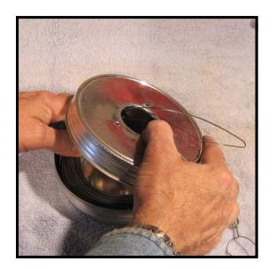
**Step 11:** With the top half of the canister ready to go in place, carefully withdraw your left hand and close the two halves of the canister together. Make sure all of the loops of the coil are within the body of the canister.
