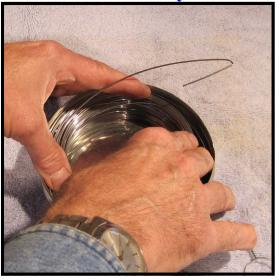
**Step 10:** Snug the coil down to the bottom of the canister. Then, while holding the coil in place with your left hand, pick up the nearby top of the canister, and run the bent end of the wire through the large central hole.
