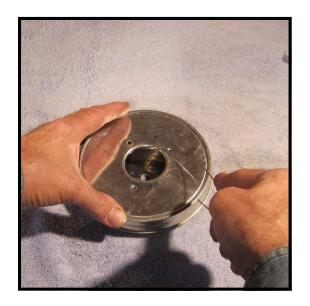
**Step 16:** While holding onto the canister with your left hand, you should be able to push the excess wire back in again. Secure the bend into one of the 1/8" holes before going any further.
