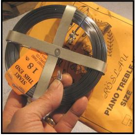
Step 3: Remove the wire coil from the envelope it came in. Notice the tag advising which end to start the wire on. This will be the end of the wire which emerges from the hole in the top of the canister.
