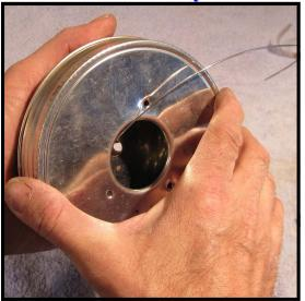
**Step 13:** Pick up the canister, holding the bottom half in your left hand and turn the top half clockwise until it is tight.
