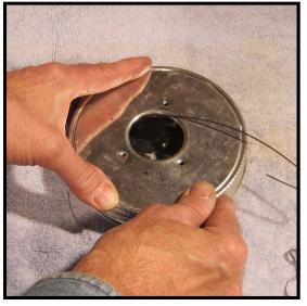
**Step 12:** Push the top half of the canister firmly down onto the bottom half. You should feel it go into place. Apply a little clockwise twist to the top half to keep it from coming apart.
