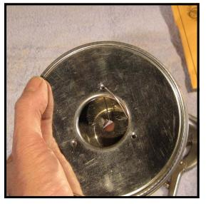
Note: With the end of the wire secured and out of the way, the wire will be easy to access without having to fish about inside the canister for the end to start with.
