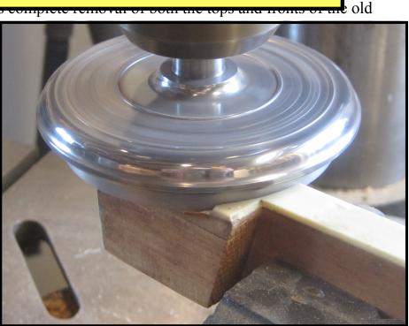
milling down process gives a completely flat surface on which to glue the new keytops.
