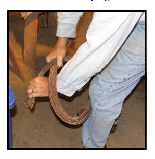
**Step 10:** Brace the bundle against your knee as shown, and pull the loose end of the bundle through the center of the loop. Pull it far enough through that it stays in place when you let go of the strings.
