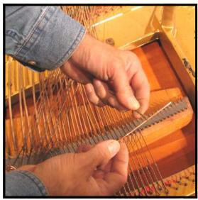
Step 5: Removing one string at a time, thread the loop of each string onto the copper ground wire. (The ground wire itself should have a loop at the end to prevent the bass strings from slipping off.) If any strings are missing from the set, mark the position of the missing strings with a felt center or front rail punching. Be very careful to keep the strings in order as you go. To avoid confusion, never remove more than one string at a time from the hitch pins.
