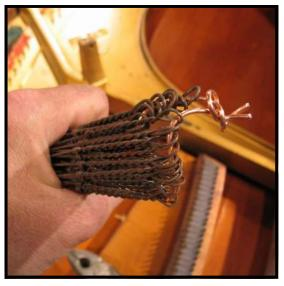
Step 6: Once the entire set of bass strings has been removed from the hitch pins and the loop of each string has been threaded onto the ground wire, put the end of the copper wire through its own loop and pull the set into a tight circle. Twist the end of the copper wire into a knot so that the set of strings is secure.
