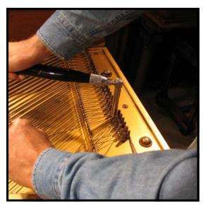
Step 3: Once the tension on the piano as a whole has been let down, move from one side of the bass to the other, backing the tension off each string another one half turn or so. (A full turn if you are restringing the bass alone.) Lift each string up and off the upper bridge with your left hand as you pivot the tuning hammer with your right.
