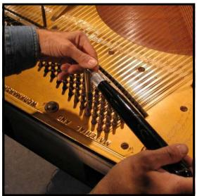
Step 2: If the bass string replacement is a part of an over-all restringing project, let down the tension on the entire piano first. Using a tuning hammer such as the nylon extension lever (Cat. No. 16), turn each pin counter-clockwise approximately three quarters of a turn, using a pattern to gradually bring down the tension from one side of the plate to the other. If the bass strings alone are being replaced, however, do not back off the tension of the entire piano.
