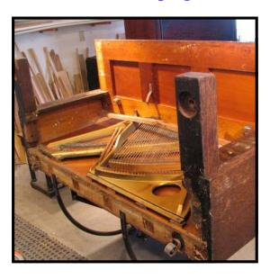
Step 1: For any restringing or repinning job involving a vertical piano, putting the piano on its back will make it easier to work on. A shop repair truck (Cat. No. 1901) makes tipping the piano onto its back an easy process. (For safety sake, always complete this procedure with two people.)
