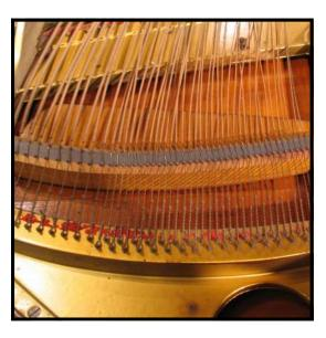
Step 4: With the entire set of strings slack across the lower bass bridge, remove the first string on the right from the bridge pins and hitch pin. Grasp the string above the bridge pins and pull upwards sharply to release. Thread the loop of the freed bass string on a copper wire. (The ground wire from a short length of Romex works perfectly for this job.)
