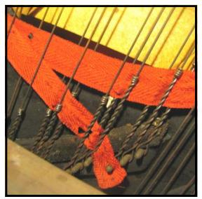
**Step 3:** Before removing the first tuning pin, check the hitch pins at the bottom of the piano to determine which stings are singletons with their own loops, and which strings are in pairs, going around the hitch pin from one tuning pin and back up to the next. The steps that are followed will differ slightly for strings that are singletons and strings that are in pairs. Wound strings will always be singletons, while steel string in the tenor and treble will usually be in pairs.
