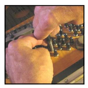
**Step 18:** With the coil on the tuning pin and the becket in the hole, insert the end of the pin into the waiting hole in the pinblock and angle it forward. The coil will unwind slightly as the pin is brought to a vertical position.
