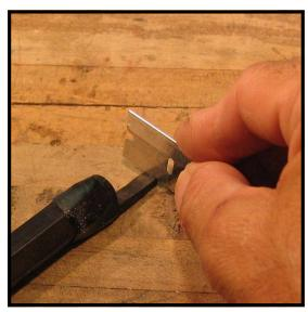
Second—With your pin punch outfitted with a sliver of rubber mute (electrical tape wrapped several times around the mute and the body of the punch will hold it securely in place), check in the piano for length. Place the punch firmly against the head of the pin. The end of the mute should just make contact with the plate. If it bows outward at all, it is too long.
