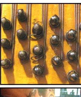
**Step 8:** Without removing the coil from the pin, use a high-torque, variable speed drill with a power tuning pin socket (Cat. No. 63) to back out the first pin. Start slowly, and watch to make sure that the becket does not catch in the hole of the pin. If it does, stop immediately to correct the problem. Back the pin out slowly in order to prevent excessive heat
