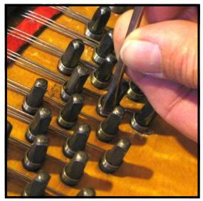
**Step 6:** Use a grand action screwdriver (Cat. No. 193), or other similar screwdriver, to remove the becket from the pins. Place the tip of the screwdriver between the coil and the pin, directly behind the becket. Use the screwdriver as a lever, with the top of the tuning pin as the fulcrum to pry the becket out of the hole in the pin. Once the end of the wire is clear of the hole, pull it slightly to the right so that it doesn't slip back into the hole as the pin is being backed out.
