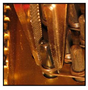
**Step 23:** Re-crimp the becket, using a pair of long nose vise grips (Cat. No. 271). This step may need to be repeated one more time, once the final adjustment to the strings have been made.
