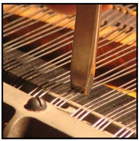
**Step 28:** Make fine adjustment to the string spacing using a string spacer (Cat. No. 133). Place the slots of the spacer over the 3 strings for the note. When the spacer is pulled off the strings, it should be quiet. If you hear a 'zing,' the strings are not evenly spaced. Adjust and recheck until the spacer may be placed on the strings and removed without causing the strings to vibrate. Be sure to use the spacer at the same point in the speaking length of the strings for every note.
