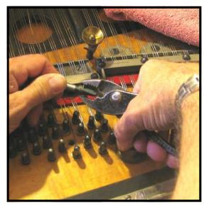
**Step 17:** Trade the needle nose pliers for a regular pair of pliers, and crimp the becket down closer to the pin.
