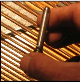
**Step 30:** After the coil has been put on the new pin, twist the pin in the direction of the winding one turn. Put the pin in the hole, and drive into place. Follow all the steps as before. With strings that are two to a note, bring the pitch up to match the other string. For the lowest notes, with one string to a note, set the pitch by going between the notes on either side.
