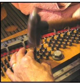
**Step 19:** Holding the tuning pin in place with your left hand, give the top of the pin two or three solid taps to start it with a ball peen hammer (Cat No. MF-1916). The pin should be driven in far enough to remain in place when released.
