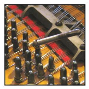
**Step 9:** When the pin has been turned completely out of the hole, it will usually fall from the socket when you lift the drill (or hand brace). If it does not, pull the pin from the pin socket. If the pin is still attached to the coil as shown, simply pull it free from that as well.
