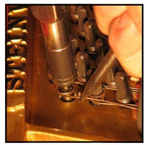
**Step 22:** With the tuning lever and the string hook, put just enough tension on the first string to take up the slack in the coil. By pulling upward on the string hook as you turn the pin clockwise, you will begin to tighten up the windings of the coil.
