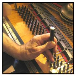
**Step 20:** Line up a pin punch (Cat. No. 174 [3"], 174A [5"] or 174B [4-3/8"]) to be in line with the pins. Be aware of the backward slant of the pins. Again, match the slant of the pins when preparing to drive the new tuning pin in place.
