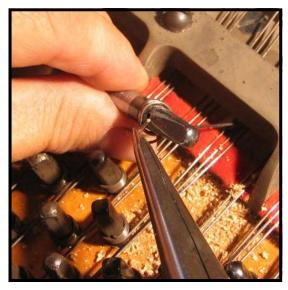
**Step 15:** With a quick motion down and back up, and the drill turning at high speed, ream the hole for the new larger pin. Wood chips should fly out as the bit is brought back up. If there is any smoke, your bit is dull, and should be sharpened or replaced.
