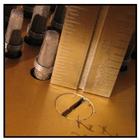
Hazard!!! If you are given or inherit a pin punch such as this one, do not use without grinding the top down smooth! Using a worn tool such as this could cause injury, as pieces could break off upon impact!
