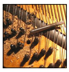
**Step 29:** Once the treble section has been completed, turn your attention to the bass. The wound strings of the bass will all be individual strings—each with its own hitch pin. Remove one pin at a time as you move from the break towards A0. Make sure that when you release the tension on each string, that it stays in place on the bridge and hitch pins.
