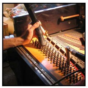
**Step 31:** With all the pins replaced, double check everything before returning the action and keys to the piano. In particular, check to make sure that the strings are correctly aligned over the bridges. Re-check the string spacing. Recrimp any beckets that don't seem tight and check the coils to make sure the windings are snug.
