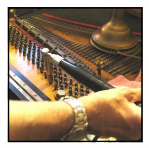
**Step 4:** Decide on a starting point, and use a nylon extension lever (Cat. No. 16), or other suitable lever, and turn the pin (for a singleton) or pins (for a pair) about 3/4 turn counterclockwise to release the tension from the string.
