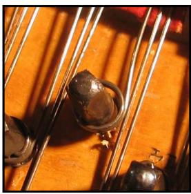
**Step 5:** Check the coils for the pins you've turned back. They should be loose enough to insert a small screw-driver in between the pins and the inside of the coil.
