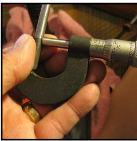
**Step 10:** Using an accurate micrometer, such as the Starrett micrometer (Cat. No. 3338) or the Starrett digital micrometer (Cat. No. 4044), measure the diameter of the tuning pin that you've just removed. If the tuning pins are the original factory pins, they are most likely size 2/0 (.282"), or size 1/0 (.276"). The piano shown in these pictures had pins that measured .264", or smaller than a size 1/0.
