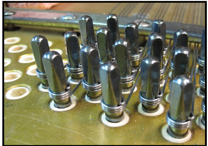
New tuning pins and strings being installed.
