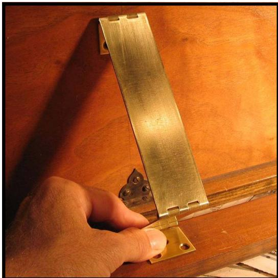
**Step 2:** Check to see that the geometry of the music desk hinge will work for the music desk in question. Actually fold the hinge in the configuration which it is to be used in, and hold it up to the music rack to see if it will fit. Check the angle of the music rack with the hinge in place. The further back the hinge is to be placed, the steeper the resulting slant of the music rack will be.
