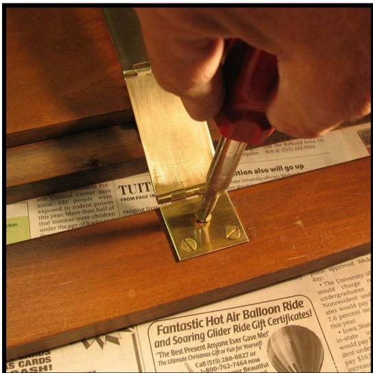
**Step 9:** Attach the hinge to the rail using the correct screws. Do not over-tighten the screws.
