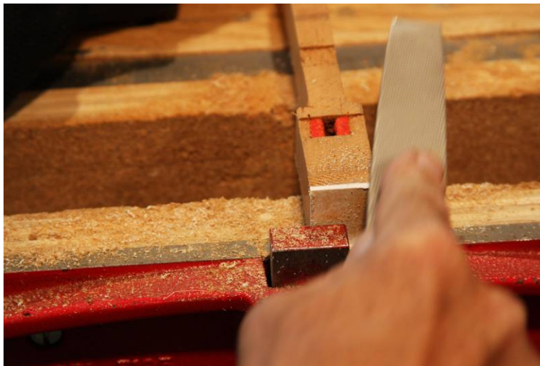
Photo 10: Filing off the excess.
