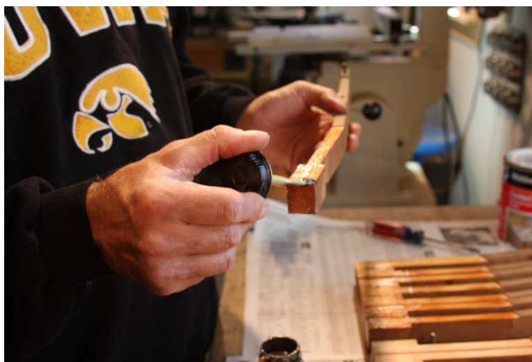
Photo 1: Applying the first coat of glue to top of keystick.
