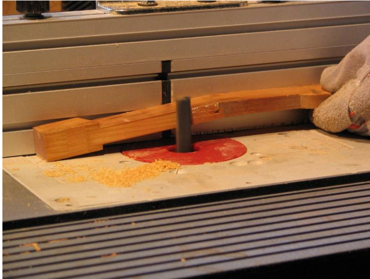
Photo 4: Using the router to surface the keytop.
