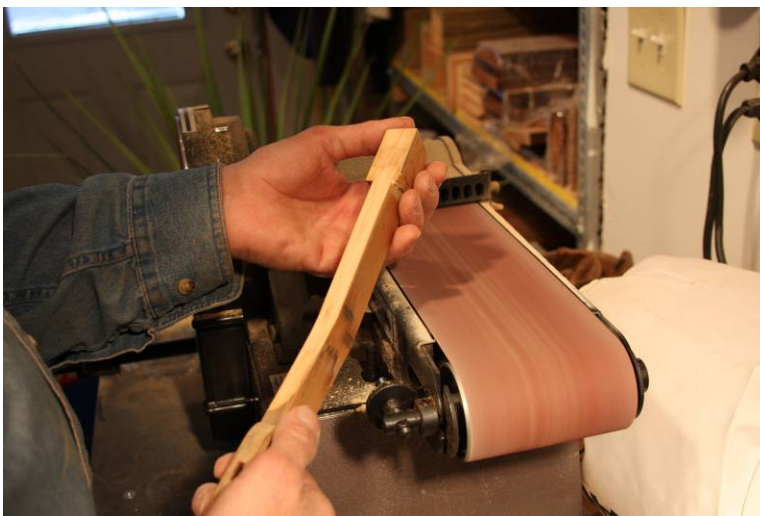
Photo 3: Used with care, old glue may be quickly removed.
