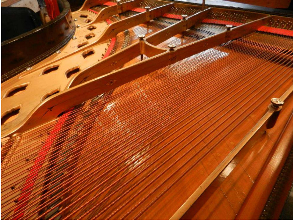
Photo 37: Restringing complete – everything cleaned and polished inside the rim of the piano.
