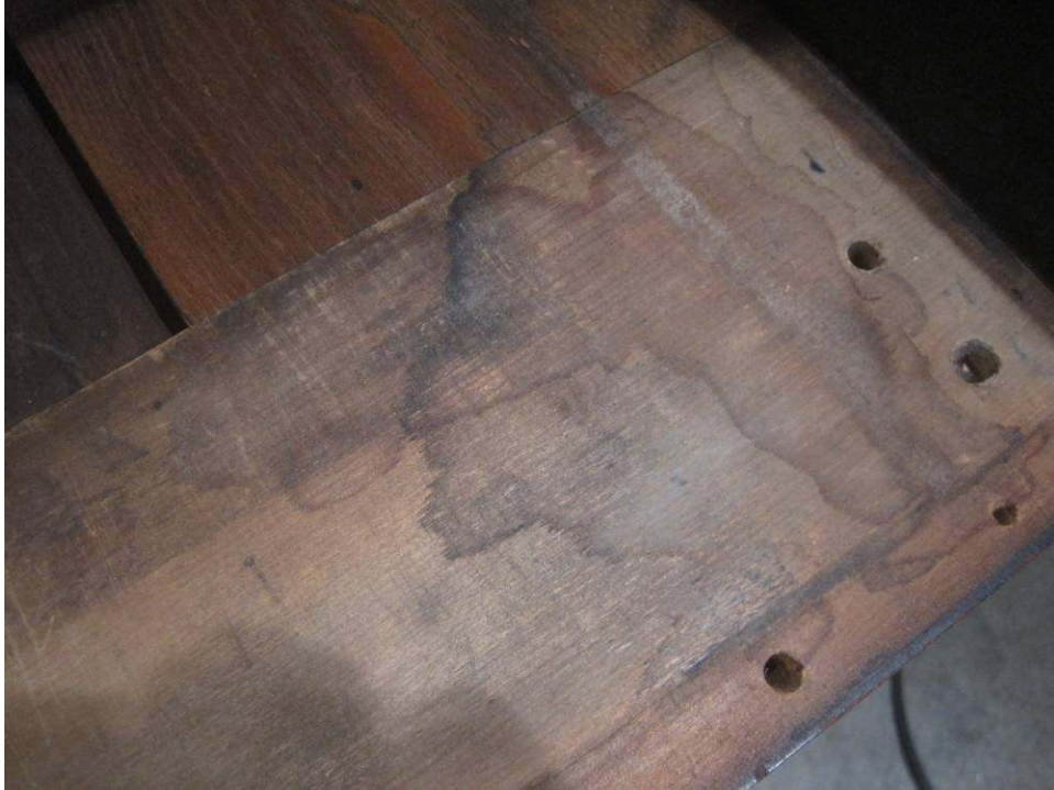
Photo 47: One other area of concern as far as the body of the piano is the keybed. This is an unfinished expanse of wood that is susceptible to retention of odors. At least, no mice had ever lived in this piano! When that happens this surface can smell like the bottom of a dirty litter box!
