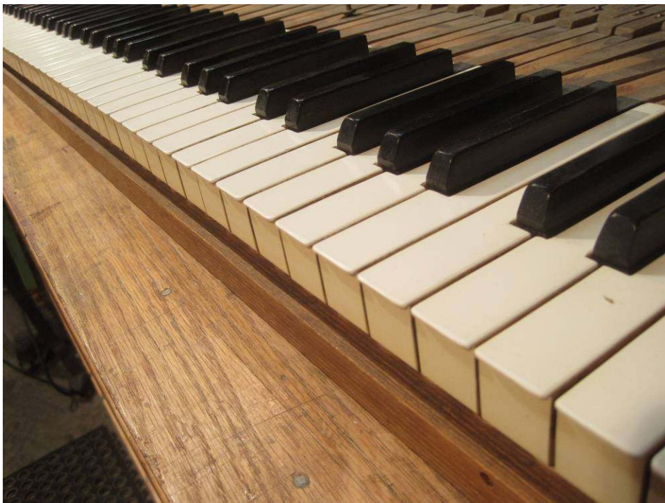
Photo 88: The leveled set of keys, ready for the installation of the wippens and hammers.
