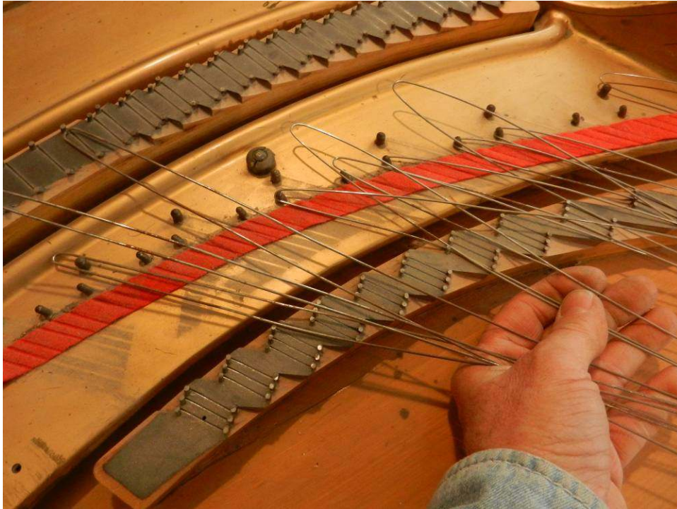
Photo 17: The treble strings are also unattached at the back at the hitchpins, but left connected on the front end to the tuning pins.
