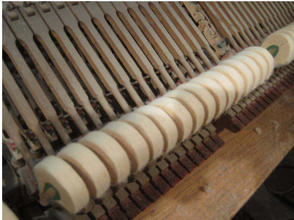
Photo 55: Once done, the surface of the hammers looks nearly new.
