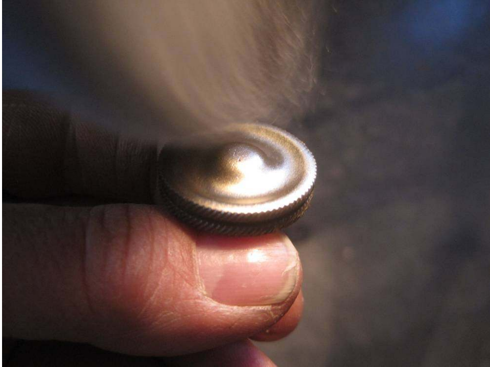
Photo 29: A wire brush wheel polishes the brass.
