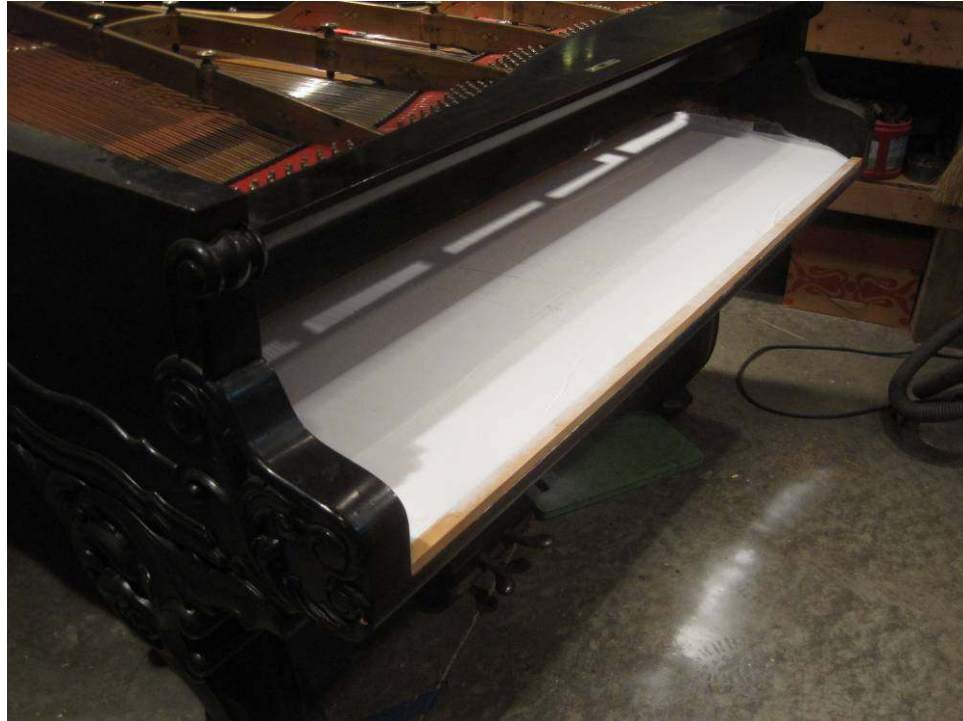
Photo 51: The inch deep layer of baking soda (24 pounds) is allowed to do its work for 7 days, while work on the action of the piano begins.
