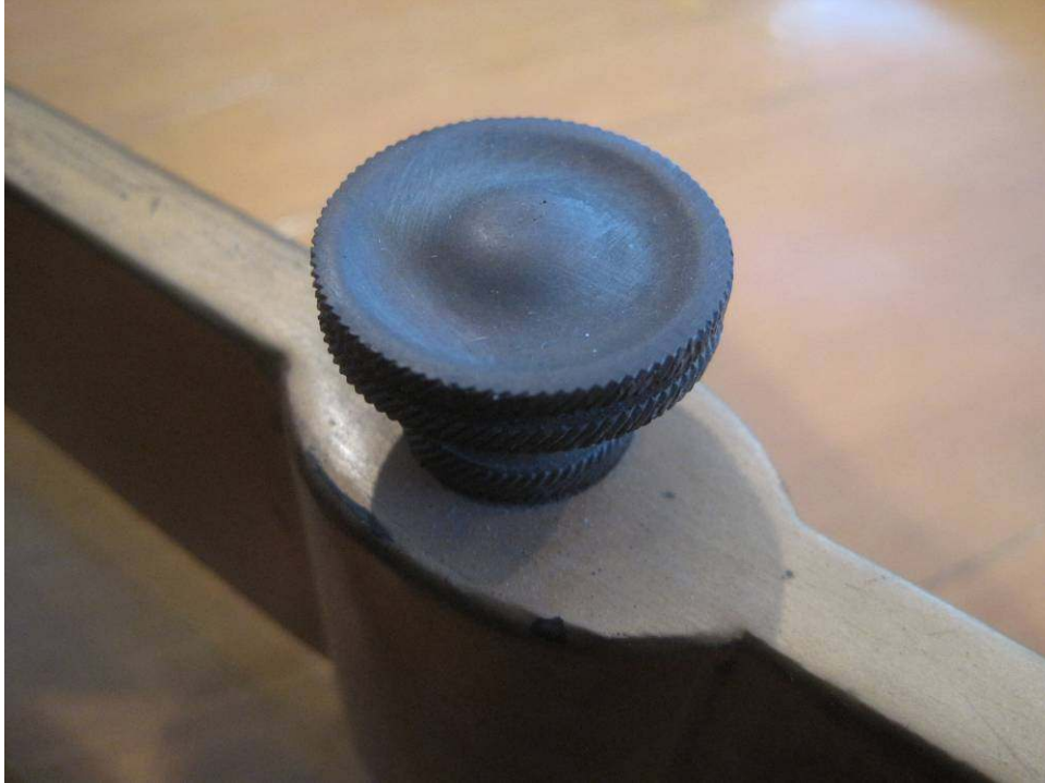
Photo 27: The layer of corrosion on the nosebolts of the cast iron plate needs to be removed. Who knows how many smoke molecules are trapped within the corrosion.
