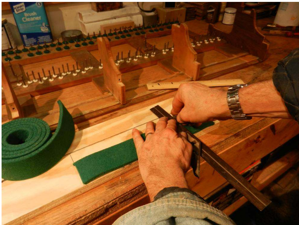
Photo 70: The 5 sections of back rail felt are cut to size and glued into place.
