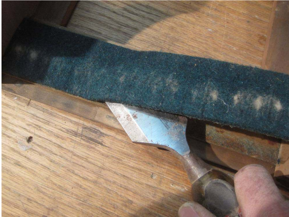
Photo 69: Finally, the back rail felts are removed, and the old glue is scraped off.
