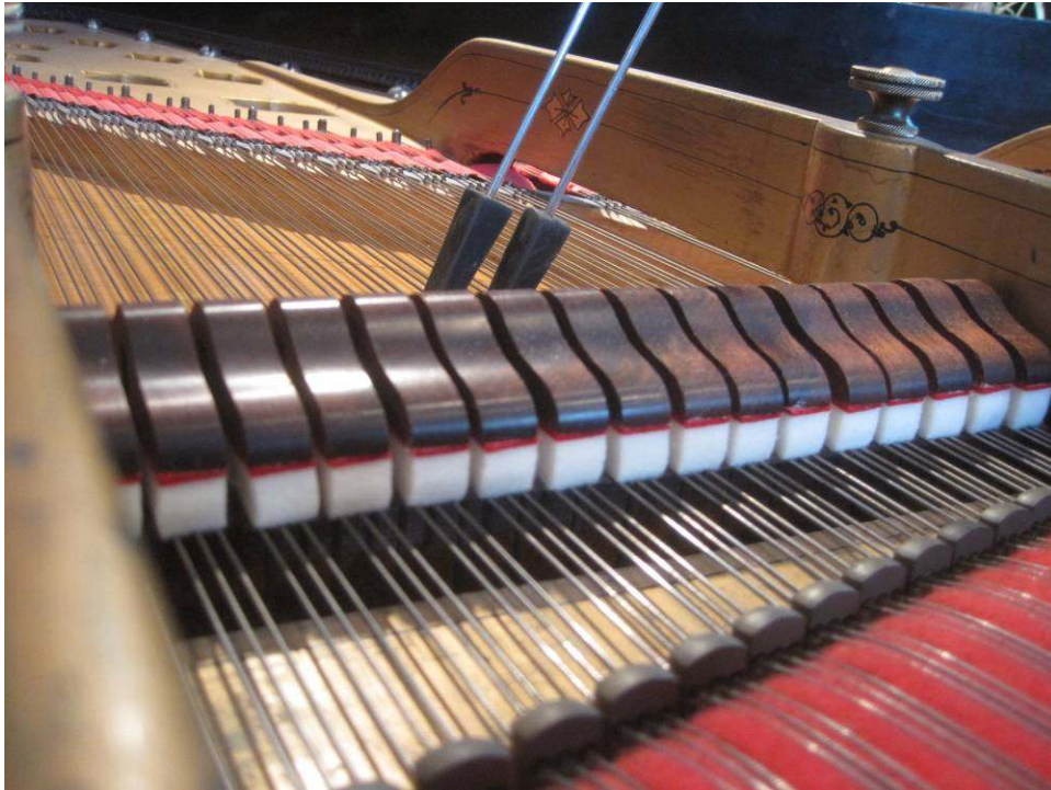
Photo 93: With the action back in the piano, tuning work may begin. The piano will be given a half dozen tunings (to restore the tension and stability) before it leaves the shop.
