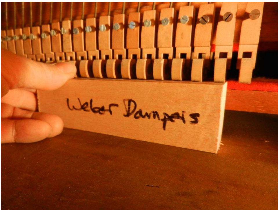
Photo 6: After vacuuming, before anything is actually taken apart, a reference block is made for the purpose of later reinstalling the new dampers at the correct height.
