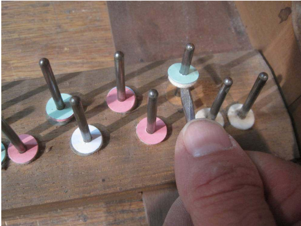
Photo 87: After the leveling papers are installed to bring the keys up to level, the papers are flipped so that they are underneath the balance rail felts.
