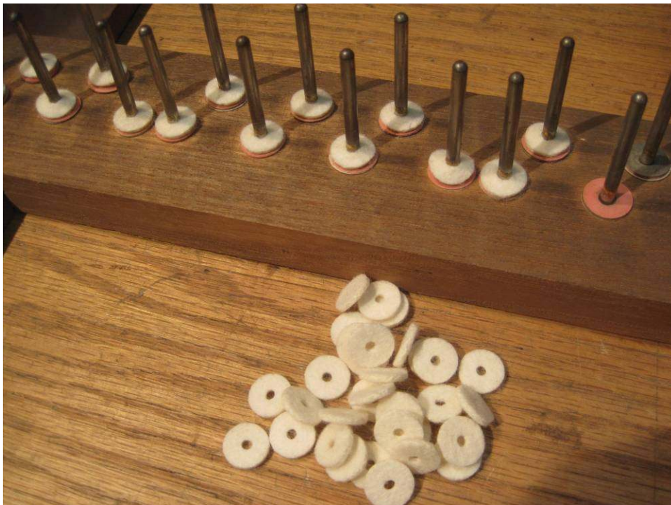
Photo 68: Followed by the balance rail felts.
