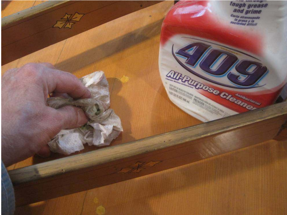
| Photo 23: The final step of cleaning is to go over the soundboard with Formula 409®. This removes any remaining oils and dust on the surface.
