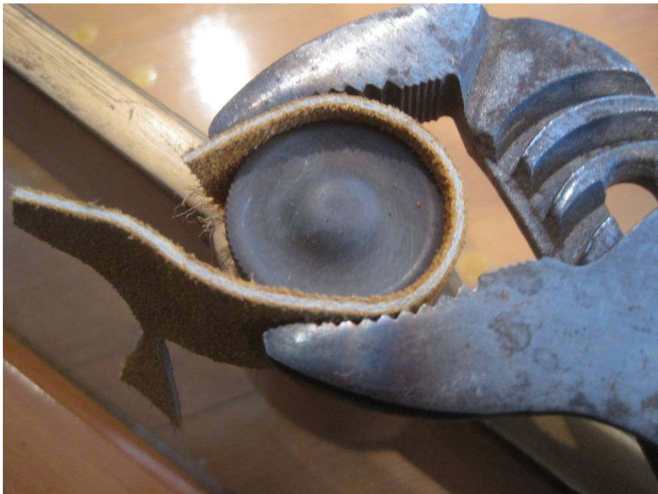
Photo 28: With the tension of the strings removed, the nosebolts may be removed one at a time. A strip of buckskin protects the edges of the brass nut from the teeth of the pliers.
