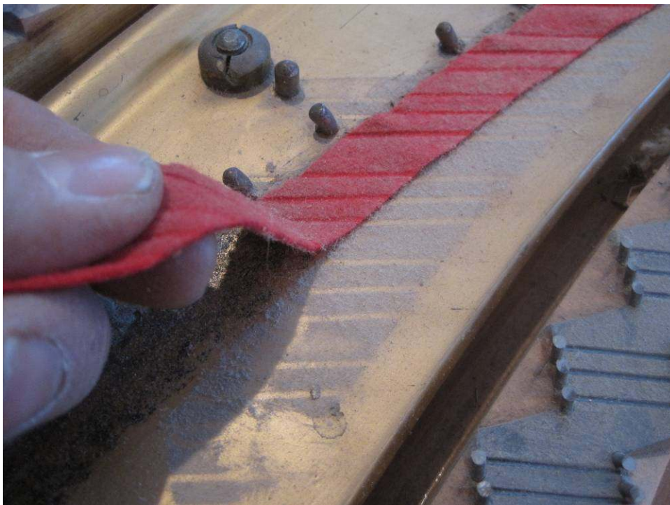
Photo 20: The plate will need to be cleaned as well. Here, the understring felt glued to the plate is removed. It will be replaced with new felt after everything is cleaned.
