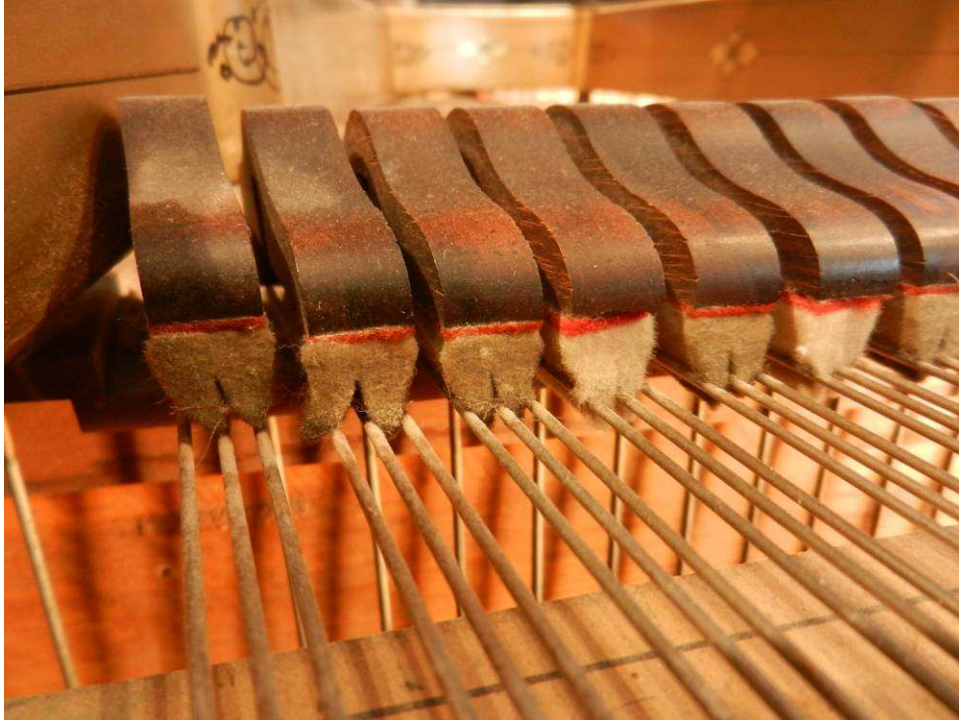
Photo 3: With the case parts removed, problem areas are clearly revealed. The old bass damper felts need to be replaced. These are soft felt, designed to absorb the vibrations of the strings when they drop back onto the strings. They are like little sponges when it comes to odors.
