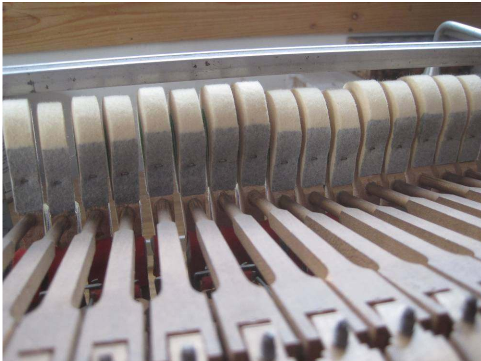
Photo 89: The hammer line, once everything was put back together, was very uneven. More regulation would need to be done, starting with bringing up the hammers to the correct height.
