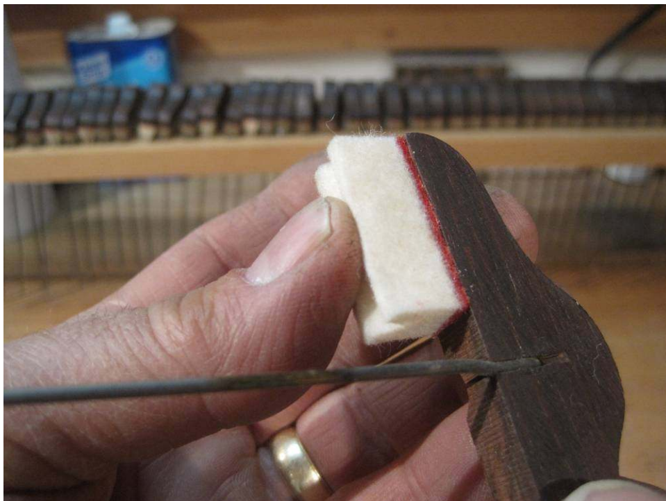
Photo 79: : . . .and the damper is pressed into place.
