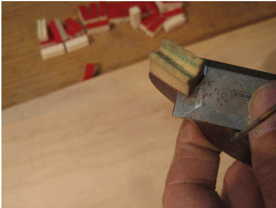
Photo 77: The felts are removed with a sharp chisel, and the underside of the wooden damper block is scraped clean of old glue.
