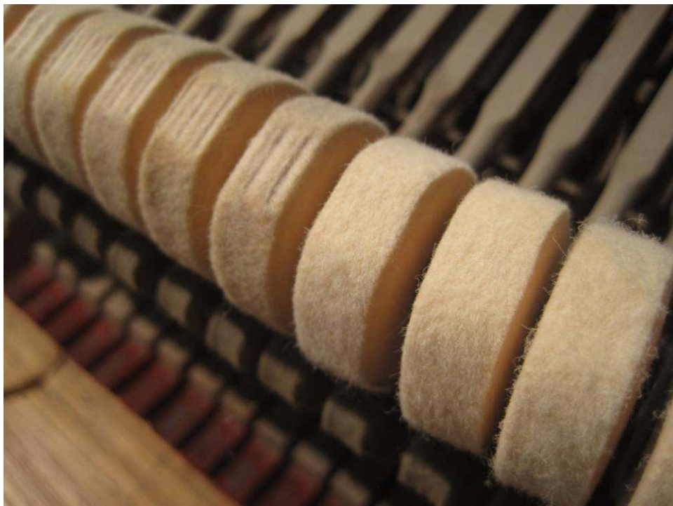
Photo 54: Hammers before filing on the left, hammers after filing on the right.
