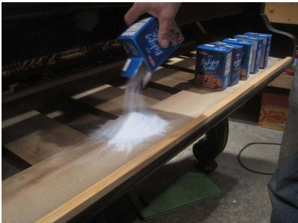
Photo 50: To make sure any lingering odor is removed, a dam is attached to the front of the keybed, and the entire surface is covered with baking soda.
