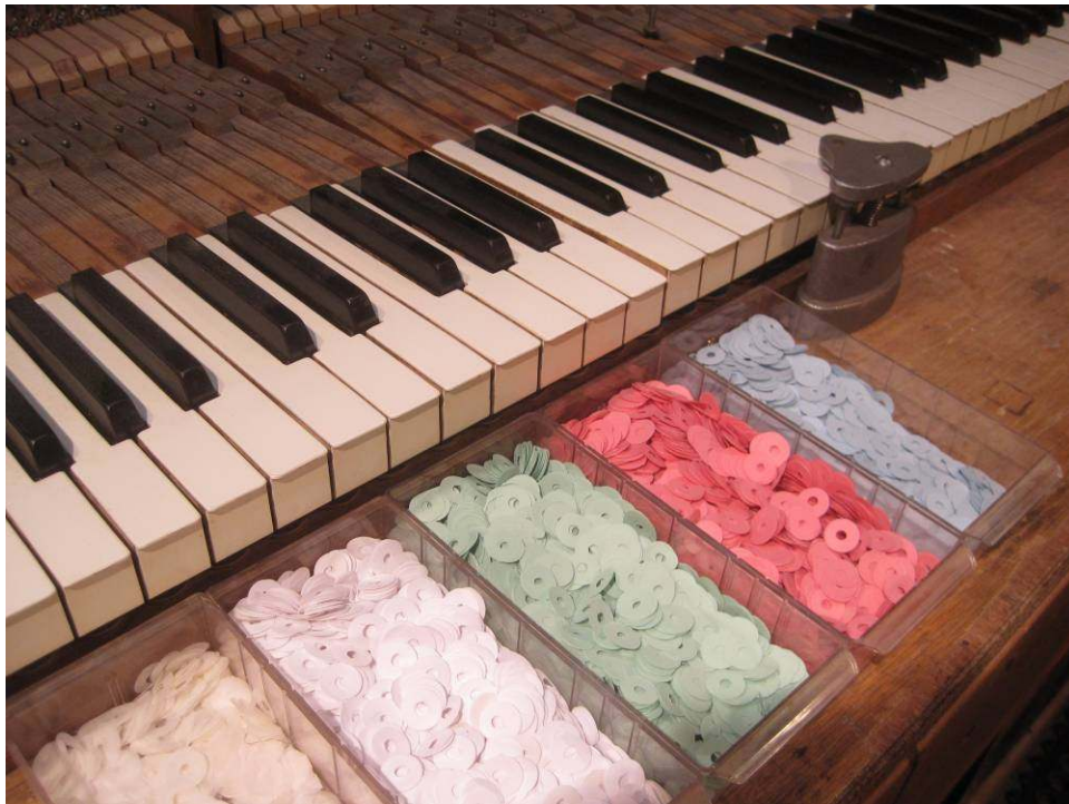
Photo 85: The polished keys are returned to the keybed. With the new balance rail felts installed, the keys need to be leveled. The naturals are done first . . .
