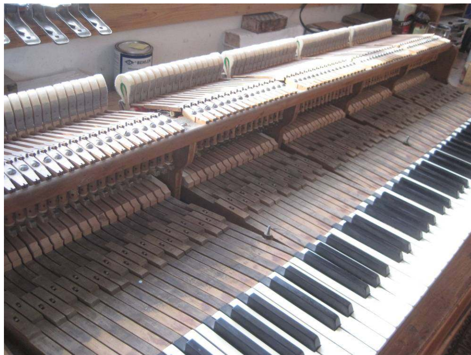
Photo 92: The action – now cleaned and regulated and ready to reinstall in the piano.
