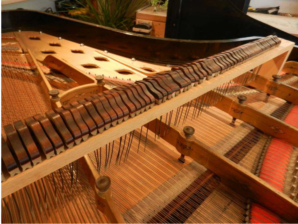
Photo 9: The dampers are stored for the time being on a special damper holder.
