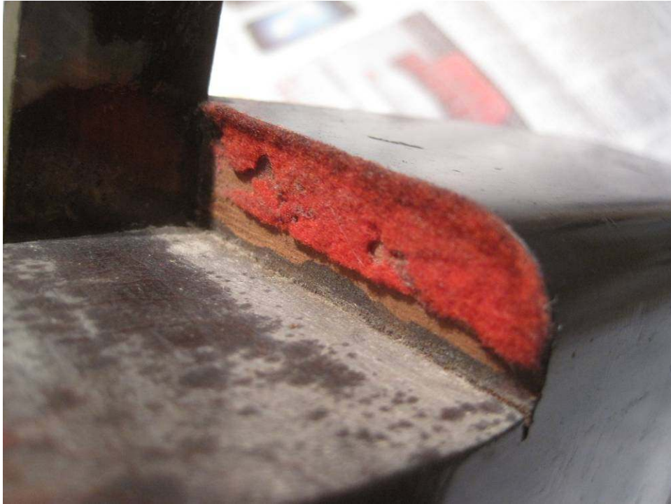
Photo 95: Worn and dirty felt on the case parts will be replace. This felt on the end block, for example, will be scraped off . . .
