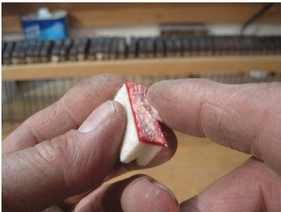
Photo 78: Titebond glue is applied. . .
