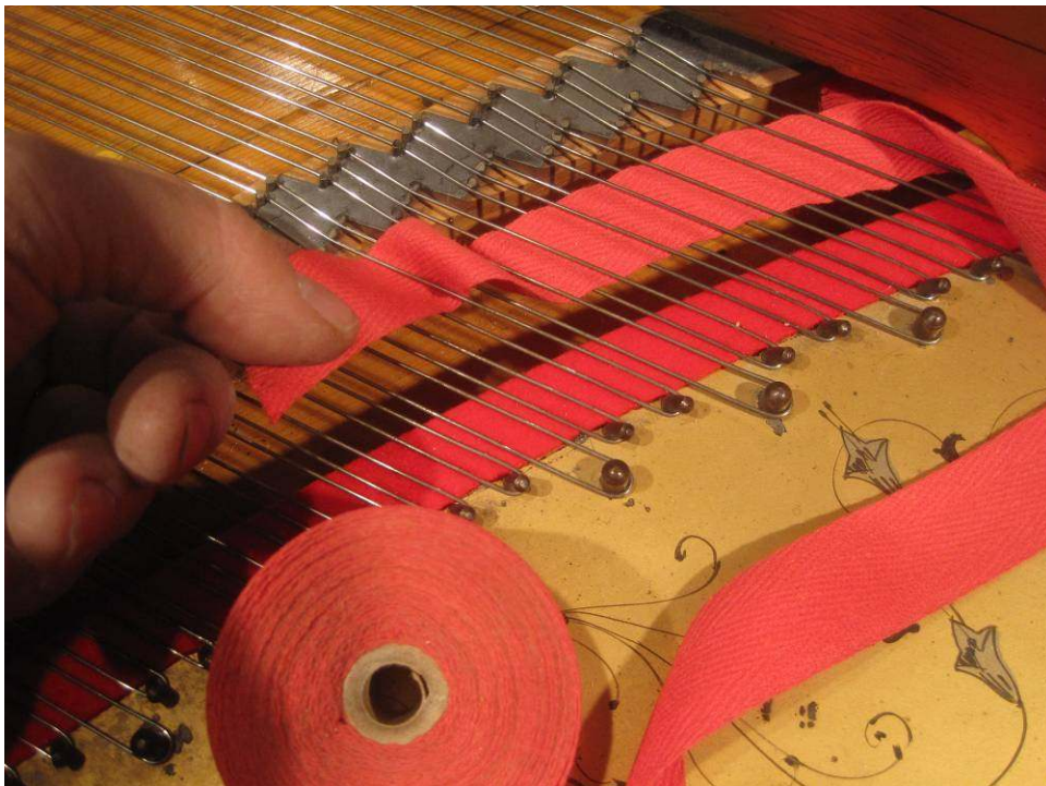
Photo 38: New understring felt is woven in.
