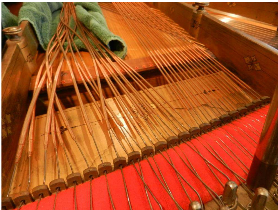
Photo 36: Bass strings, as they are being reattached and brought up to tension.
