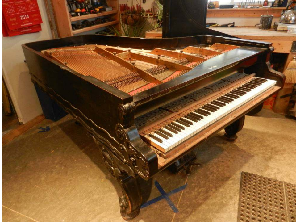
Photo 2: The first step was to disassemble the case. The lid, fallboard, end blocks, etc. were removed and stored on a piano parts dolly.
