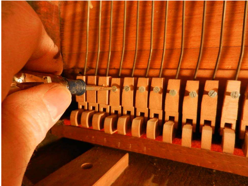
Photo 7: The damper set screws are loosened
