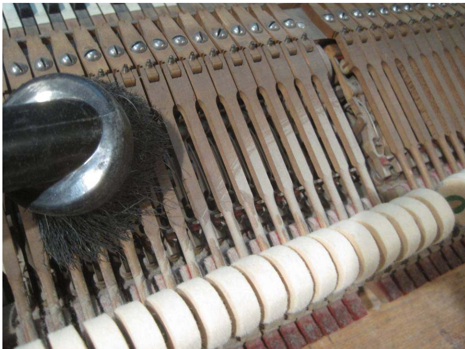
Photo 56: The old debris and new dust from filing is vacuumed up.
