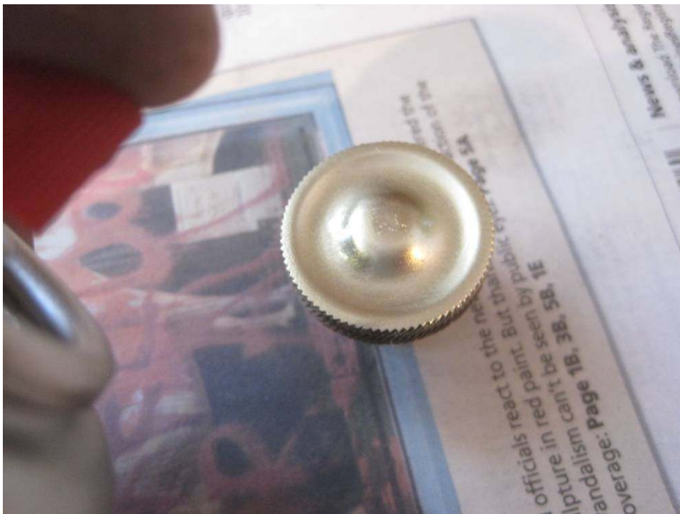
Photo 30: The polished brass is then sprayed with lacquer to prevent future corrosion, then replaced.
