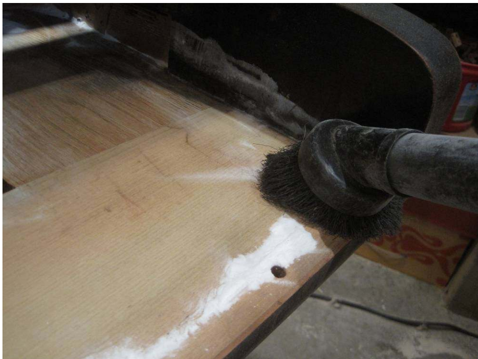
Photo 84: After brushing out the baking soda layering the keybed, it is also vacuumed and blown clean with compressed air.
