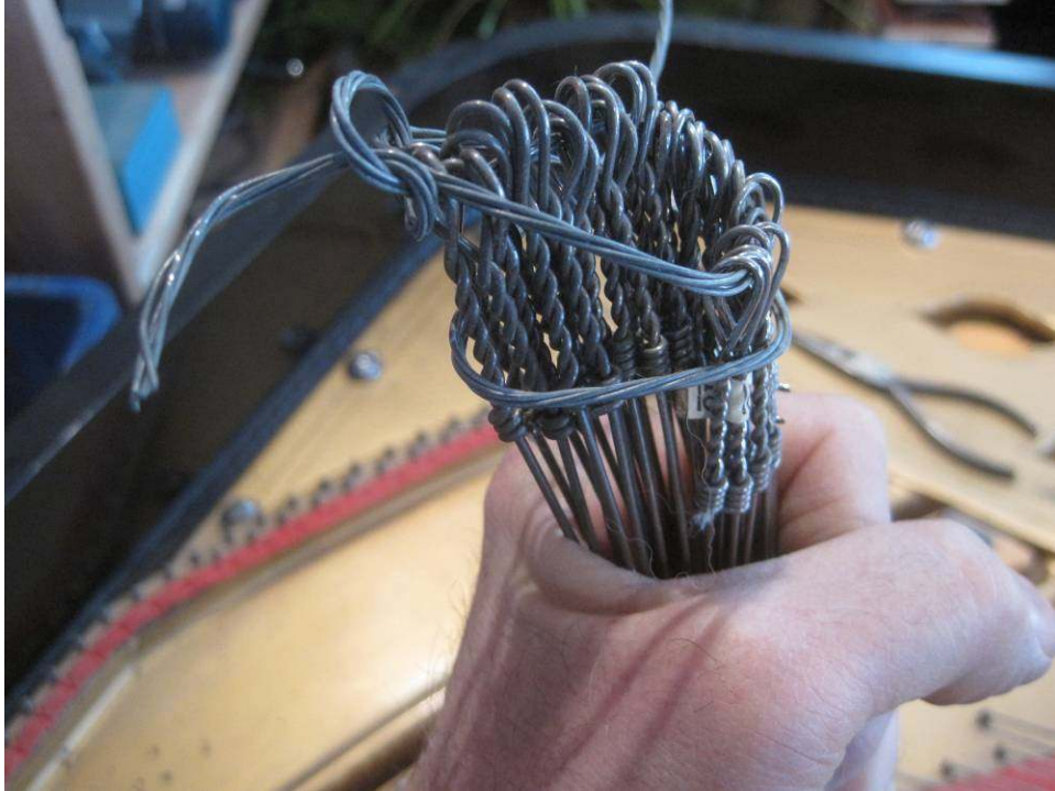
Photo 13: The bass strings are bundled together in correct order by running a wire through the hitch pin loops at the back of the strings.
