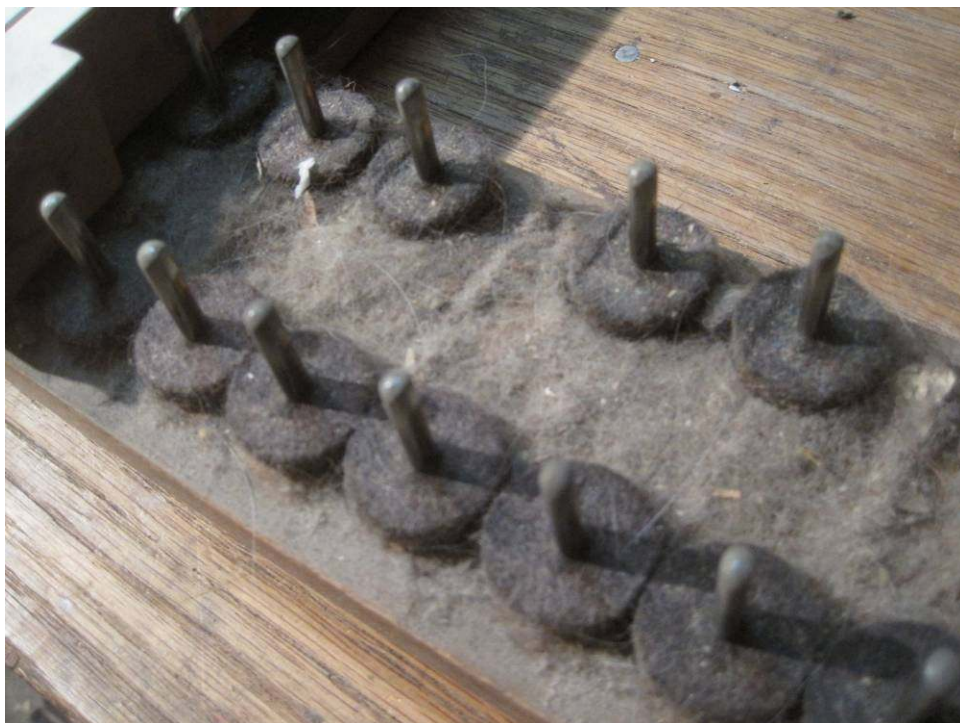
Photo 66: Obviously a problem area. Cleaning and felt replacement will make a big difference here.
