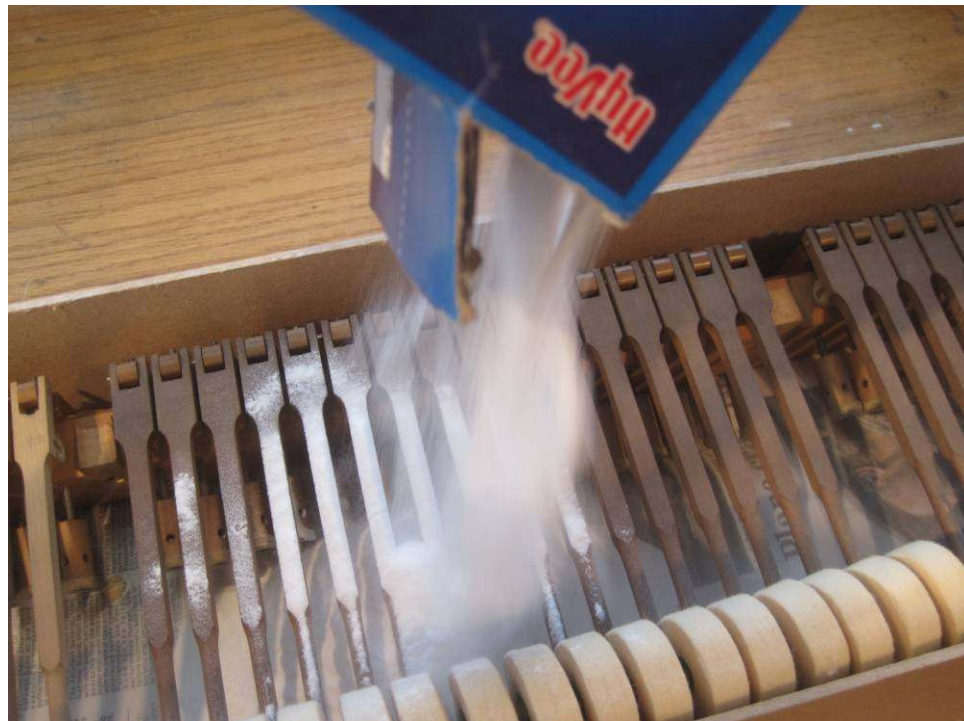
Photo 58: . . . and covered with baking soda.
