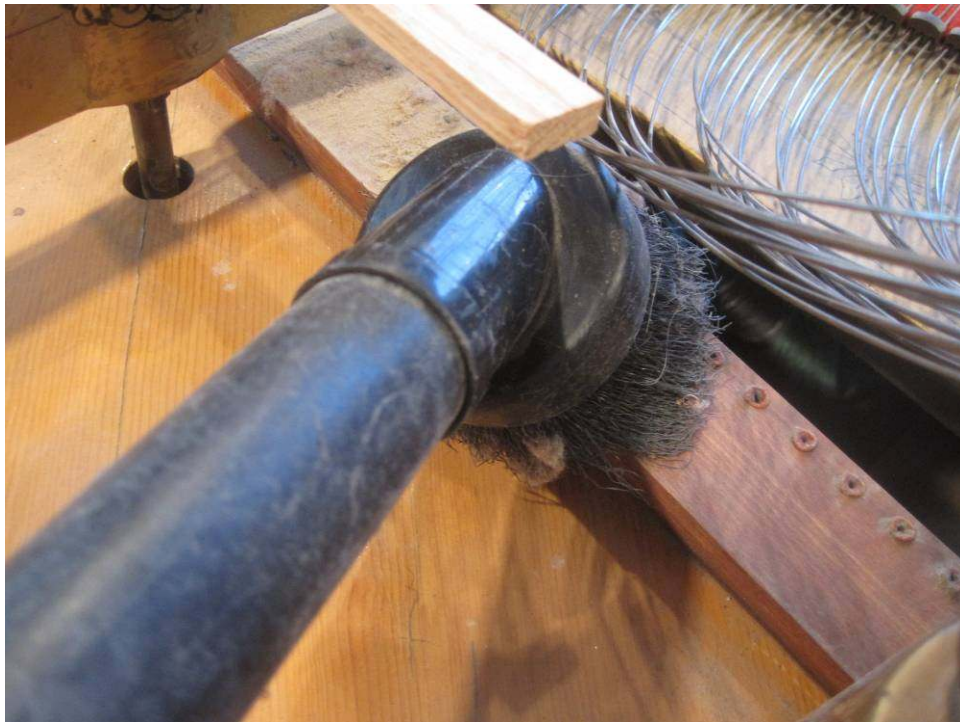
Photo 21: Loose dust is first vacuumed . . .
