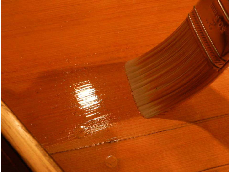
Photo 31: Before strings are put back on, the soundboard is coated with a sealing coat of shellac.
