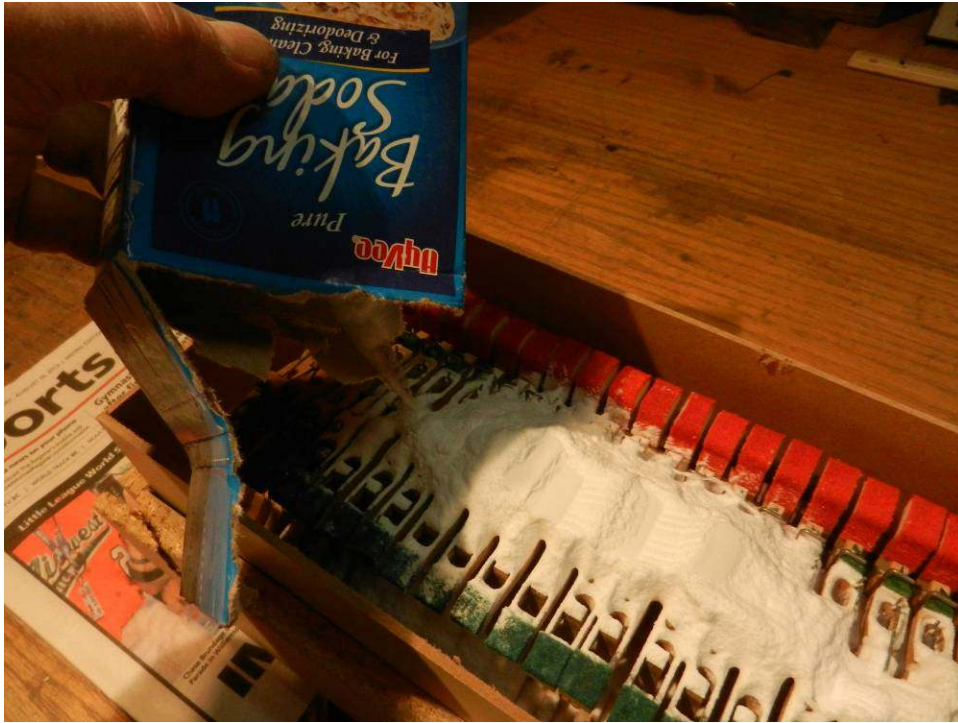
Photo 63: A slightly smaller custom box is made, another trip to HyVee for more baking soda (28 pounds), and the entire set is covered.
