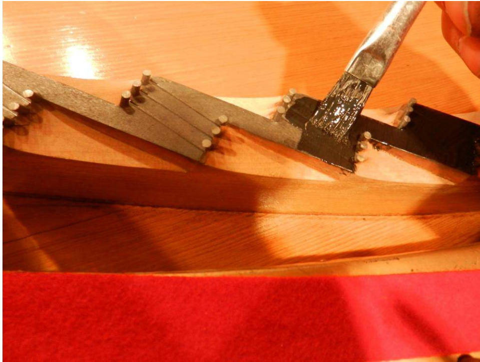
| Photo 33: The last step before restringing is to coat bridge surfaces with Dag ® , a lubricant especially designed for bridges and similar areas where friction must be kept to a minimum.
