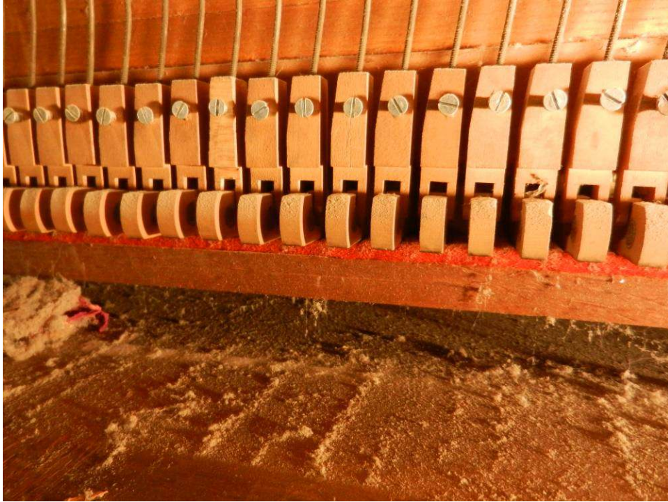
Photo 5: The piano action is removed to reveal the damper control mechanism (the back action) down below the level of the strings. Filthy conditions with debris that would also soak up odors would obviously need to be cleaned up.
