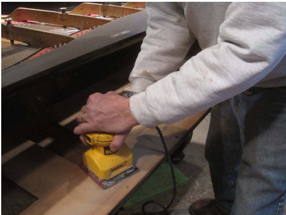
Photo 48: The clean-up of the keybed begins with a light sanding.
