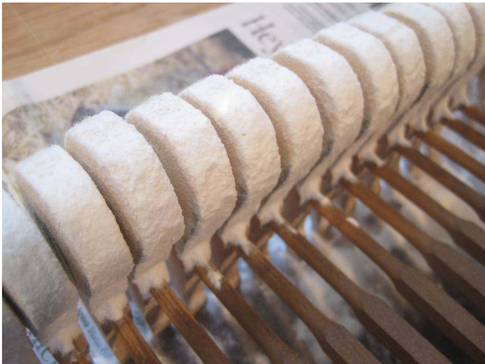
Photo 82: Time to unbury the hammers and wippen and clean off all the baking soda – along with any odors absorbed by the soda. Here are the hammers after removing them from the box they were in.
