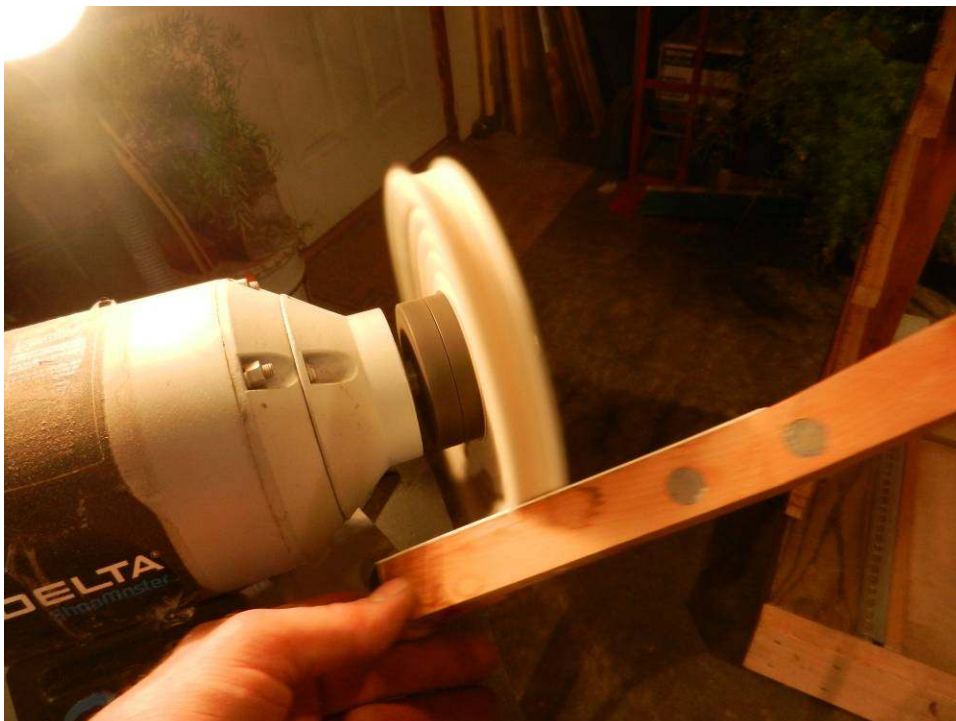
Photo 74: . . . then buffed with a cotton buffing wheel and a special polish (one for the white keys and another for the black).
