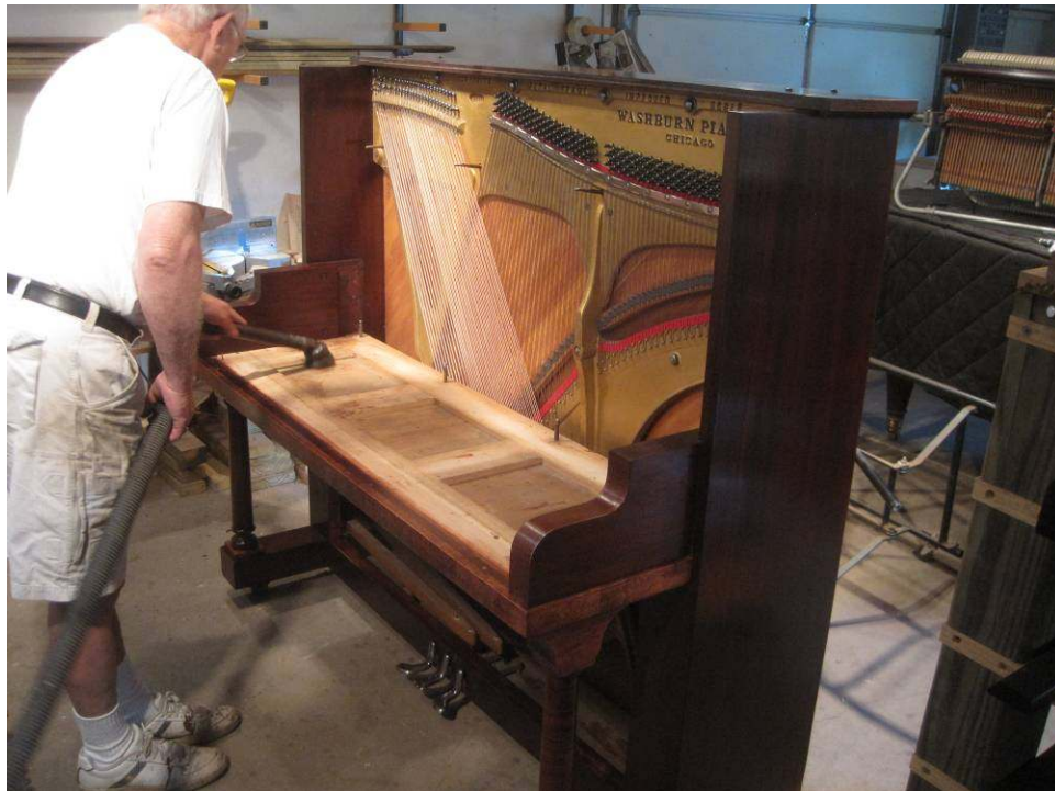
Photo 110: Dave vacuums up the keybed, in preparation for reinstallation of the keys.
