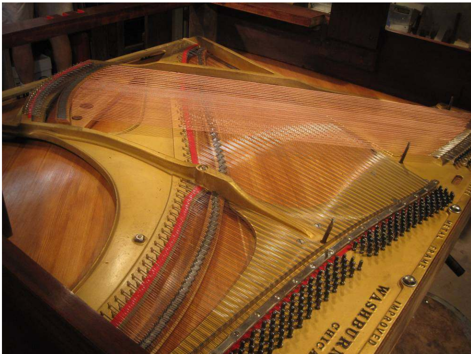
Photo 96: Newly strung piano seen from the top with 18 tons of tension now back on the plate.
