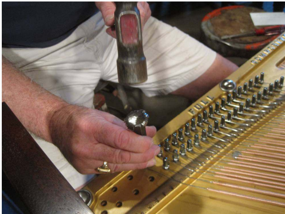
Photo 94: Each string is attached to a 2 1/2" long tuning pin which is pounded into the pinblock using a special pin punch. The string is then drawn up to an approximation of the correct tension.
