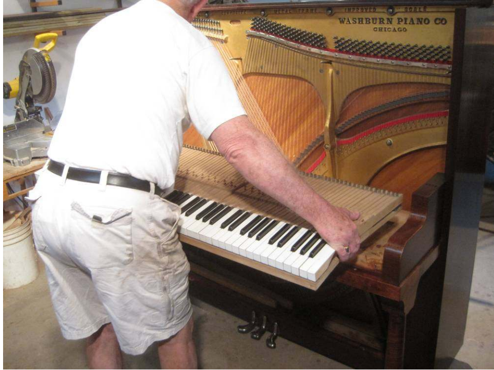
Photo 111: The keyframe with keys attached is reinstalled.
