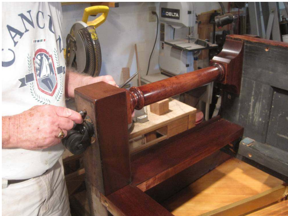
Photo 104: The pillar legs are screwed into place
