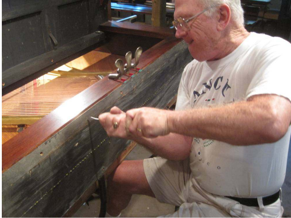
Photo 105: Dave screws the floor of the piano with pedals attached back onto the piano. The line of dried glue drops along the repaired seam will be chiseled off.
