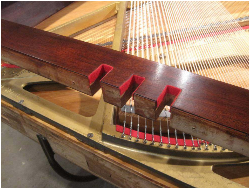
Photo 97: With the stringing done, the case may be reassembled. The first case part to go back into place is the toe rail, with newly refelted slots for the pedals.
