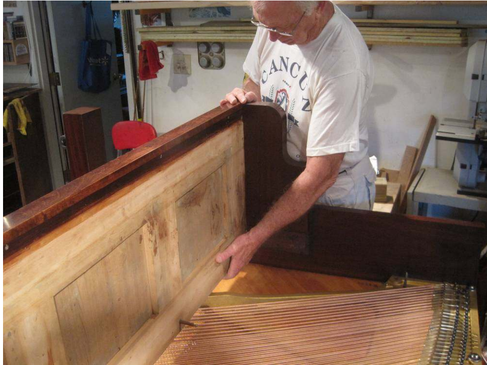
Photo 101: The keybed is returned to the piano.
