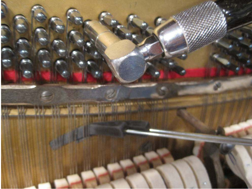
Photo 119: The first tuning is done with at least three more to follow.
