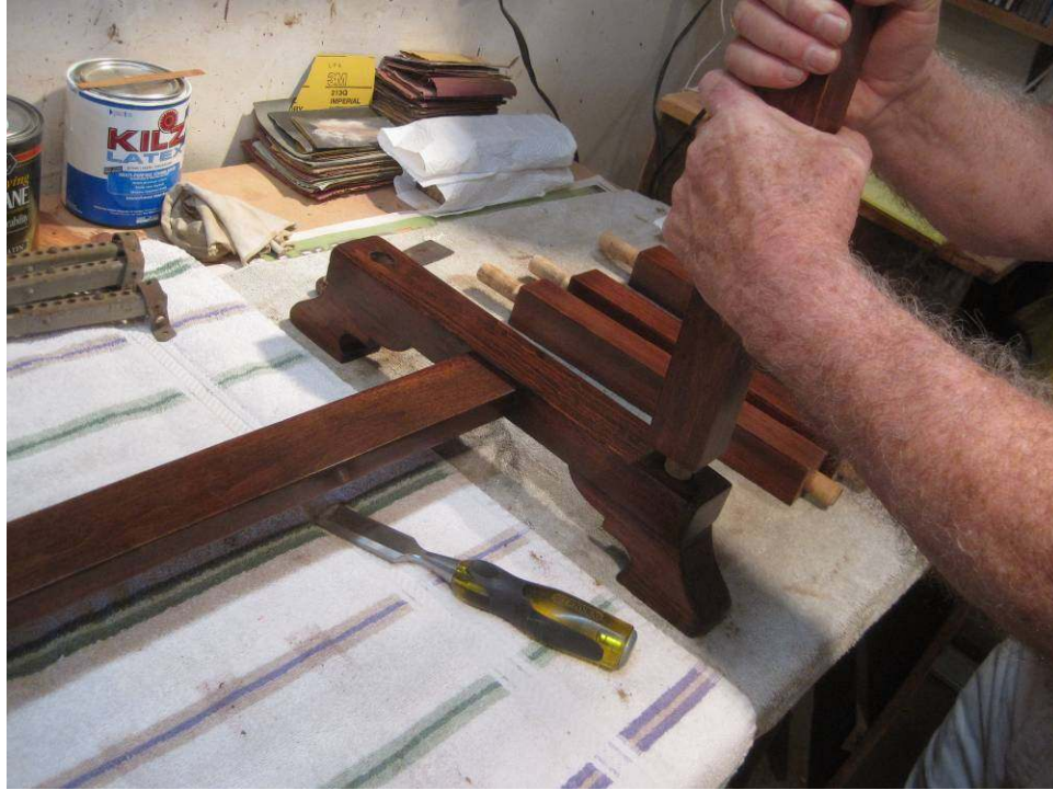
Photo 99: With the glue curing on the floor repair, Dave turns his attention to the bench. The bench had been disassembled before refinishing. Here the legs are glued in place into the base.
