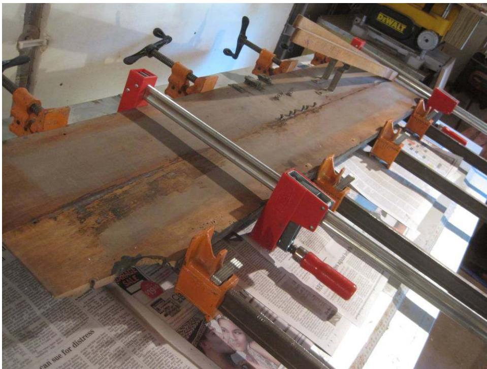
Photo 98: The floor of the piano needed repair before returning to the piano. The two boards of the floor had split apart and needed to be reglued.
