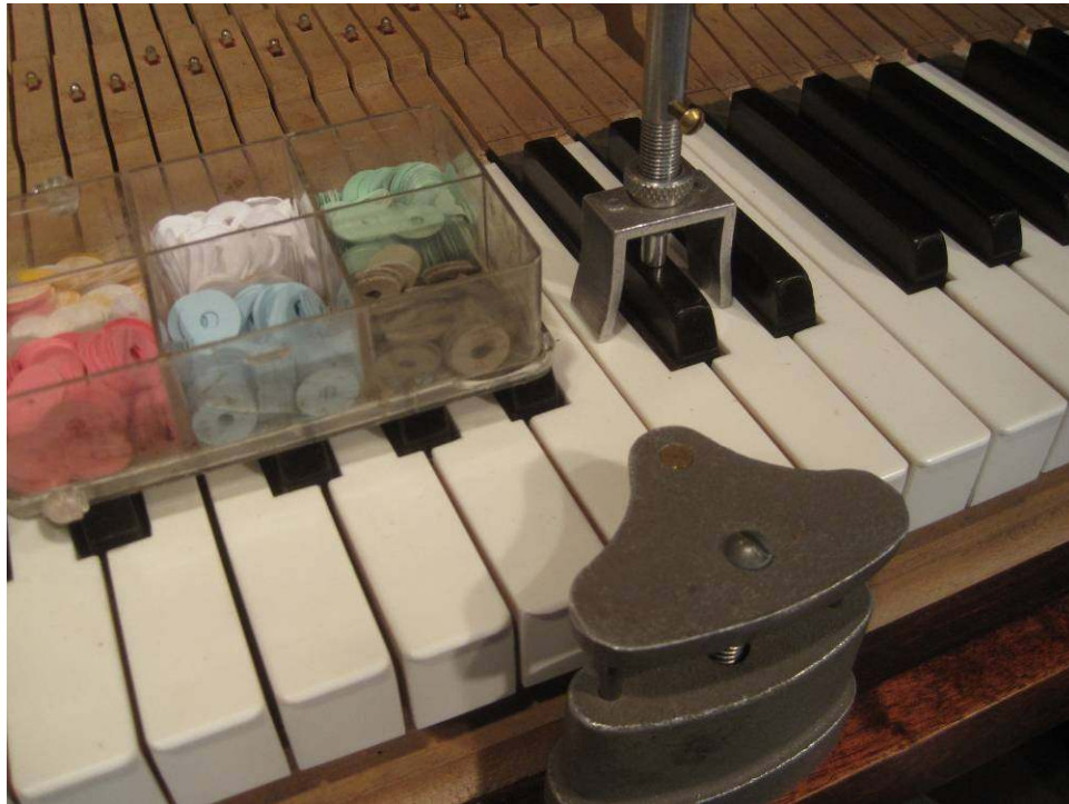
Photo 115: The keys, both naturals and sharps, are leveled.
