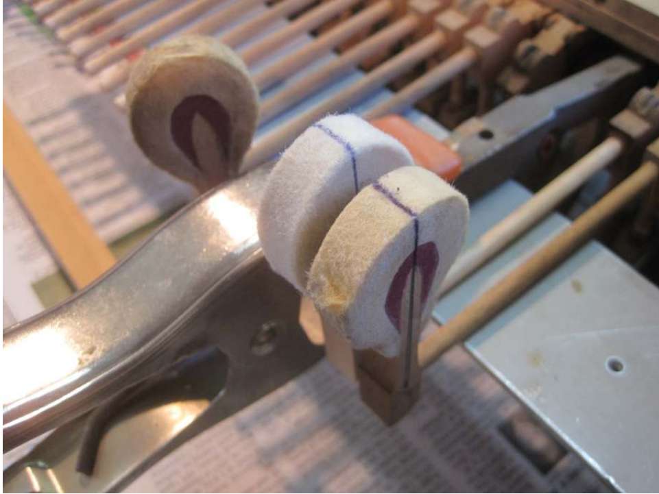
Photo 60: The action is laid on its back on the bench (to make squaring up the hammers easier) and the process begins. The first step is to match the strike line of the new hammers and match with that of the old hammers.
