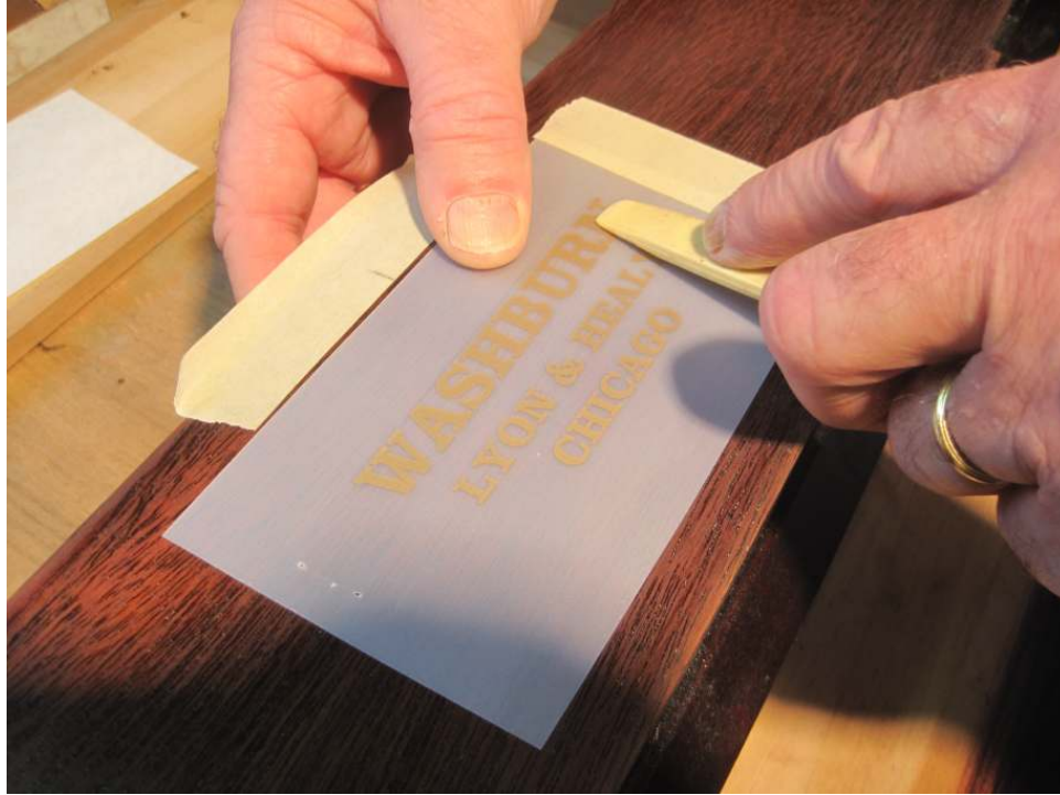
Photo 86: Dave uses a burnishing tool to transfer the lettering to the surface of the fallboard. This is done in between varnish coats so that the lettering is sandwiched in between layers of finish.
