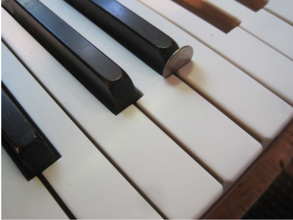
Photo 52: When correctly done, the distance between the notch and the front of the sharps is equal to the width of a dime. .
