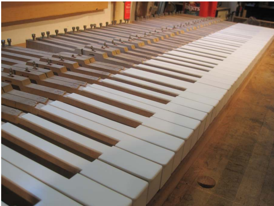
Photo 53: The entire set of new keytops, installed, filed and buffed.
