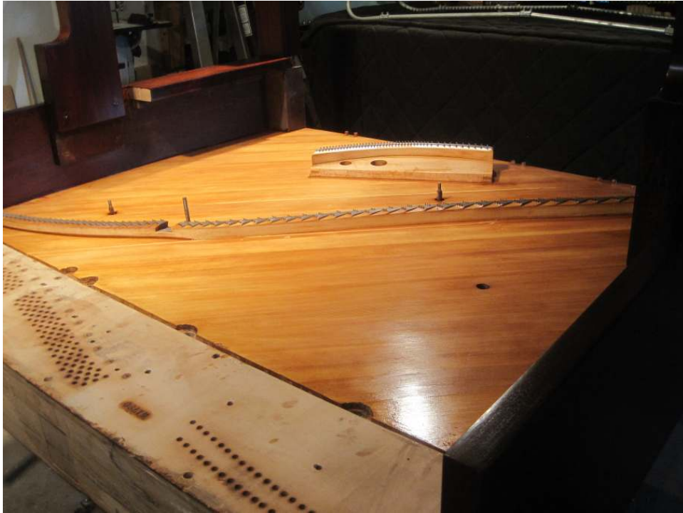
Photo 84: The finished soundboard. It has a very nice resonance to it – thump it and it vibrates for a long time – a very good sign!
