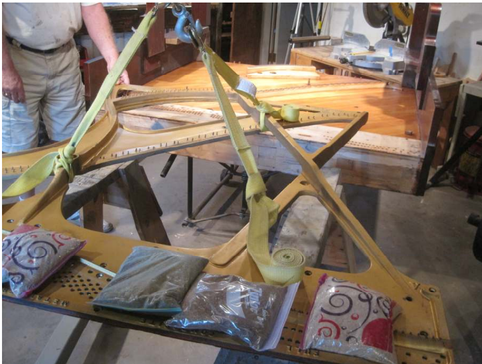
Photo 91: The plate is lifted off the sawhorses with bags of sand on one end to balance it and keep it level. The sawhorses will be pulled free, and the piano rolled under the plate. Three bolts must be aligned before it is lowered into place.
