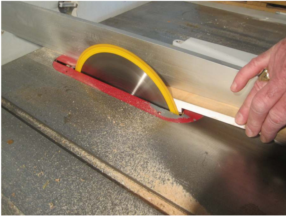
Photo 44: During times that a finish coat is drying, Dave turns his attention to the keytops. After removing the old ivory tops for safekeeping, Dave runs the keysticks through the table saw to shave off a bit of the wood to allow for the new, thicker tops, and to provide a consistently level surface for the new keytop material.
