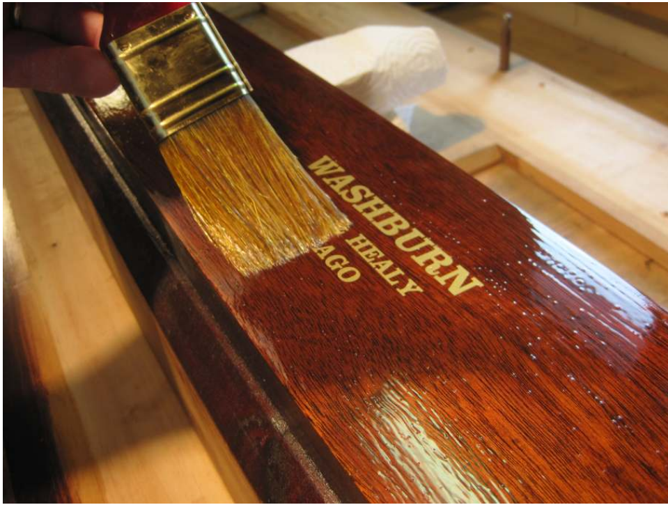
Photo 88: The first of several more coats of polyurethane is applied.
