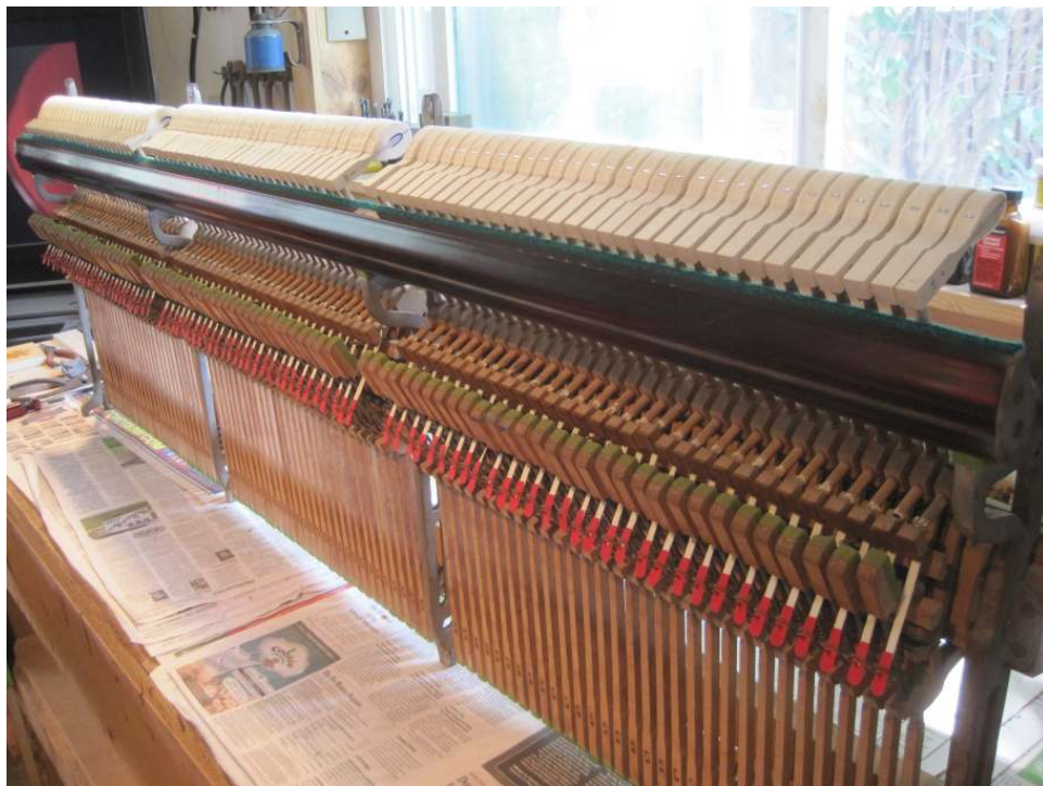
Photo 77: Except for the dampers, the restoration of the action is complete, and it's ready for reinstallation in the piano, once the piano is ready for it.
