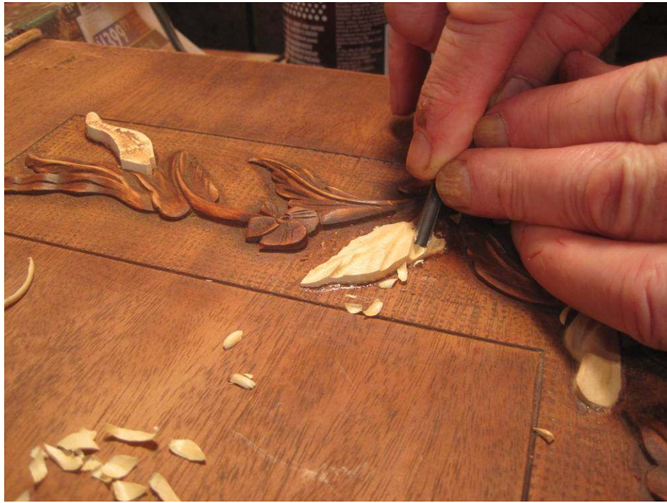
Photo 32: Before staining and varnishing the case, some missing carving must be replaced. Here Dave finishes the detail of a leaf to replace one that was missing.
