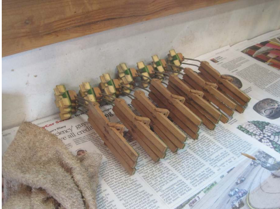
Photo 59: The dampers must also be taken off. Here, the bass dampers have been removed, numbered and stacked up out of the way.
