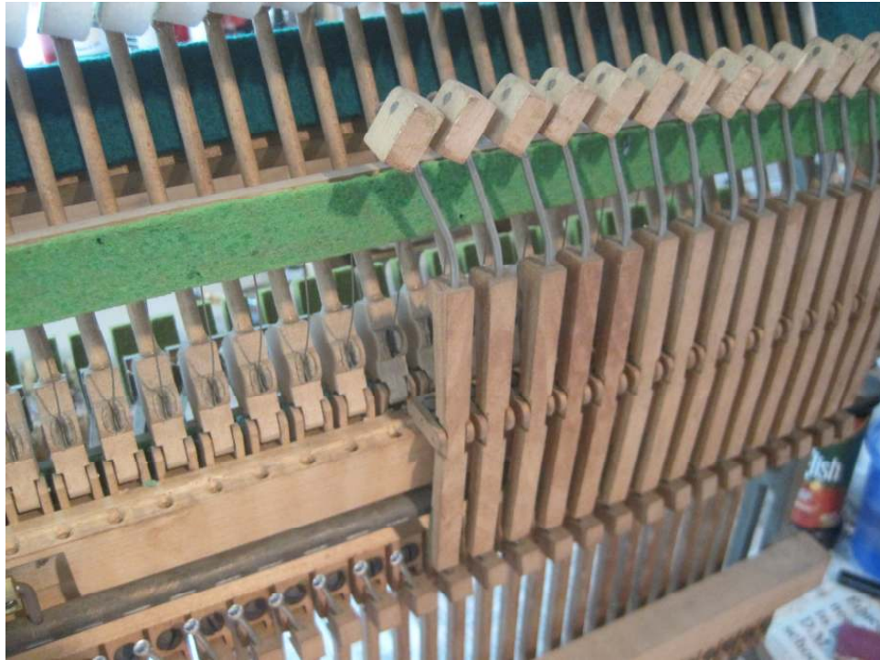
Photo 74: The damper levers are returned to the action. The new felts will be glued in place with the action in the piano so that they may be precisely fitted to the strings.
