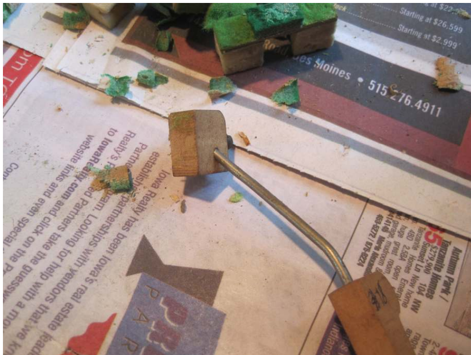
Photo 73: Damper head with felt scraped off.
