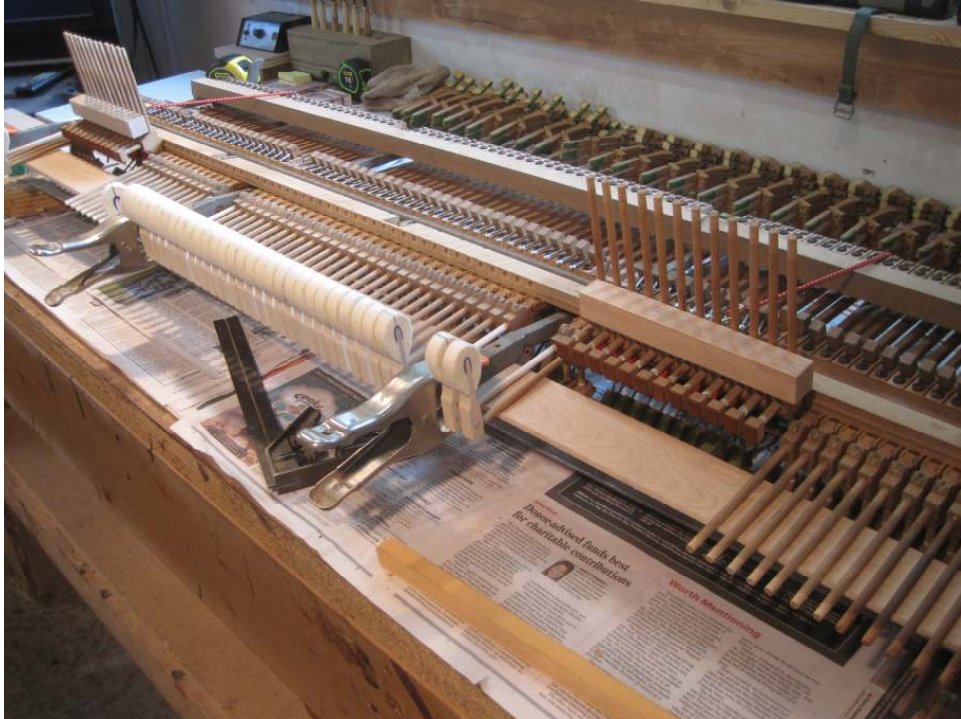
Photo 65: This photo shows the project in process. The middle section of hammers have been completed, and I'm just beginning work on the treble section. The red bungee cords keep the adjacent hammers up and out of the way to make gluing the hammer being worked on easier.
