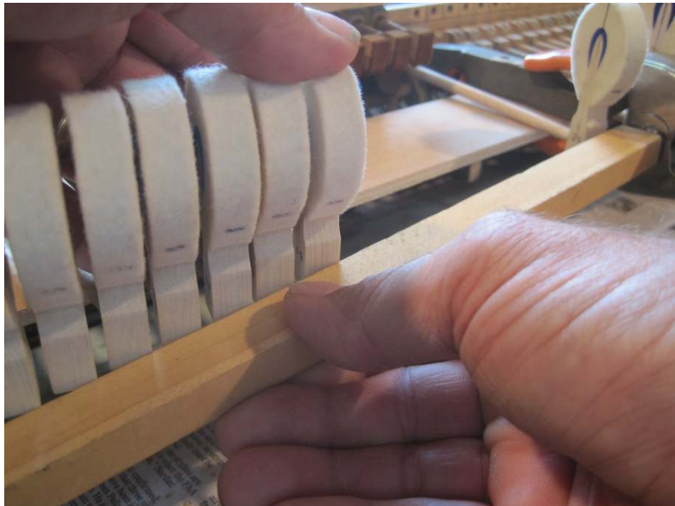
Photo 63: Using the end hammers of the section for reference, the in between hammers are checked with a straight edge for an even line.
