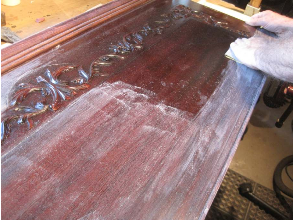
Photo 40: Buffing between coats is done with 400 grit wet/dry paper.
