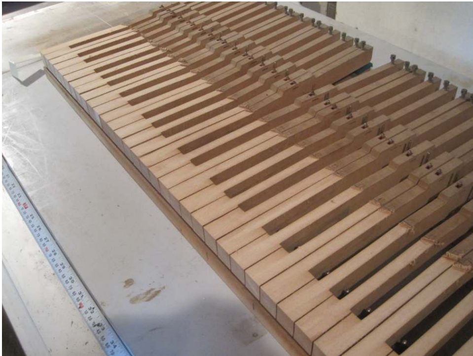
Photo 45: The keys on the keyframe ready for the installation of new keytops.
