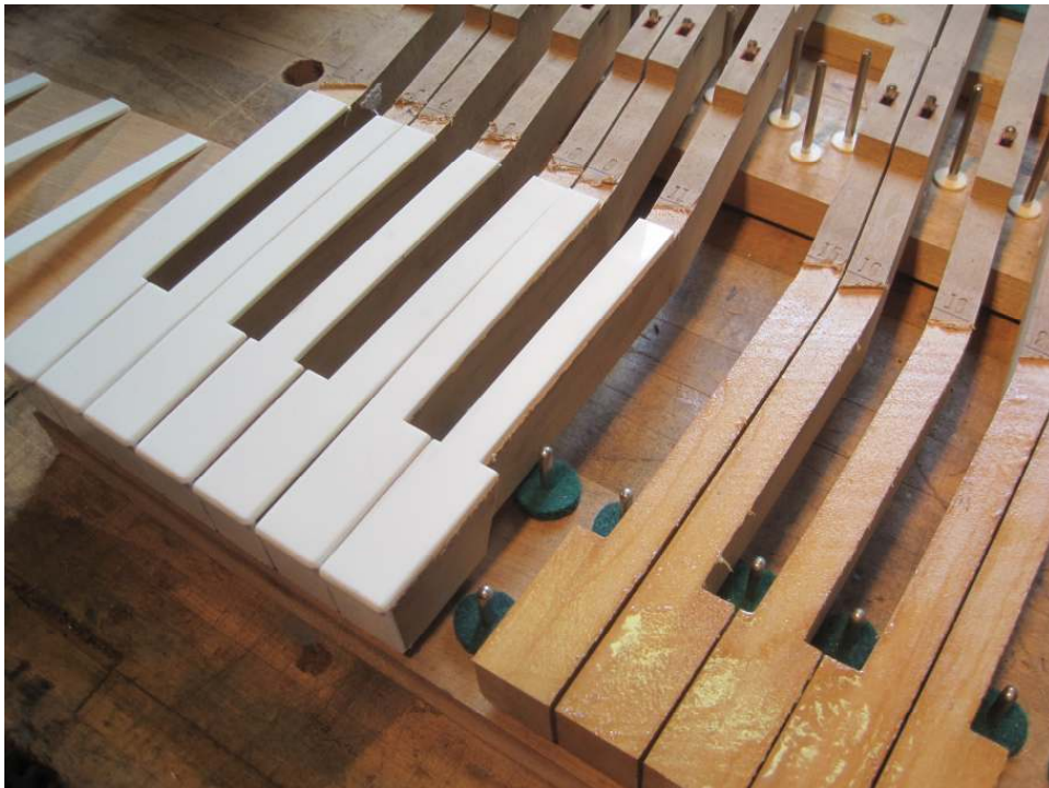
Photo 47: The first octave of keytops glued in place.
