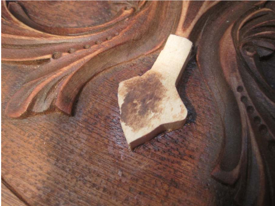
Photo 34: The first step is to cut the shape from basswood stock and glue it down to the background.
