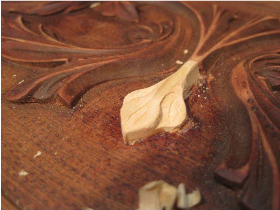
Photo 36: The finished leaves, with veins scribed in, will blend in once stained and varnished to the point where it will be nearly impossible to distinguish the new from the old.
