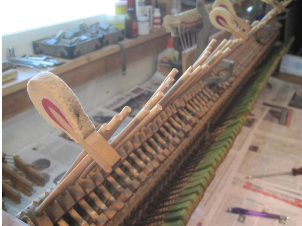
Photo 58: Before hammer replacement can begin, a few more things must be removed from the action to allow access. The hammer rest rail is first taken off, which accounts for the uneven line of hammer shanks in this photo.
