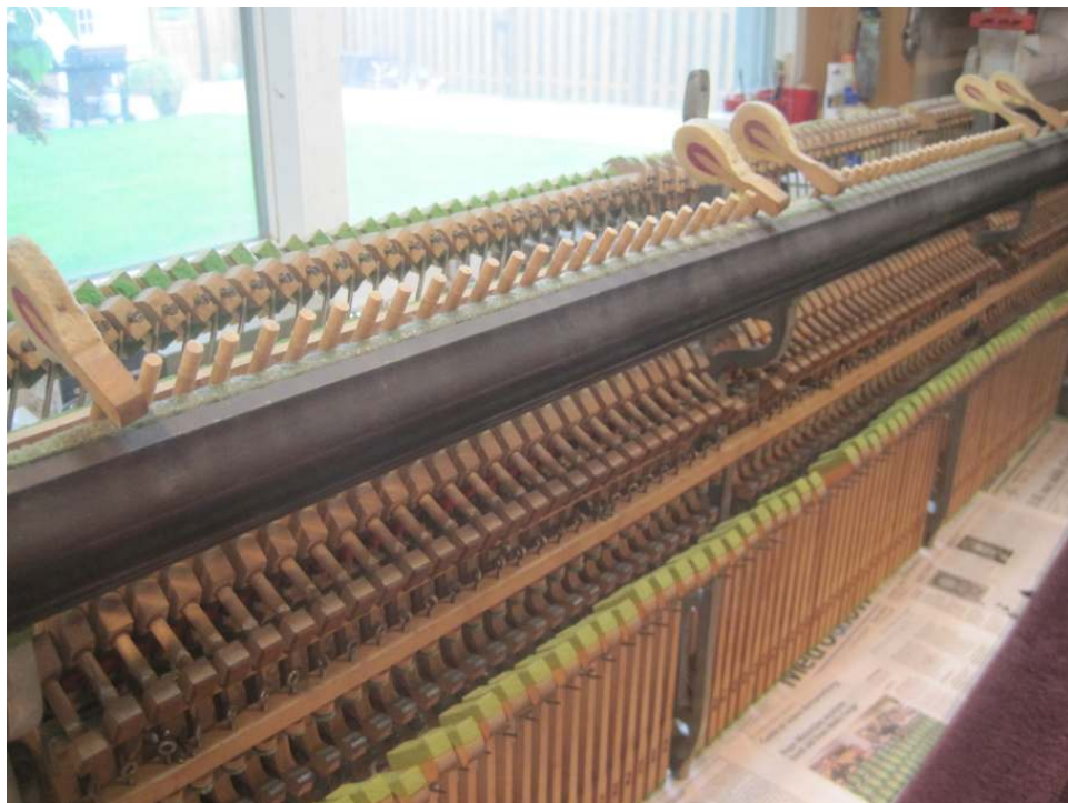
Photo 57: The only original hammers left are ones intentionally left at the end of each section to serve as guides for the new parts.
