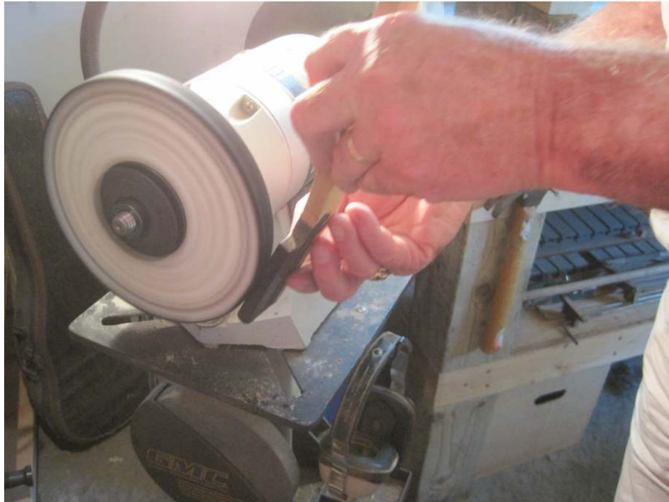
Photo 54: The original ebony sharp keys are buffed using a buffing wheel and a special ebony polish
