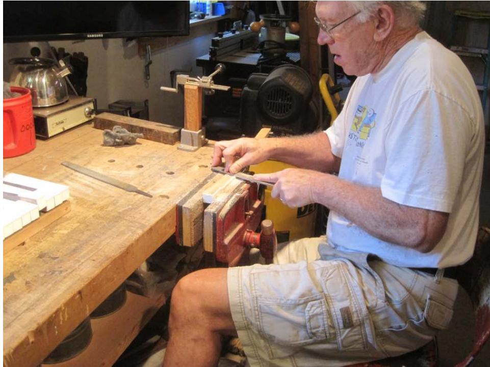
Photo 48: Dave files the sides of the new tops. The keytop material is slightly oversized, and must be filed flush with the sides of the keysticks.
