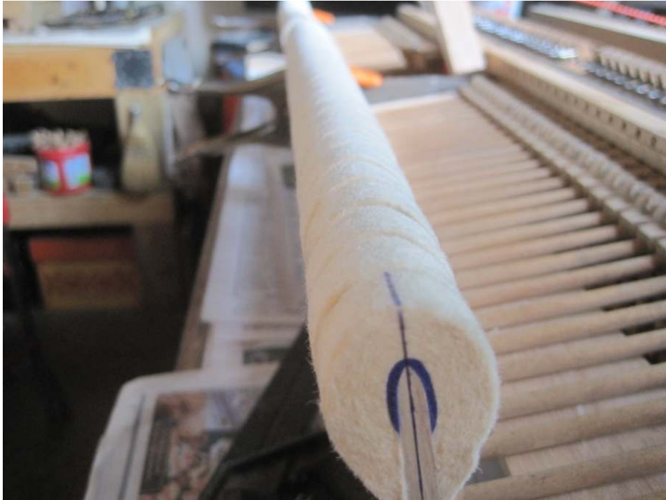
Photo 64: Done correctly, the hammer line should be perfectly straight.
