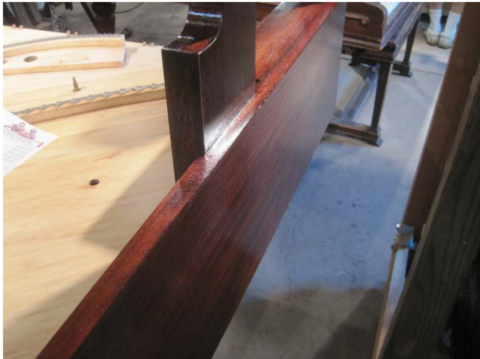
Photo 39: The side and arm of the case with one coat of finish. This first coat will be rough to the touch when dry and will need to be buffed before the second coat is applied.
