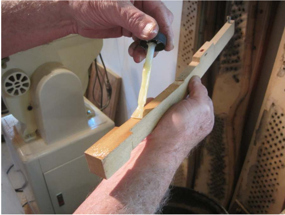
Photo 46: Dave applies a coat of contact cement to the keystick. The wooden surface will receive two coats of cement (to allow for absorption), and the keytop itself will be coated once.
