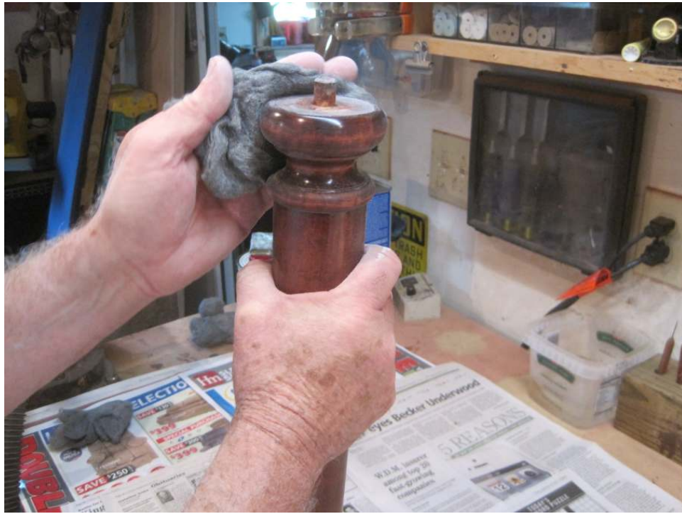
Photo 78: Back in the main room, Dave continues work on the case. Here he buffs the 3 rd coat of finish on a leg – the beauty of the new finish is starting to show!
