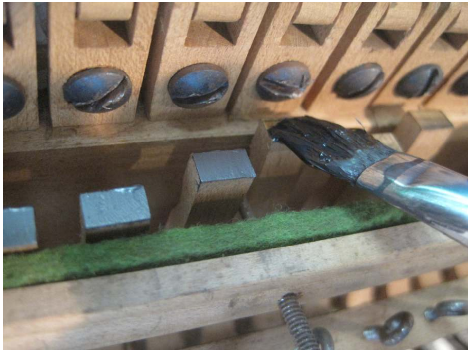
Photo 75: Another important detail is attended to – the tops and heels of the jacks are painted with DAG – a specialized lubricant to make wood to leather contact points more slippery.
