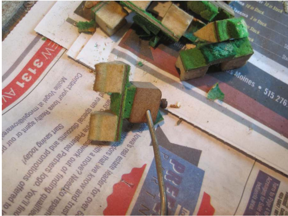
Photo 72: New damper felts are to be installed. The old dampers are removed, but the wooden damper heads and levers are reused.
