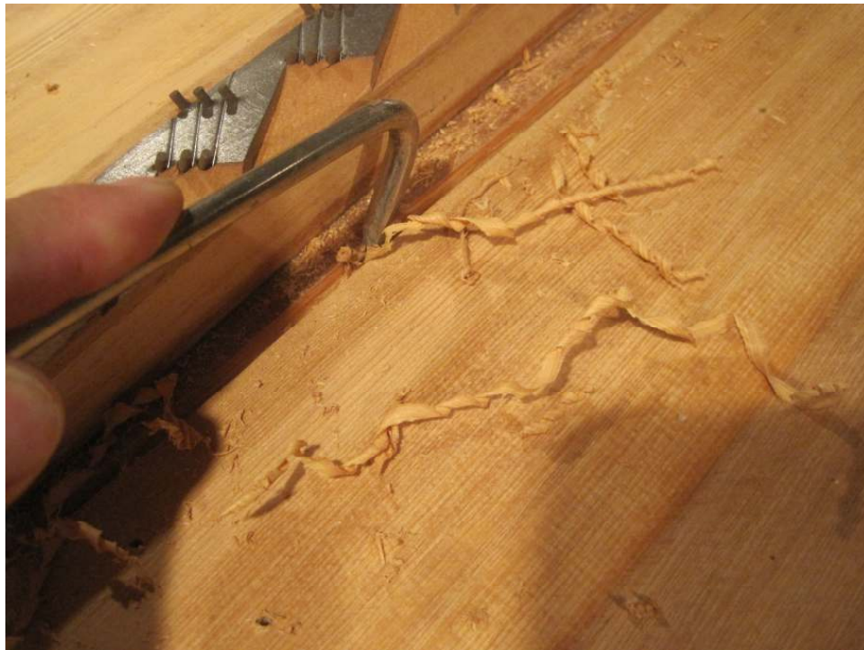
Photo 79: While Dave is finishing up work on the case, I turn my attention to the soundboard while Dave finishes up work on the case. The soundboard has been dried, revealing 3 cracks. Here, I use a v-gouge to open up a crack running next to the treble bridge.
