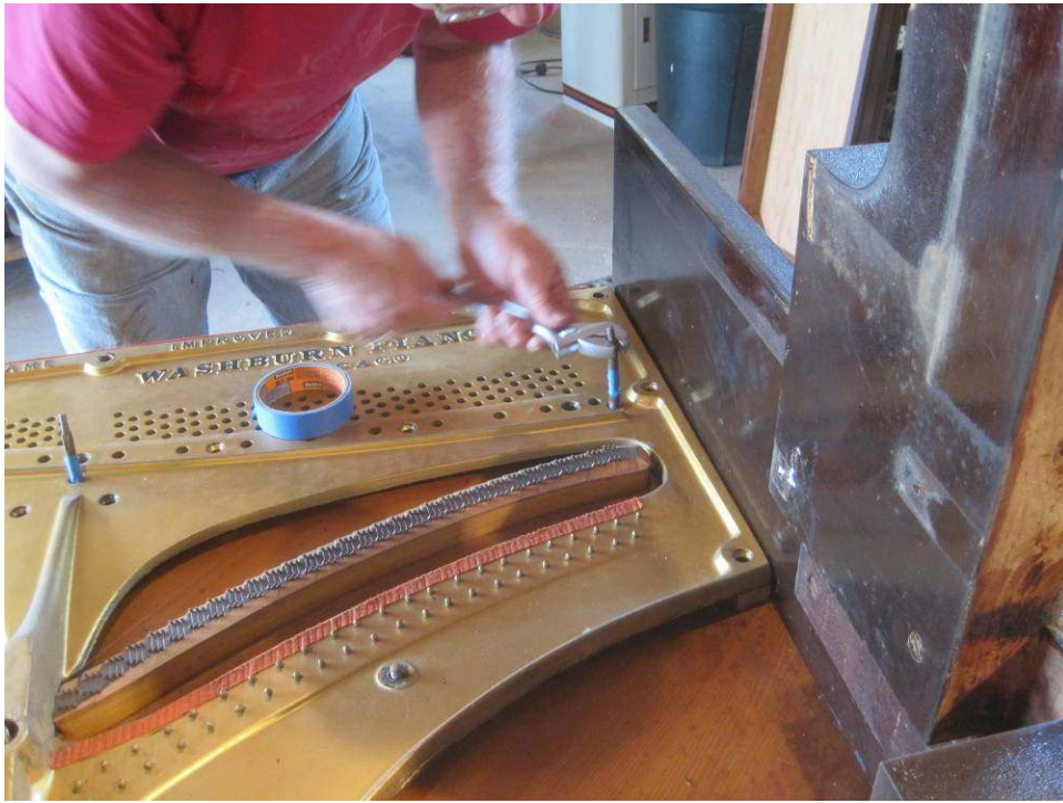
Photo 13: Dave removes all bolts and nuts holding the plate to the piano.
