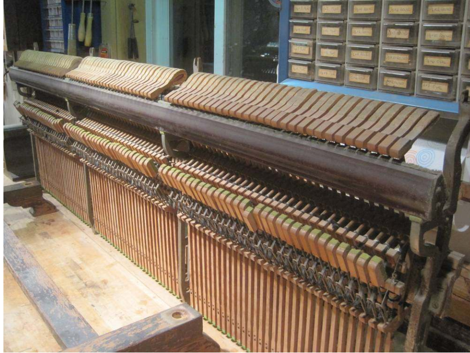
Photo 6: The action is also removed from the case and placed on a bench for servicing.
