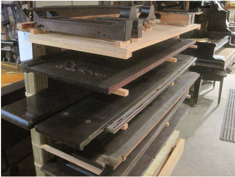
Photo 5: The first step is to disassemble the case with all removable parts stored on a parts trolley. This makes the refinishing process much more efficient.
