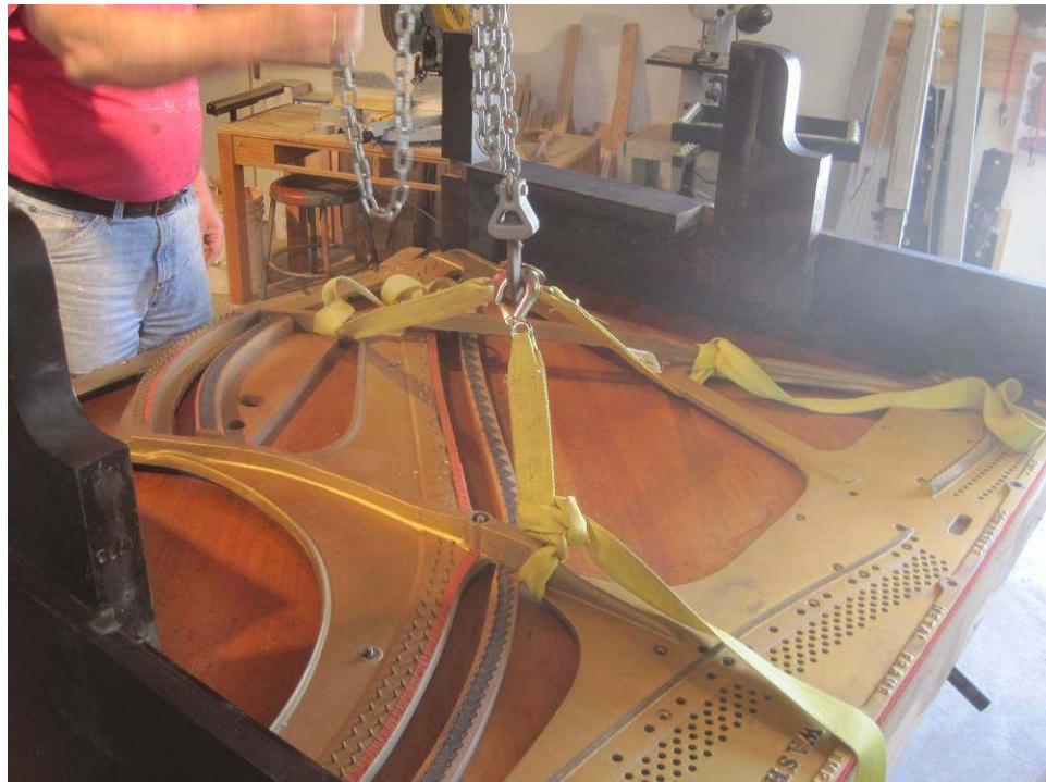
Photo 14: The plate is attached to our hoist. Canvas straps instead of chains lessen the chance of damage to the finish of the plate.
