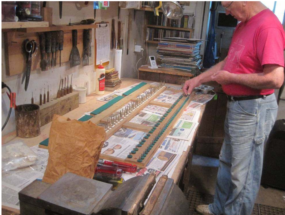
Photo 20: All the old felt is removed and replaced with new. The next step for the keys will be to remove the old ivory and replace the keytops, but that will have to wait for awhile.
