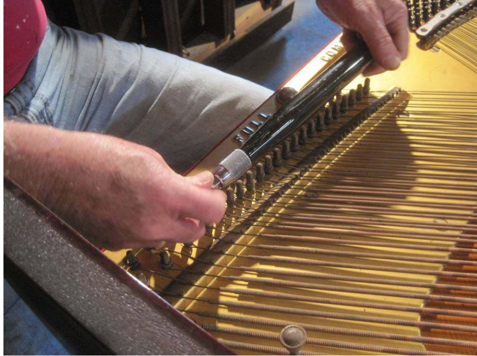
Photo 9: Dave now lets off the tension from all the strings in preparation for removing them.
