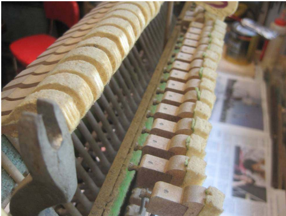
Photo 22: Replacing the hammers will be my first order of business. Like the bass strings, the hammers vary from piano to piano, and must be duplicated.
