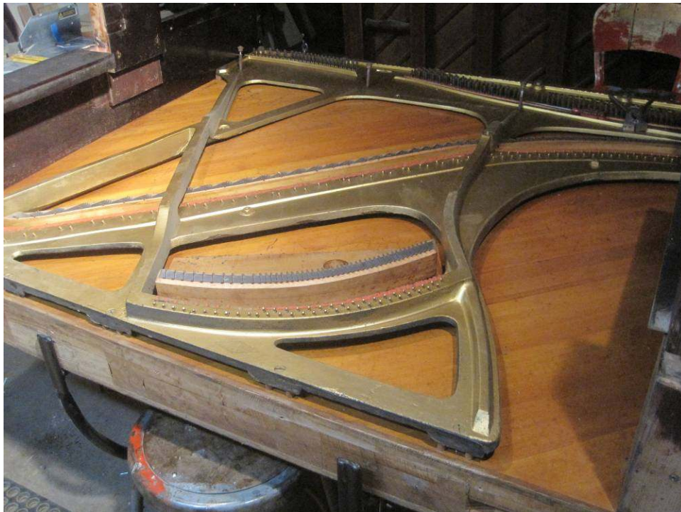
Photo 12: The piano without strings. The last part left to remove is the cast iron plate. This is necessary in order to repair and refinish the soundboard.
