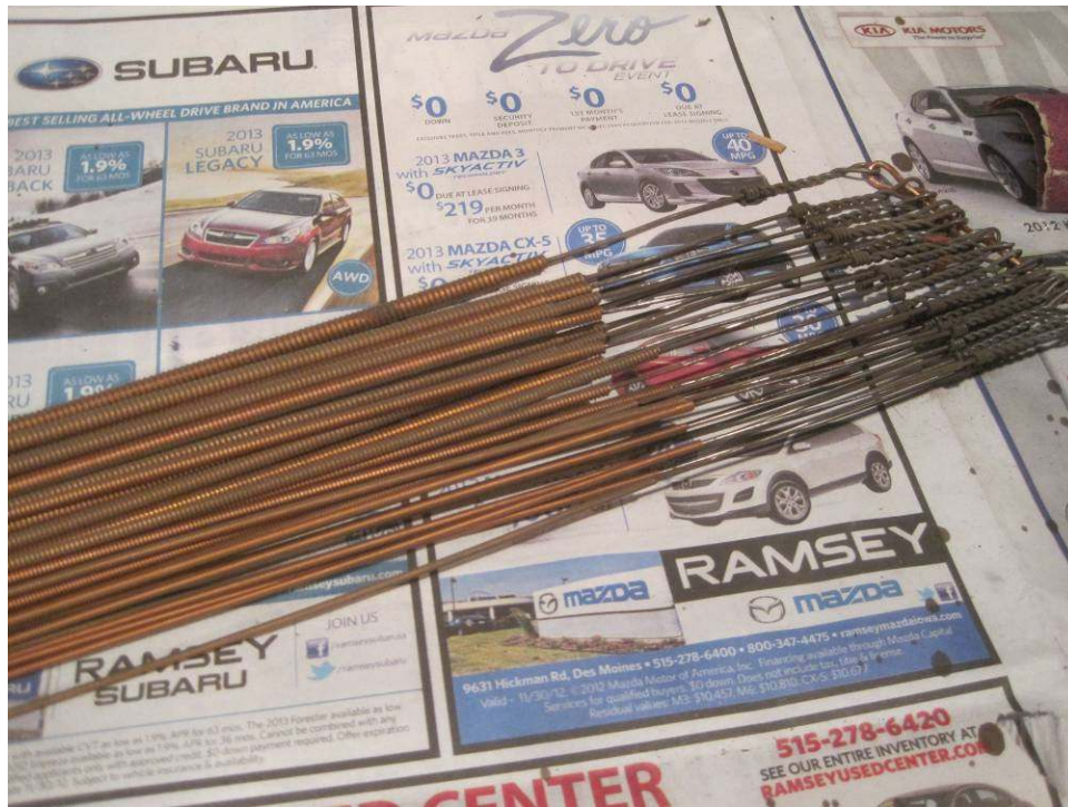
Photo 11: The bass strings are bundled together and sent off to Schaff Piano Supply to be duplicated. The size and length of strings differ from piano to piano, making exact duplication necessary.
