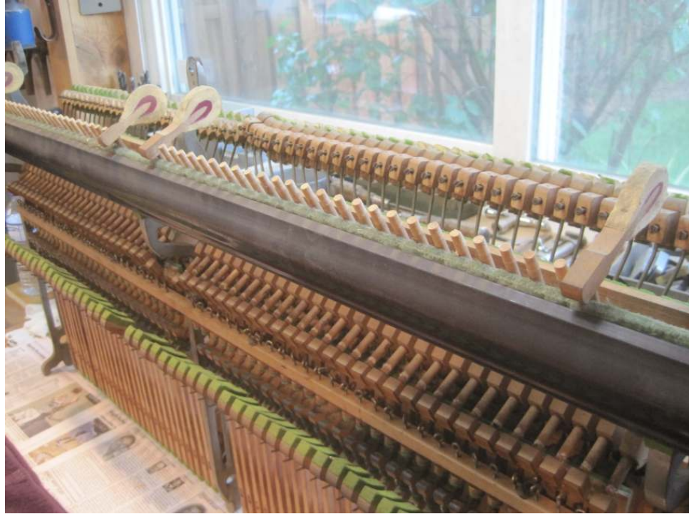
Photo 27: The action with hammers (with the exception of the guide hammers) and bridle straps removed.
