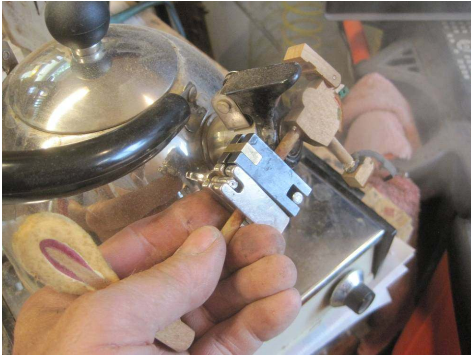
Photo 23: The end hammer assembly from each section is removed and the hammer butt steamed off of the shank. These 6 hammers / shanks will be sent off to Schaff for duplication of the entire set.
