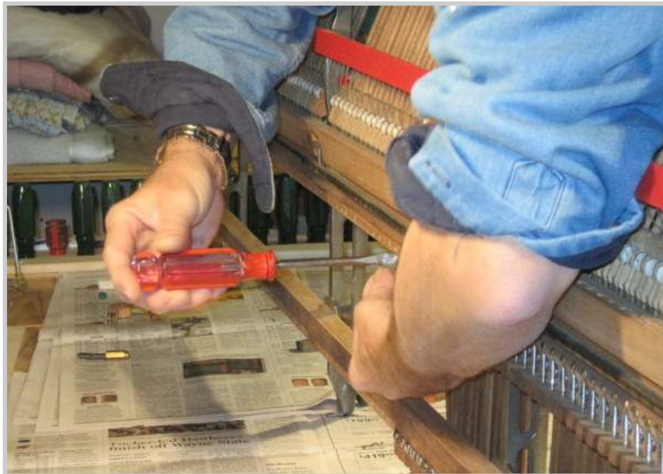
Photo 433: Leaning over the top of the action to start the screw for the whippen flange works well.
