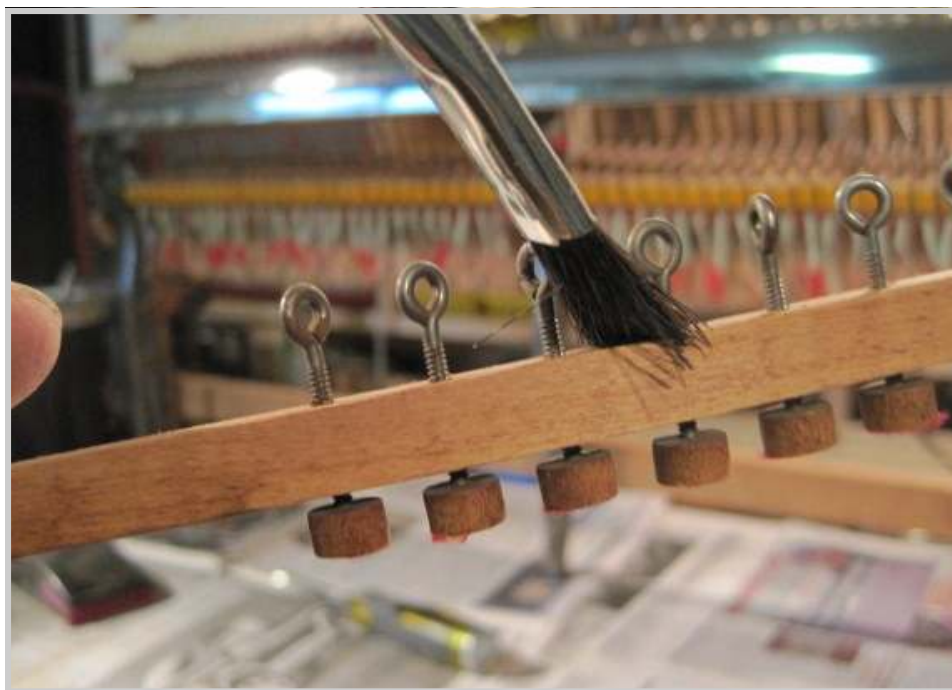
Photo 426: Once the punchings are removed, the rail itself is cleaned with a stiff brush.
