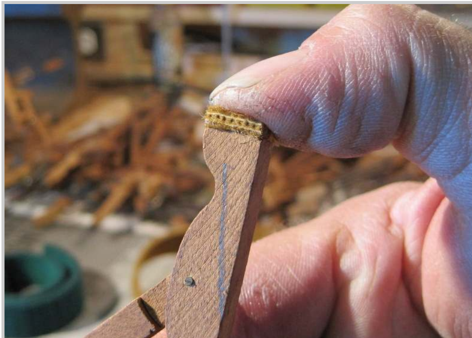
Photo 423: A square of sticker cloth is glued with hot glue to the bottom of the sticker. This is the contact point between the brass capstan at the back of the key and the whippen.
