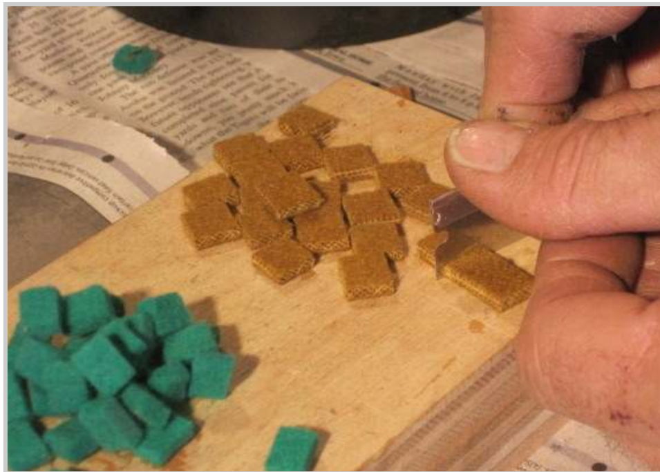
Photo 422: The last two pieces of felt are made ready. The brown sticker cloth is razor cut from a long roll. The hammer butt felts for the topside of the jacks comes precut.
