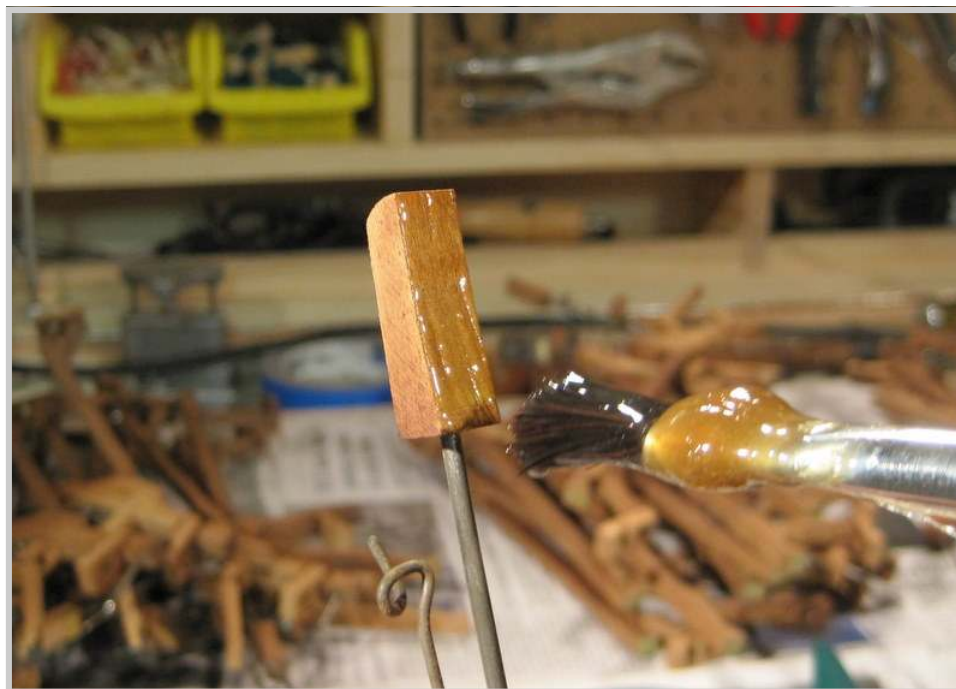
Photo 418: Each backcheck is coated with hot glue.
