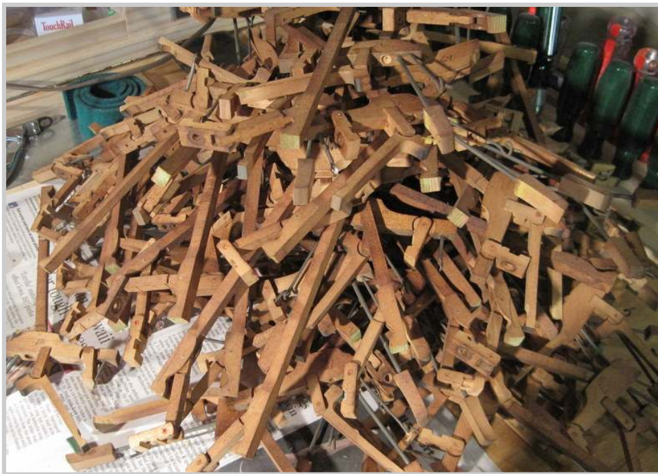
Photo 408: The whippens, now on the opposite side of the bench, are now stripped clean and ready for refelting.
