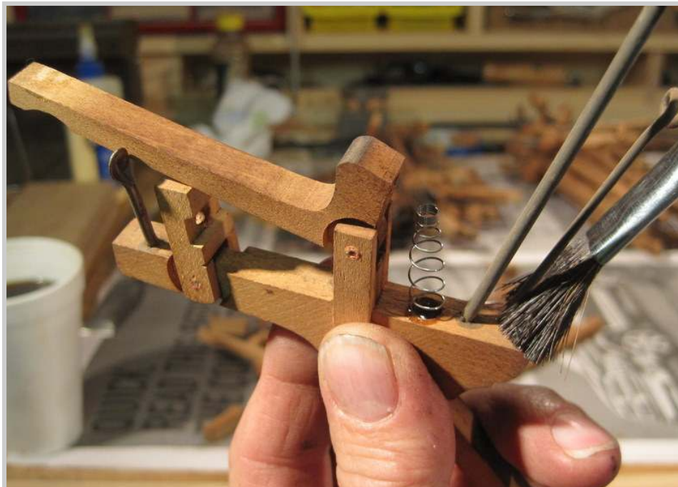
Photo 413: Remaining vestiges of stubborn dirt around the bridge wire and the backcheck wire is removed with a stiff bristle brush.
