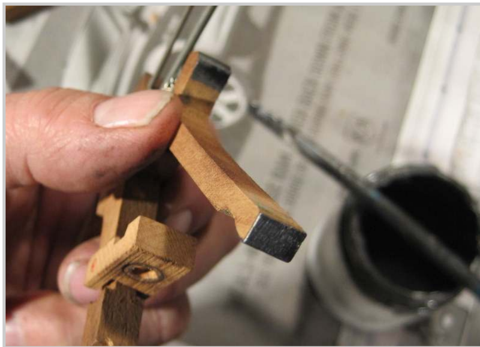
Photo 415: The heel of each jack is likewise lubricated with Dag, so that it slips freely from under the regulating button once contact is made.
