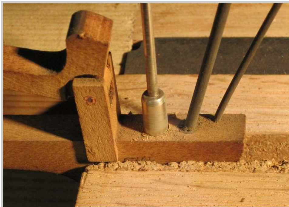
Photo 404: A jack spring hole reamer attached to an electric drill makes short work of cleaning out well.
