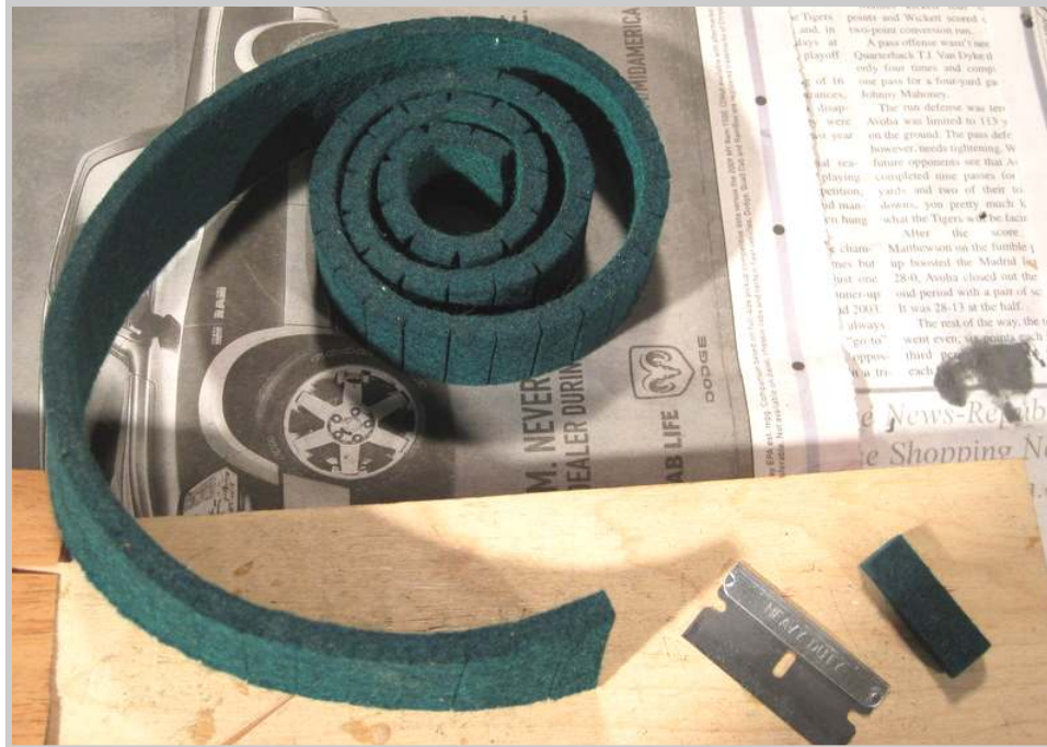
Photo 417: Backcheck cloth is cut from precut strips.
