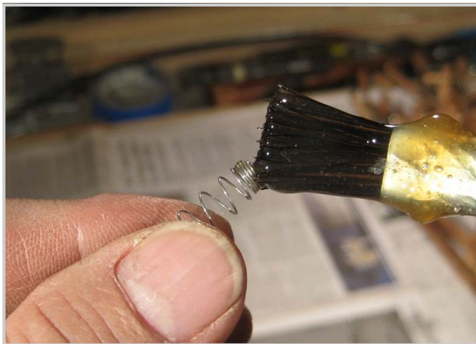
Photo 410: The bottom coil of the jack spring is swabbed with hot glue.
