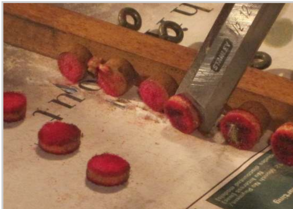
Photo 425: The next order of business is to slice the old felt punchings off of the regulating buttons of the let-off rail with a sharp chisel. A light sanding with 100 grit paper finishes this job.
