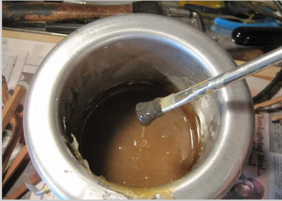
Photo 409: The hot glue, which has been on for some time, is checked for the correct degree of runniness. Constant monitoring is required to keep the glue at the optimum consistency. The addition of a little water, or a few glue crystals are needed from time to time.
