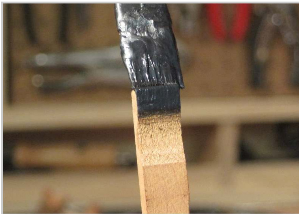
Photo 414: Dag® 154 Graphite lubricant is applied with an artist brush to the nose of each jack. This aids in the free functioning of the jack as it propels the hammer towards the strings. At the last moment before the hammer makes impact, the jack slips out from the hammer butt buckskin, so that the hammer strikes the strings under its own momentum.
