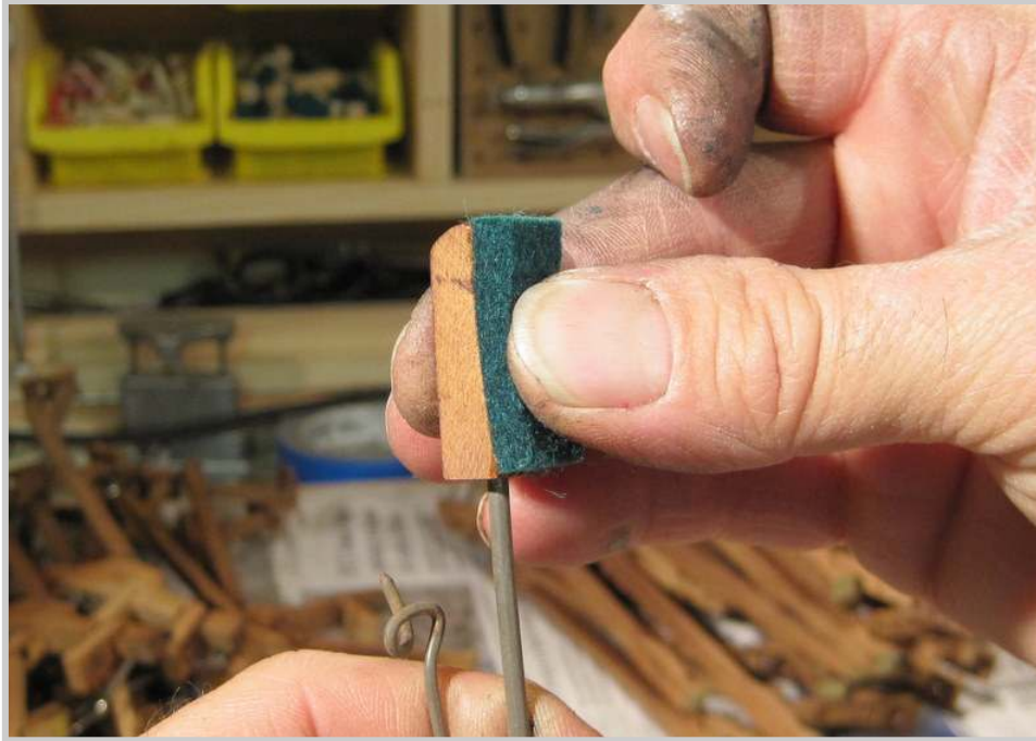
Photo 419: The backcheck cloth is positioned and held firmly in place for several seconds.
