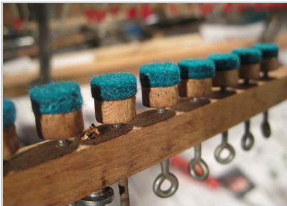
Photo 428: The newly refelted let-off rail.
