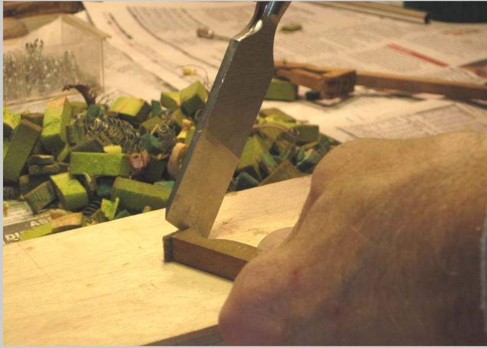
Photo 399: The sticker cloth is cut off of the bottom of the sticker using a sharp chisel in a swivel motion with the point firmly planted in the chopping block.
