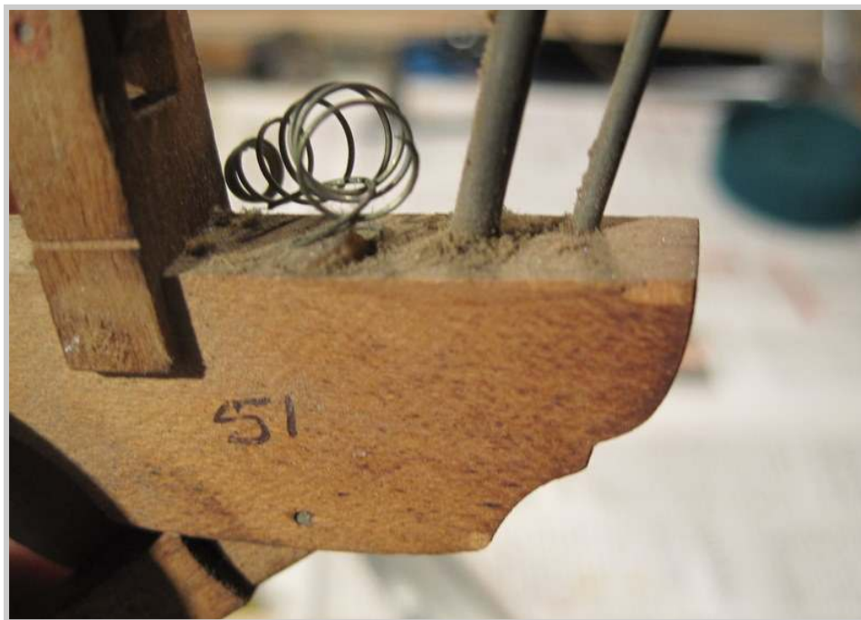
Photo 402: A broken jack spring signals the necessity to replace the entire set of springs. Once a particular part start breaking, total replacement of that part is the best course of action to avoid problems down the road.
