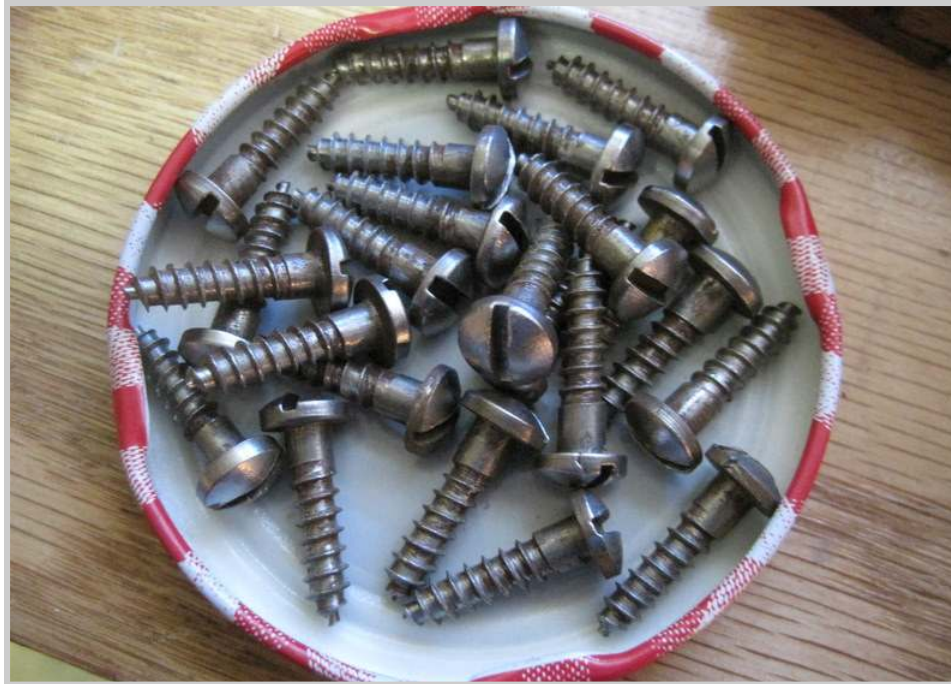
Photo 429: The flange screws used to attached the whippens to the action are now polished on the wire wheel. My daughter, volunteering to help, took each screw from its numbered hole in the screw holder, polished them, and tossed them in the lid of a jelly jar. Ah, well. Never criticize your children for being helpful.
