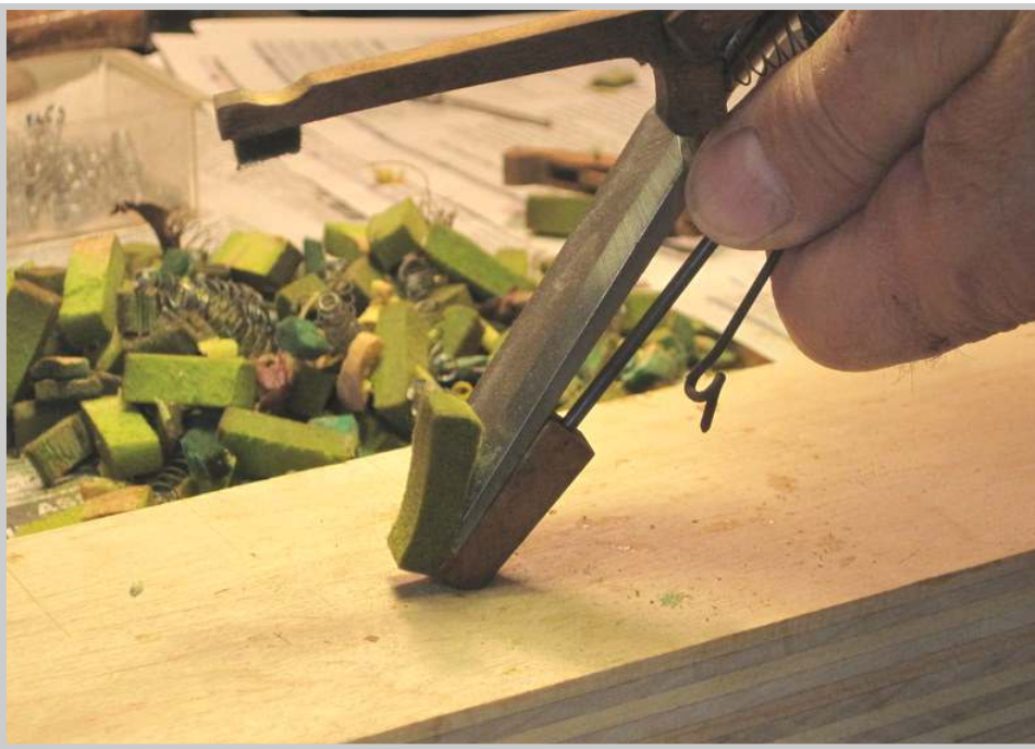
Photo 399: The sticker cloth is cut off of the bottom of the sticker using a sharp chisel in a swivel motion with the point firmly planted in the chopping block.
