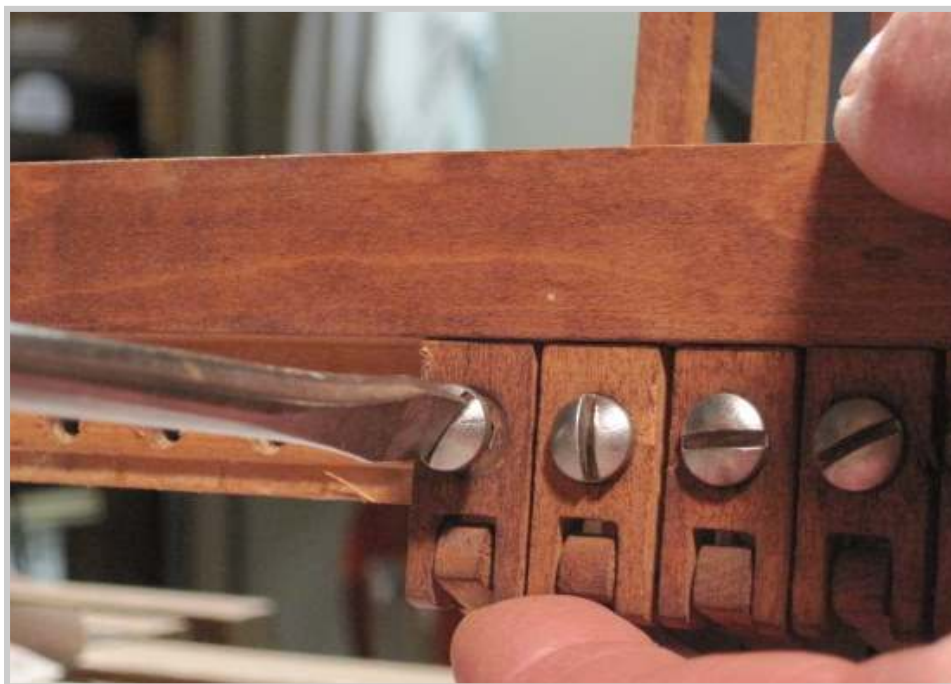
Photo 434: The sticker flange screw is inserted into the lower action rail.
