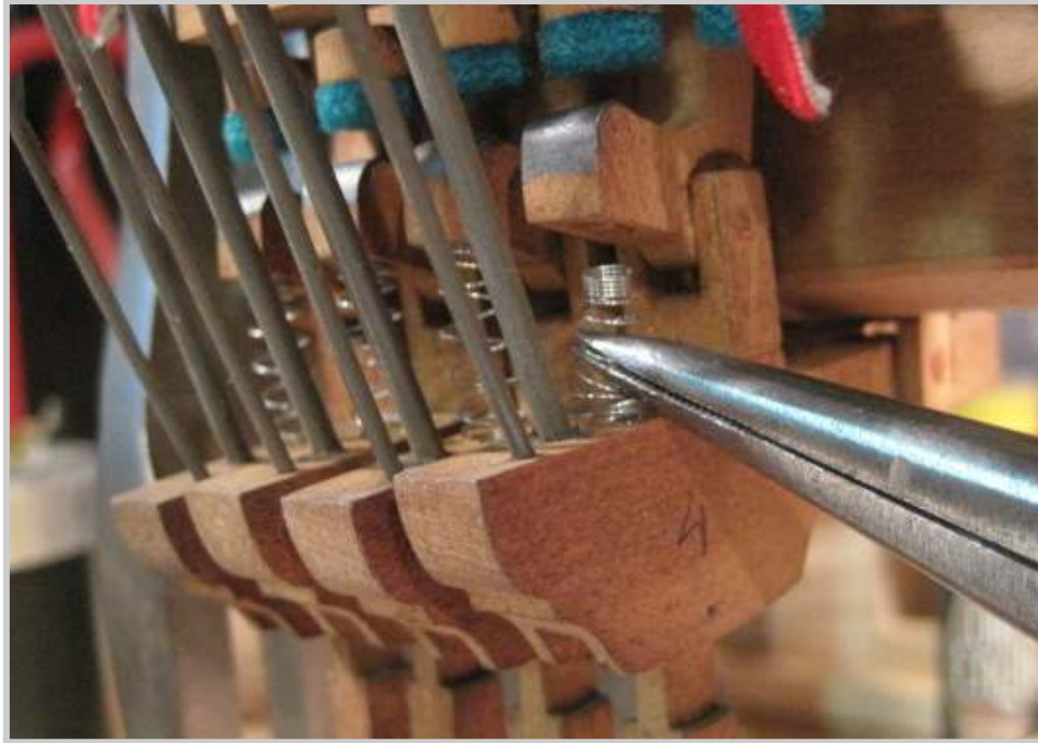
Photo 435: The jack spring is compressed slightly with a pair of needle nose pliers, so that its upper coil may be inserted into the well on the bottom of the heel of the jack.
