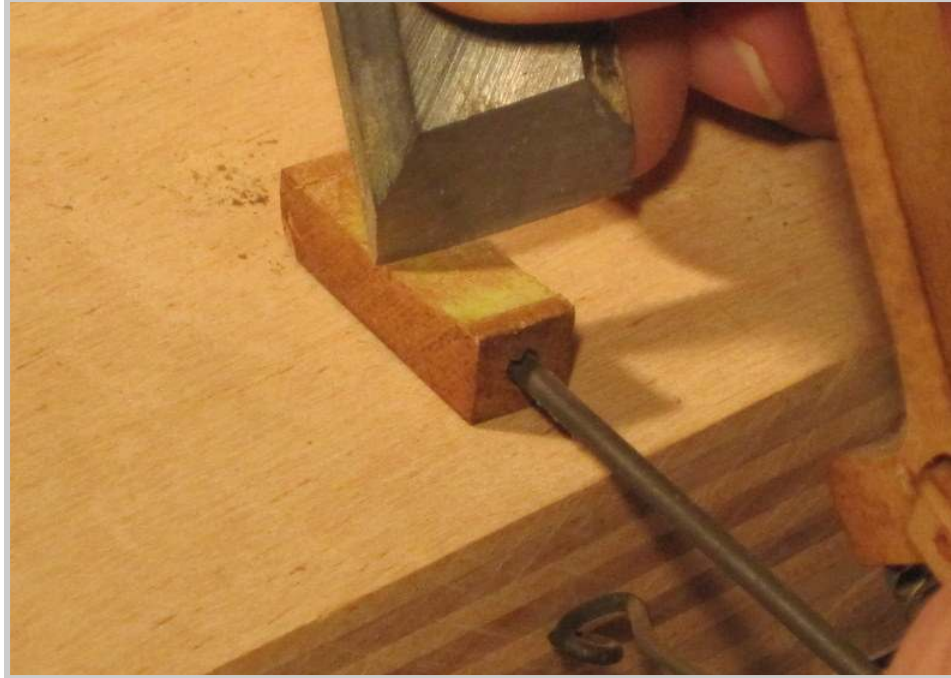
Photo 401: Glue and felt adhering to the wooden backcheck are scrapped off leaving a clean surface to glue new backcheck felt onto.
