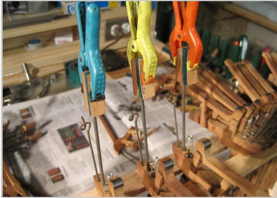
Photo 421: For one final time, the whippens are returned to the drying rack to allow the glue to cure.
