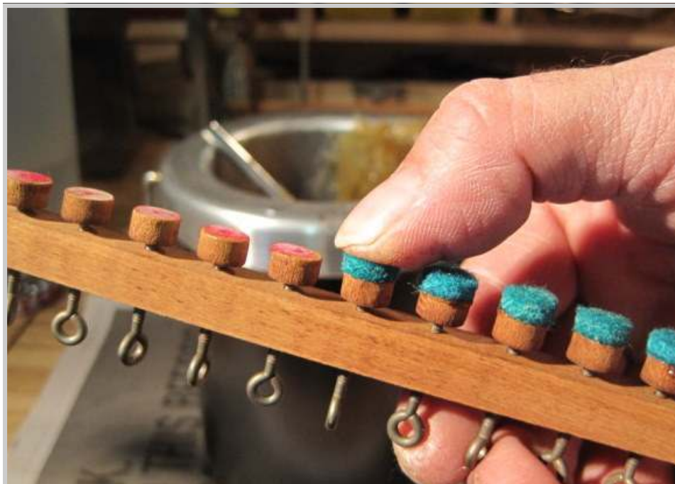
Photo 427: New punchings are glued into place with hot glue.
