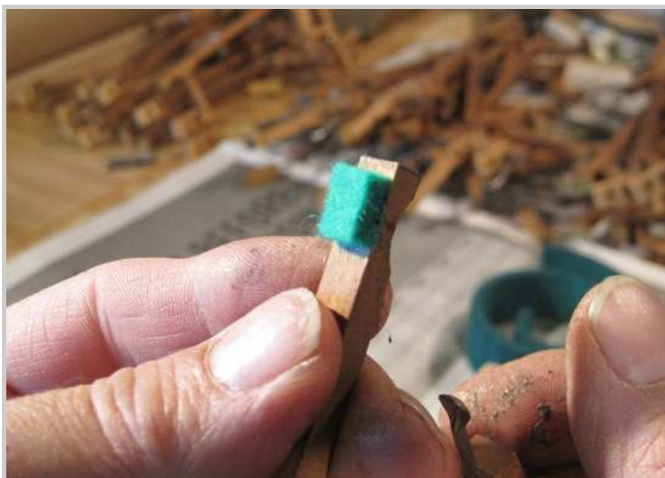
Photo 424: The final piece of felt to be replaced is the square of hammer butt felt which is glued to the topside of the jack.
