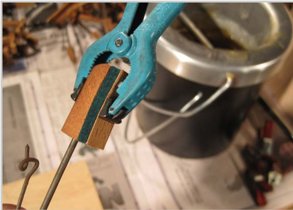
Photo 420: A miniature clamp is then applied with a small rectangle of veneer used to even out the pressure over the length of the cloth.
