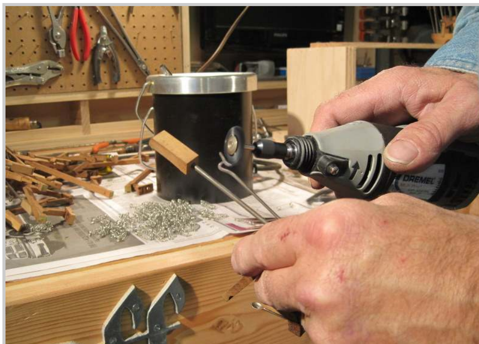
Photo 406: Before anything new is added, however, a burnishing of the bridle strap wires with a miniature wire brush in a Dremel tool is done as a final touch in the cleaning up process.
