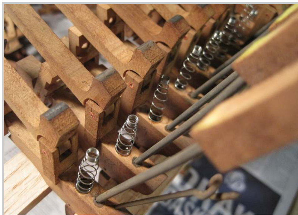
Photo 412: The whippens are then placed on a rack with the springs straight up and down while the glue cools and cures.
