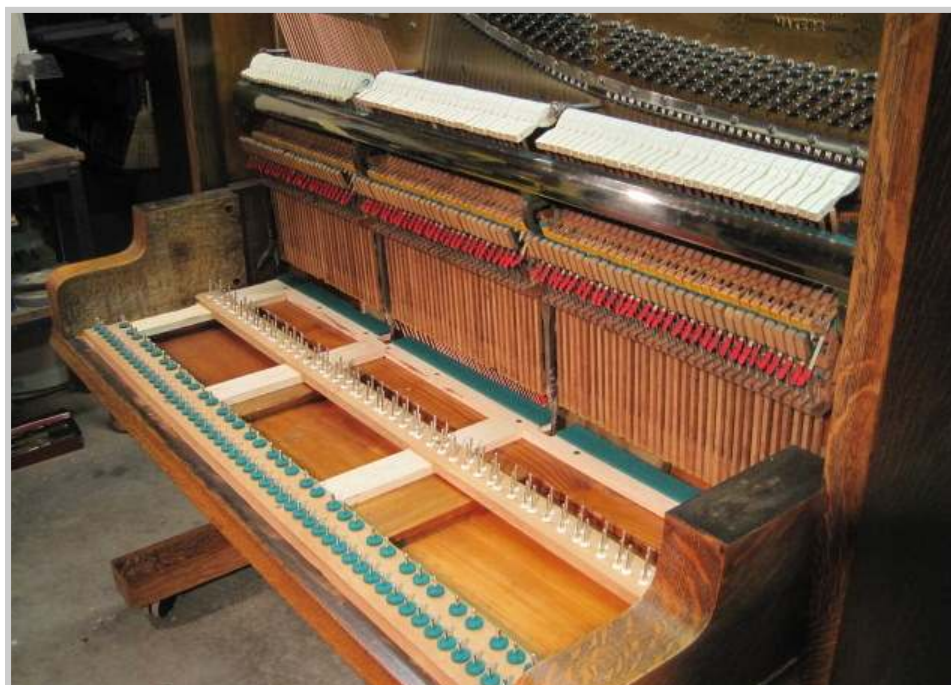
Photo 438: With the whippens all reinstalled, the action is returned to the piano for the time being.
