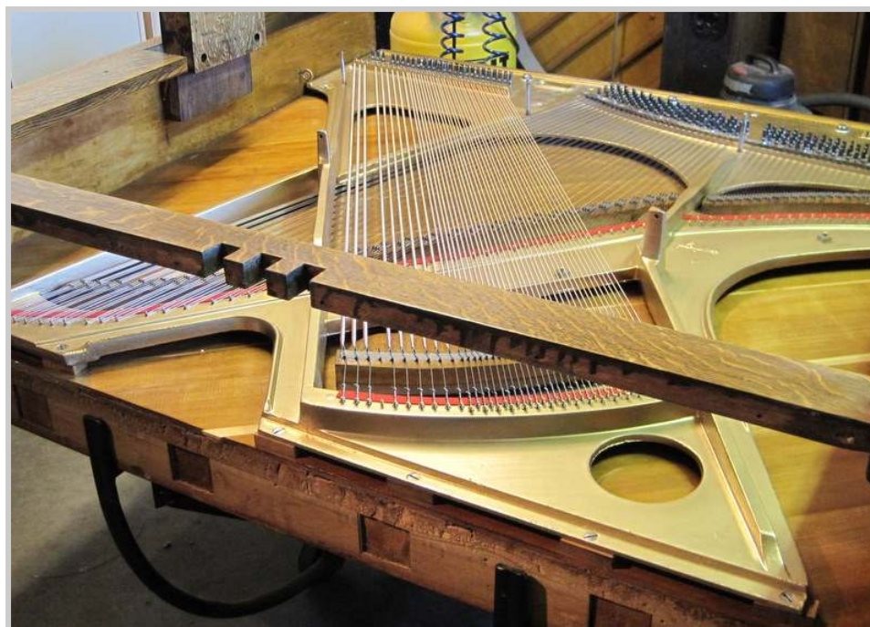
Photo 306: The toerail is returned into position.
