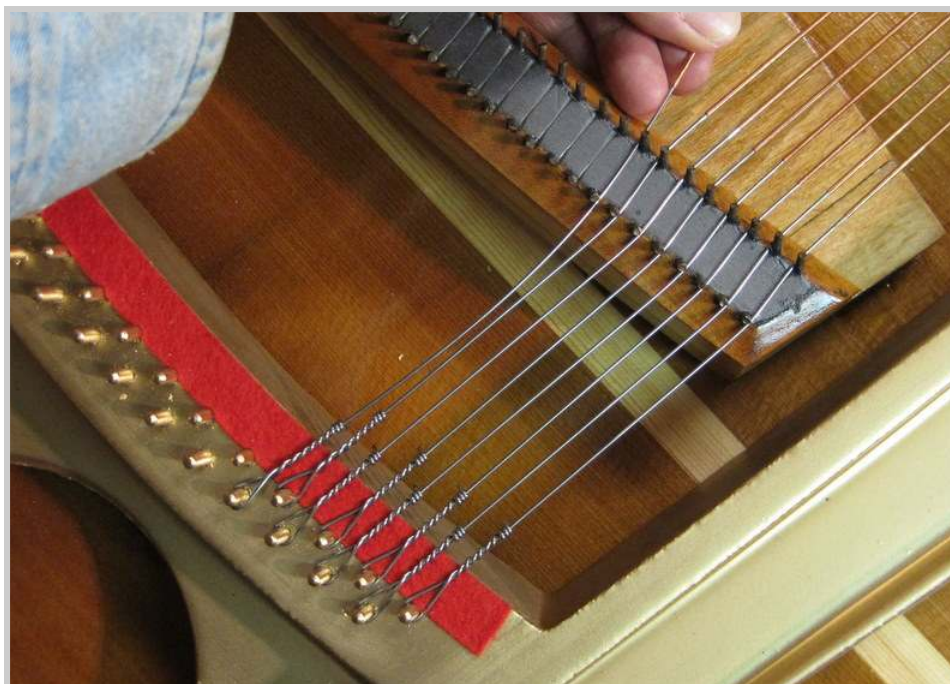
Photo 292: The installation of the bass strings is simpler than the treble strings in that each string is a single entity. The string is simply anchored to the hitchpin, instead of being looped around it as are the treble strings.
