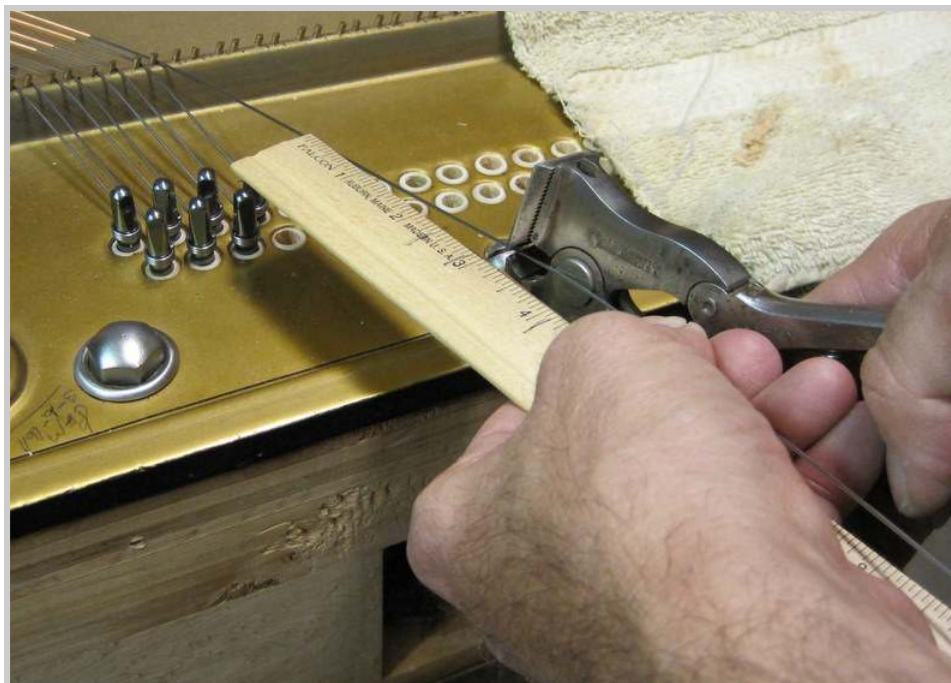
Photo 293: The string is stretched tightly across the upper bridge pin, measured at 3 1/4" from the center of the tuning pin hole, and cut.
