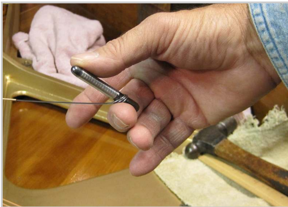
Photo 296: Unlike treble string, the copper wound bass strings are installed with a twist. Before the pin is inserted into the pin hole, the wire is turned one revolution in the direction of the winding.
