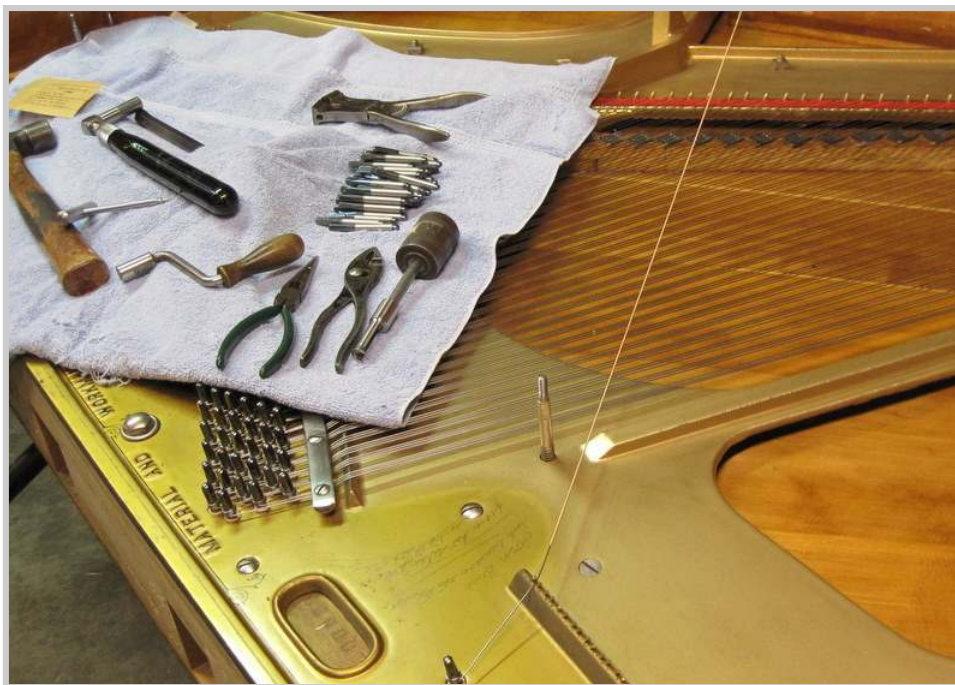
Photo 290: With tools laid out, the first string is put in.
