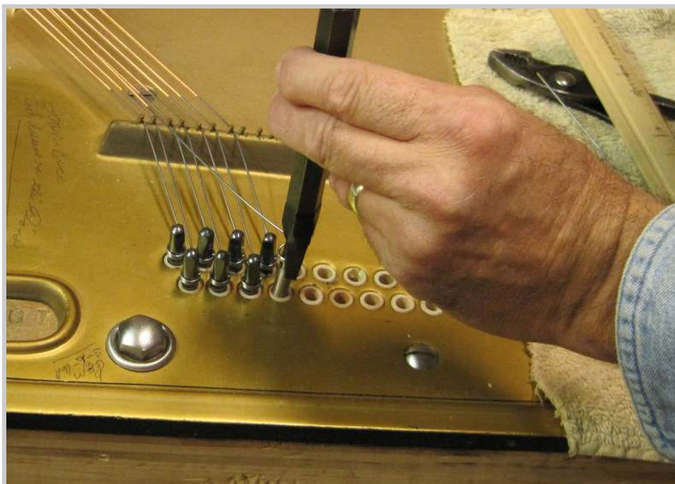
Photo 298: Using the pin punch with depth gauge, the pin is pounded in nearly all the way to the stopping point.
