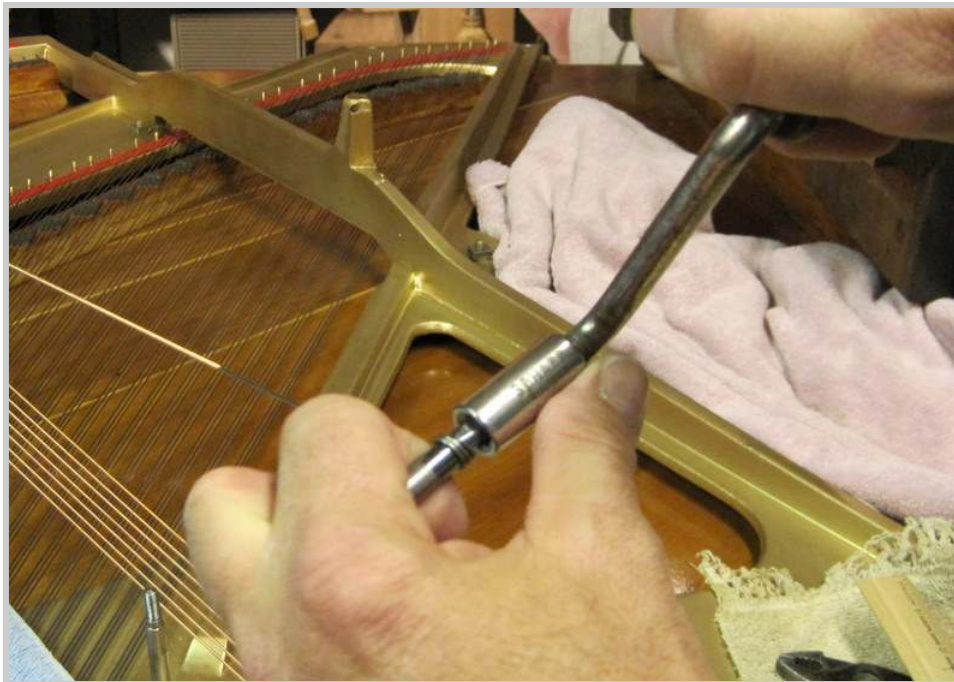
Photo 295: Using the tuning pin crank, a coil is made with three turns.
