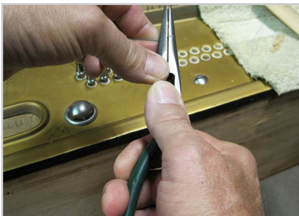
Photo 294: The end of the wire is bent with a 90 degree becket.
