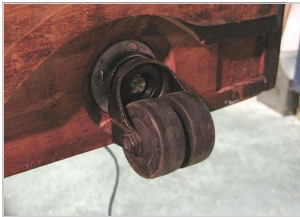
Photo 310: . . . followed by the casters. These double-wheeled Rubberex casters work soooo much better than the old steel wheels.
