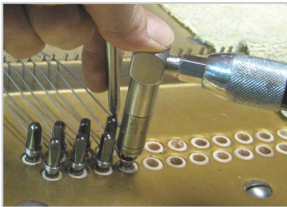
Photo 300: While turning the pin with the tuning hammer, the coil is tightened using the string hook.
