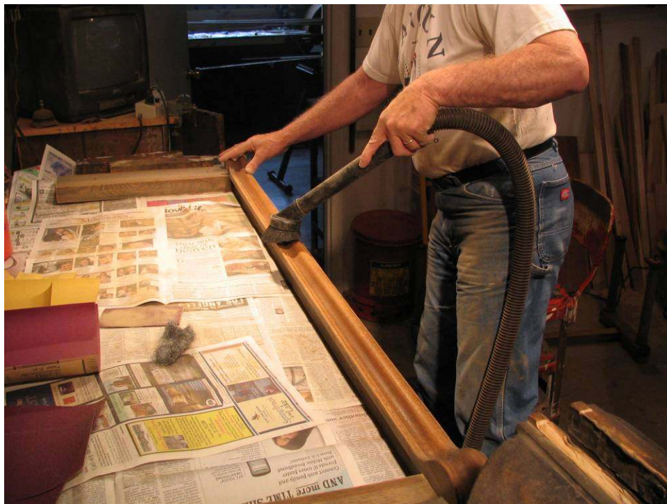
Photo 82: Following sanding, each part is vacuumed. This will be repeated before staining, and before each coat of finish is applied. The idea is to prevent the accumulation of dust in the shop as each step is completed.
