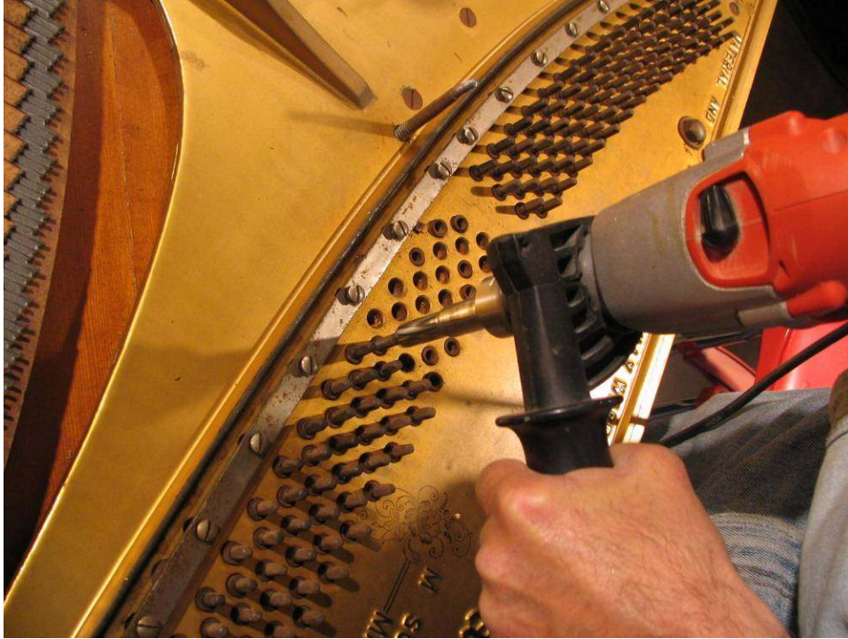
Photo 77: With Dave done stripping the body and removing the layer of newspapers, I begin removing pins with a drill equipped with a power tuning pin socket. With the old pinblock material to be replaced, heating the pins with rapid removal is not a problem.
