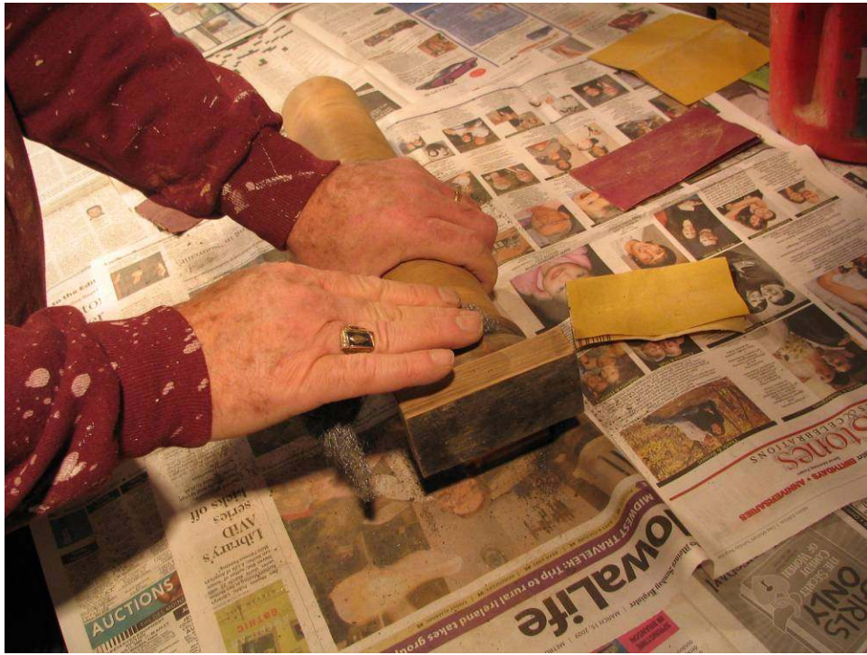
Photo 81: With the stripping of the case completed, Dave begins steel wooling and sanding the case parts. The #3 steel wool is used first to remove any stripper residue. He then progress from 100 grit, to 150 grit and finally 220 grit sandpaper for each piece.
