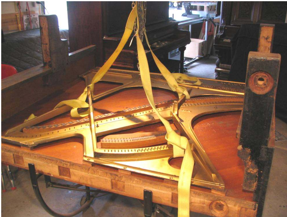
Photo 87: Straps are attached to the plate at 3 points. Each strap is connected to a hook on a 1000 lb. capacity chain hoist. Straps are double knotted to prevent slipping.
