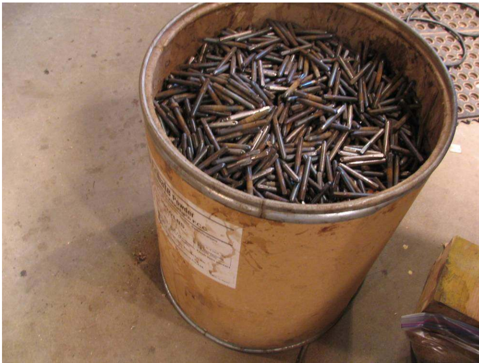
Photo 78: Used tuning pins are thrown into the recycling barrel.
