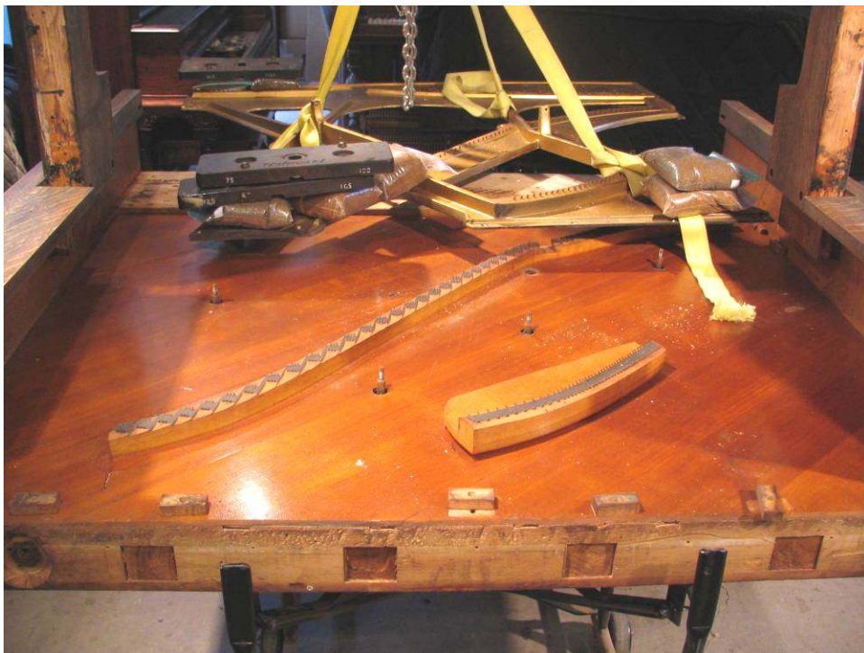
Photo 88: The plate is lifted several inches and the piano is rolled out from under it. The bags of sand and weights are used to balance the plate so that it lifts evenly.
