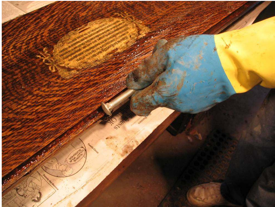
Photo 82: Here Dave uses the rounded head of a bolt to strip the edge of the lid. The decal has stripper applied to it, and will scrub off with steel wool.
