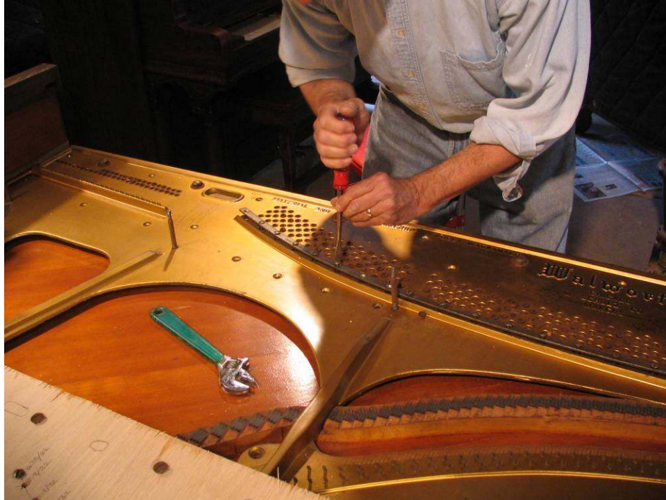
Photo 84: The plate screws are removed, followed by the pressure bar screws. Each of these screws has been measured for its height above the plate, using a combination square marked in 32nds of an inch. The heights are recorded on the wooden holder where they won't be lost.
