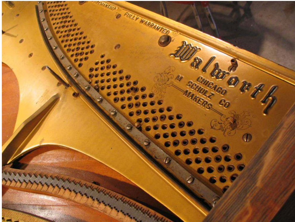
Photo 79: Plate with pins removed. What bushings are left will fall out or be punched out after the plate is removed from the piano.
