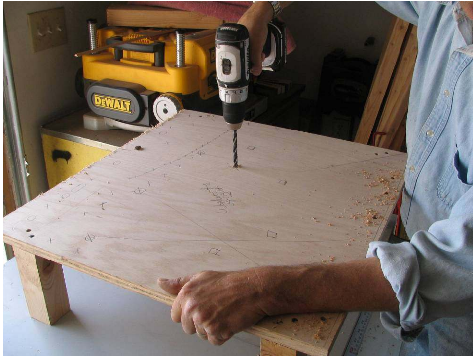
Photo 83: With the screw pattern drawn out, I drill holes for the various sizes of screws which will be removed. The legs of the holder are long enough that the longest screws are given adequate room.
