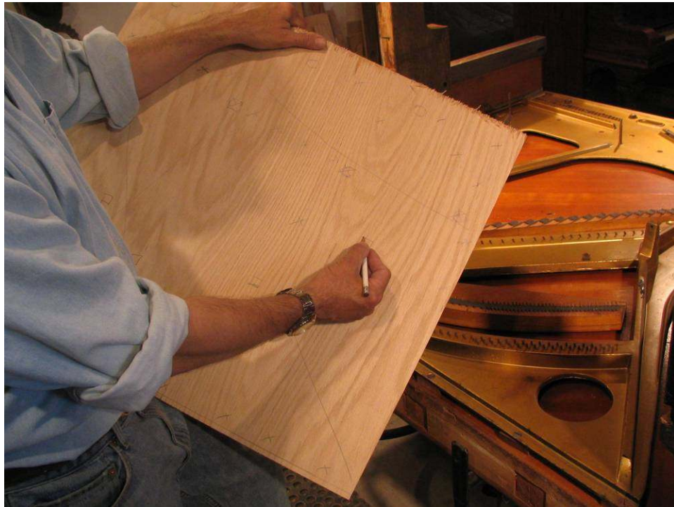
Photo 80: With the pins out, the various plate screws must be removed and stored before the plate may be pulled from the piano. A wooden holder for the screws is marked with their locations.
