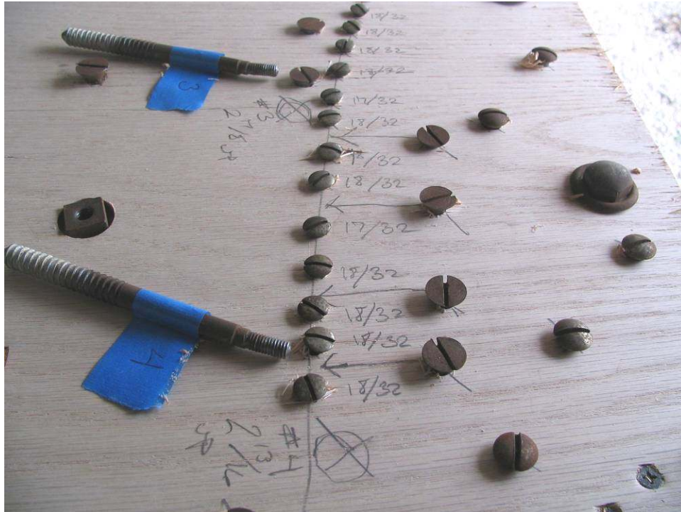
Photo 85: All the screws are now safely stored with pertinent information until the piano goes back together again.
