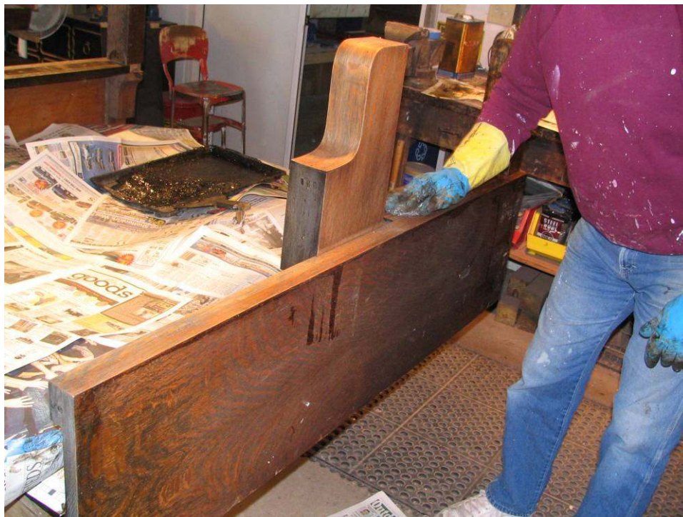
Photo 70: With his checklist ready to go (sometime in the future) Dave begins stripping the body. The cast iron plate is kept safe from stripper with layer upon layer of old newspaper.
