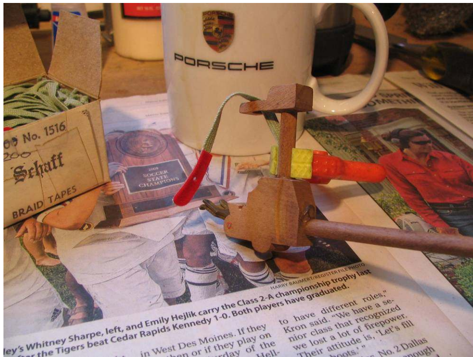
Photo 72: Clamp in place, the glue is allowed to set. Another technique is to double up the end of the strap, and to use a tiny brad to affix it to the catcher shank. A true purist would, I suppose, insist on removing the catcher shanks to insert the end of the strap in the hole.
