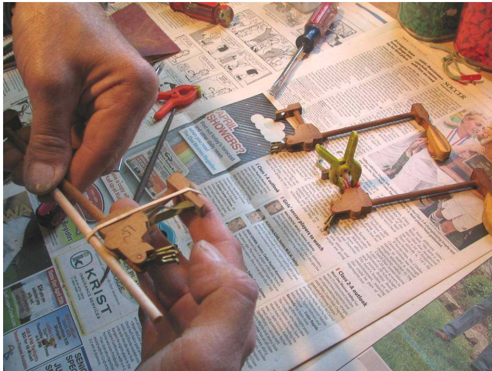
Photo 75: Using a hammershank flattened on one end, the spring felt is clamped into place. To work, the rubber band stretches from the catcher to above the position of the felt.
