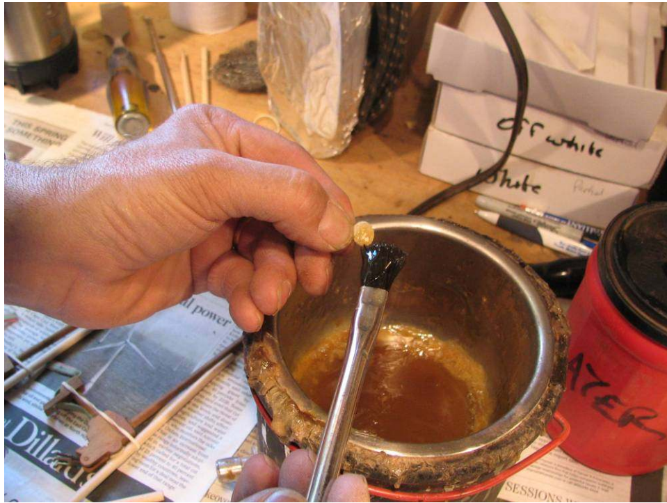
Photo 73: Hot glue is applied to a spring felt.
