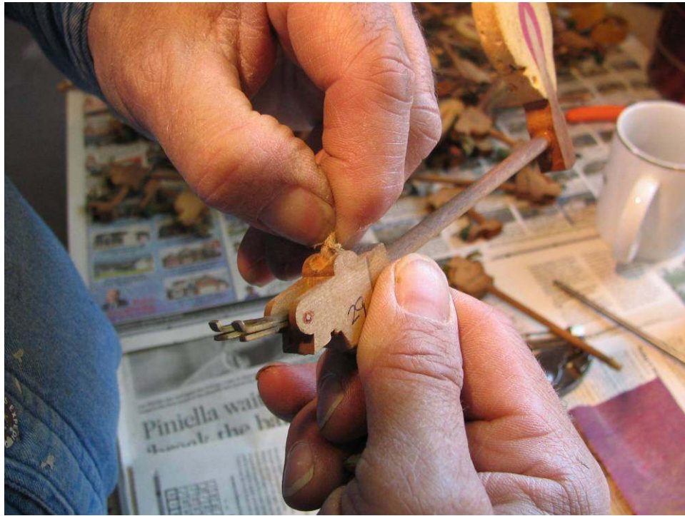
Photo 65: The spring felt is easily removed by hand.
