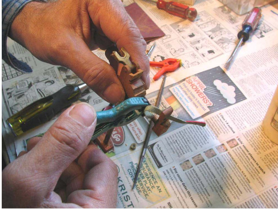
Photo 71: At my bench, I apply a drop of Titebond to the end of the braided bridle strap. The strap is then clamped in place on the underside of the catcher shank. For some reason, I find that hot animal hide glue does not work particularly well on the braided strap.
