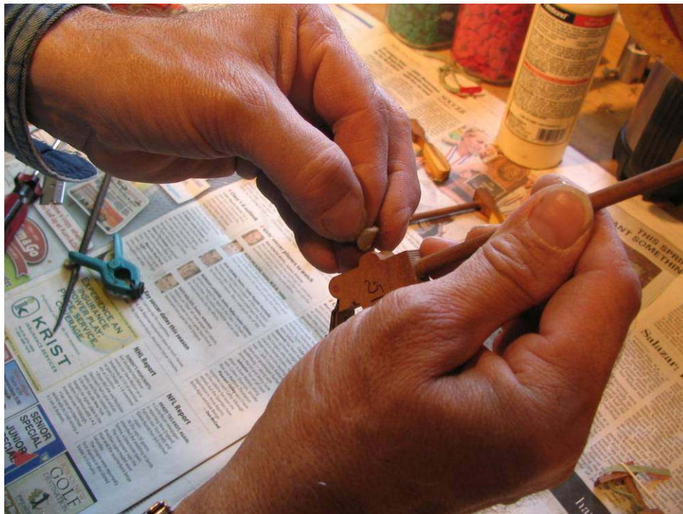
Photo 74: Using a thumb and two fingers, the felt is creased slightly and placed in the groove.
