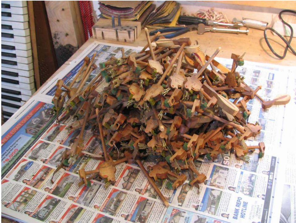
Photo 61: Project for the day. All the buckskin and felt, except the center pin bushings, will be stripped from the old hammer butts in preparation for new. This stack of parts, by the way, represents a victory over my obsessive /compulsive nature. Five years ago, these parts would have all been neatly stacked in ranks and columns. Looking at the stack as I write this, I notice it is very symmetrical and neat. Hmmm.
