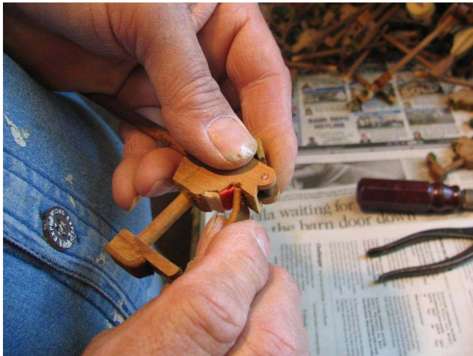
Photo 64: Removing the hammer butt buckskin by pulling it free from the slot that it is inserted in. This piece is glued on either end and pulled tight over the underlying felt. The white felt is glued in place, and is removed by using a small, flat-bladed screwdriver to scrape it out of its recess. The red felt is glued on the slot end only, and is removed with a sharp chisel.
