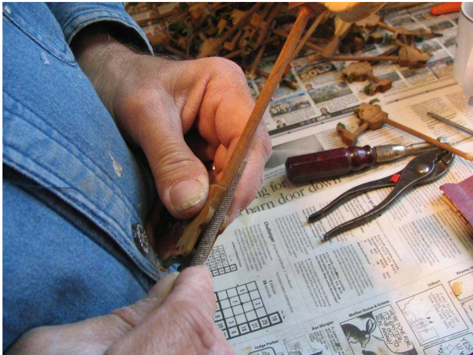
Photo 66: Residue of the felt and glue is removed with a rat tail file. In all, seven individual pieces of buckskin and felt are removed from each hammer butt. The process takes a couple of minutes per butt.
