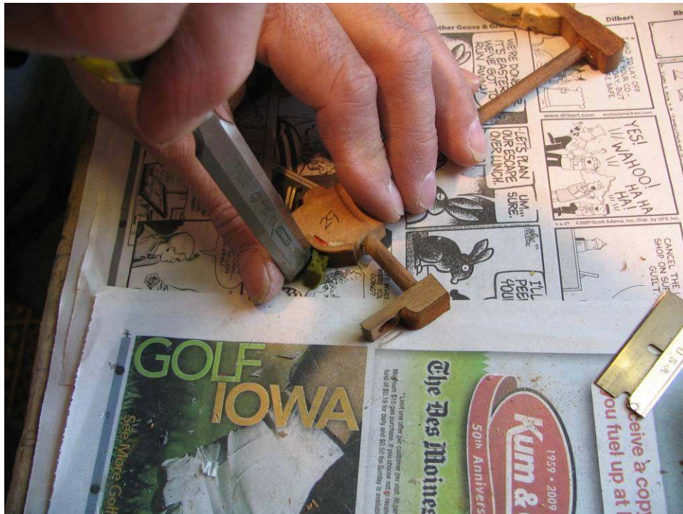
Photo 63: Piece by piece, the felt and buckskin are removed with a chisel or razor blade. The necessity of this procedure becomes more and more evident as I proceed. The hammer butt felts and the felt squares on the inside of the catcher are the worst, but also the red and white felts under the hammer butt buckskin are in very bad condition, so much so that on some hammer butts, daylight can be seen under the buckskin. The result would be that support for the jack would be spongy at best.
