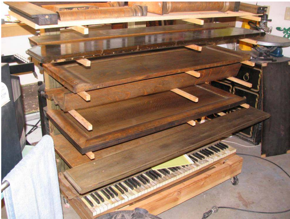
Photo 68: To his credit, Dave does have most everything stripped and ready for sanding and veneer work (but not staining). The one part near the top of the parts trolley which is not stripped is the underside of the front part of the lid, which has a decal. Whether we strip that or not is up to the owner, who is scheduled for a visit later in the day. Dave's choice is to strip, mine is to save. It will be the owner's call, however.
