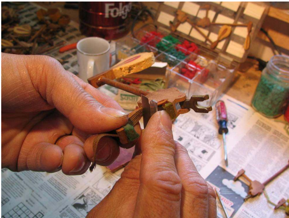
Photo 62: Taking a hammer assembly from the pile, I begin the process of removing the old felt. Instead of just snipping the original bridle strap, I will be cutting the old strap flush to the hammer butt. The new braided strap will be cut to the correct length and glued to the underside of the catcher shank.
