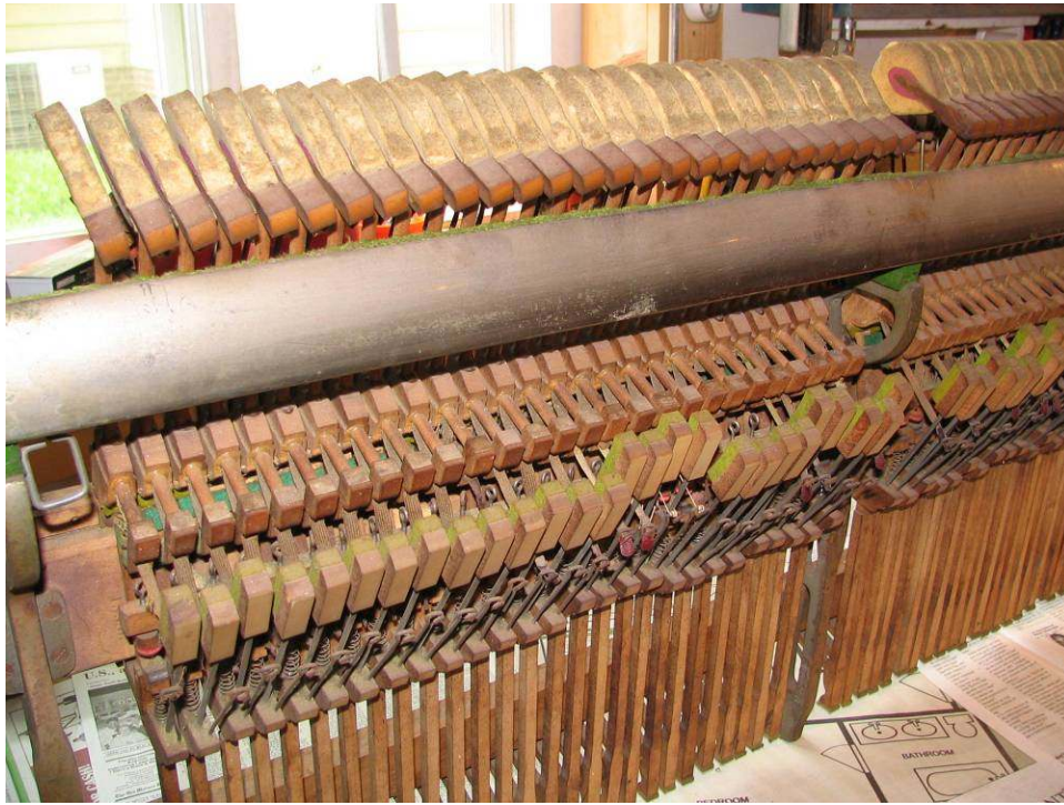
Photo 41: With the strings ready to take to the post office, the action is put on the bench for its initial inspection. Deciding what to replace, and what to simply clean is always an issue. On this action, for example, the back check felts show little wear, and will just need to be cleaned.
