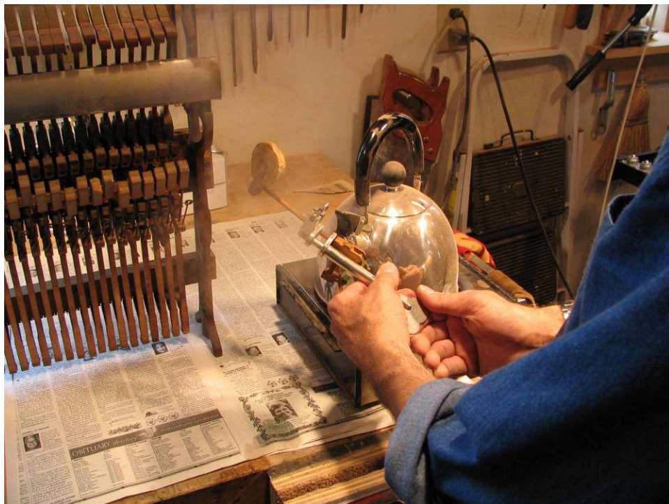
Photo 44: For each of these end hammers, the shank is removed from the hammer butt by softening the glue joint with steam and using a special hammershank extractor and clamp.
