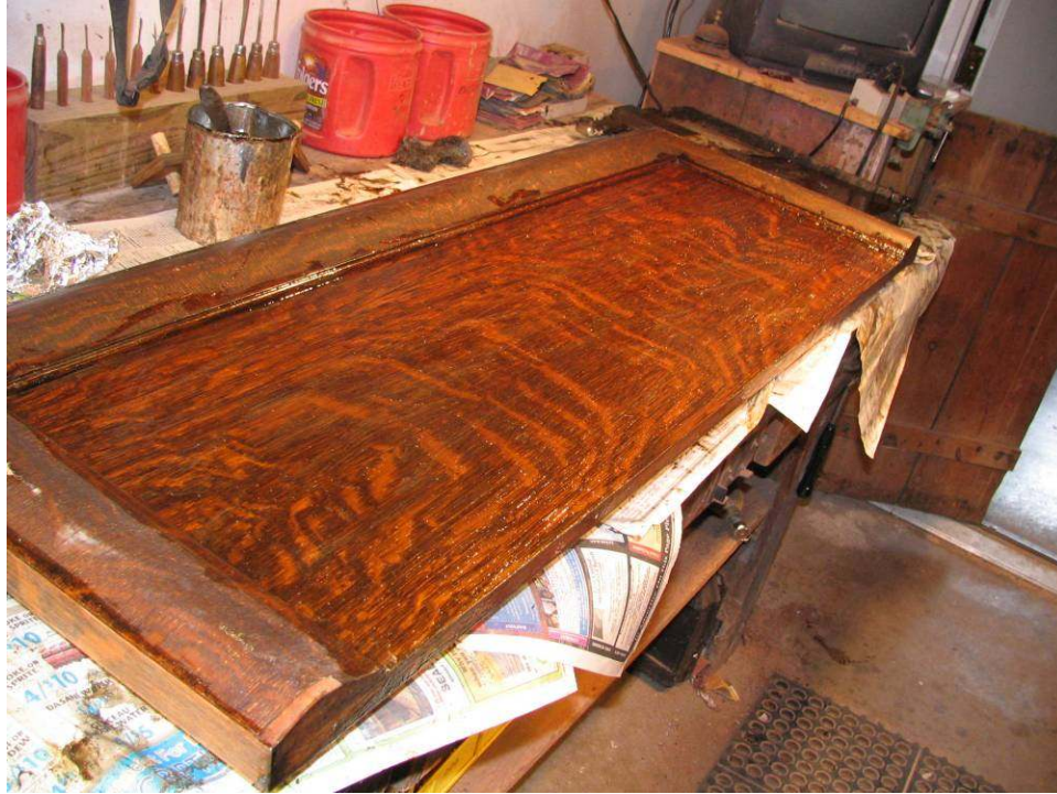
Photo 47: While I work on boxing and addressing the string and hammer samples, Dave continues his work stripping parts. Here, the stripper does it work on the front board of the piano.
