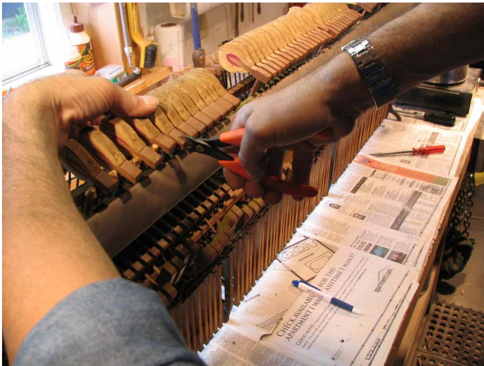
Photo 49: On the action bench, I finish the morning by removing the odd numbered hammers from the action. When the new hammers come back from the factory, I'll put on the even hammers first, using the remaining odd hammers as a guide. Snipping the old ones off as shown is the most efficient method.
