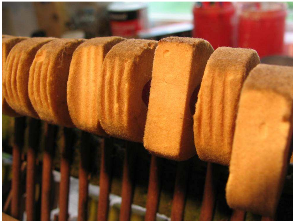
Photo 42: With the hammers, it's another story. Some "technician" in the past apparently thought that removing the string marks was best solved by simply sawing off the fronts of certain hammers. Imagine the tone produced! Gives a new meaning to the term "blocking hammer."
