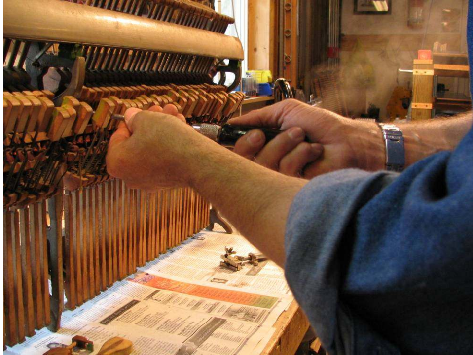
Photo 43: To have the hammers duplicated, the end hammers from each of the three sections of the action are removed to be sent in as samples. Here the hammer butt assembly, with attached hammer shank and hammer from the end of the treble section is being removed from the action.
