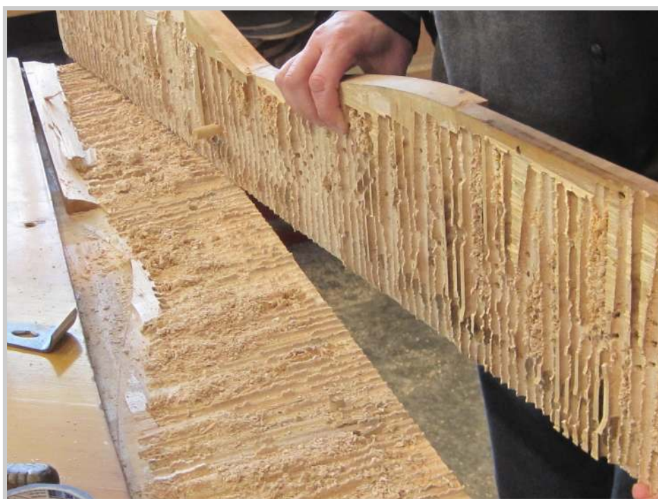
Photo 134: Using this method, probably 95% of the old pinblock is now removed from the back assembly. To finish the job, the remaining layer of old pinblock will be removed. (The split-off chunk of wood seen near the top is from a separate runner of wood that was butted up to the pinblock.)
