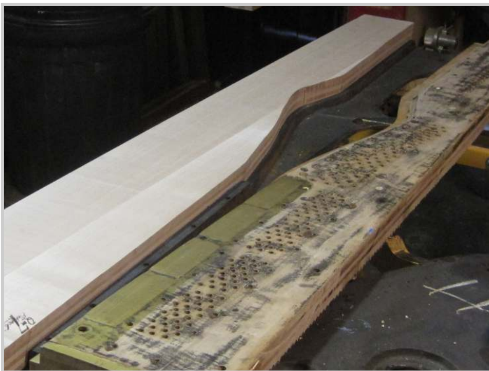
Photo 138: In another room of the shop, the cast iron plate is on sawhorses, ready to fit the new pinblocks. This will have to wait until next time as well - time is always shorter than you would like. The advantage of this method of pinblock removal is that the surface of the old pinblock is untouched, leaving it available to refer to.
