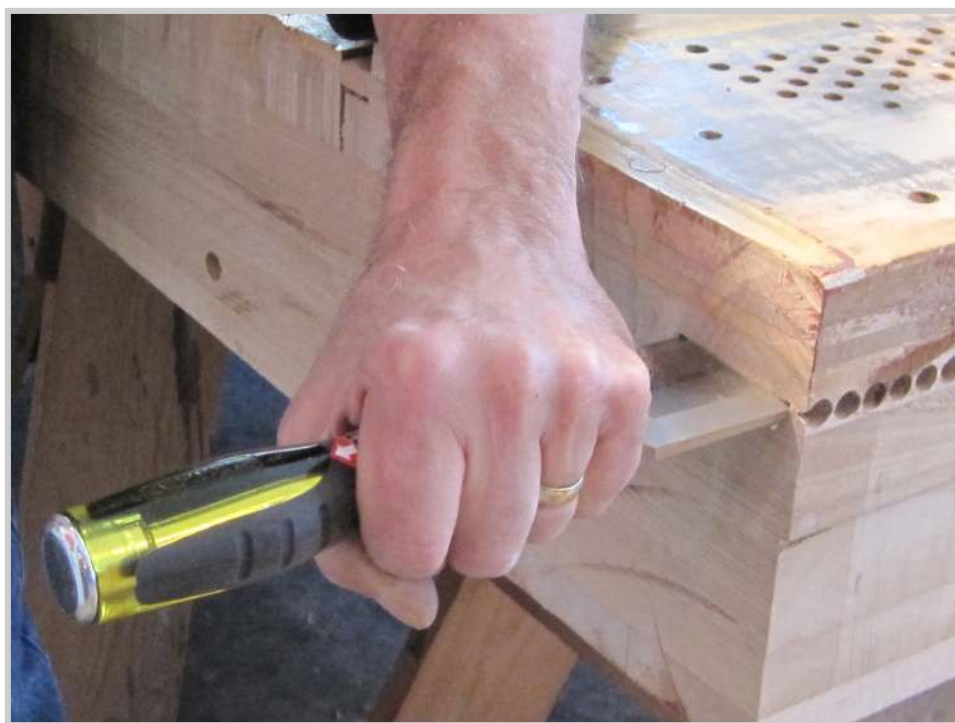
Photo 128: Using a chisel and a ball peen hammer, I take the first step in breaking apart the pinblock from its wooden backing.
