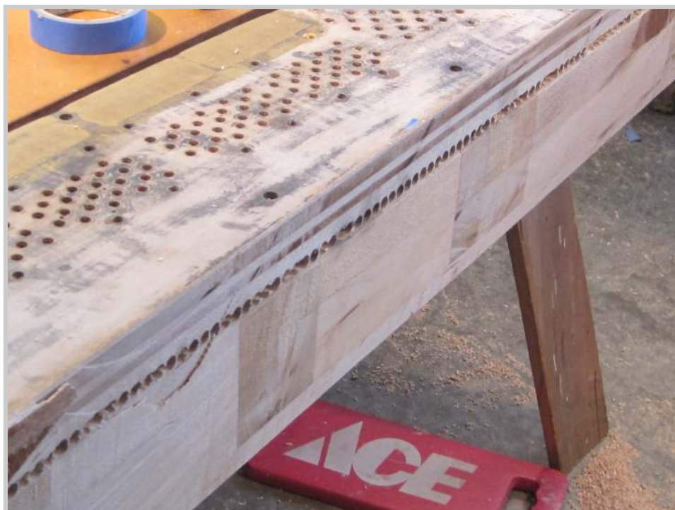
Photo 127: After lunch we get back at it, and before long the entire length of the pinblock is undercut with holes..
