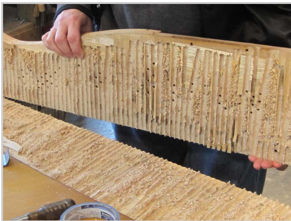
Photo 133: Voila! The pinblock comes off in one complete piece!
