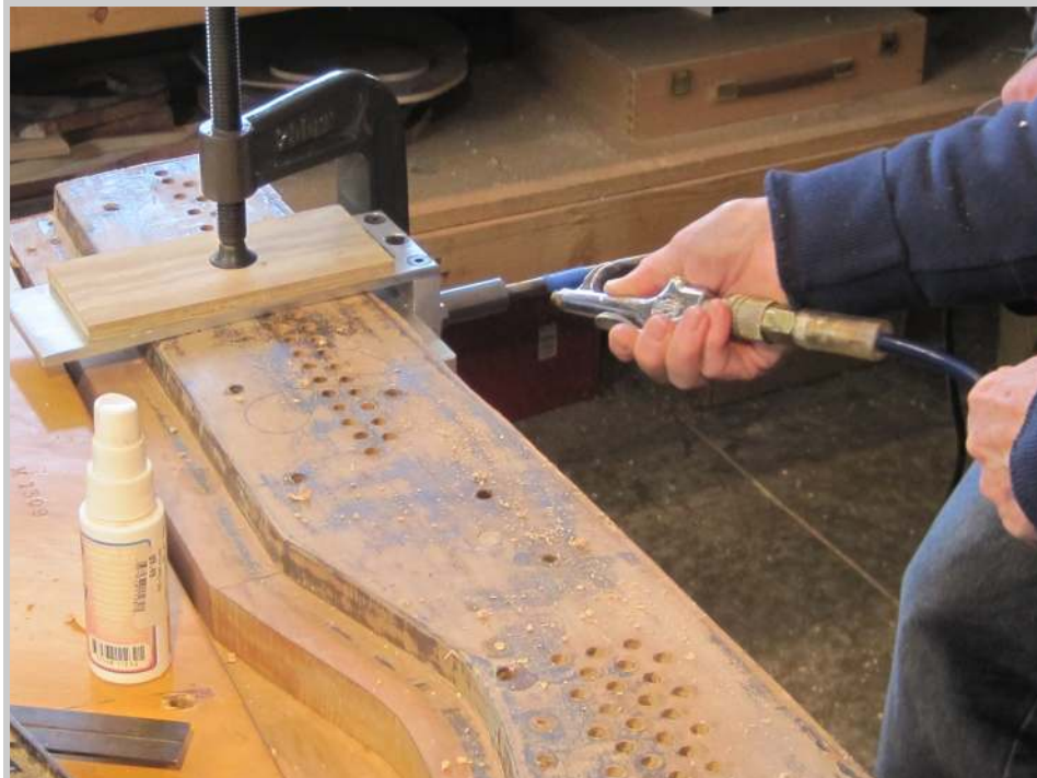
Photo 126: The jig from Bolduc is just a great tool for this job. After each hole is drilled, the clamp is loosened, the jig is moved over one place with the guide pin being inserted into the new hole, and drilling commences once again. Keeping the bit cool and sharp proved to be very important.
