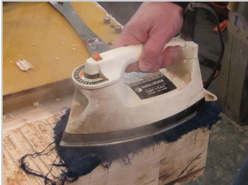
Photo 136: A damp rag and steam iron are brought into action to help soften the glue joint.
