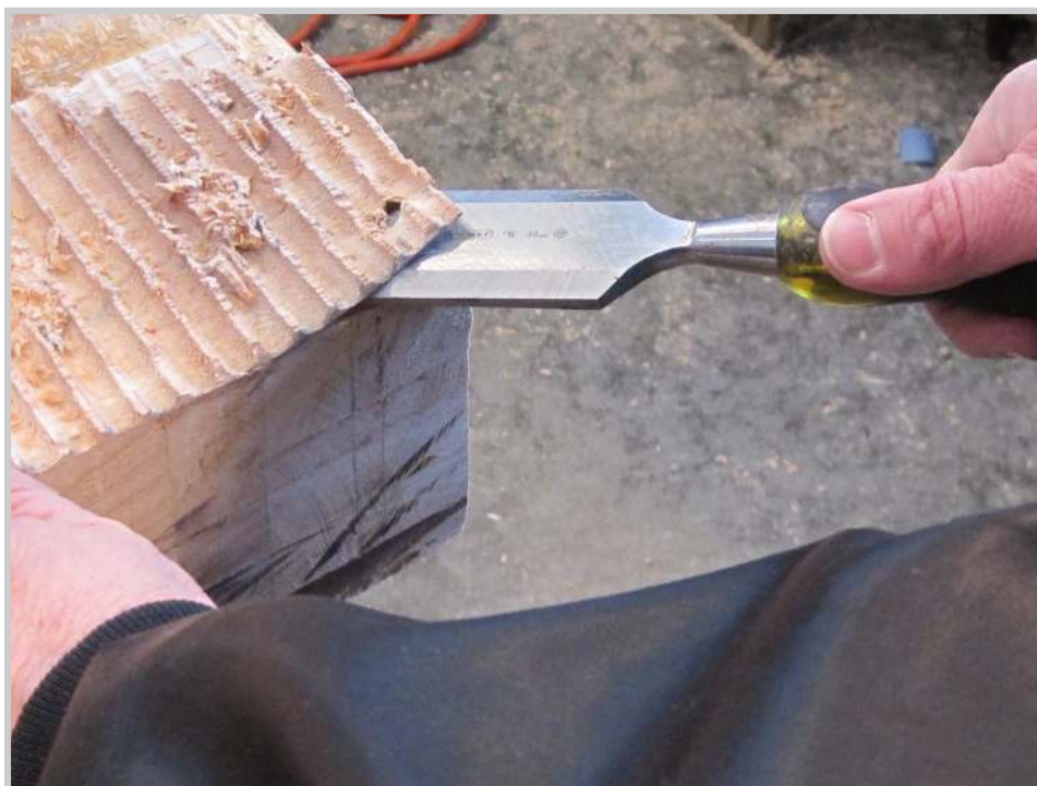
Photo 135: Steve tries removing the remnants of pinblock material with the chisel. The corner is loose, but further in the glue still holds tight.
