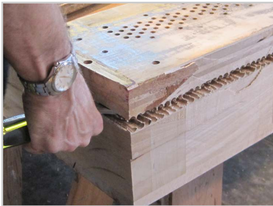
Photo 130: With the blade of the chisel driven in as far as it will go, I lift up, and a cracking sound fills the room.
