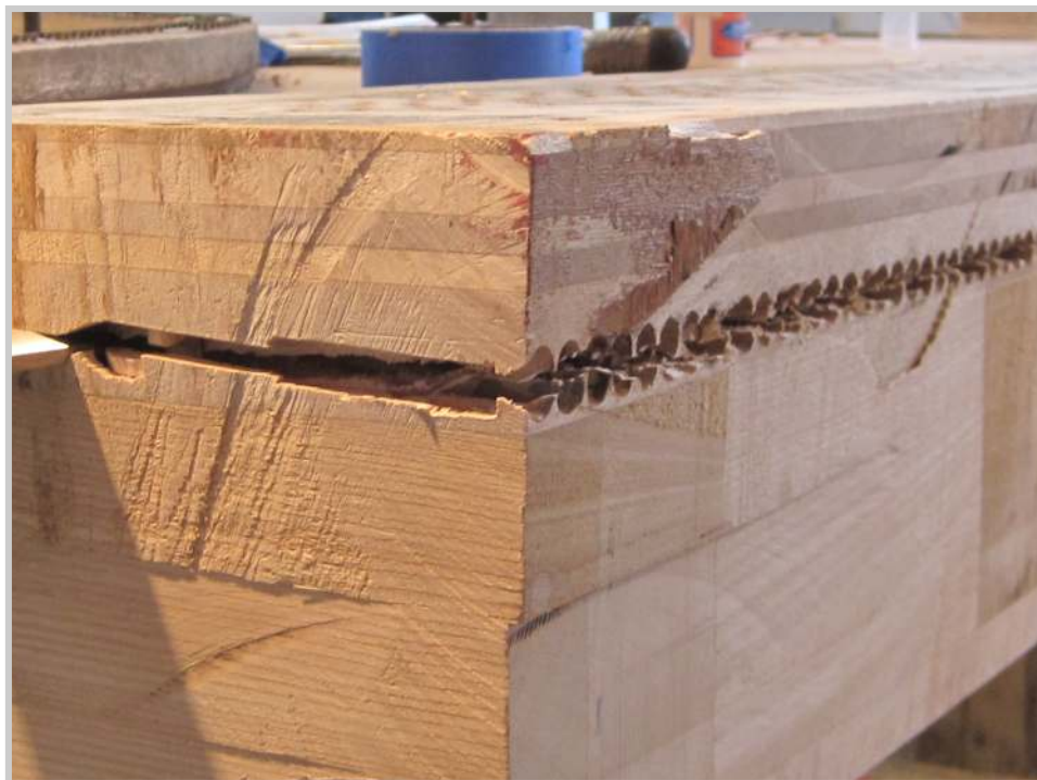
Photo 129: With a little effort on my part, the separation of the pinblock from the wooden framework of the piano begins. The line of holes are not quite touching, but are separated by a thin wall of wood. Just under the holes, the seam between the pinblock and the framework can be seen in the above photo.
