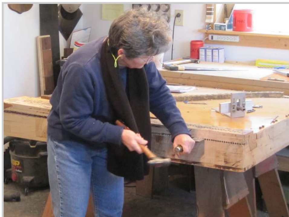
Photo 131: Bev uses the chisel and hammer to extend the split near the treble end of the pinblock.
