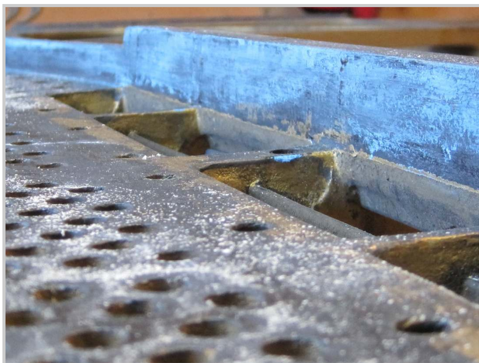
Photo 124: The flange of the cast iron plate that the pinblock will be fitted up against.
