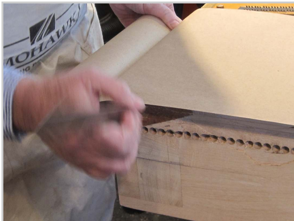
Photo 112: To round the day out, the decision is made to spend the remaining time in cutting the new pinblocks. The first step is to unroll contractor paper over the old pinblock to mark the lower edge of the pinblock. On this piano, unlike on most uprights, the pinblock is fitted to a flange on the underside of the cast iron plate.
