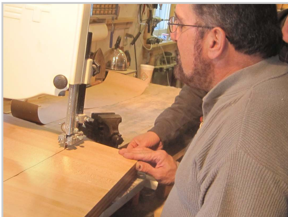
Photo 119: The WNG block is fed into the saw, with a person on either end and one in the center. The new blade cuts easily through the 2" maple, with no strain on the band saw.
