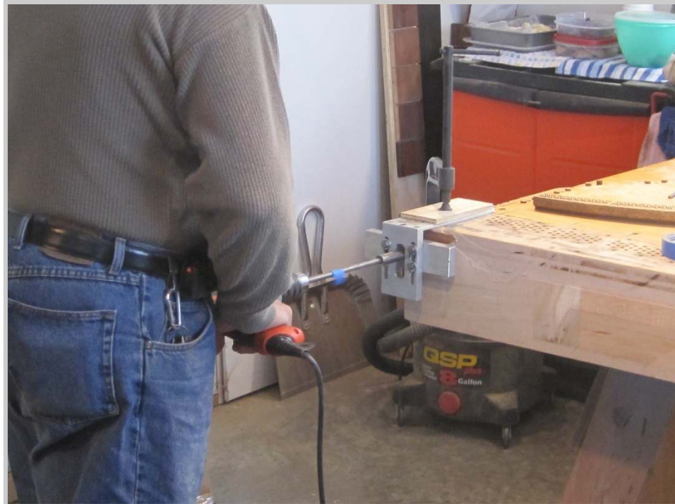
Photo 101: Chapter member Angelo Georgou tries drilling one of the first holes. Despite a new bit, drilling through the century old hard rock maple is tough going. You must firmly lean into the drill to advance the bit.
