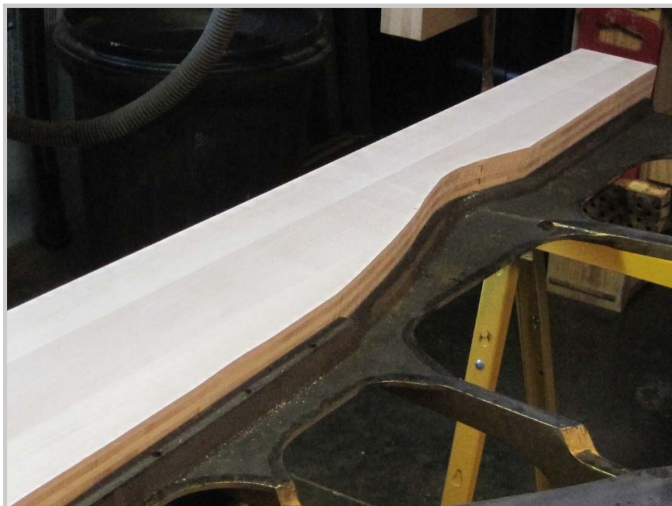
Photo 122: The fit of the Bolduc pinblock to the cast iron plate is checked out. A bit of grinding will need to be done on all three of the pinblocks to complete the fitting process.
