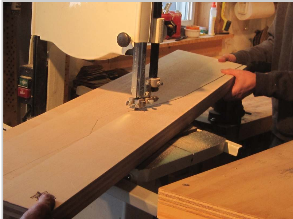
Photo 120: The Central Michigan block being cut, with the person to the left guiding the pinblock through the curves, and the person on the right stabilizing the pinblock as it comes off the table of the saw.
