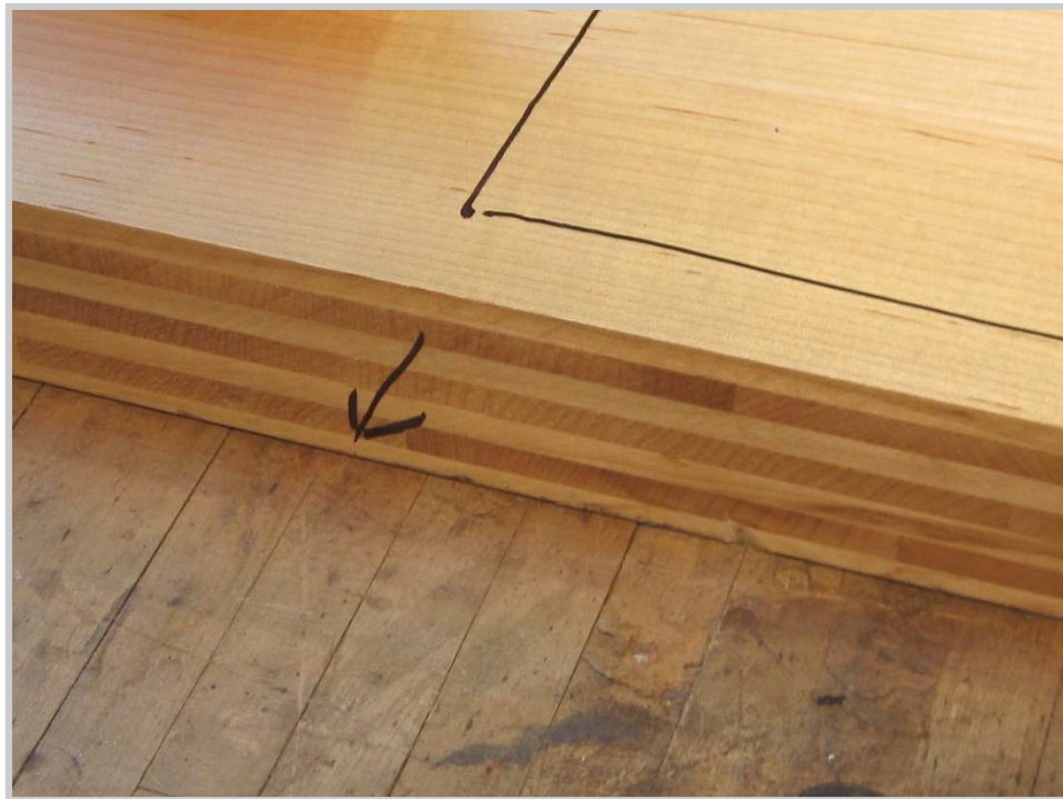
Photo 117: The slant of the cut is marked on the side of the pinblock.
