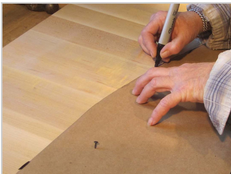
Photo 114: She then uses a marker to transfer the line produced to one of the new pinblocks.
