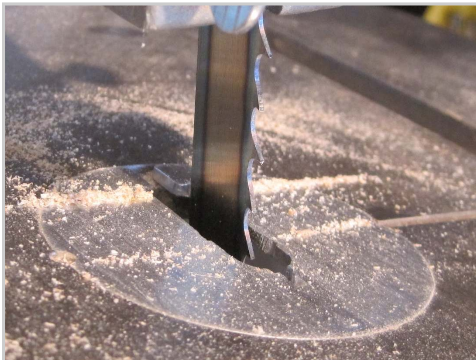
Photo 118: The 3/4" blade is set at a 3.5 degree angle to the table to match the angle of the inside of the flange on the cast iron plate. The closer the match of the cut surface of the pinblock to the flange, the less work will need to be spent in fitting the pinblock.
