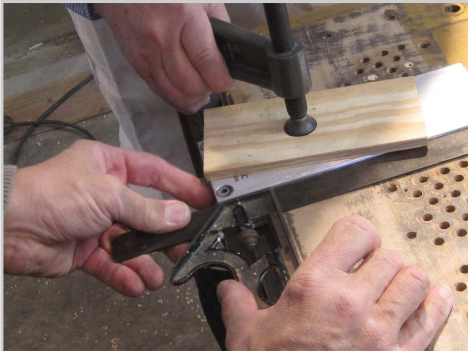
Photo 103: Advancing the jig after each hole is drilled becomes a team activity, with one person removing the clamp and the other person squaring the jig up.
