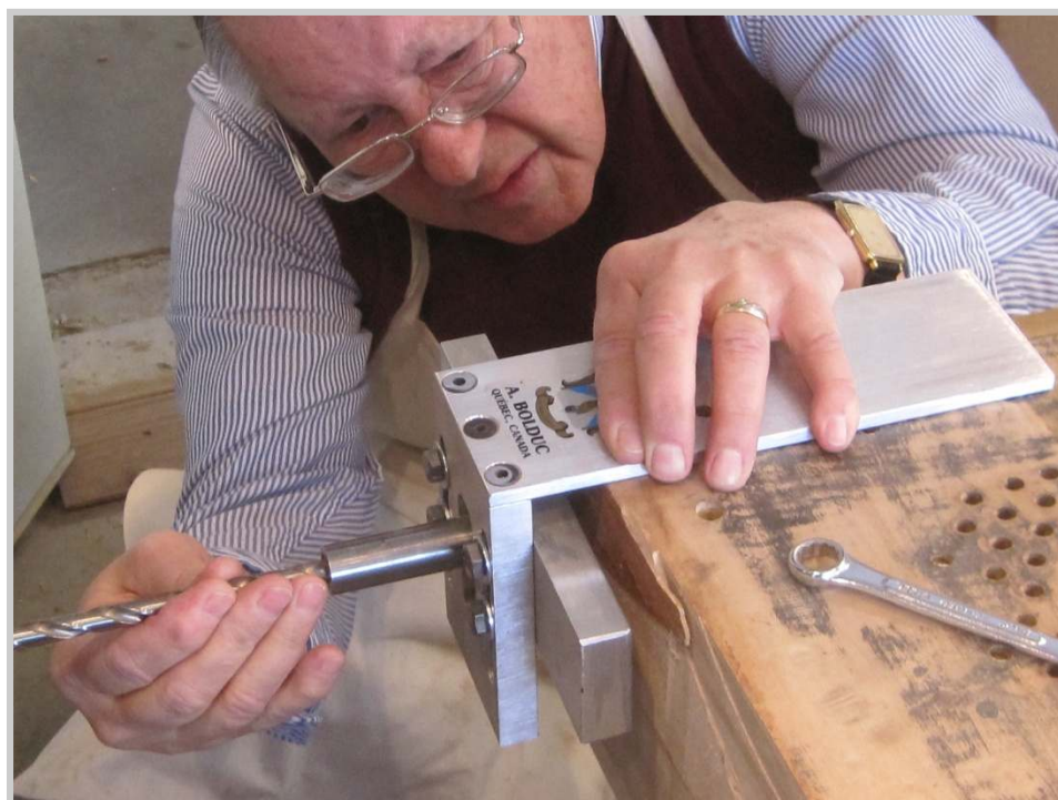
Photo 99: Neil Donald starts off the day by adjusting the jig from Bolduc Piano that will be used in undercutting the old pinblock. Here he sets the depth for the drill bit guide. The beauty of this system is that the face of the pinblock is preserved for later reference. If a router were used, there would be nothing left of the old block to refer to.
