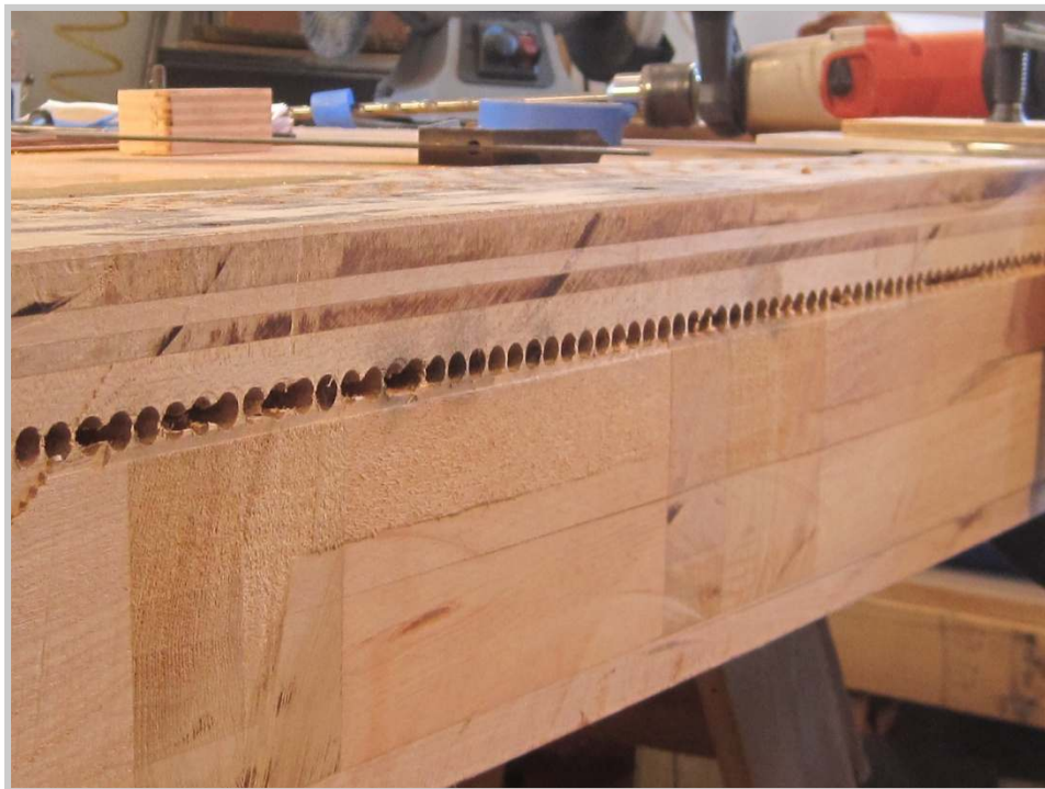
Photo 111: By mid-afternoon, the line of holes extends most of the distance to the opposite side of the pinblock. Not enough to complete the removal on this day, but close enough that an easy morning of work at the next meeting will finish the job.
