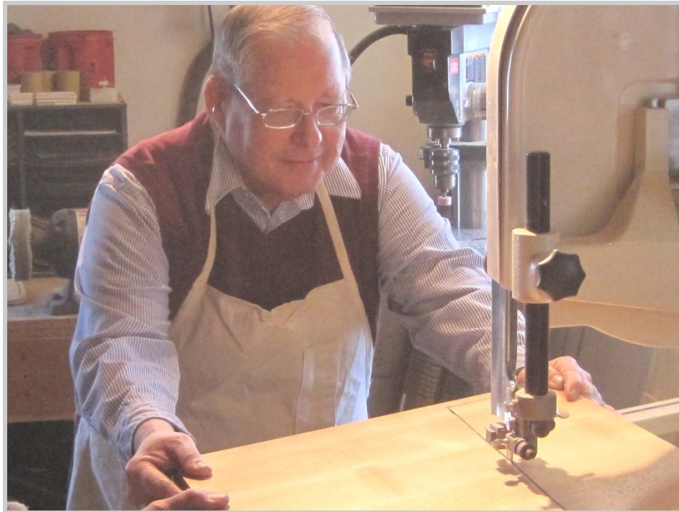
Photo 121: Don Neil finishes the cut on the WNG pinblock.
