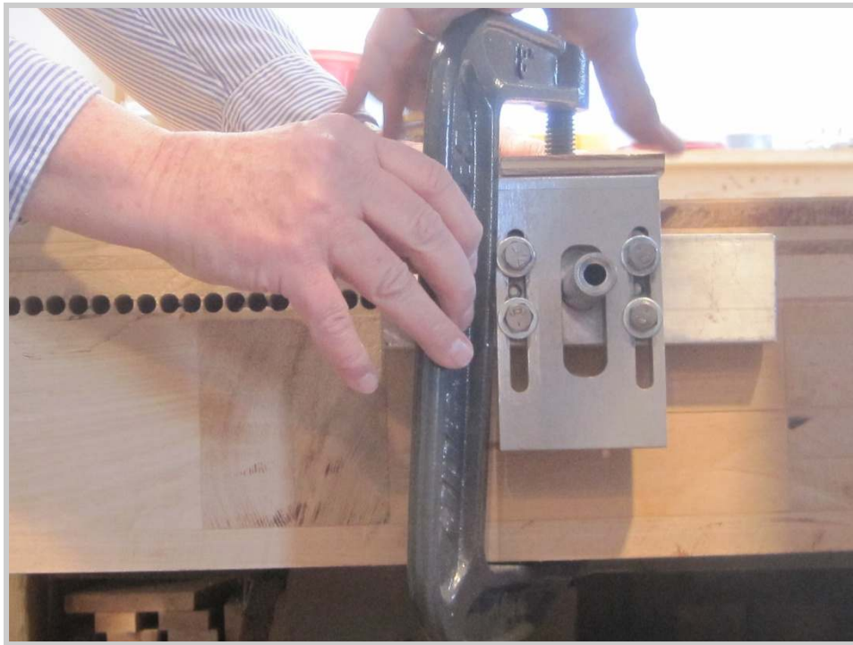
Photo 110: As the line of holes length, the process of resetting the jig becomes more efficient, with the chapter members working together like a pit crew at NASCAR changing tires.
