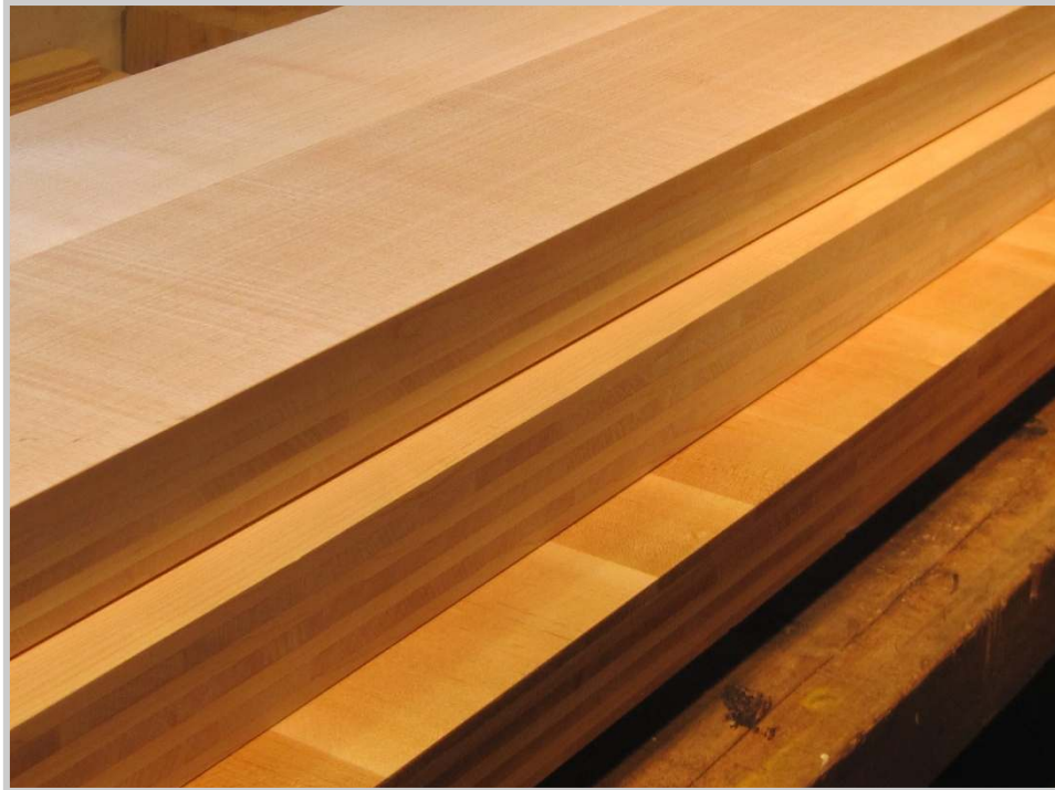
Photo 115: From top to bottom, the new pinblocks from Central Michigan Piano, Pianos André Bolduc and Wessell, Nickel and Gross. All three are great examples of premium pinblocks.
