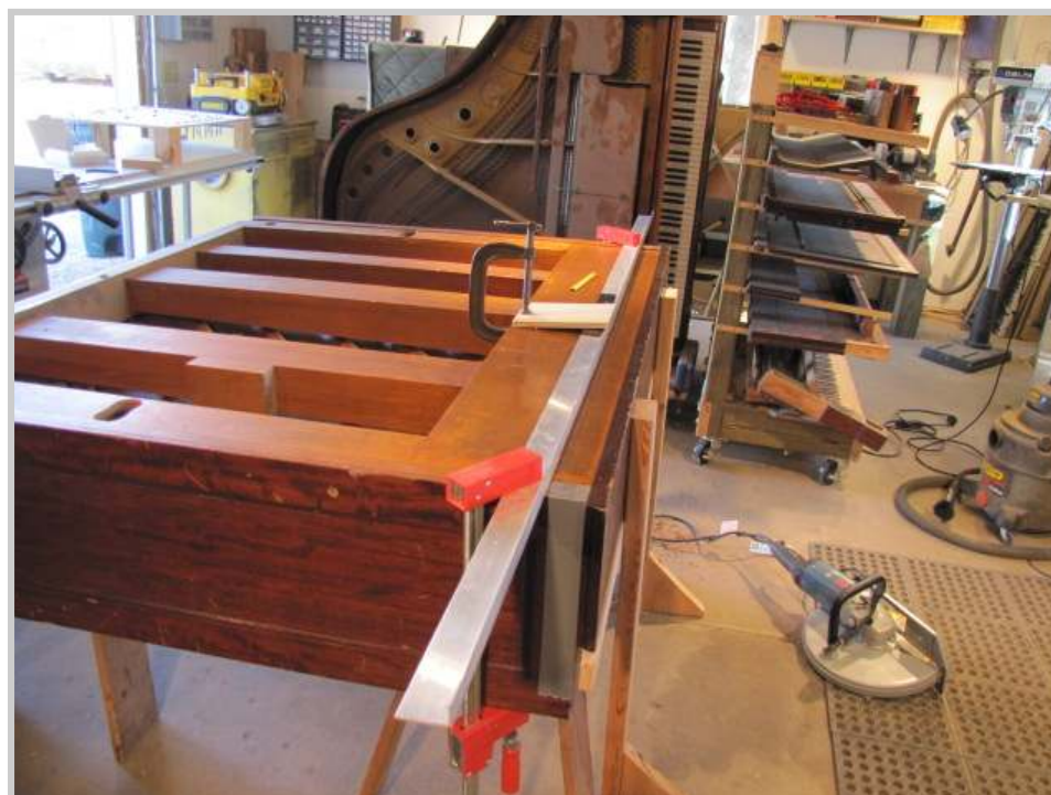
Photo 70: A straightedge for the saw to run along is clamped at a distance of 2 1/16" from the underside of the top.
