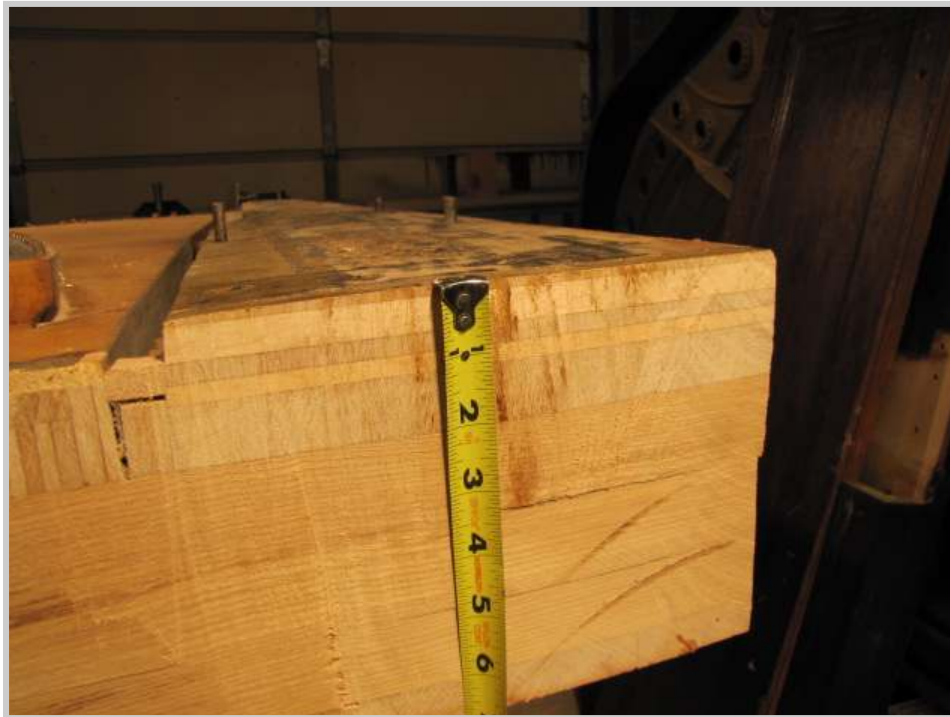
Photo 82: The side of the pinblock exposed. Five unequal layers totaling 2" in thickness.
