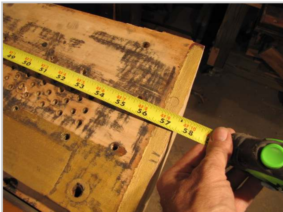
Photo 83: The width of the pinblock. The old block will be routed out from side to side.
