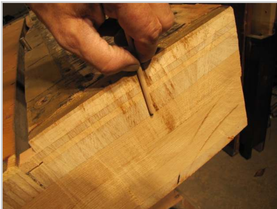
Photo 85: The old pinholes extend to the full 2" depth of the original pinblock.
