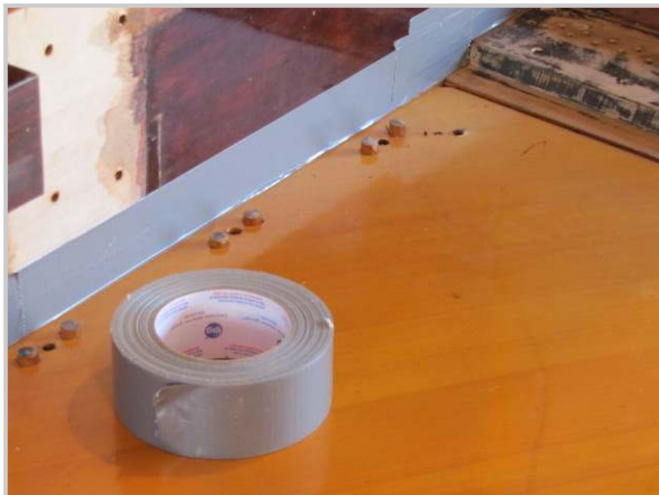
Photo 57: Big projects often have simple beginnings. Here, tape is applied to help prevent damage to the veneer on the inside of the case during the sawing operation to follow.
