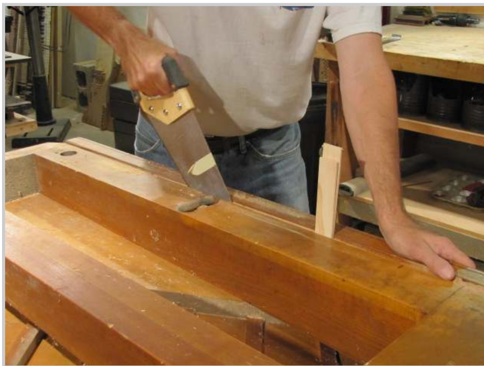
Photo 78: Additional sawing is necessary, but because of the width of the sides, using the cut-off saw is not possible. After briefly using the reciprocating saw, I settle on a sharp hand saw with its stiffer blade. As the cut progresses, wedges pry the side away from the post. I occasionally test to see if the glue joint will crack.
