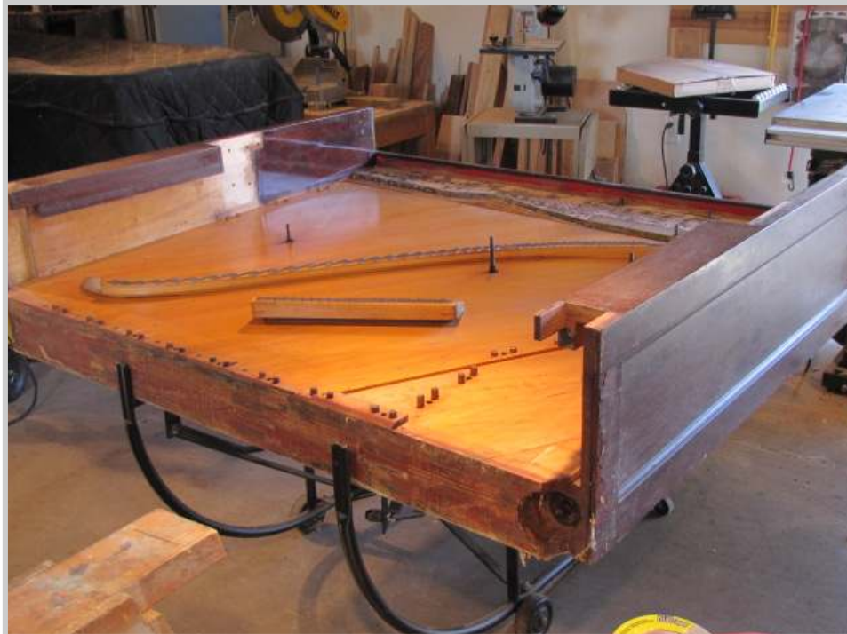
Photo 56: Before the next official shop day of my chapter of the Guild, I want to remove the back of the split top, and the sides of the piano, so we can focus on the pinblock, case parts, action work and other details which are more suited to a group effort. .
