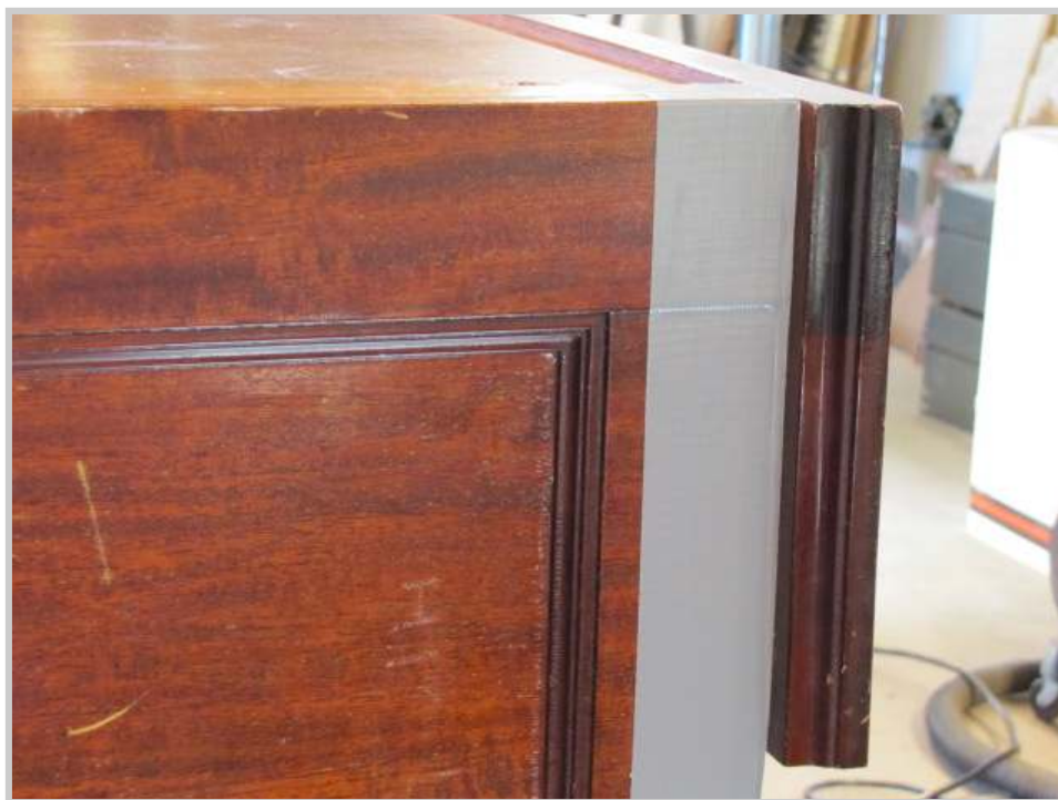
Photo 68: Veneer along the top of the sides is taped off to prevent chipping.
