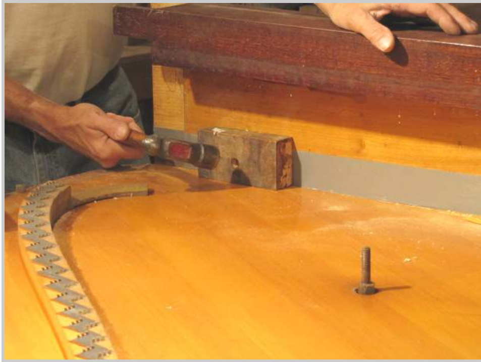
Photo 80: I then go to work on the opposite side. Besides prying, I attempt to break the glue joint with some sharp raps of a ball peen hammer. The joint finally gives way.
