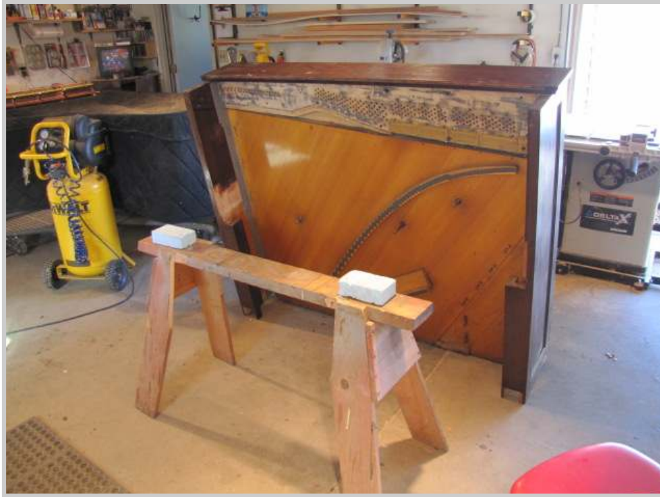
Photo 59: Although this looks precarious, it's really not. Without the cast iron plate, the piano is relatively light and balances in this position quite easily.
