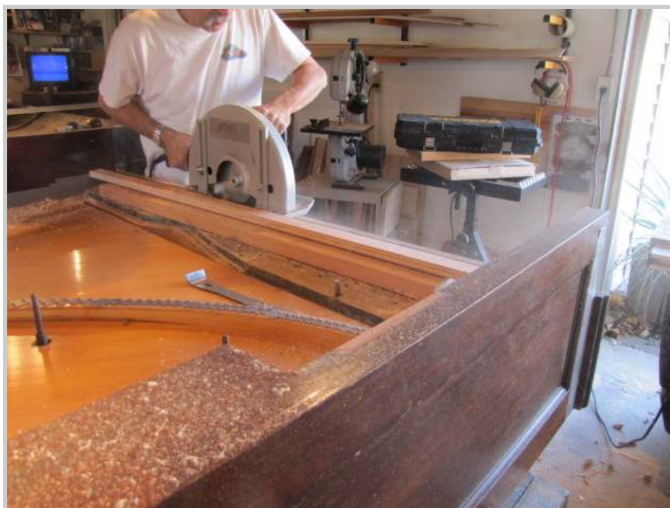
Photo 72: With the cut from the backside completed, the piano is turned over so that a cut may be made from the front side. Even going at it from both sides, the top is not completely removed.
