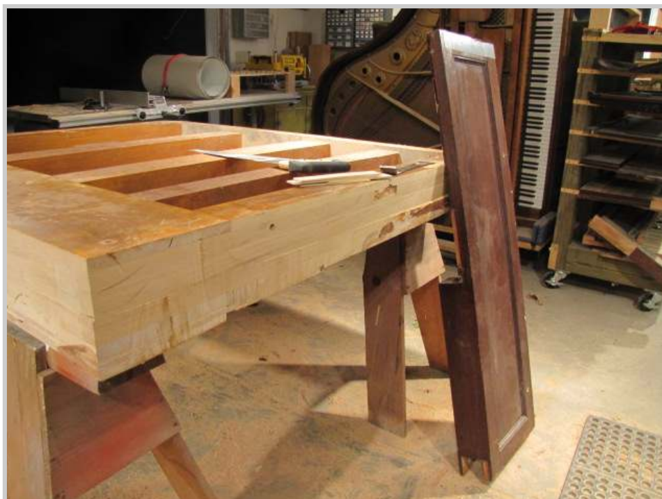
Photo 79: Finally, with most of the glue joint cut apart, I am able to break the side free. A little veneer from the inside of the case adheres to the framework, but not bad.
