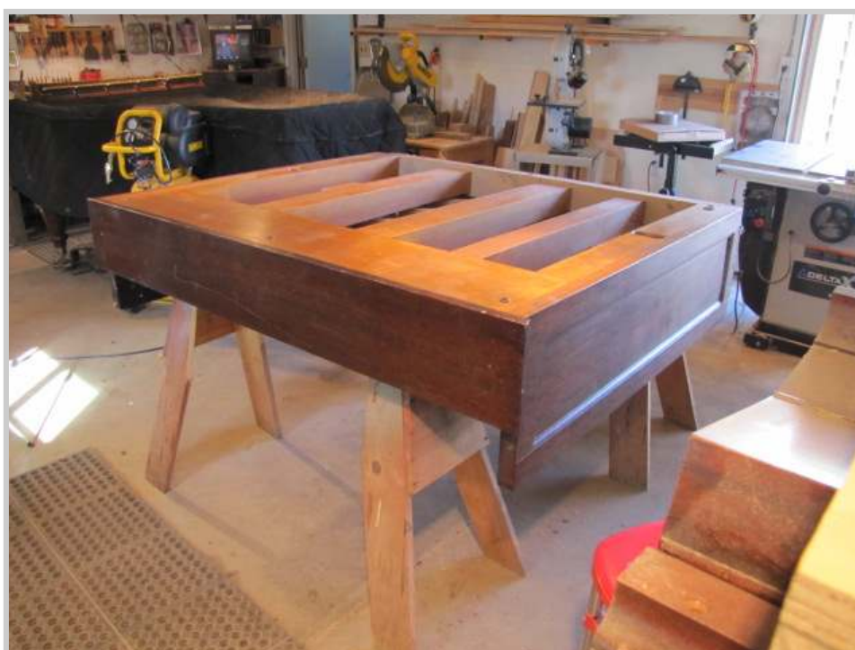
Photo 64: Before that can be done, however, the top needs to come off, since it overlaps the sides.
