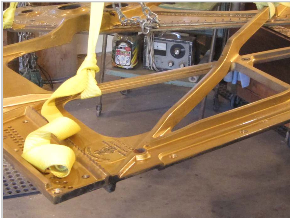
Photo 51: With the piano rolled out from underneath, the plate hangs in mid-air for a moment, before being lowered to the ground. Once untied from the straps, it's tilted on end to be moved to a safe spot for storage.
