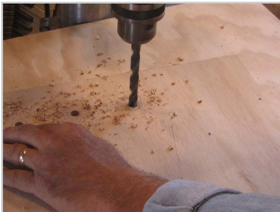
Photo 40: Holes are drilled in the storage board large enough that the plate screws will easily drop through to the head of the screw.
