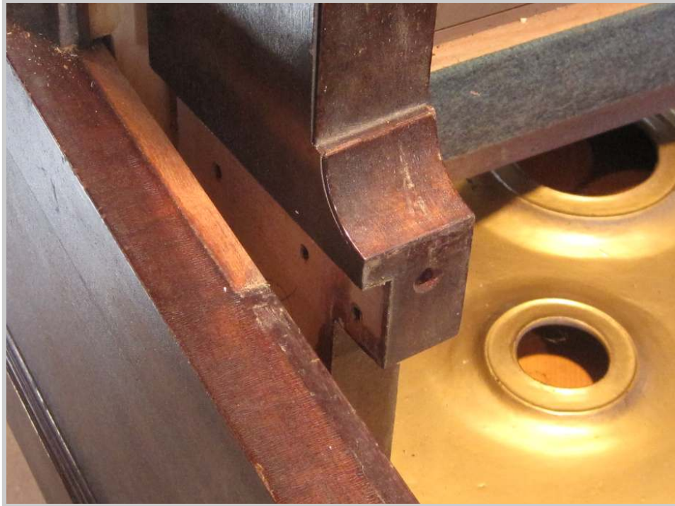
Photo 19: The arms also come off effortlessly. Usually these are screwed and glued to the sides. On this piano, when the screws are removed, the arms come right off. Cool!
