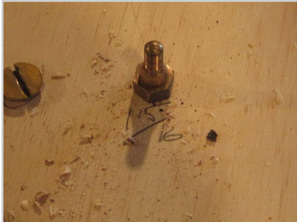
Photo 44: The height of each action bracket bolt is labeled right on the storage board. Post-It Notes have been known to peel off and blow away.
