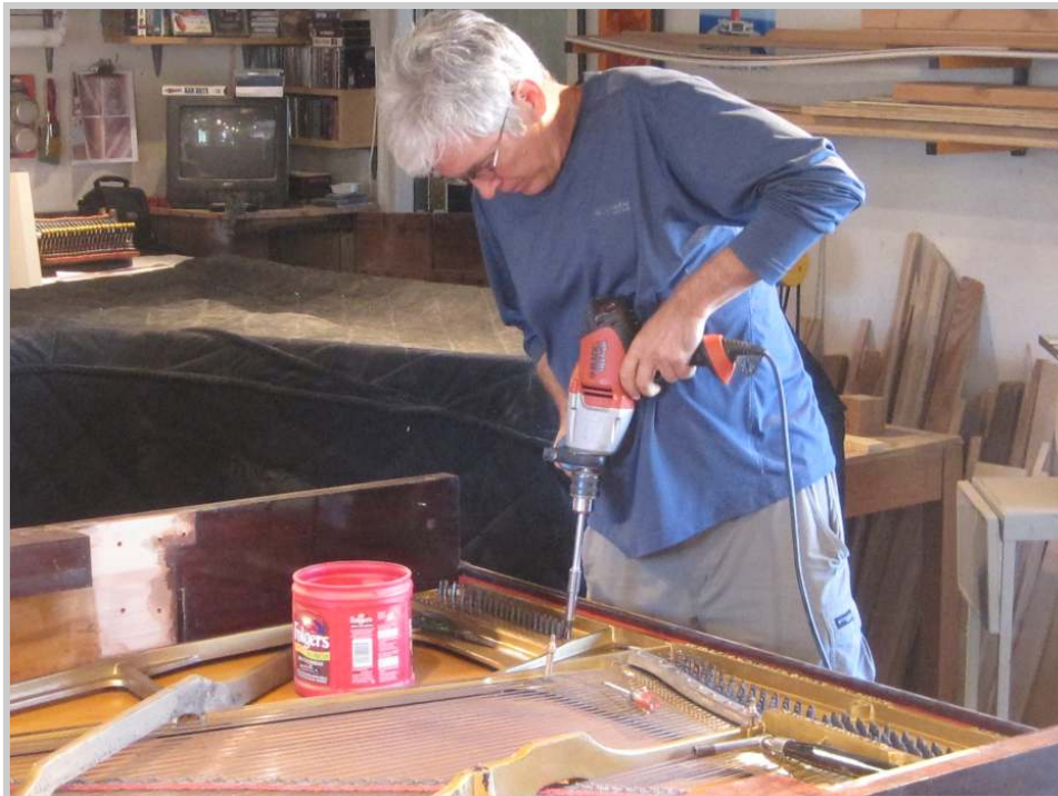
Photo 29: Tom Russell, RPT from Ames, stops by in time for lunch at Jimmy's, and then volunteers to give a hand for a short time. Here, he uses a drill to back out the old tuning pins. Back in the day I always did this job with a brace and bit. Isn't electricity a great thing?
