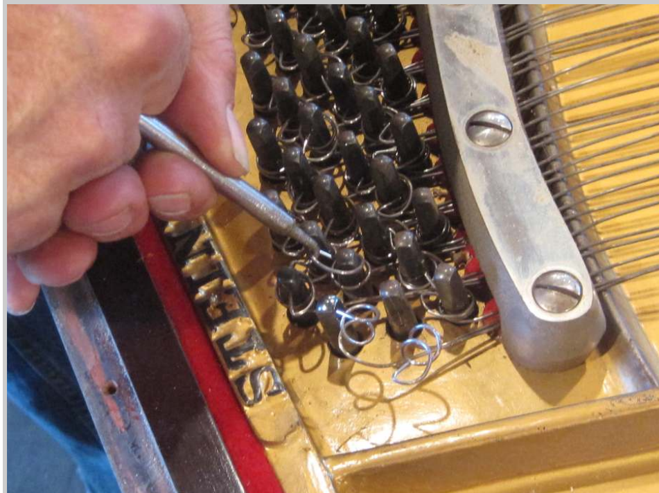
Photo 32: A string hook is then used to yank the coils free from the tuning pins.
