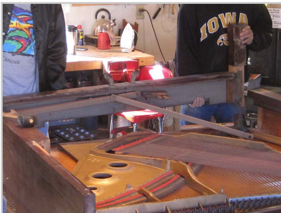
Photo 22: . . . and the entire lower portion of the piano comes off.
