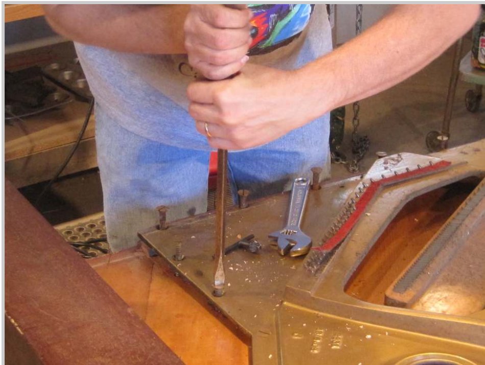
Photo 41: Using a large squared-shanked, flat-bladed screwdriver, the plate screws are removed. The wrench helps to get reluctant screws started (in most cases).
