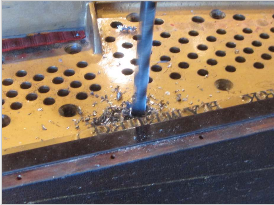
Photo 45: Perhaps because things had been coming apart too easily all day, 6 plate screws were absolutely frozen in place, defying our every attempt to turn them. After actually having a large screwdriver break trying to turn one of the screws, the last case option was resorted to - drilling out the head. The remainder of the screws will be removed later using an Easyout.
