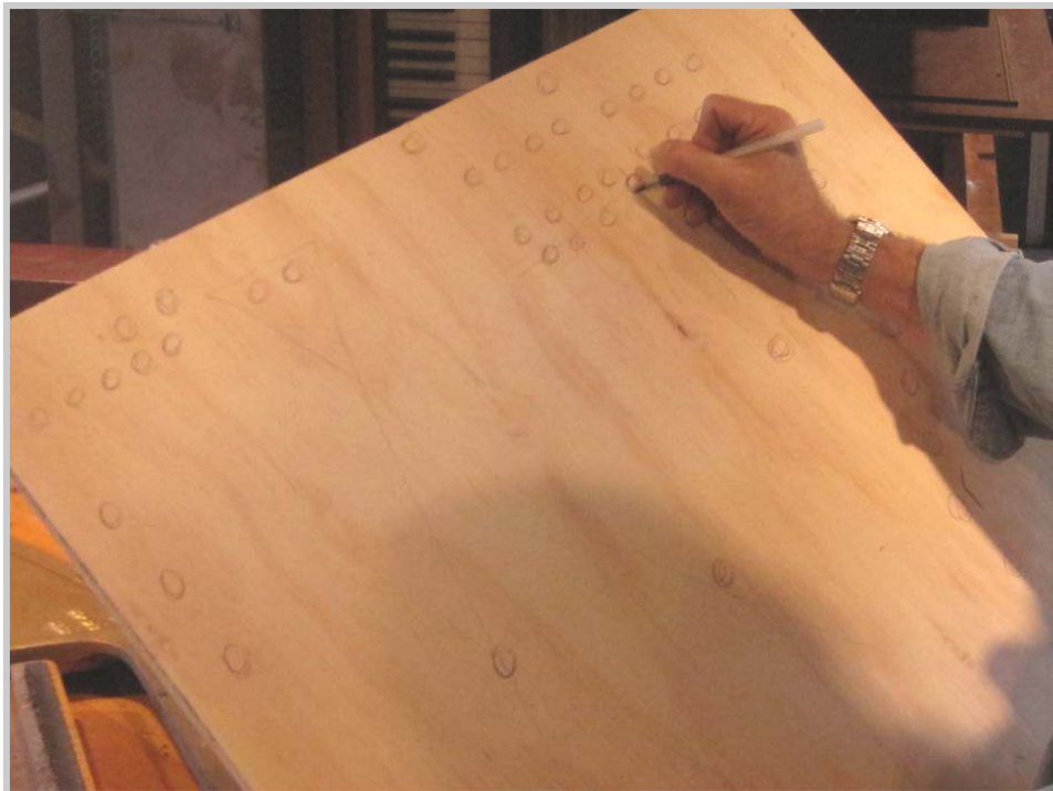
Photo 39: A storage board is drawn up for all the plate screws and bolts. It is essential that each plate screw be returned to the correct position. Sizes vary dramatically.
