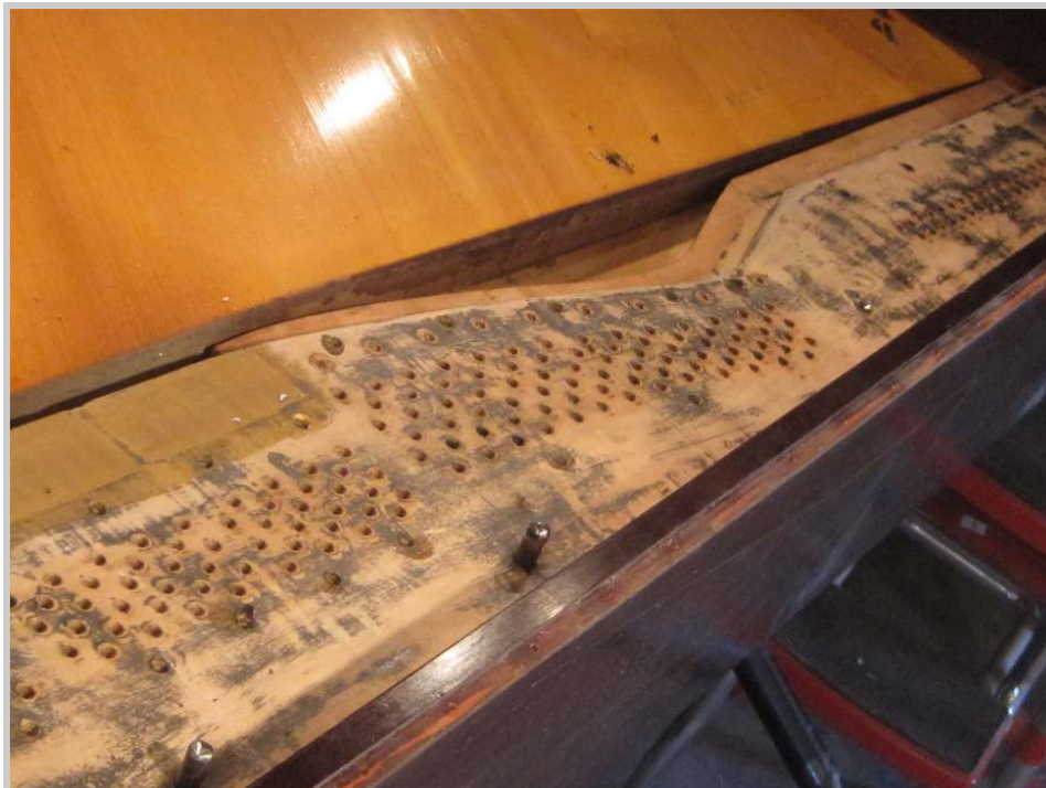
Photo 53: The pinblock is more complicated than what I anticipated. A curved cut inside a fitting bead will be necessary. More work than I was thinking, but very doable.
