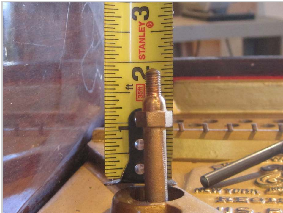
Photo 43: With action bracket bolts, it is important to measure the distance that they protrude from the plate. When these are eventually screwed back into place, the amount that they are turned down will be duplicated.
