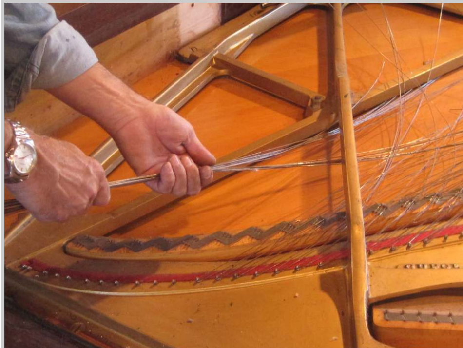
Photo 36: At this point, the remaining wire is pulled from the bridges and off of the hitchpins, removed and added to the recycling box.
