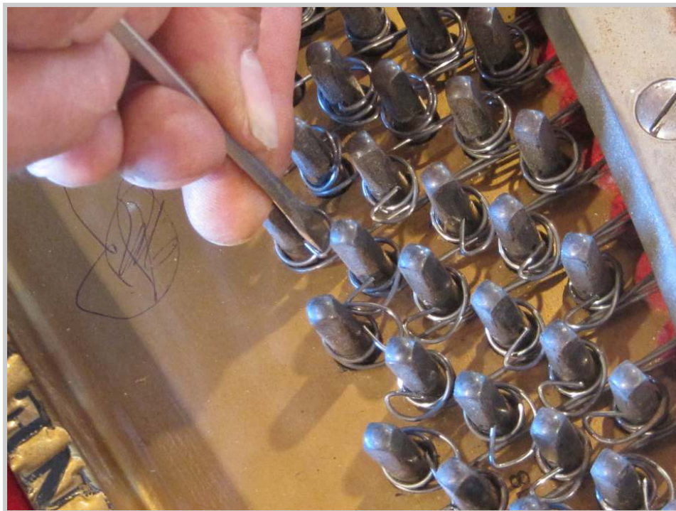
Photo 31: With the tension off from the strings, a small flat-bladed screwdriver is used to pop the becket loose from the pins.
