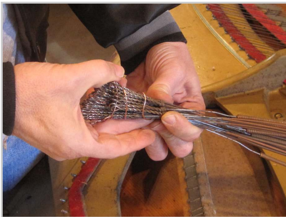
Photo 26: On the lower end of the piano, the bass strings are pulled loose from their hitch pins and bundled together with a copper wire.
