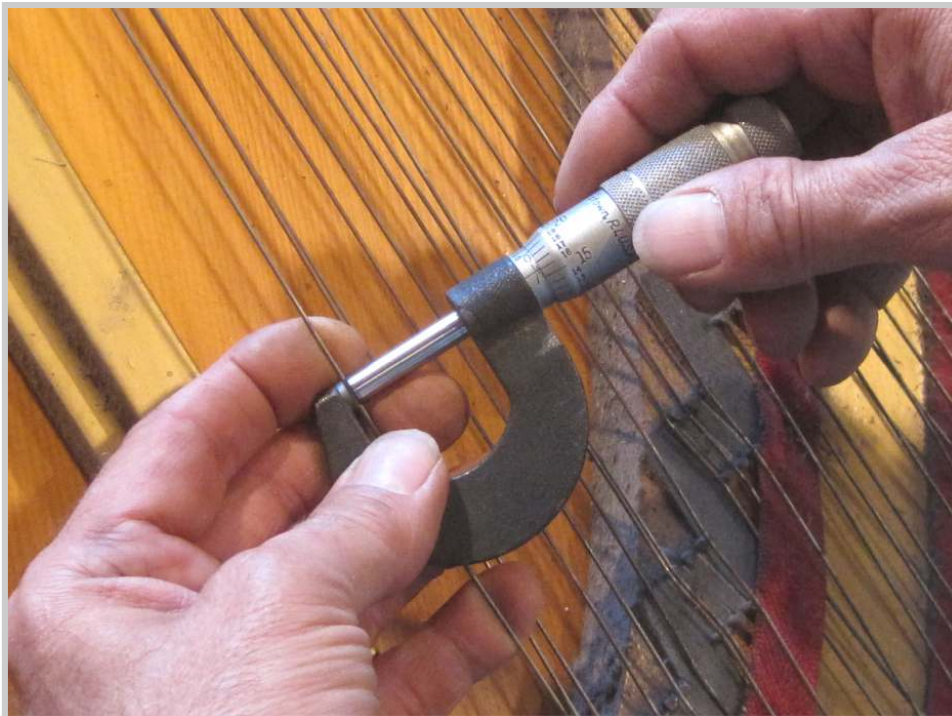
Photo 35: Before pulling the strings loose on the bass end, the wire sizes may be miked, although on this piano the gauges were stamped on the plate at the factory.
