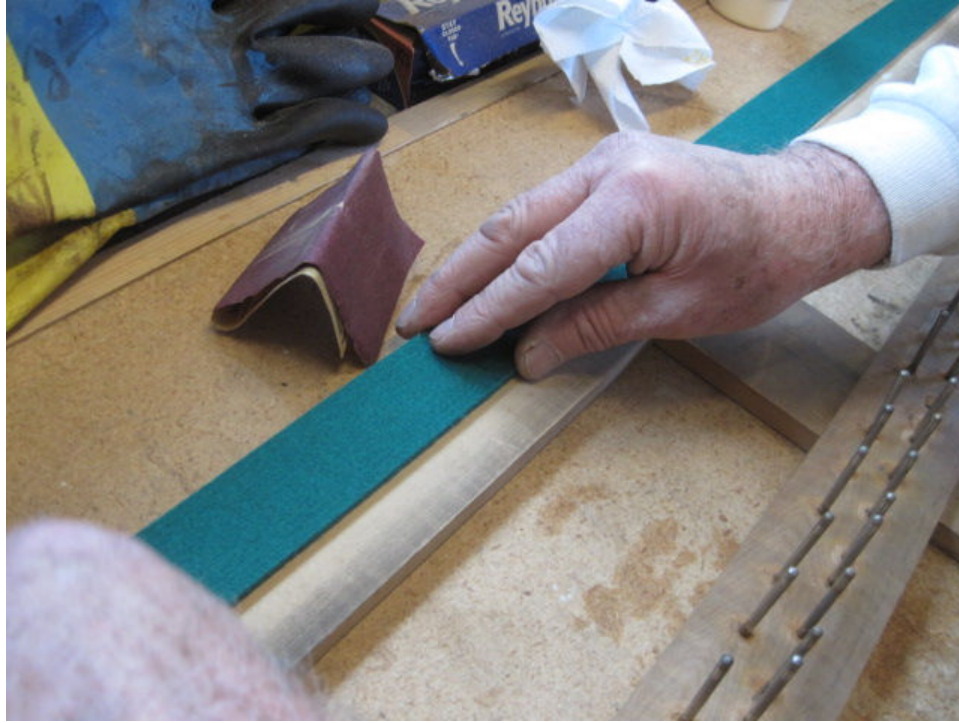
Photo 19: Back rail felt matching the thickness of the old felt is glued in place. Titebond is applied to the front of the felt, but not the back so that the transmission of sound when the keys fall back into place is kept to a minimum.
