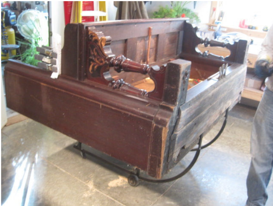
Photo 24: At a convenient break in the action, we put the piano on its back so that the casters, legs, arms and keybed might be removed. The more the case is disassembled, the easier the job of stripping and refinishing becomes, and the better the results.
