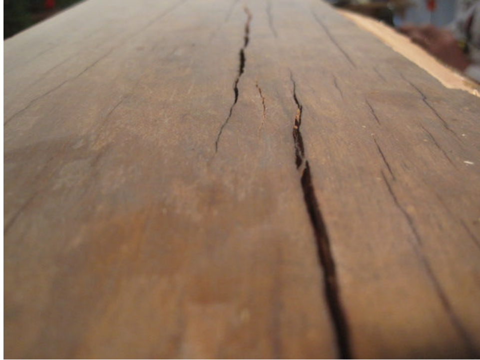
Photo 11: With the lid off of the top of the piano, I become concerned about the condition of the maple cap covering the top of the pinblock and the back posts. The cap is glued in place, and my guess is that the cracks signal a separation between the pinblock and the back posts and framework.
