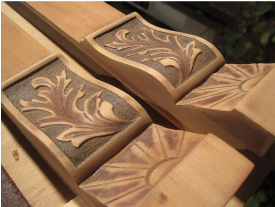
Photo 22: Each part progresses from the stripping bench to the sanding bench where the original beauty of the case begins to be revealed.
