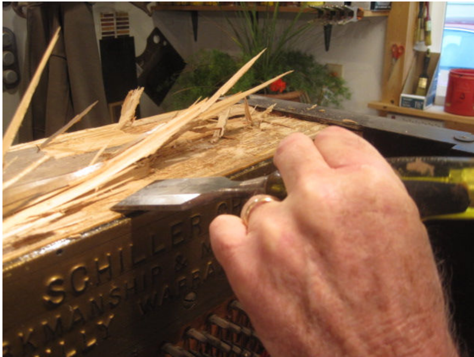
Photo 12: Dave thinks he can chisel the top off (obviously not in one piece – we'll have to make a new maple cap later down the road). The going is slow, however, and I set up the router to mill the top off.
