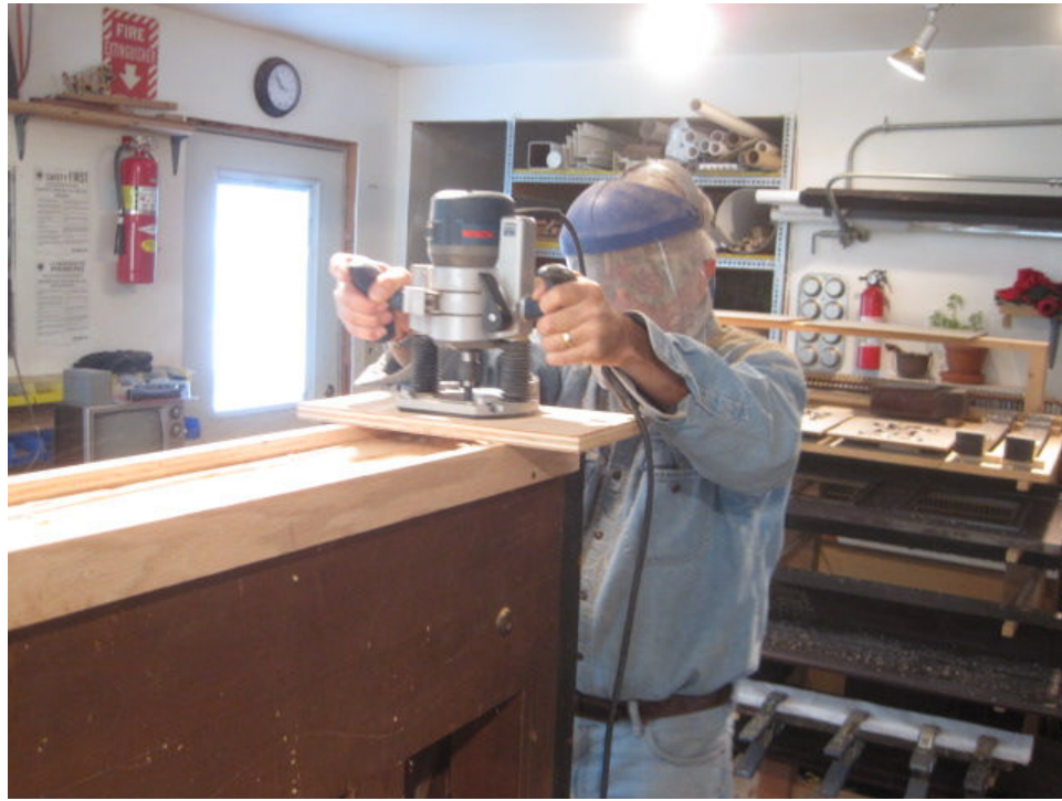
Photo 13: With chips flying at me at eye level, the regular goggles by themselves don't cut it. The rails on the front and back of the piano keep the cutter at an even level. The rectangle of plywood attached to the router and serving as its faceplate is wide enough to span the two rails.
