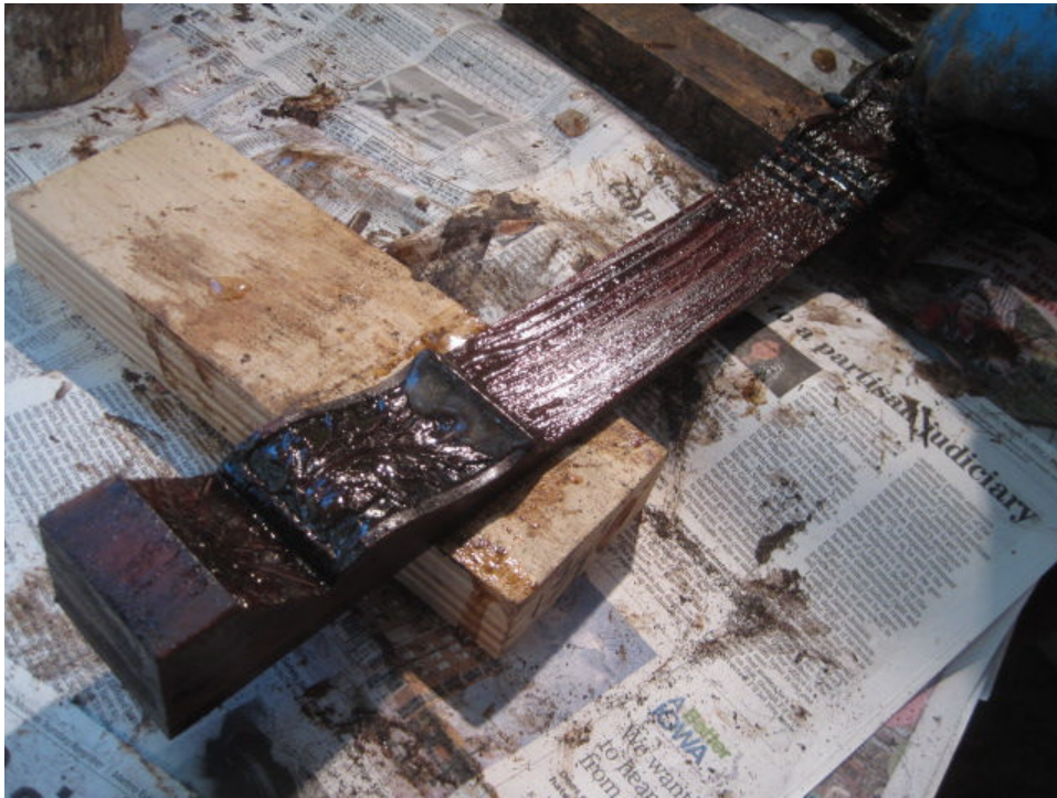
Photo 21: One piece at a time, Dave begins stripping parts. Multi-tasking works well at this stage, in that the stripper needs time to do its work. With several pieces coated with stripper, Dave will return to refelting the keybed, or a task in progress on another bench.
