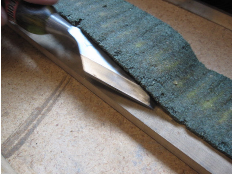
Photo 18: With the keys removed, and the keyframe on a bench, Dave removes the keybed felts.
