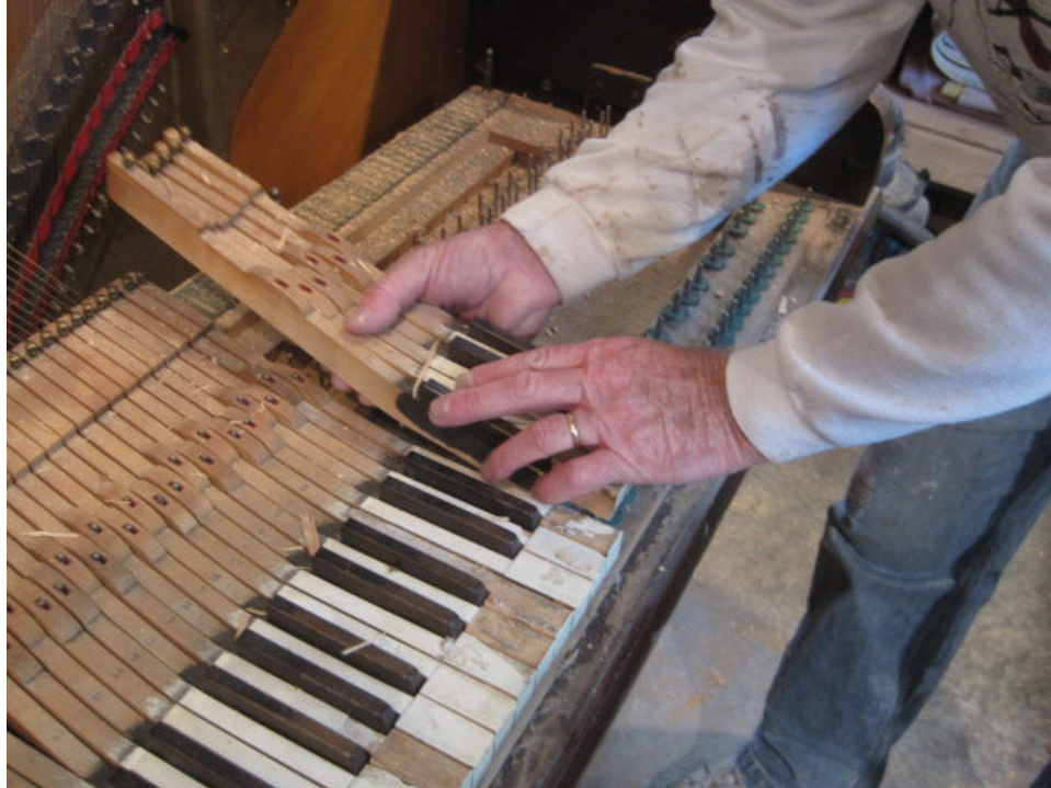
Photo 16: As I use the router up above, Dave removes the keys from the keyframe. The arms and keybed will eventually come off for easier stripping and refinishing.
