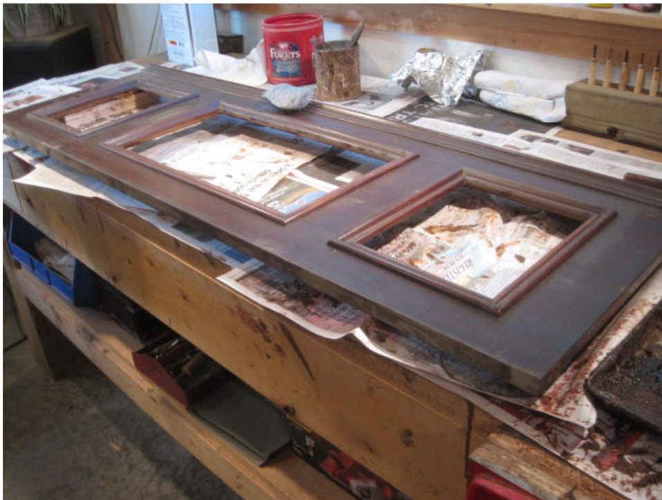
Photo 8: Dave (Richardson's) job on this piano will be to refinish the case, and do the repinning and restringing. Mine end will involve the keyset (keytop replacement and rebushing), hammer head replacement, regulation, etc. Dave starts removing and disassembling case parts and gets a bench set up to begin stripping and sanding.
