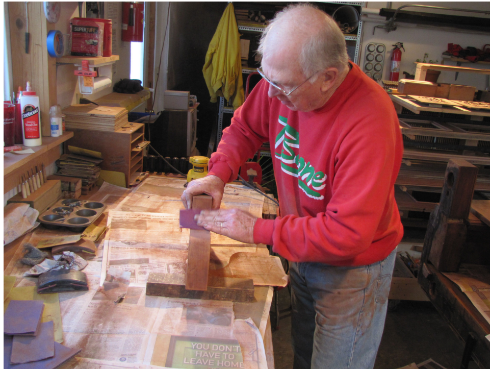
Photo 25: Dave presses on with the sanding, here working on one of the arms of the piano. Breaking the case down to its individual parts eliminates many of the tight corners which cause problems when sanding and buffing.
