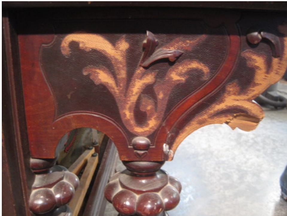
Photo 6: The case presents some challenges. This scroll work will need to be replicated. Time consuming, yes, but really fun work to do! The highly visible pattern is a lucky break. Also, the scroll work on the opposite leg is completely intact, which will take the guess work out of the duplication process.
