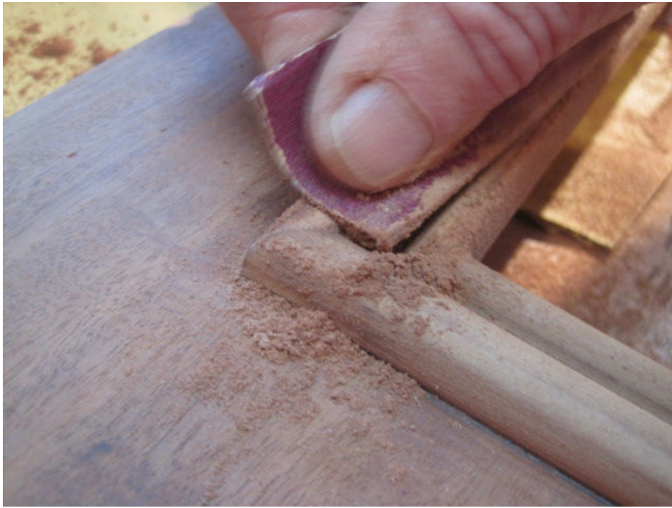
Photo 23: Hand sanding takes a lot of time and patience. The process we use is to go from 100 grit paper to 150 and finish with 220 on each piece. While we use palm sanders on large flat surfaces, such as the kneeboard and sides, many pieces are done strictly by hand.
