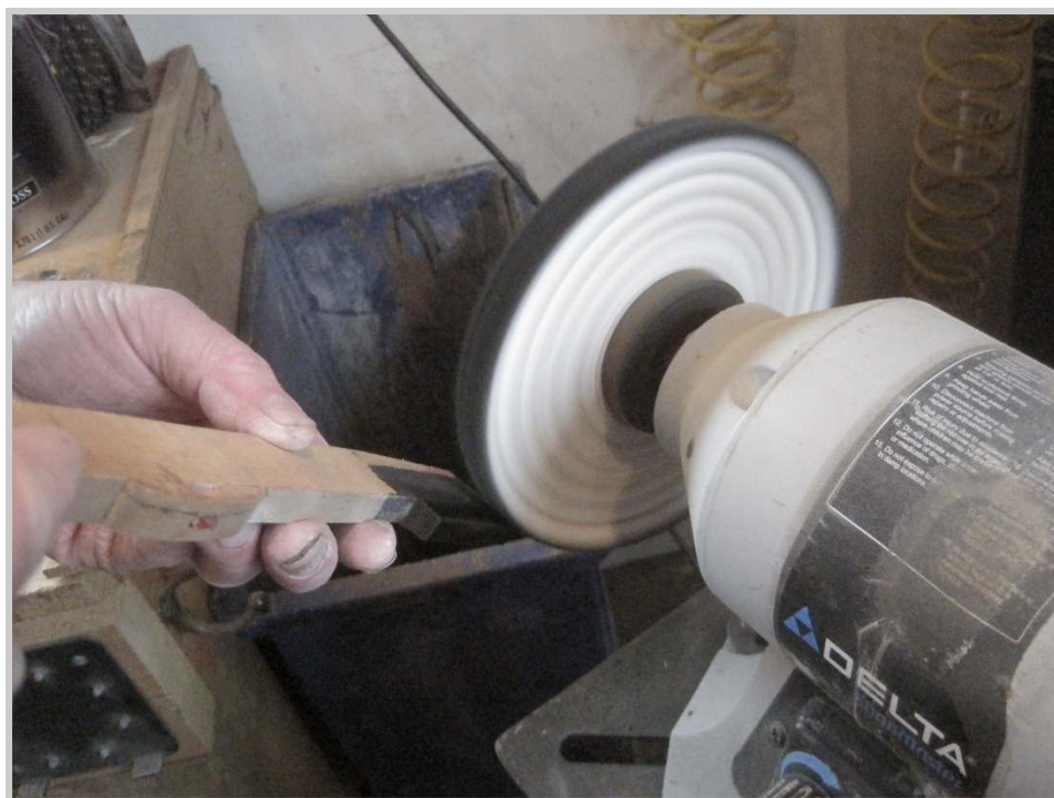
Photo 35: The ebony sharps are buffed with a special compound to bring out the beauty of the wood. .
