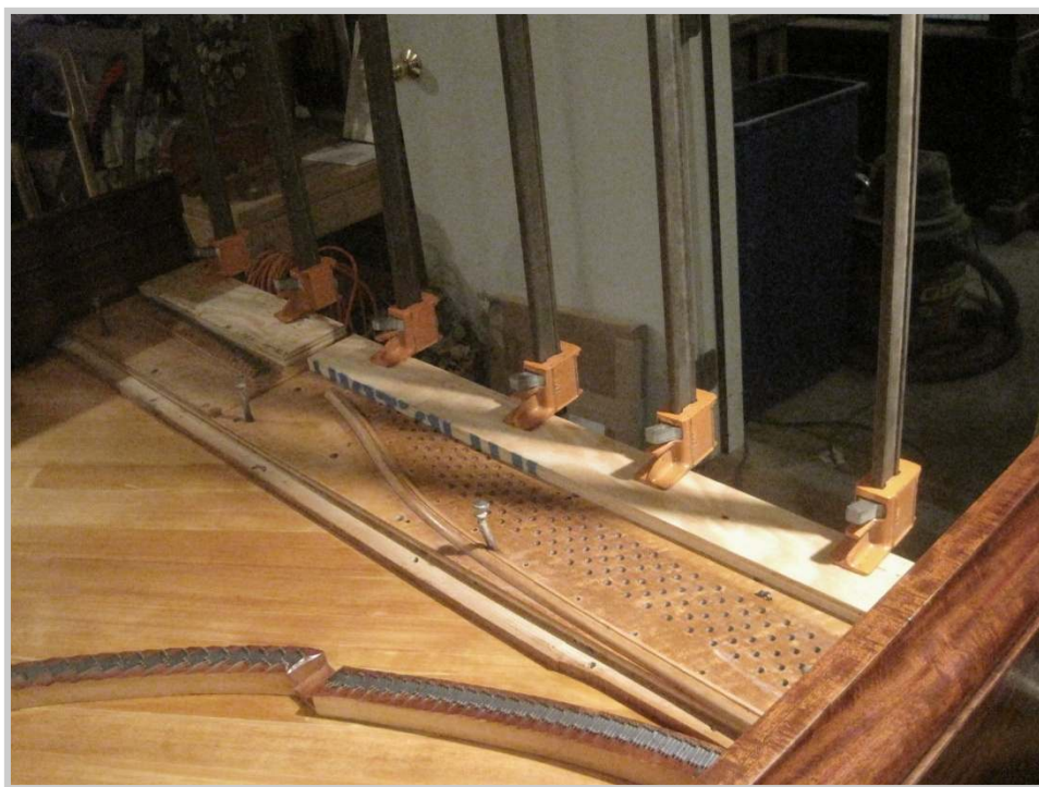
Photo 68: Before the plate is reinstalled, one other repair must be made—that of the loose joint between the pin-block and the back. Titebond glue is worked into the joint, then clamps are applied overnight.
