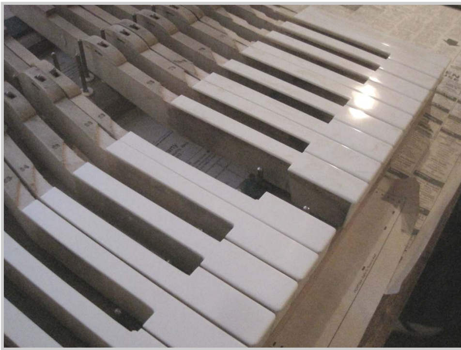
Photo 32: New keytops are hand filed after being glued on. The satin finish of the keytops to the left in the photo is a result buffing off the sheen with 0000 steel wool.
