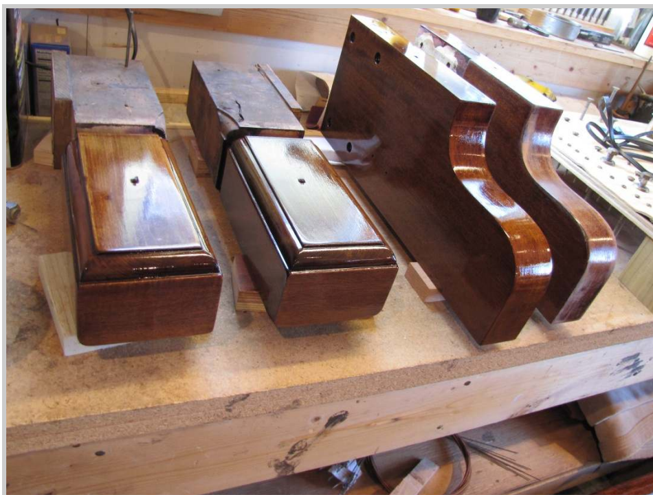
Photo 39: Parts after second coat has been applied. The arm on the far right is just one coated. Each coat of polyurethane is buffed between coats with 600 grit paper.
