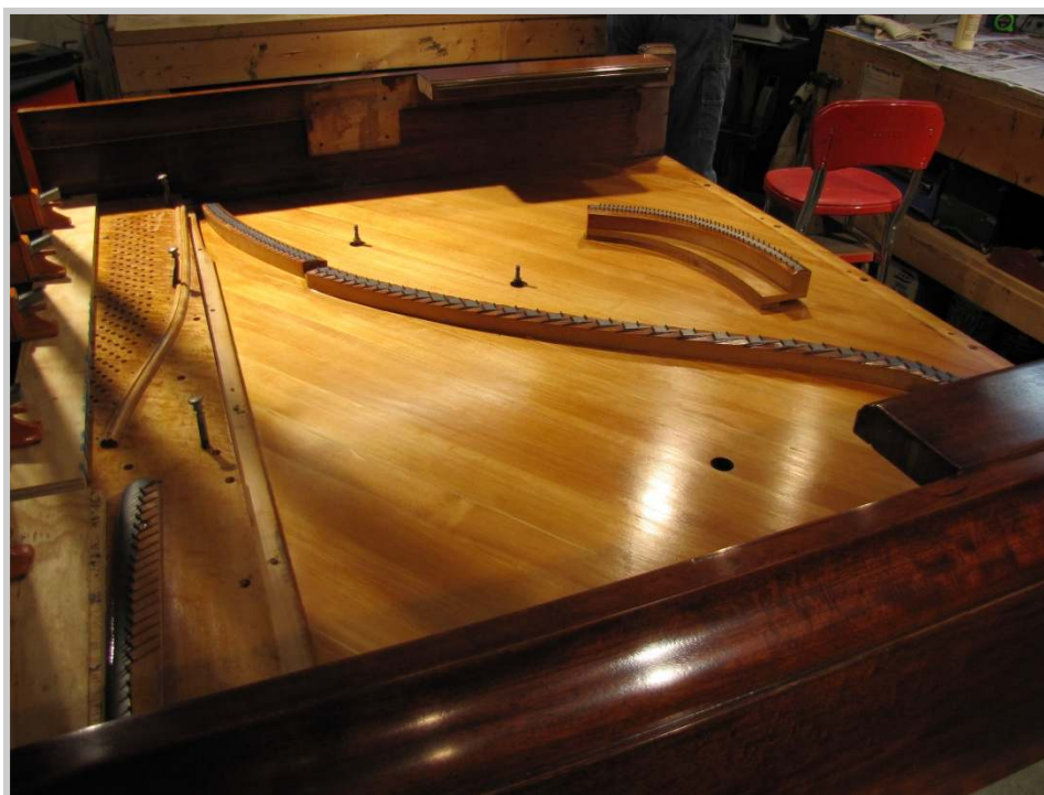
Photo 70: The completed soundboard, with bass bridge reinstalled. The bridges have also been shellacked, with the upper surfaces painted with DAG ® , a specialized lubricant. All is ready for the reinstallation of the cast iron plate, which has been cleaned and is ready to go.
