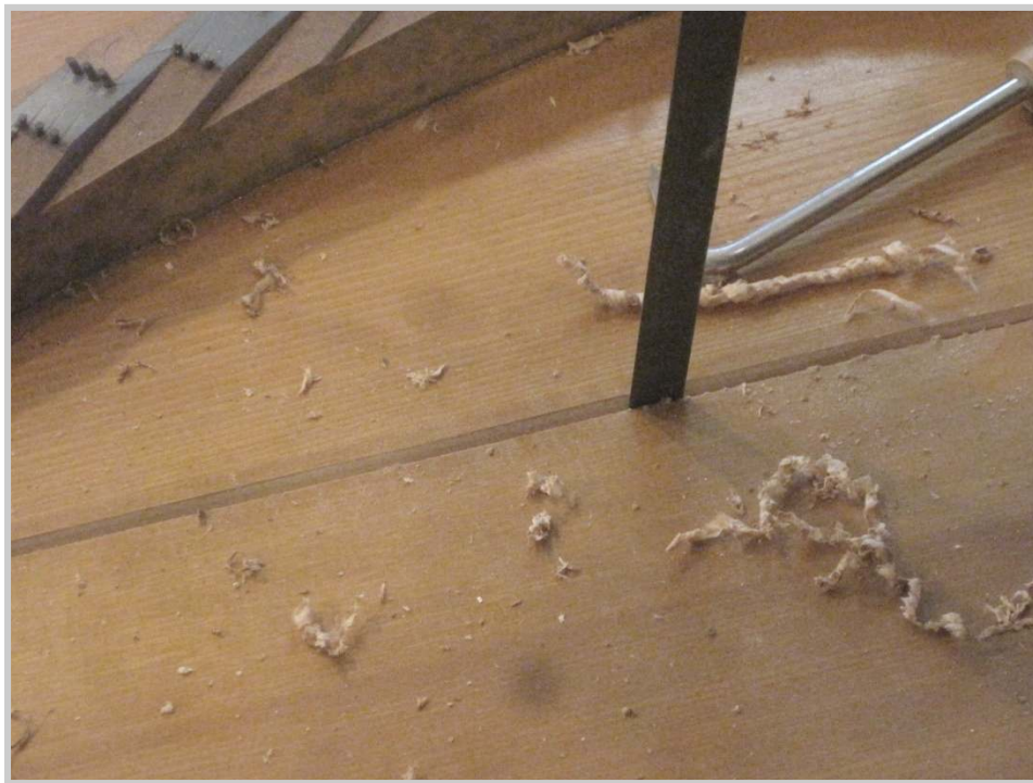
Photo 50: A piece of thin steel is used to easily find the ribs. Moving the steel from side to side, it will knock up against the solid ribs while cutting through any remaining material at the bottom of the v-shaped gouge. The start and stop point for each rib is marked with a scratch line on the soundboard.
