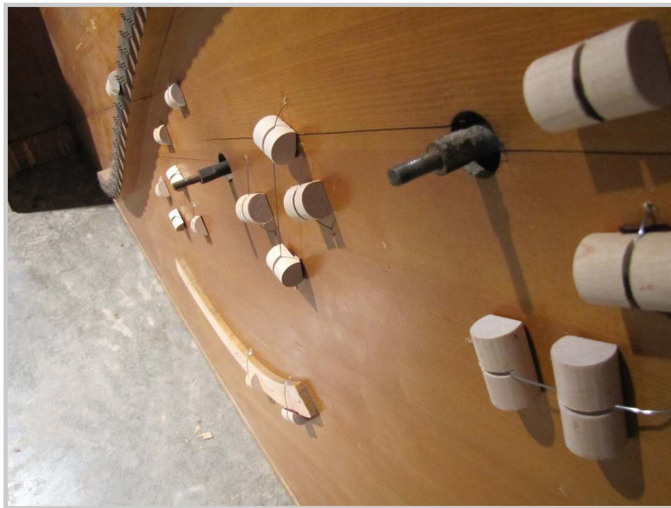
Photo 44: The wire clamping system as seen from the front of the soundboard.
