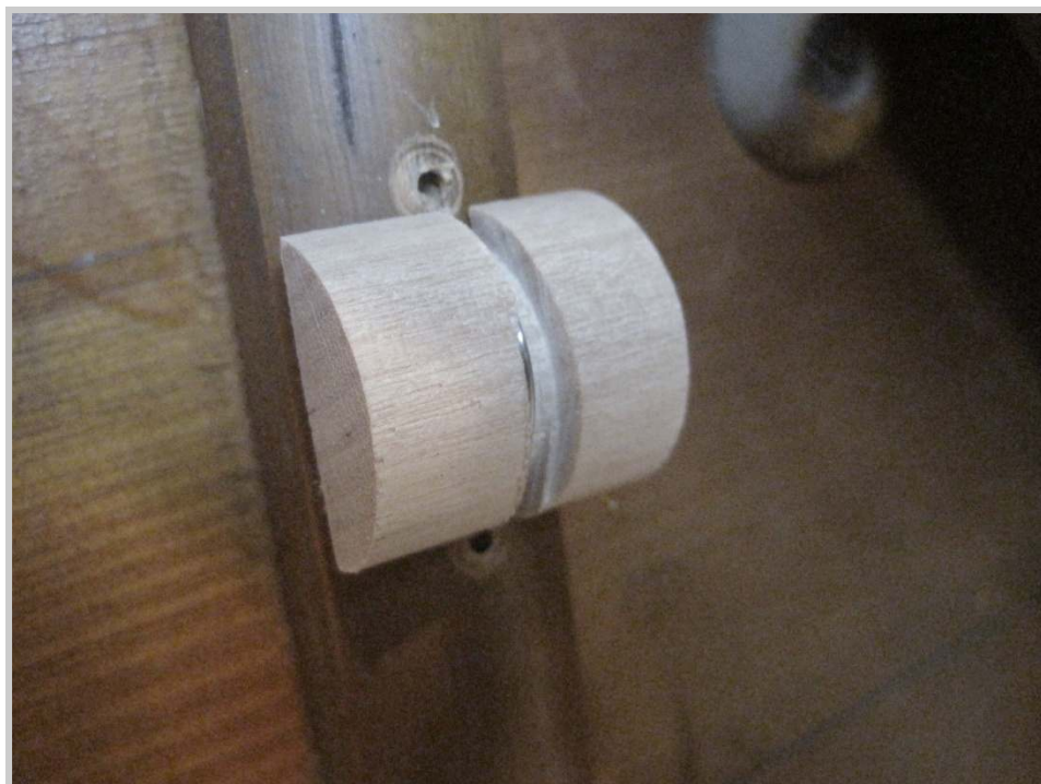
Photo 43: This is the device that makes this method work. Piano wire is threaded from the front to the back of the soundboard and around half-rounds which are channeled to allow the wire to easily slide as it is tensioned. The only damage to the ribs and the soundboard are the 1/16" holes drilled to allow for passage of the piano wire..
