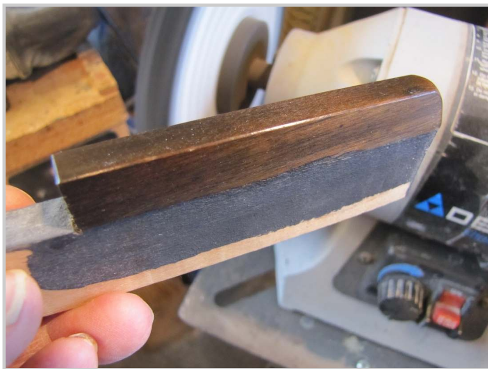
Photo 36: The beautiful reddish brown finish of the ebony sharps is brought out by polishing.
