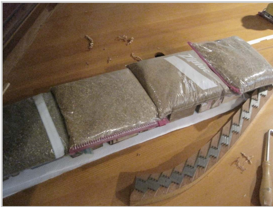
Photo 60: For tight fitting shims, bags of sand provide enough weight to hold the shim in place while the fast-acting glue sets. Gorilla glue expands a bit, filling any tiny discrepancy between the sides of the groove and the shim.
