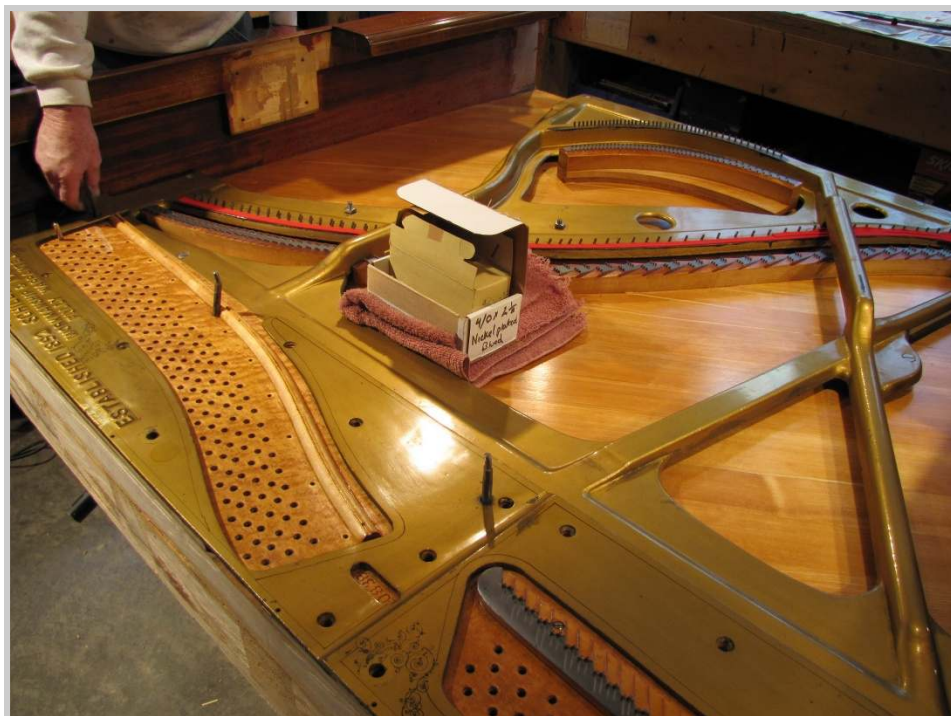
Photo 76: Test pins (both size 3 and size 4) are driven. The size 3's max out at 60 inch pounds, not enough.
