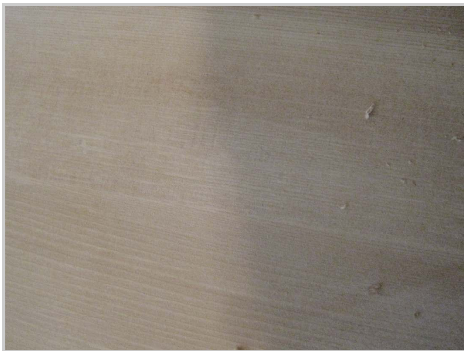
Photo 64: Well-fitted shims will blend in to the point of invisibility when the soundboard is sanded down. The only evidence of shims will be a difference in coloration with the shim material usually being a lighter shade.
