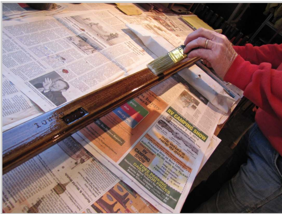
Photo 38: Turning to the case parts, Dave applies three coats of polyurethane to each case part. Staining was done to match the original finish, which will be preserved on the inside of the lid. The first two coats applied are high gloss for hardness— the final coat is satin for the desired appearance.
