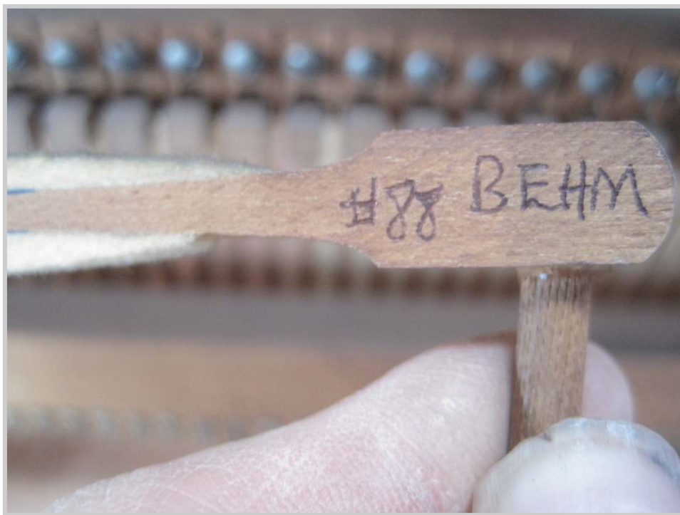
Photo 28: End hammers of each section have been removed from the action and are numbered to send to Schaff Piano Supply Company for duplication.
