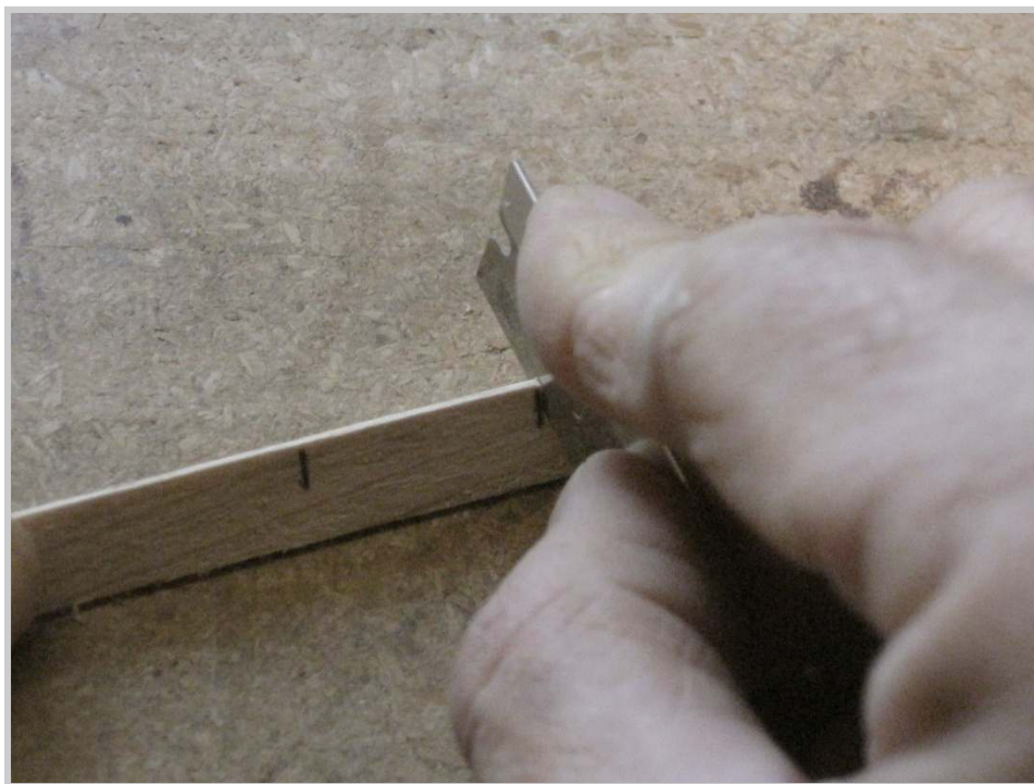
Photo 51: The sides of the shim to be used are marked for notching to match the scratch lines on the soundboard. The edges of the notches are first scored with a sharp razor by rocking it back and forth.
