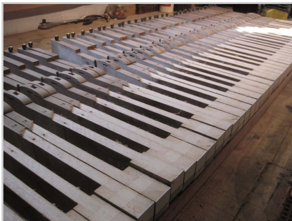
Photo 31: Turning our attention to the keys, I prep the surface of the natural keys for installation of new keytops. Since the new tops are a bit thicker than the original ivory, the very top of the keysticks are shaved off to compensate for the difference. The old fronts will also be removed prior to the installation of the new tops.
