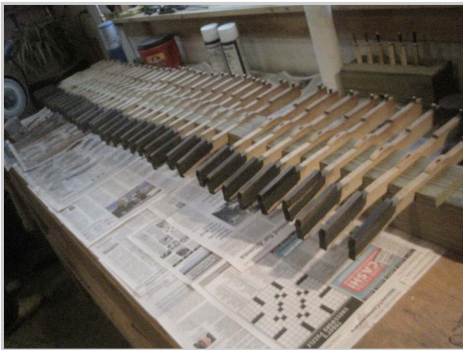
Photo 34: Sharp keys are placed in racks and the old lacquer finish is stripped off.
