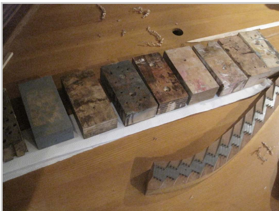
Photo 59: A row of wooden blocks are placed over the shim, with a layer of folded paper towels in between the shim and the blocks to prevent adhesion of the two wood surfaces. The paper towels will stick to the shims, but are easily scraped off once the glue has dried.
