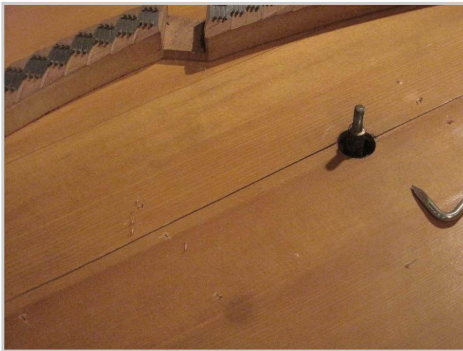
Photo 46: Laying the piano on its back once again, it is time to tackle the cracks which have opened up in the dry shop air. (The tiny holes which were used for the gluing of the ribs to the soundboard will be filled, and will be nearly invisible when the board is finished.)
