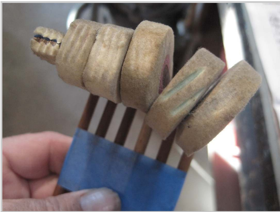
Photo 30: Wear and tear on the sample hammers being sent in for duplication—a clear need for replacement and not just a simple filing and shaping.
