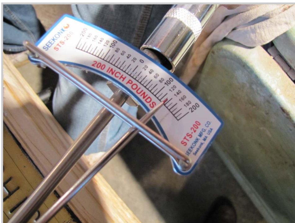
Photo 77: Size 4 pins test out at over 120 inch pounds—much more suitable. Smooth, tight turning, no ratcheting whatsoever. Blue, size 4 Denro ® pins will be used.
