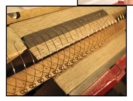
The springs are given fine adjustments while the set is held in place in the vise so that each of the springs lines up perfectly with its neighboring springs. Adjustments from sideto-side, and up and down are required to even out the line. A new length of fresh spring rail felt is now glued to the back of the hammer spring rail. It is essential that this felt be of the correct width and thickness. This felt is clamped in place in a press overnight to ensure adhesion.
