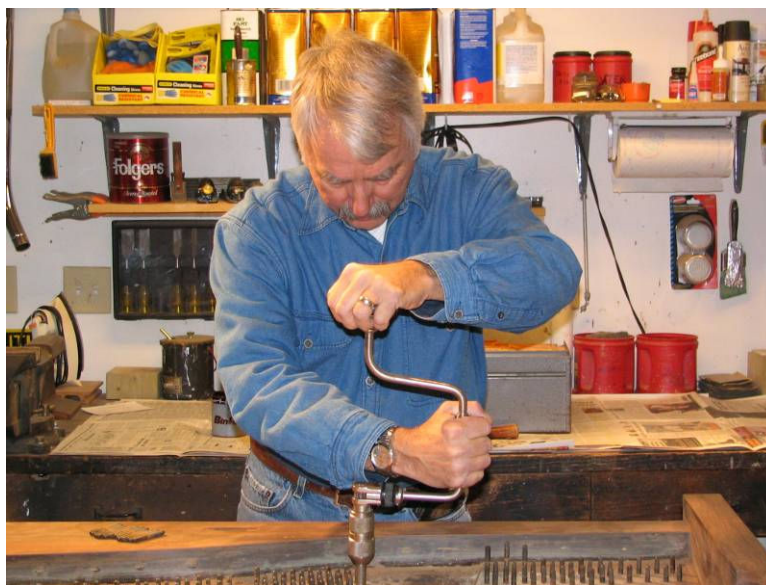
Photo #6: Removing pins using a brace
