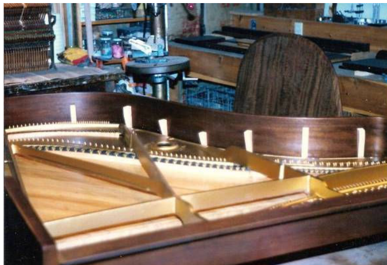
Photo 9: Positioning the plate using wedges
