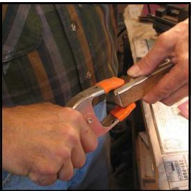
**Step 49:** Holding the back of the plate down with the thumb of your left hand, (it should still feel very hot) quickly apply a key spring clamp to the front of the key, slightly back from the very front of the key. Tilt the clamp slightly as you apply it so that the bottom jaw is slightly further back than the top jaw. (This will help prevent the ivory from pulling away from the seam between the front and the tail.)
