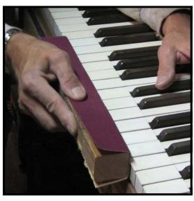
**Step 65**: Use a 11" piece of 2" x 2" lumber as a sanding block to even out the front edges of the keytops. Work back and forth across the keyset, checking your progress frequently to avoid taking off more ivory than absolutely necessary. Once the stand-outs are even with the surrounding keytops, quit.
