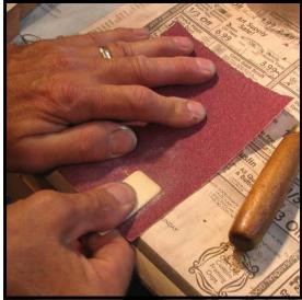
**Step 30:** Once the underside of the ivory has been scraped, turn the key over and sand with a coarse (100 or 150 grit) sandpaper. It is best if the gluing surface of the ivory be slightly roughed up and not too smooth, to guarantee a better glue joint between the ivory and the keystick. Sand one half of the ivory, then flip it around and sand the other half.
