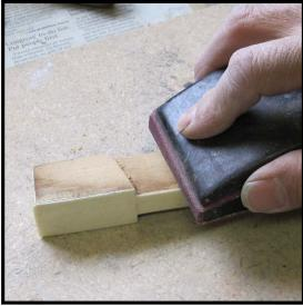
**Step 56:** Using sandpaper with a sanding block, remove the excess glue and any discoloration on the sides of the keys. Start with 100 grit paper and finish with 150 or 220 grit.
