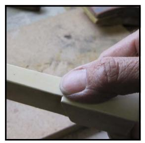
**Step 58:** Check the joint between the head and the tail for unevenness in height. A discernable difference in thickness will mean that either the head or the tail will need to be sanded down flush.
