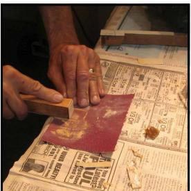
**Step 17:** Finish by cleaning off any remaining residue with sandpaper. Use 100 or 150 grit paper turned grit side up on your bench.
