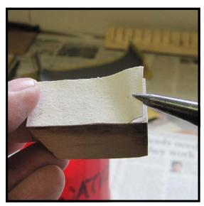
**Step 44:** Apply the wafer to the top of the keystick, making sure that it's up tight against the seam between the front and the tail.
