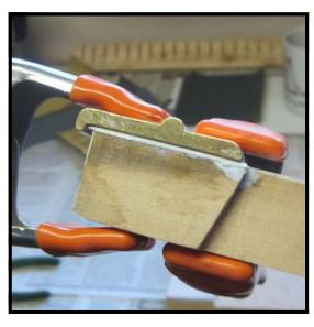
**Step 51:** Examine the ivory from the side to make sure that the back of the keytop has not lopped over the top of the front edge of the tail. Make sure also that the ivory has not slid slightly from side to side, leaving a portion of one side of the key uncovered, while the opposite side has an excess of ivory hanging over.
