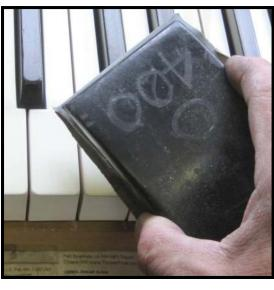
**Step 67:** Round the front edges of the keytops with a sheet of 400 grit paper on a sanding block. Use easy strokes, rotating the block slightly on each stroke. Work back and forth across the keyset until a even, gentle rounding is obtained. Follow this up with several swipes of 600 grit.
