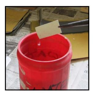
**Step 43:** After 30 seconds, remove the wafer from the water and tap off any excess.
