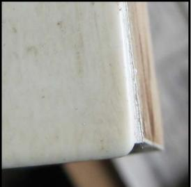
**Step 54:** When the clamps come off, you should find that the ivory has bonded solidly to the keystick. Any glue which has extruded from the joint will be hard to the touch and sandable.
