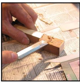
**Step 16:** Again try using a sharpened chisel. Instead of scraping the adhesive off, it is some times more effective to slice it off. Keep the flat side of the chisel flush with the top of the keystick, and swivel it back and forth across the surface to remove as much of the substance as possible. Again, be cautious not to remove wood from the keystick itself.
