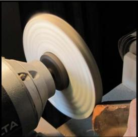
**Step 68:** With your final shaping of the ivory complete, it is time for polishing. Start by loading your dedicated polishing wheel (Cat. No 475) with Tripoli bar polish (Cat. No. 425). Set your grinder on its lowest speed. As you work, occasionally rake your wheel clean with a flat-bladed screwdriver and refreshen with polish.
