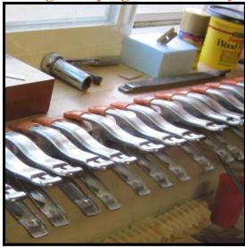
**Step 39:** Have your set of key spring clamps ready to use. Either two or three clamps per note will be required, depending on the method used. Both methods will be explained.
