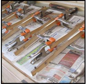
**Step 53:** Once the clamps have been applied to each key, set the assembly aside for the glue to cure. If you have a limited number of clamps, I would recommend working until you run out, then leaving everything clamped up at least an hour before continuing. Ideally, a set of either 104 clamps, or 156 clamps (for 3 to a note) would allow you to finish the entire set, then leave all 52 notes clamped to cure overnight.
