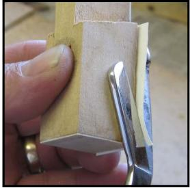
**Step 36:** Hold your curved nose scissors (Cat. No. 164) so that you cut the excess fabric of the wafer along the side of the keystick. It is important that the inside edge of the scissor run along the wood of the keystick, as shown. Once you've done the side, trim the front edge as well.
