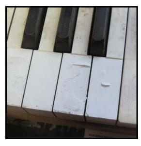
**Step 9:** With the ivory heads removed, the keystick itself will need further preparation. In many vintage pianos a linen backing was used between the ivory and the keystick. Before the ivories are reglued, this backing needs to be removed, even if the fabric is in perfect condition. Leaving the fabric on would result in the keytop being too high in comparison to the tail.
