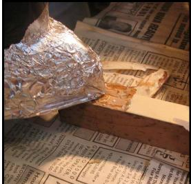
**Step 15:** For adhesive of such tenacious nature, try a direct application of heat to soften the substance, but don't be surprised if this is ineffective. (Be sure to cover your iron with foil to avoid a transference of the adhesive from the keystick to the surface of the iron.)
