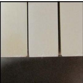
Hint: By eye-balling the fronts of the keys as you go, you can avoid oversanding. As you get close to an even line of keytops, check with a straight edge.
