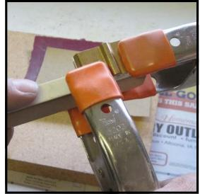
**Step 50:** Apply a second clamp as shown, this time tilting it slightly from side to side so that the bottom jaw is again further back than the top jaw.
