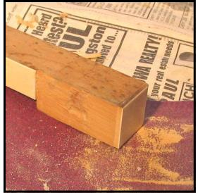
**Step 18:** At this point, ascertain the condition of the keystick. A bit of roughness is tolerable, but a missing chunk of wood such as is visible in the photo (notice the key is turned side-ways), needs to be filled.
