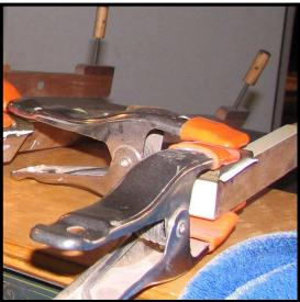
**Step 52:** If any error in positioning is discovered, remove the clamps, quickly reheat the brass plate, then reclamp with whatever corrections are necessary.
