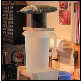
The upshot of all of this is that, unless I'm missing something here, using cement wafers in combination with brass plates works well <u>if</u> the plates are heated, but not well at all if the plates are cold, especially when used for shorter times. By heating the plates, good adhesion is achieved after as short of time as an hour. Thus, the procedure would be feasible in the field, if done before a tuning.
