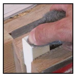
**Step 57:** Next, place the keytop in your vise to clean the front. Use 0000 steel wool (Cat. No. 412-4/0) if only a light cleaning is necessary. If heavy cleaning is needed, start with 400 grit paper, followed by steel wool.
