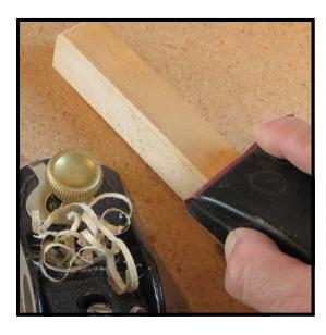
**Step 25:** Finish the procedure by using a small block plane (Cat. No. MF-33) to shave off the bulk of the excess, then by sanding the sides of the cap flush with the original keystick. (*Note: Refer to catalog for picture of actual plane.*)
