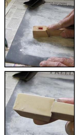
**Step 60:** Place the grits of sandpaper you are going to use face up on your bench, and sand the ivory by holding the keystick face down as shown. If unevenness between the head and tail exist, start with 400 or 500 grit, and sand until the joint is smooth. Then switch to the 800 grit paper to remove the sanding marks of the coarser paper.
