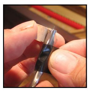
**Step 13:** A depth gauge for your drill bit should be made. I would recommend using tape instead of a store-bought metal depth gauge. The tape will be less likely to mar the finish of the plate. Either masking tape or electrical tape works well for the job.
