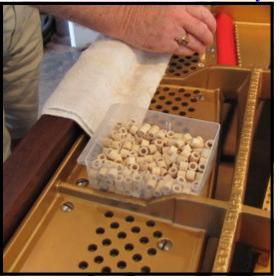
**Step 9:** Have a container of the correct size of bushings close by the work area. Drape a towel over the front of the stretcher while you work to avoid scratching or bumping the finish.
