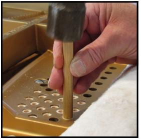
**Step 11:** Finish tapping each bushing in using a wooden punch the same diameter as the bushings.
