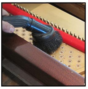
**Step 16:** Once the set of bushings has been drilled, finish the job by vacuuming up the work area in preparation for the next step in the restoration process.
