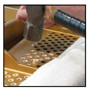
**Step 10:** Start each bushing by lining up the bushing with the hole, then rapping it once or twice with a ball peen hammer (Cat. No. MF-1916). Make sure that the bushing is going in straight.
