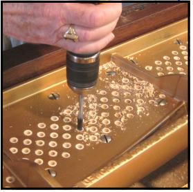
**Step 14:** Quickly drill each hole. An in and out motion with the drill following a pattern as you work will make short work of the process.
