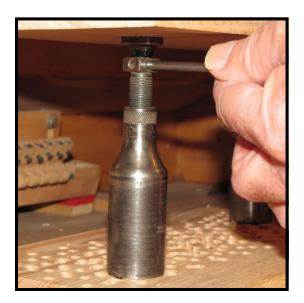
**Step 7:** Use a piece of hardwood above and below the jacks to even out the pressure. Turn the screw of the jacks up until the pinblock is firmly supported.
