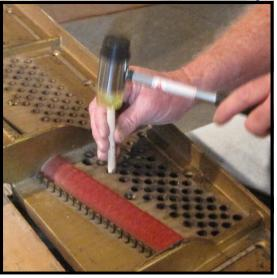
**Step 4:** Each bushing should pop loose with one or two good taps of the mallet.
