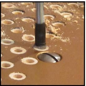
Caution: Refresh the tape often during the operation to avoid having it bunch up, thus throwing the depth of the cut off. If you drill too deeply, your drill bit will be down into the pinblock, possibly enlarging the top of the hole slightly. In this photo, it can be seen that the tape is beginning to bunch up and should be replaced.
