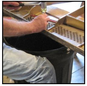
**Step 3:** By sitting on a stool, you should be able to pull yourself up to a handy distance from the plate to work. Tap the bushings out into the waste basket using a mallet and a wooden punch.
